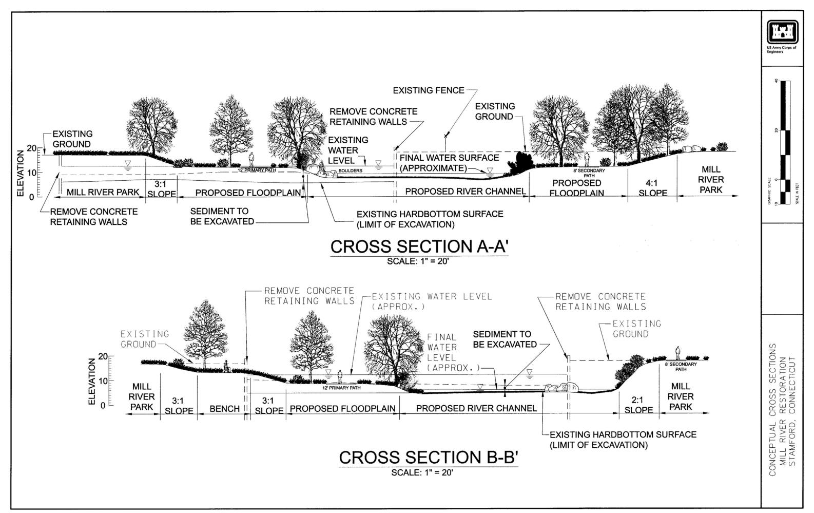
Figure 19. Cross Sections of Proposed Restoration and Dam Removal within Mill River Park (See Figure 15 for locations of cross sections)
