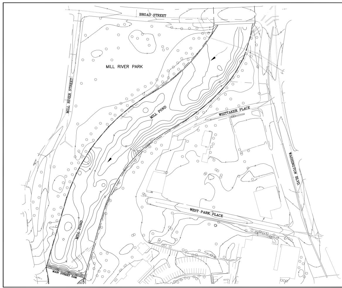
Figure 6. Bathymetric Survey of Mill Pond
