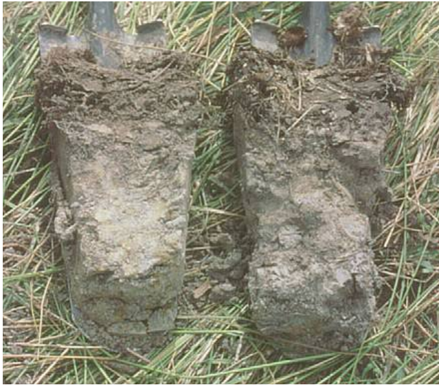
Figure 43.—The profile on the right is from a drained wetland adjacent to a ditch. The profile on the left is from an area not affected by the ditch. Both soils meet the requirements for indicators F3 (Depleted Matrix) and A11 (Depleted Below Dark Surface) and thus are hydric soils.
