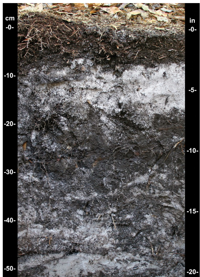
Figure 10.—Indicator A5 (Stratified Layers) in sandy material. This soil also meets the requirements of indicator A6 (Organic Bodies).
