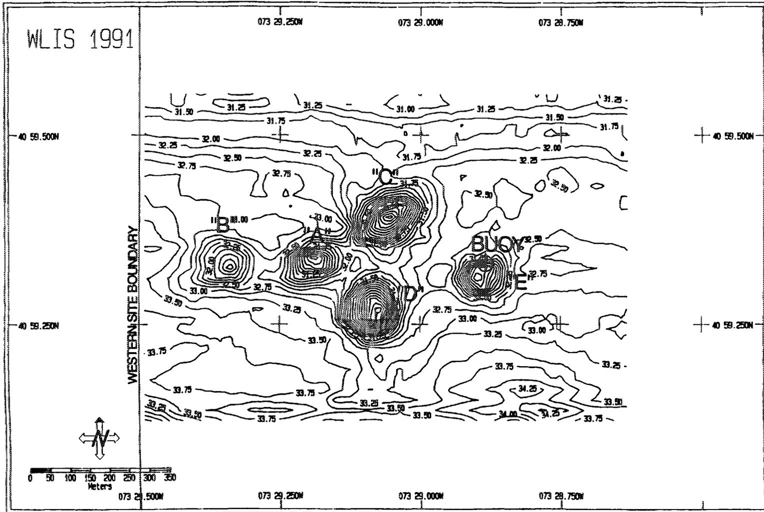
Figure 3-2. The June 1991 bathymetric contour plot of WLIS. Contours at 0.25 m intervals.
