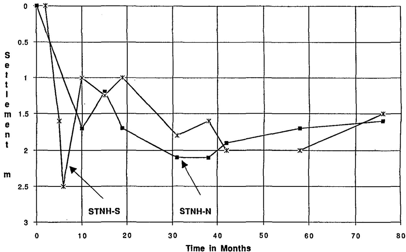
**Figure 4-1.** Rate of consolidation at the center of disposal mounds located at the Central Long Island Sound Disposal Site (CLIS). Note that substantial consolidation of sediments continued in the 4 - 5 months following termination of disposal and long-term increase of mound height (possibly due to ambient sedimentation; Poindexter-Rollins 1990).
