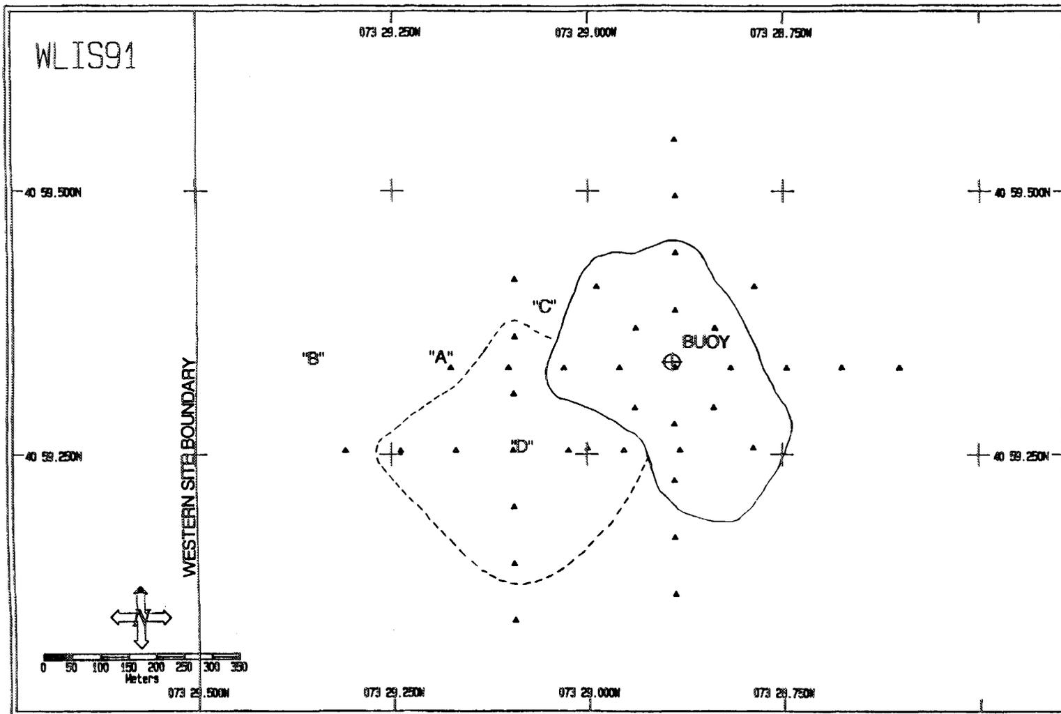
Figure 3-5. The mapped distribution of dredged material deposited during the 1990-1991 disposal season (solid line) based on REMOTS® sediment-profile photography and acoustically observed changes in depth. This material is adjacent to and overlaps some sections of the dredged material footprint developed during the 1989-1990 disposal season (dashed line).
