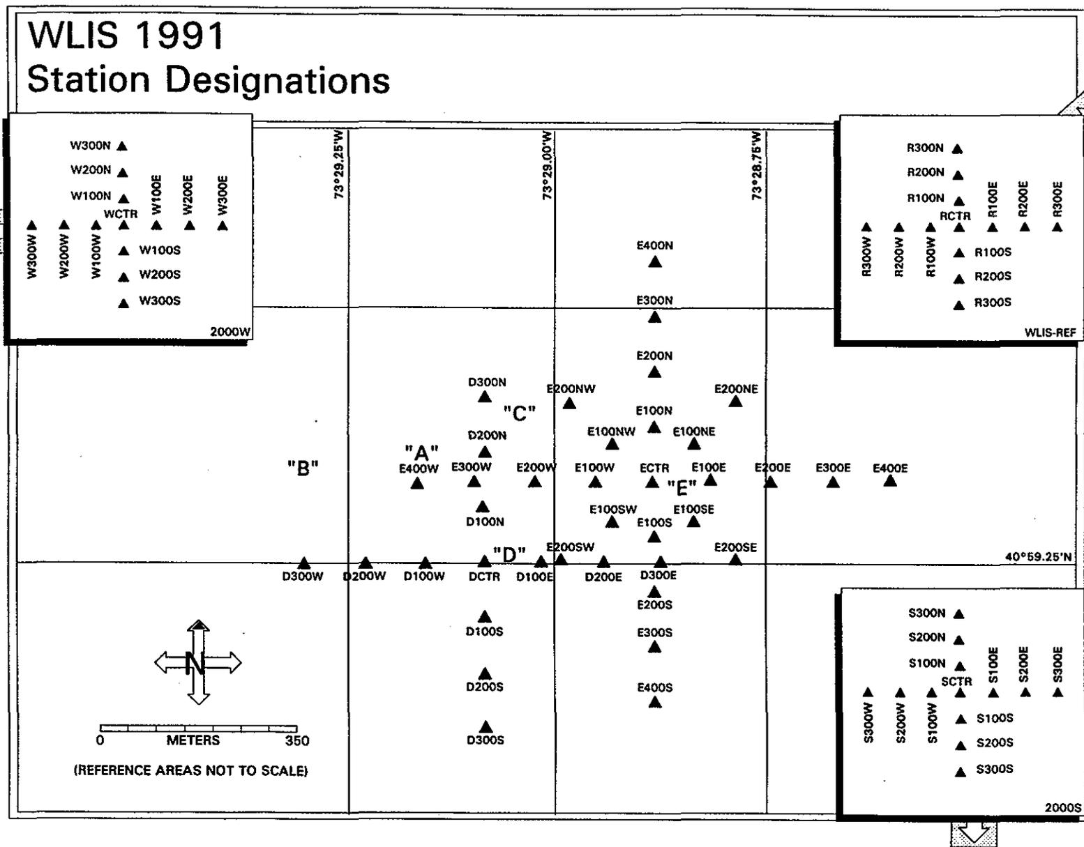
**Figure 2-1.** Locations and designations of the REMOTS<sup>®</sup> stations at WLIS and reference areas, June 1991. Thirteen-station cross-shaped grids with 100 m spacing were used at the three outlying reference areas (200W, 2000S, and WLIS-REF).
