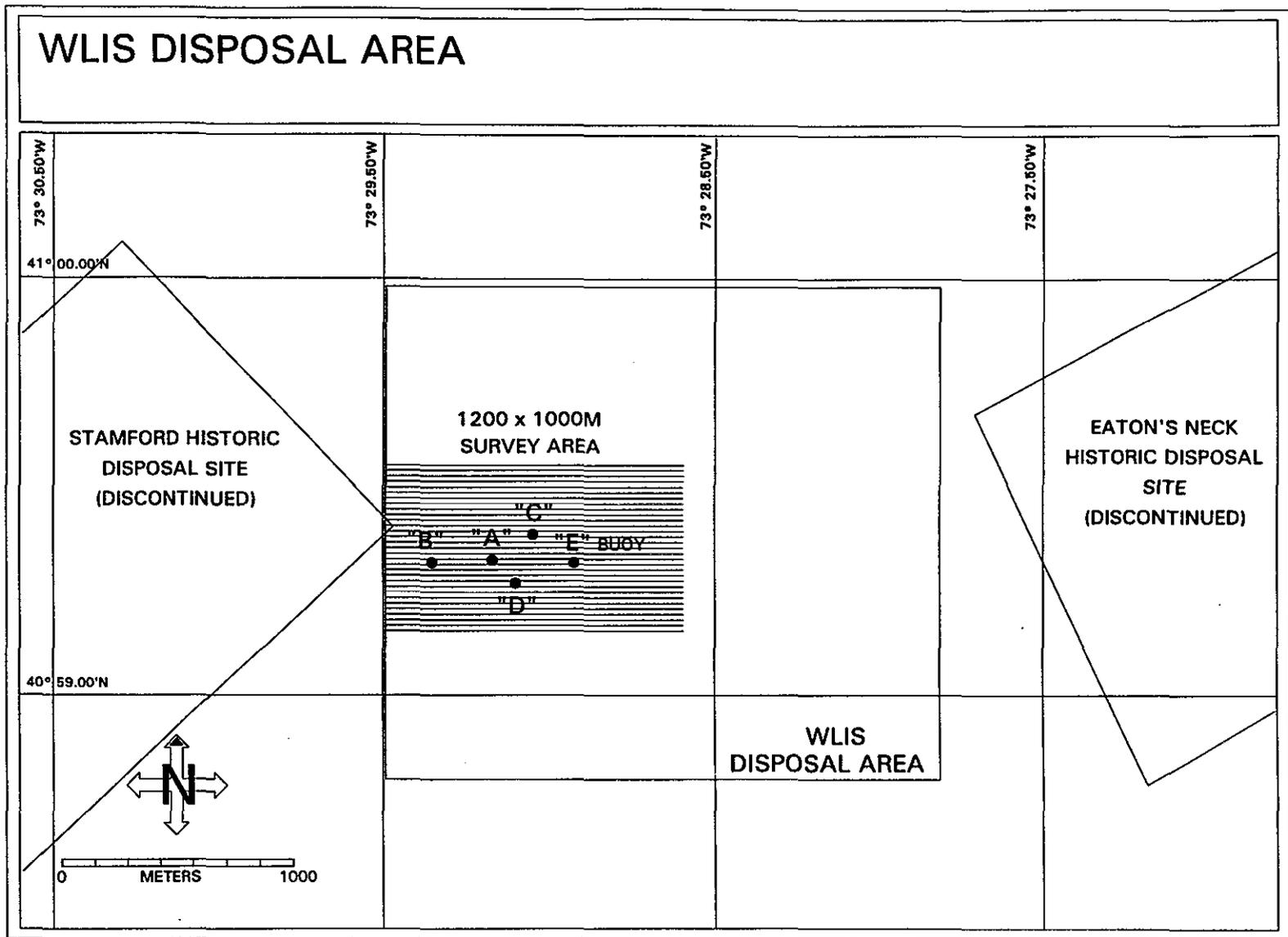
**Figure 1-2.** The WLIS 1991 bathymetric survey grid. The discontinued Stamford and Eaton's Neck Disposal Sites border WLIS to the west and east. The buoy location ("E") for disposal operations during the 1990-1991 disposal season is also shown.
