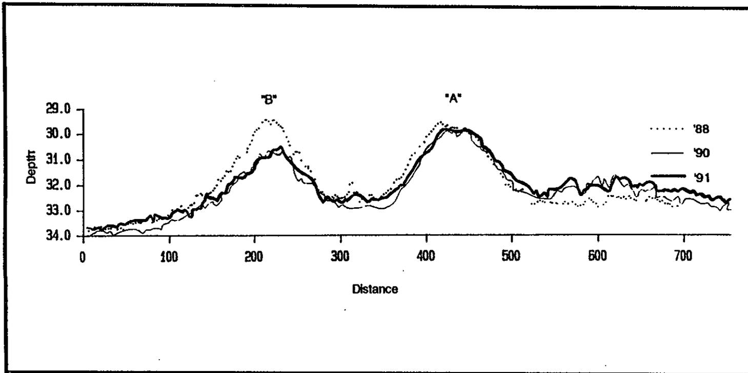
**Figure 4-2.** Overlays of the 1988, 1990, and 1991 depth profile plots from lane 18 of the bathymetric survey grid. The 1.0 m decrease in the WLIS "B" mound height observed during the 1990 bathymetric survey was attributed largely to mound consolidation.
