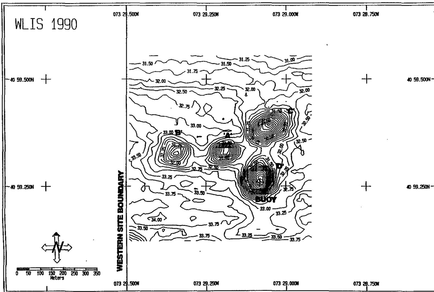
Figure 3-1. The July 1990 bathymetric contour plot of WLIS. Contours at 0.25 m intervals.
