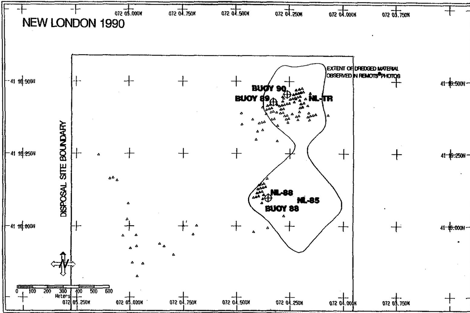
**Figure 4-3.** Plot of reported barge disposal positions (LORAN-C) between October 1988 and June 1990. Contour line delimits extent of dredged material observed in REMOTS® photographs. The nineteen points scattered to the southwest represent the reported disposal positions of the M/V *Nancy G*. We believe these positions do not represent the actual disposal locations which were reported to be near Buoy 90.
