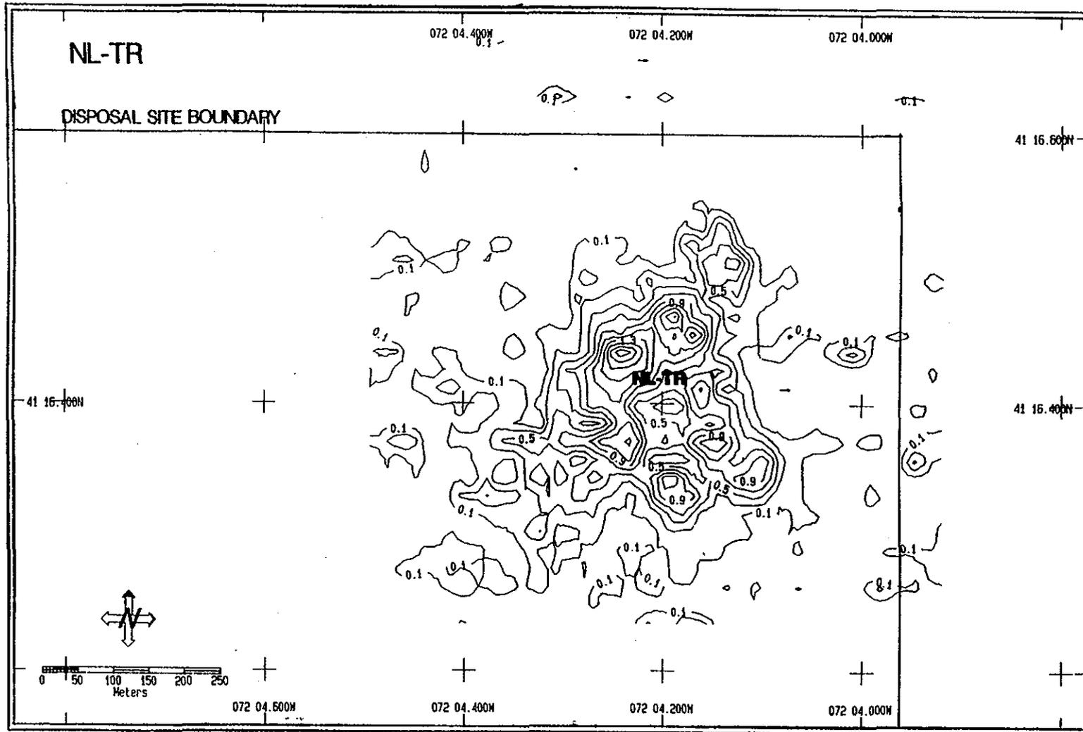
Figure 3-4. Depth difference (in meters) contour map based on comparison of the August 1988 and July 1990 precision bathymetric surveys in the vicinity of the NL-TR mound, New London Disposal Site
