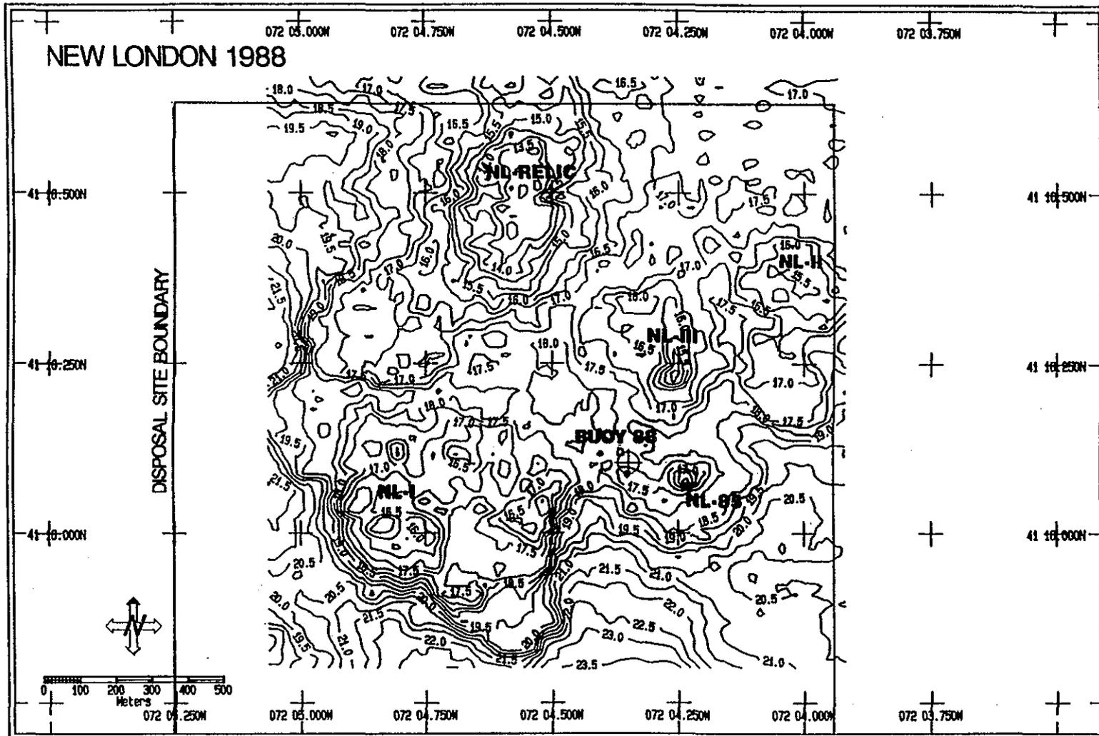
Figure 3-1. Contoured bathymetric chart of the New London Disposal Site (depths in meters) with relic disposal mounds and buoy position, August 1988
