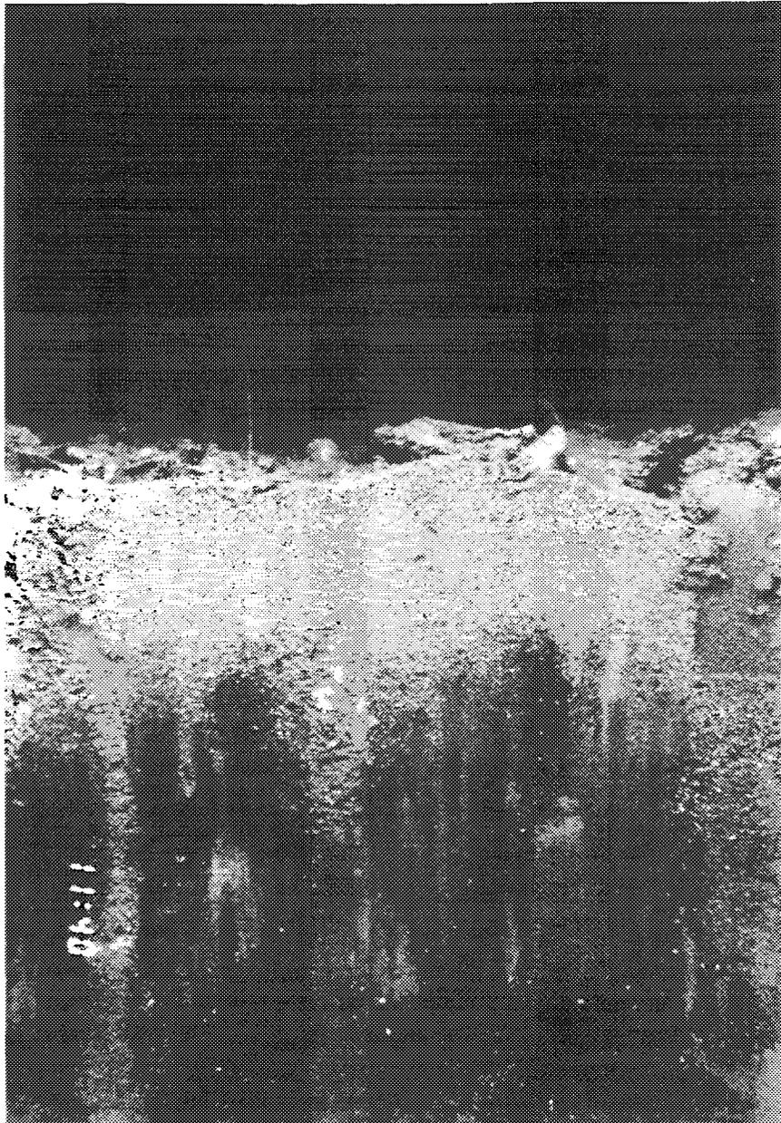
**Figure 3-8.** REMOTS® photograph at NL-85, Station N300N, showing poorly sorted sands overlying muds
