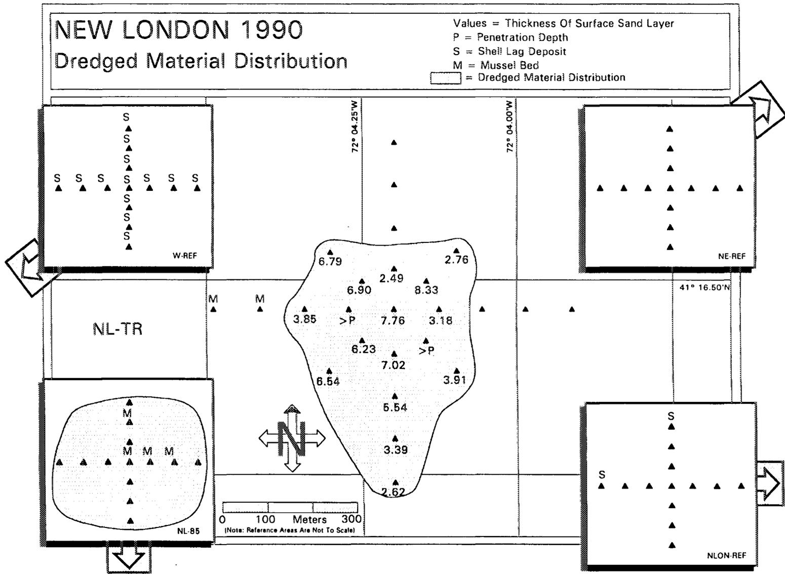
Figure 3-7. Distribution map of dredged material, surface sand thickness, and unique station characteristics at the New London Disposal Site and reference stations
