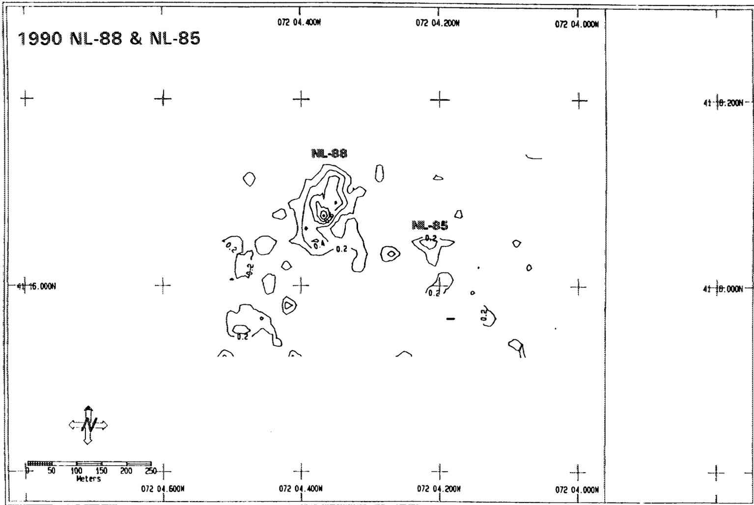
Figure 3-5. Depth difference (in meters) contour map based on comparison of the August 1988 and July 1990 precision bathymetric surveys in the vicinity of the NL-88 and NL-85 mounds, New London Disposal Site
