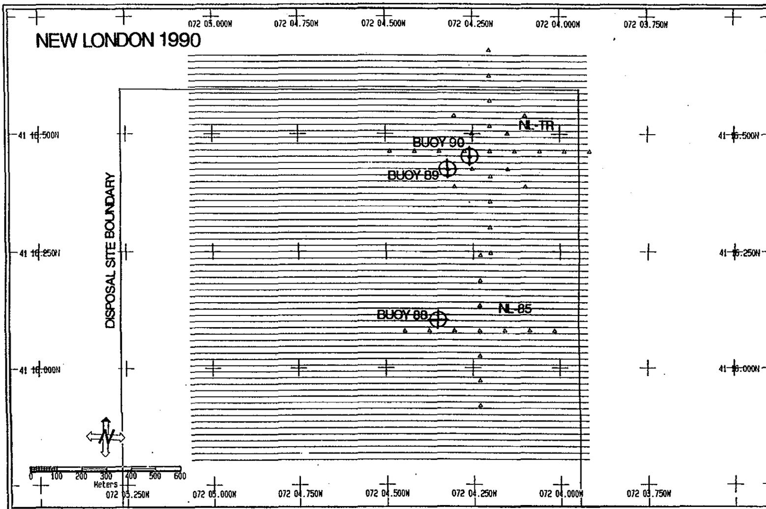
Figure 1-2. Map of New London Disposal Site precision bathymetric survey lanes and REMOTS® survey grid occupied in 1990
