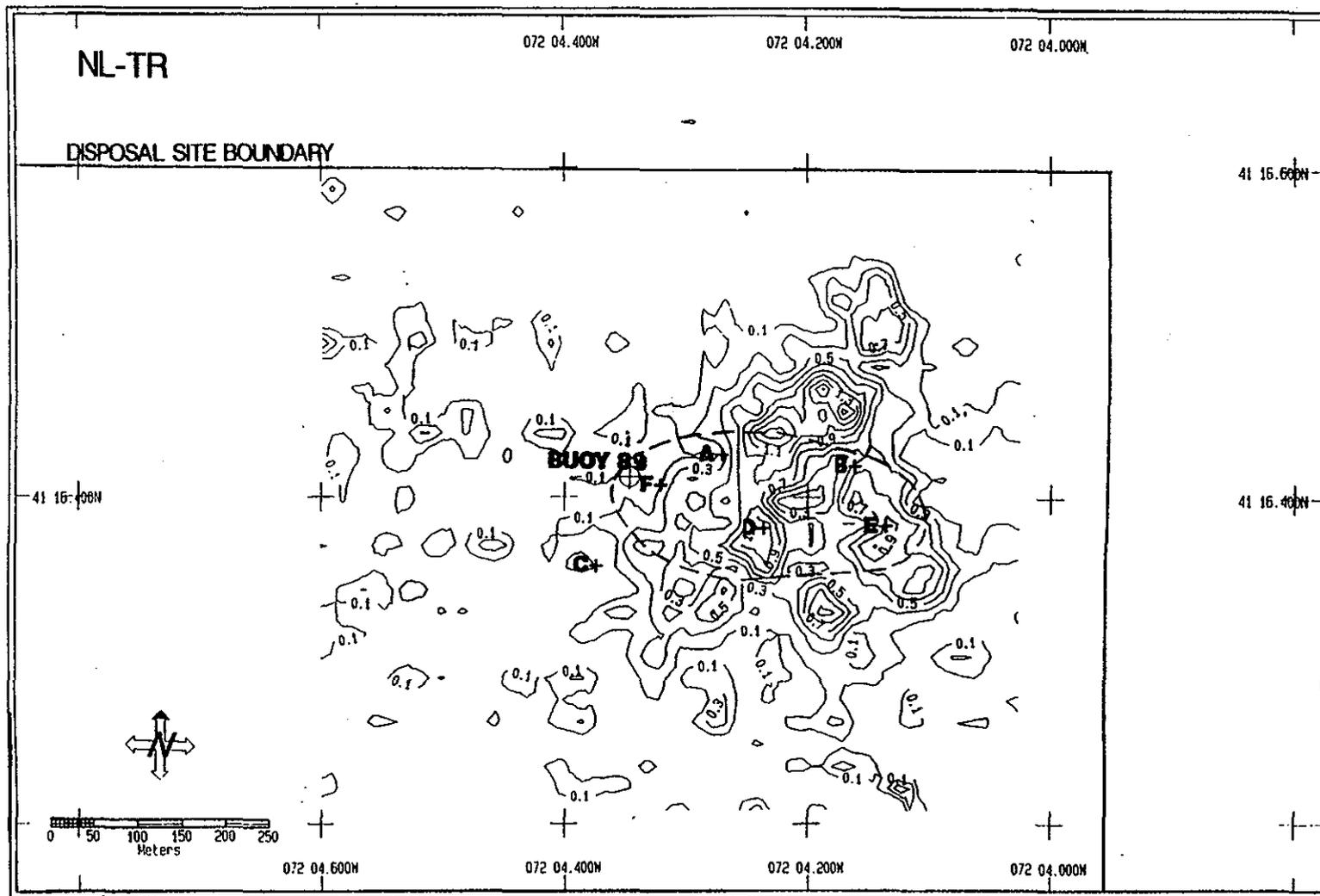
Figure 4-2. Depth difference contour plot (depth in meters) of the Thames Shipyard and Repair Company disposal location (NL-TR) showing the distribution of cap material deposited between October 1988 and July 1990. Positions mark the intended disposal points listed in Table 1-1. Dashed line indicates areal extent of underlying dredged material initially deposited at this location.
