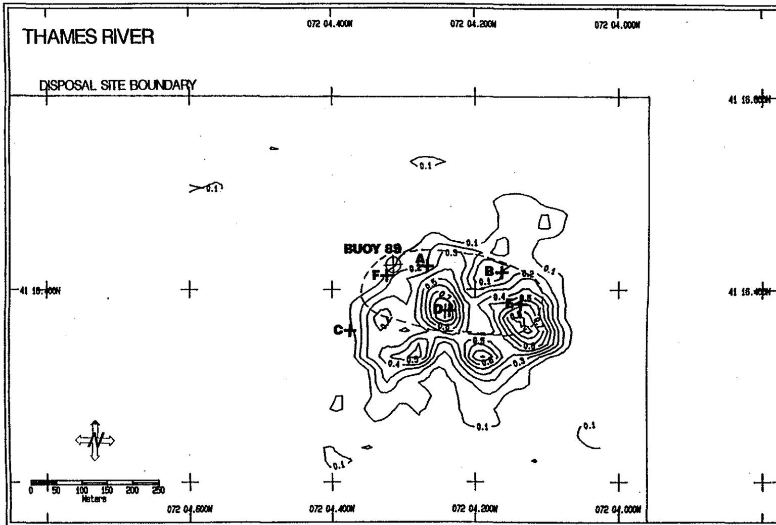
Figure 4-1. Depth difference contour plot of the Thames Shipyard and Repair Company disposal location (NL-TR, depth in meters) showing the distribution of cap material deposited between October 1988 and February 1989. Dashed line indicates areal extent of underlying dredged material initially deposited at this location.
