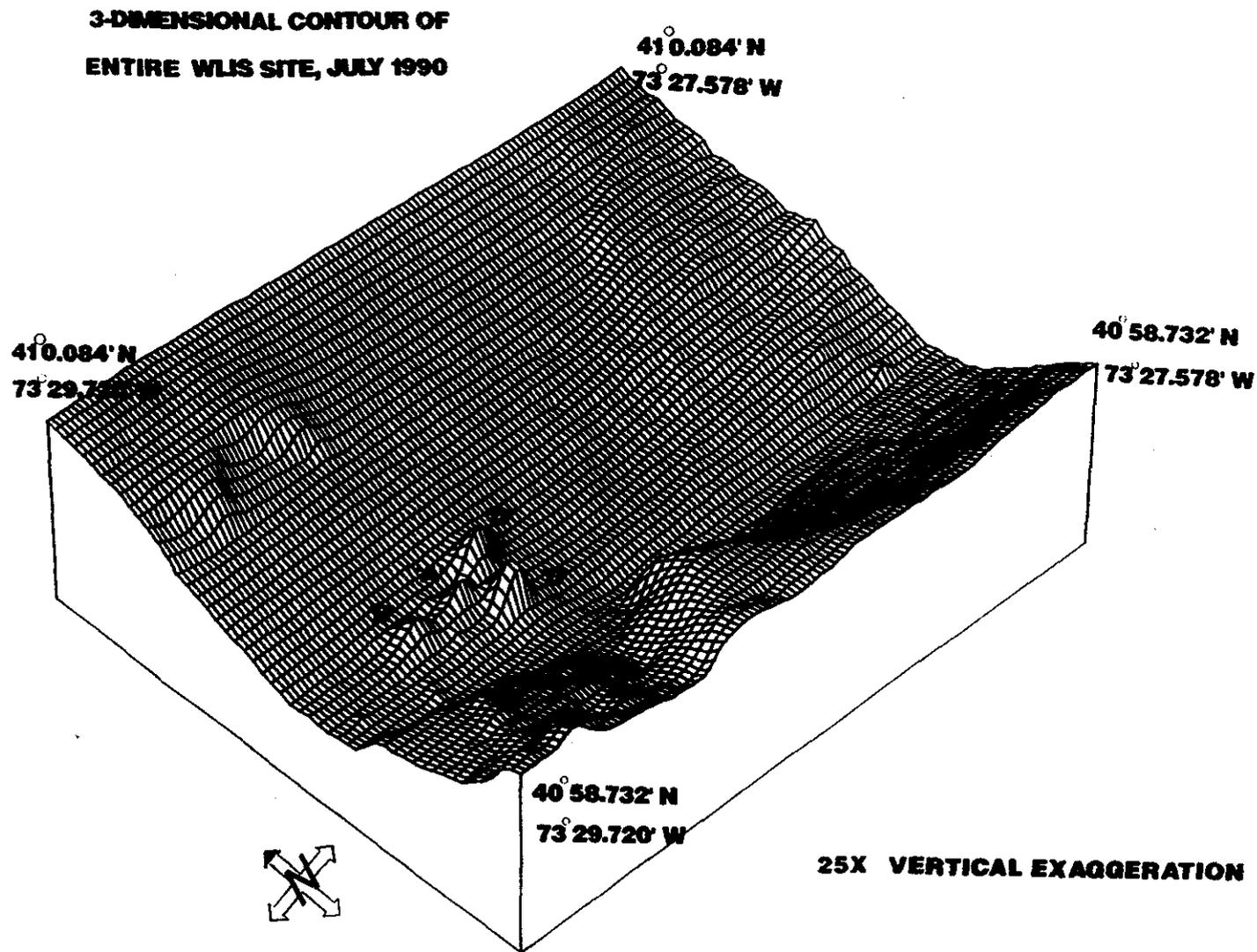
Figure 3-7. Three dimensional bathymetric plot of the WLIS Disposal Site, July 1990. The "A", "B", "C", and "D" disposal mounds are visible in the lower central portion of the plot.
