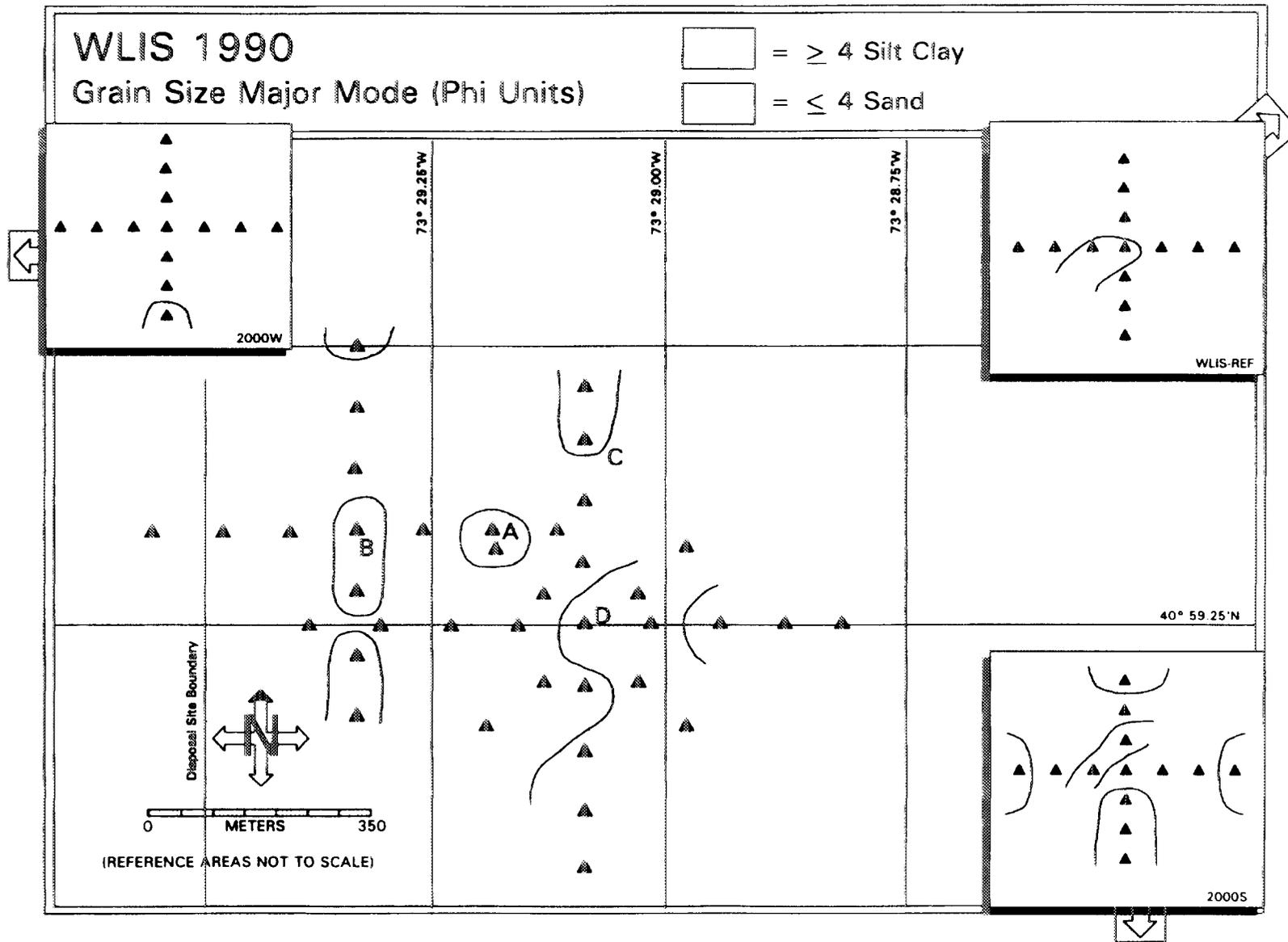
**Figure 3-11.** Distribution of sediment grain size major mode (phi units) at the WLIS Disposal Site and reference stations, July 1990. Contours delineate regions where grain size major mode (in phi units) was 4-3 phi or less.
