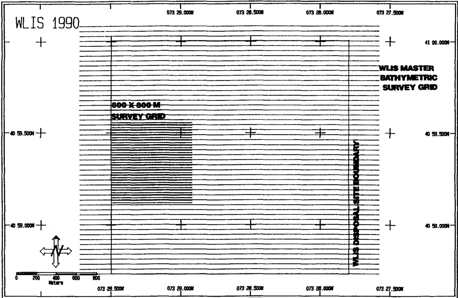
Figure 2-1. The 800 X 800 m and 3000 X 2500 m bathymetric survey lanes at WLIS, July 1990.
