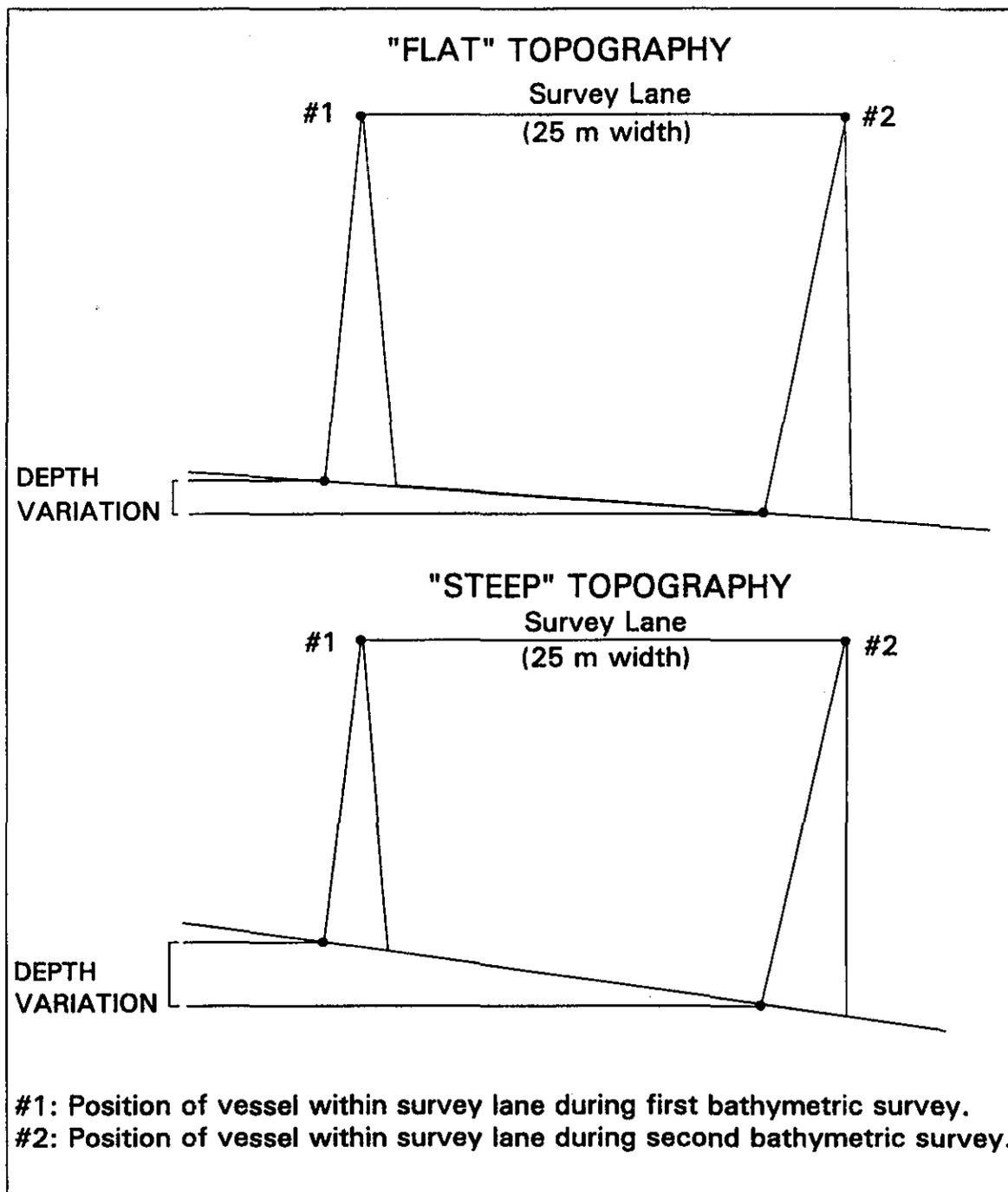
**Figure 4-2.** Possible variation in recorded depths within a bathymetric survey lane can increase with sloped topographies.
