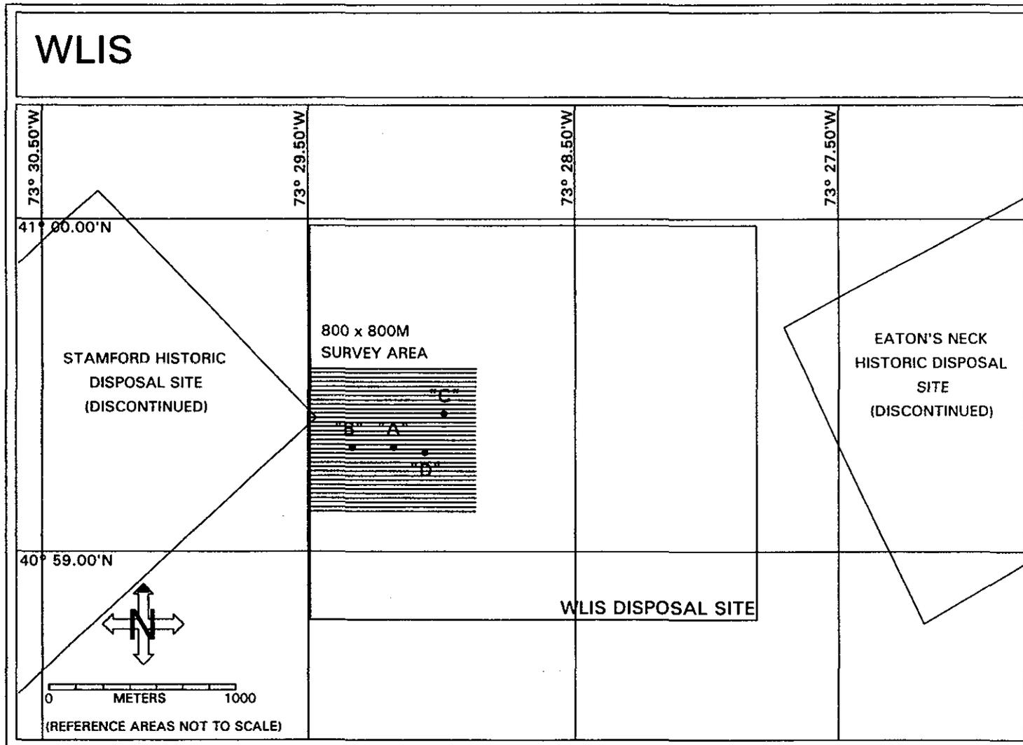
**Figure 1-1.** The Western Long Island Sound (WLIS) Disposal Site showing 800 X 800 bathymetric survey lanes and the location of the four disposal mounds ("A", "B", "C", and "D") near the western site boundary.
