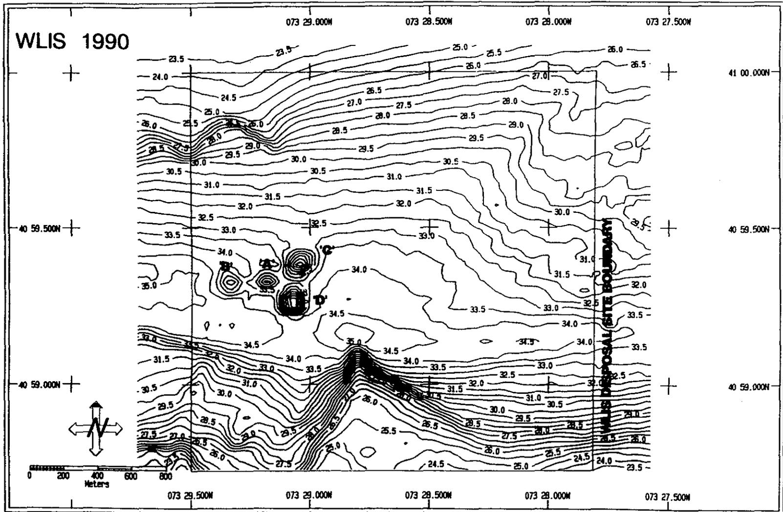
Figure 3-6. Bathymetric contour plot of the WLIS Disposal Site, July 1990. The four disposal mounds ("A", "B", "C", and "D") are clearly visible in the central, western region. The WLIS site boundary is also indicated. Contours at 0.5 m intervals.
