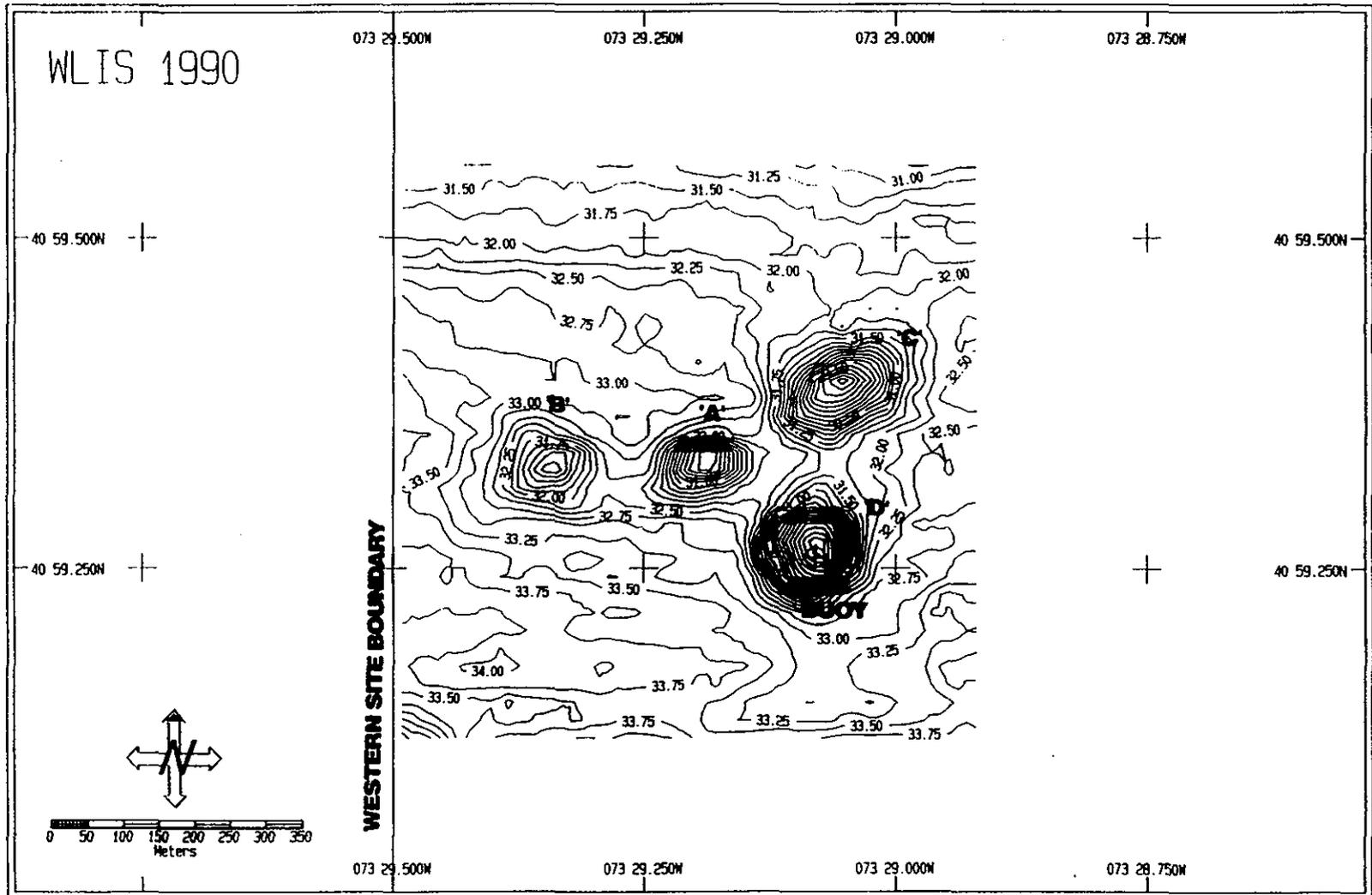
**Figure 3-2.** Bathymetric contour chart of the WLIS Disposal Site, July 1990, showing the "A", "B", "C", and "D" disposal mounds. The location of the disposal buoy during the 1989 - 1990 season is also indicated. Contours at 0.25 m intervals.
