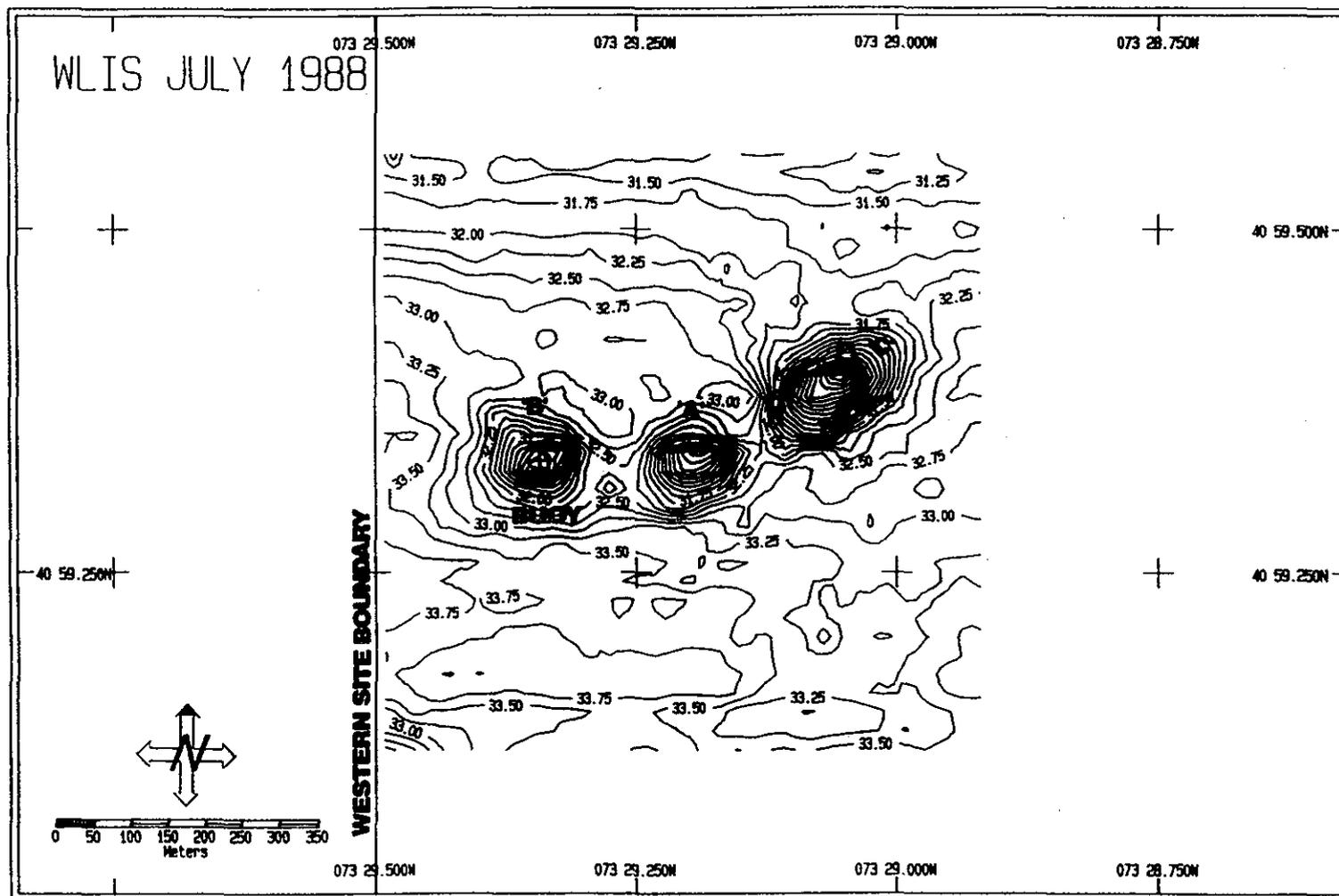
**Figure 3-1.** Bathymetric contour chart of the WLIS Disposal Site, July 1988, showing the "A", "B", and "C" disposal mounds. The location of the disposal buoy during the 1987 - 1988 season is also indicated. Contours at 0.25 m intervals.
