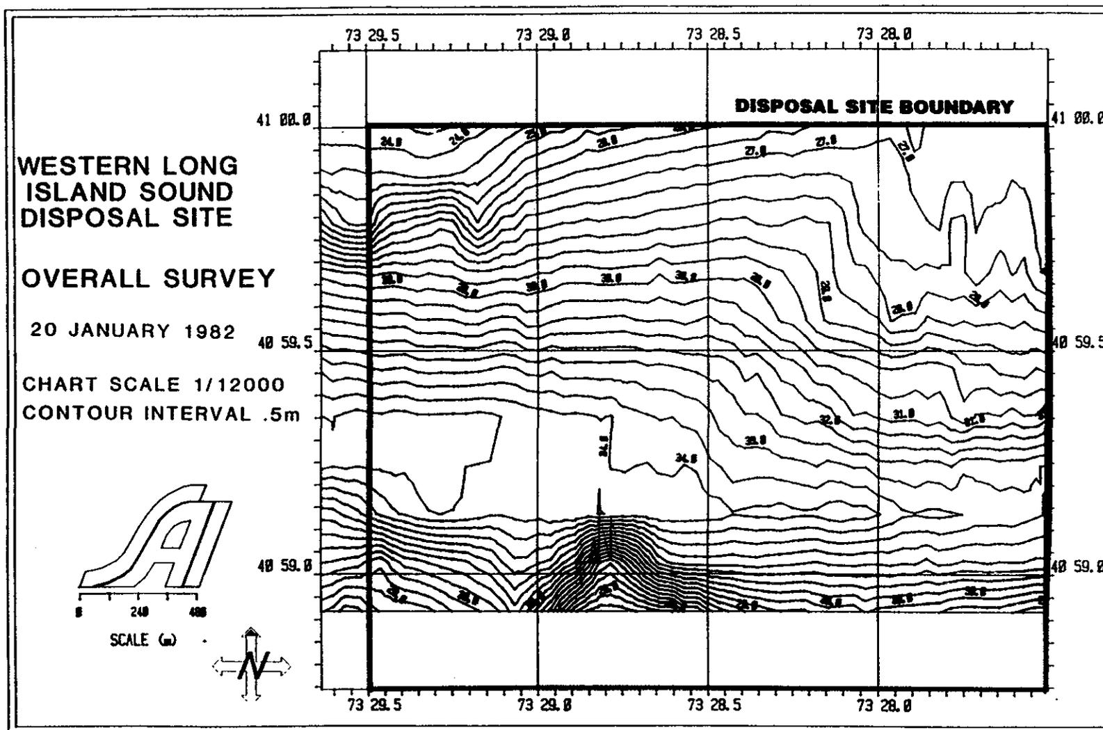
Figure 3-5. Bathymetric contour plot of the WLIS Disposal Site, January 1982. The southern site boundary extends below this plot. Contours at 0.5 m intervals.
