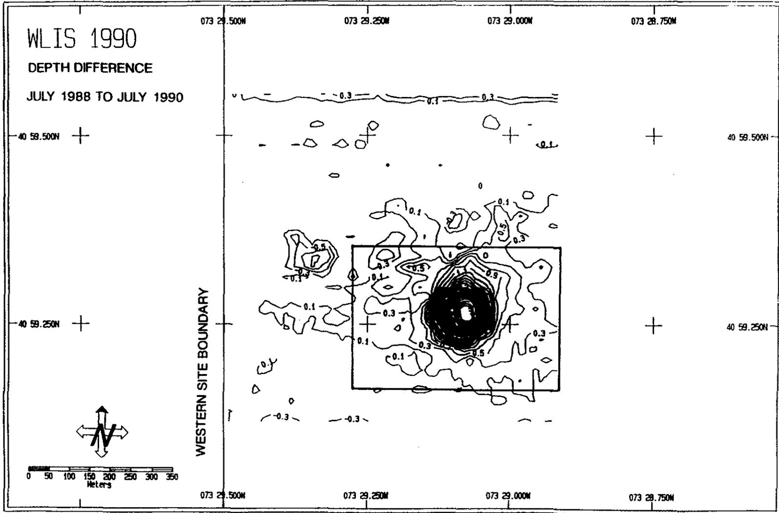
Figure 3-3. Depth difference contour plot at WLIS, July 1990. Boundaries surrounding the WLIS "D" mound delineate the 500 X 350 m region used to calculate the volume of accumulated dredged material based on depth difference analysis. Contours at 0.2 m intervals.
