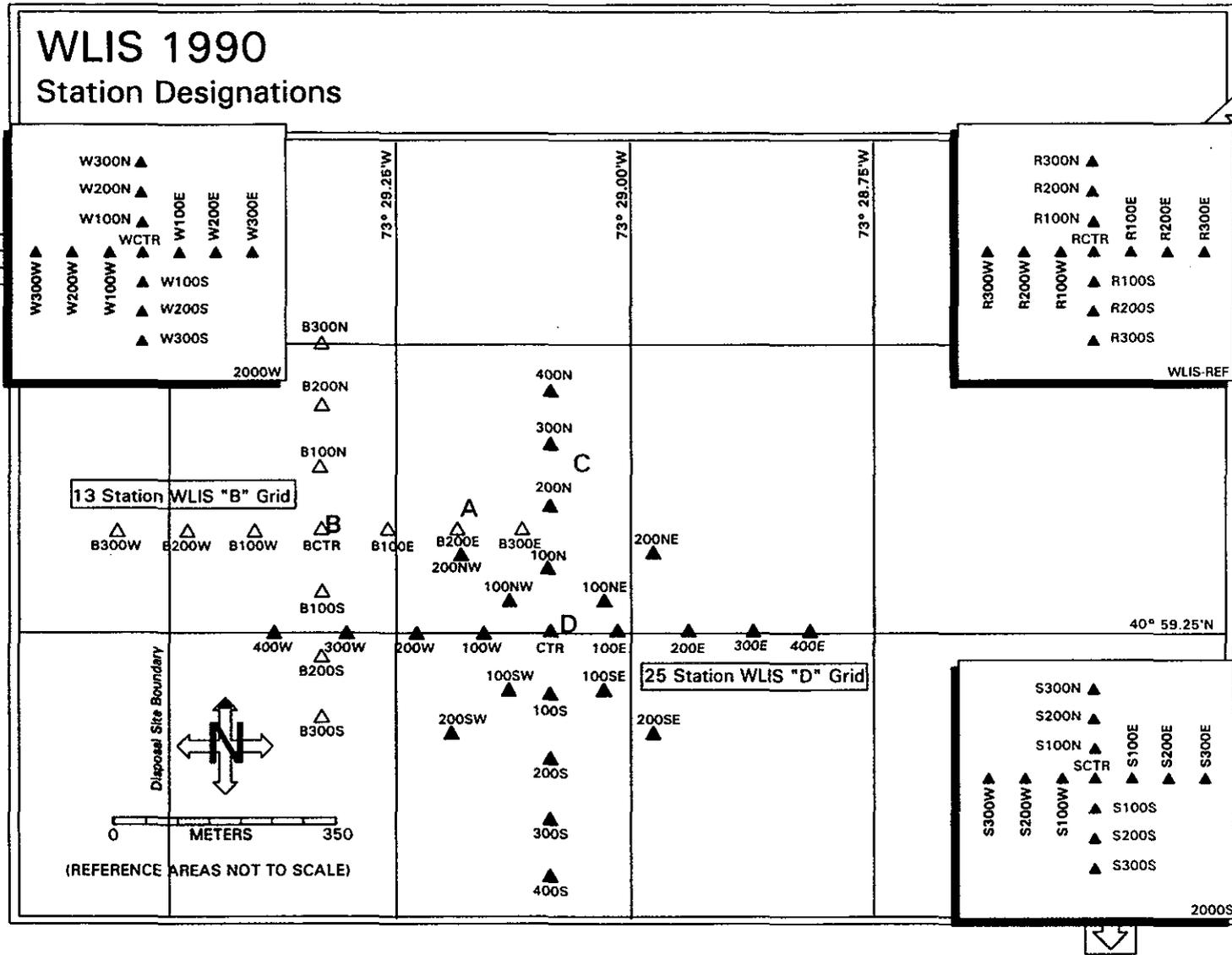
**Figure 2-2.** Locations and designations of the WLIS "D" and "B" REMOTS® stations at the WLIS Disposal Site, July 1990. Cross-shaped grids with 100 m spacing were used at the three outlying reference areas 2000W, 2000S, and WLIS-REF). The locations of the "A", "B", "C", and "D" mounds are also indicated.
