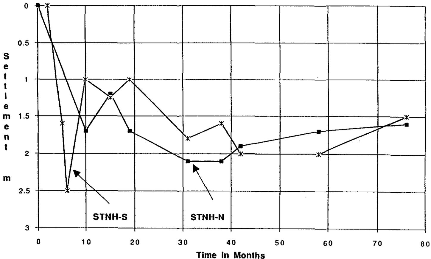
**Figure 4-1.** Time rate of consolidation at the center of disposal mounds located at the Central Long Island Sound (CLIS) Disposal Site. Note that substantial consolidation of sediments likely continued in the 4 - 5 months following discontinuation of disposal. (From Poindexter-Rollins, 1990).
