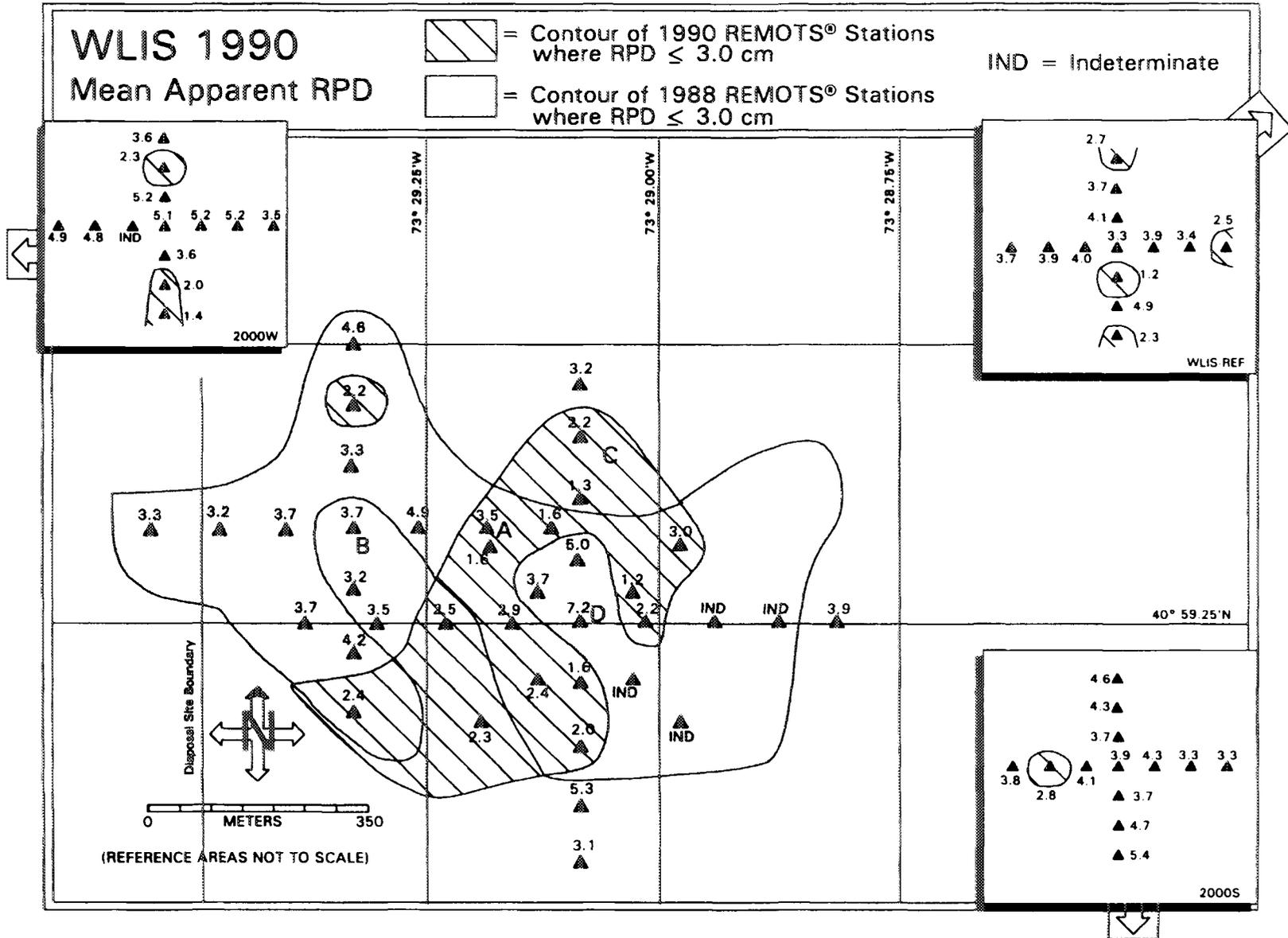
**Figure 3-16.** Mapped distribution of mean RPD depths at on-site and reference stations, WLIS Disposal Site, July 1990, with overlay of 1988 on-site data. Contours delineate areas where average RPD was ≤ 3.0 cm. IND = indeterminate due to camera over-penetration.
