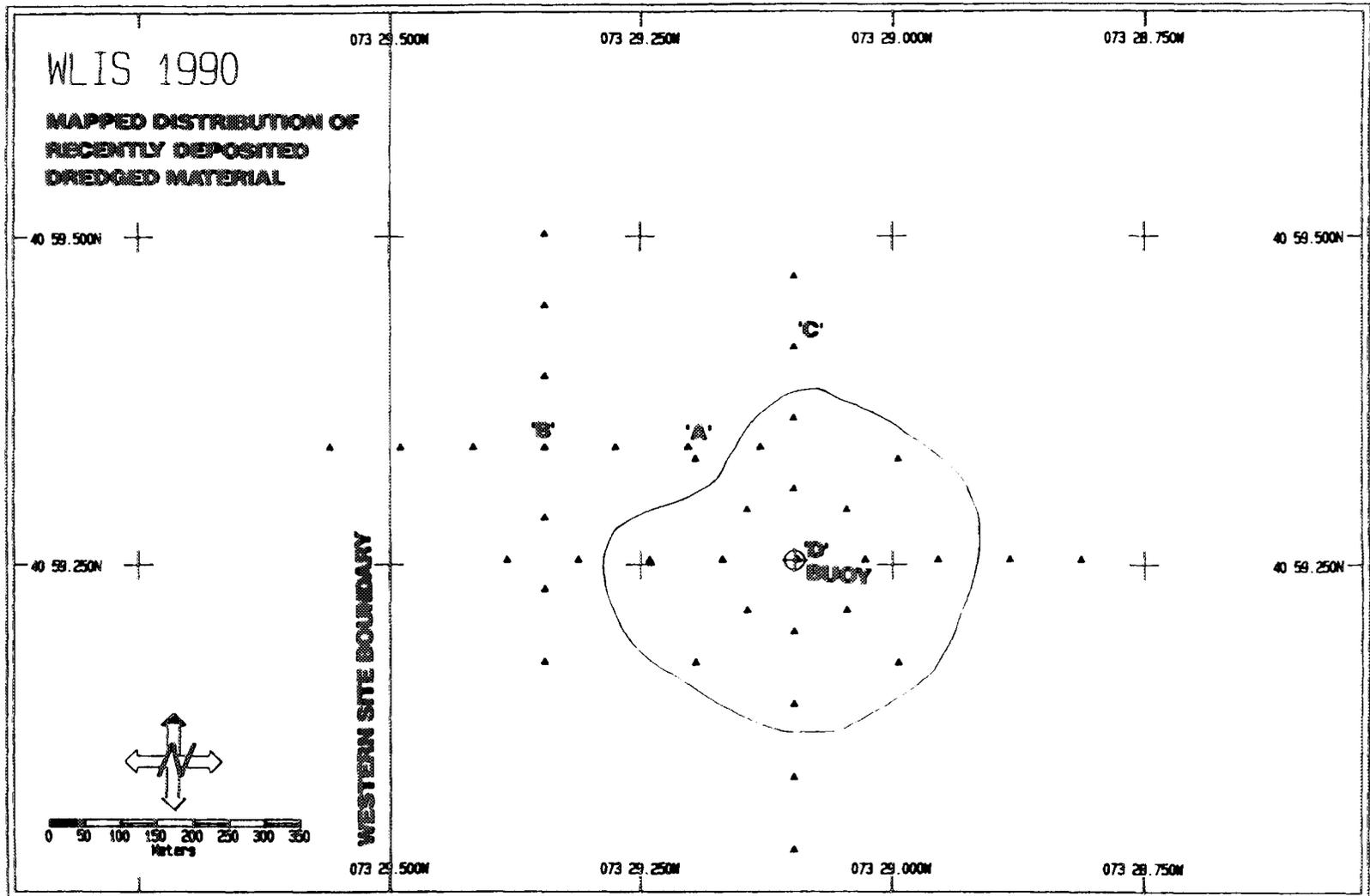
Figure 3-8. The mapped distribution of recently-deposited dredged material (between the July 1988 and July 1990 surveys) based on 1990 REMOTS® sediment-profile survey at the WLIS Disposal Site, July 1990.
