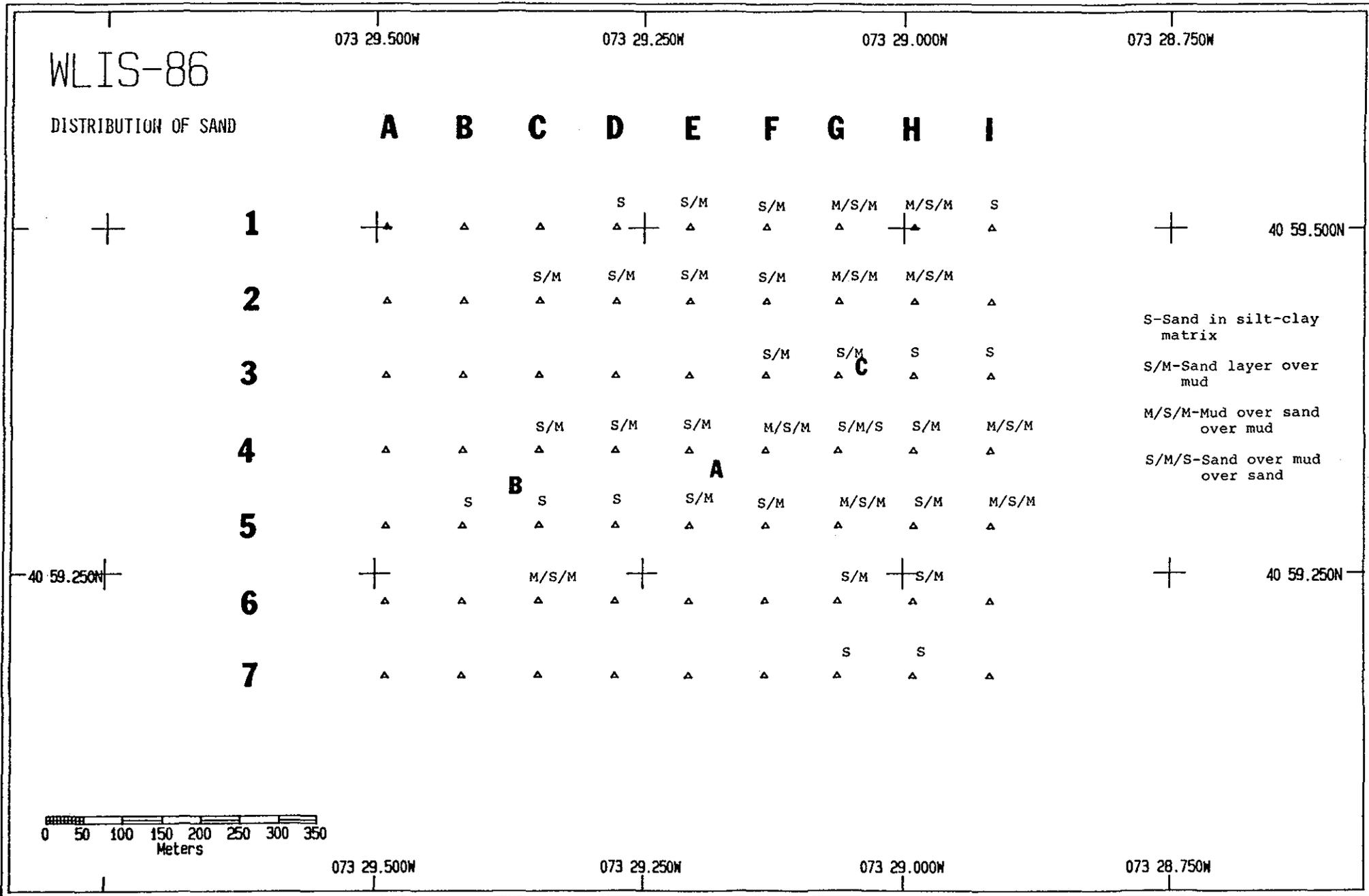
Figure 3-4. The distribution of sand and sand layers in the survey area.
