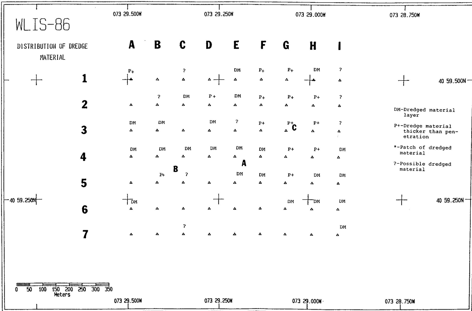
Figure 3-6. The distribution of dredged material in the WLIS survey area.
