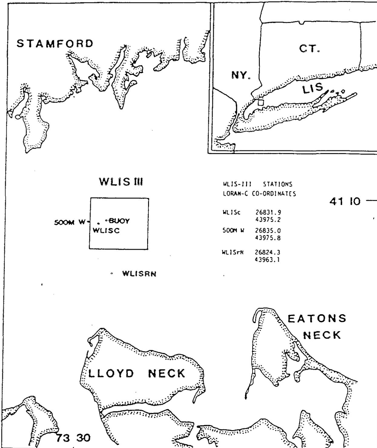
Figure 1. The Western Long Island Sound (WLIS) disposal site depicting the locations of three mussel monitoring platforms at WLISC, 500 MW and WLISrN, as well as the disposal buoy.
