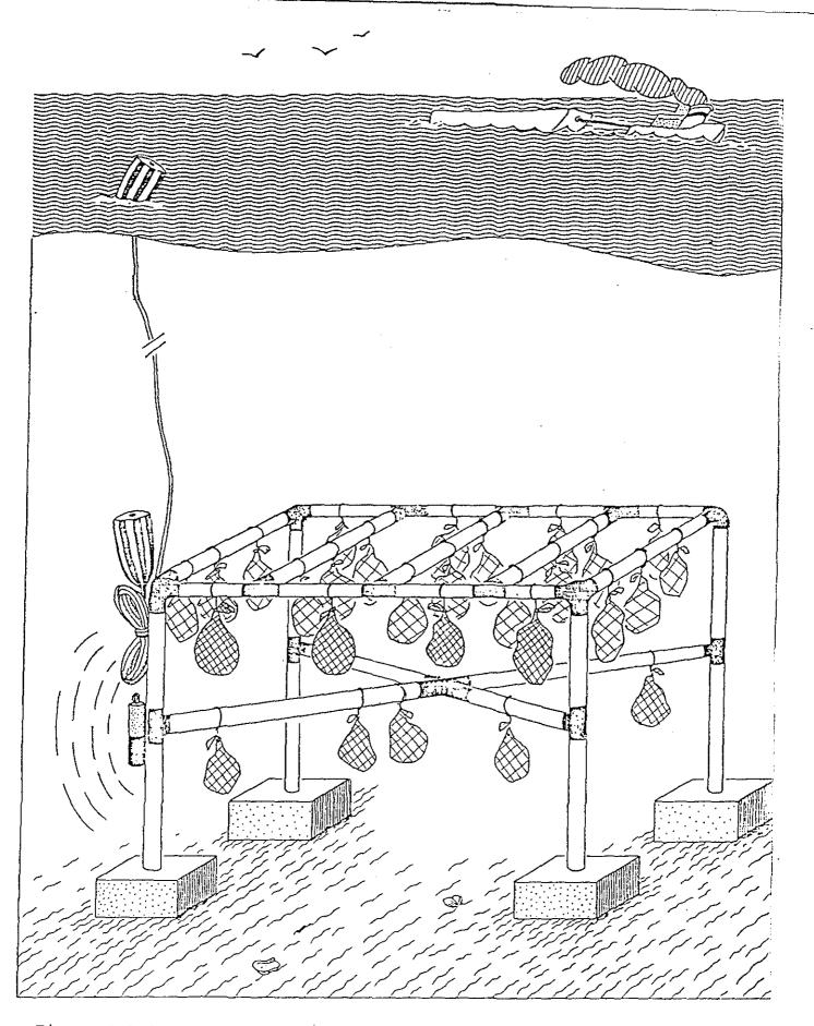
Figure 2.1-2. PVC platform used in maintaining shellfish at various monitoring stations.
