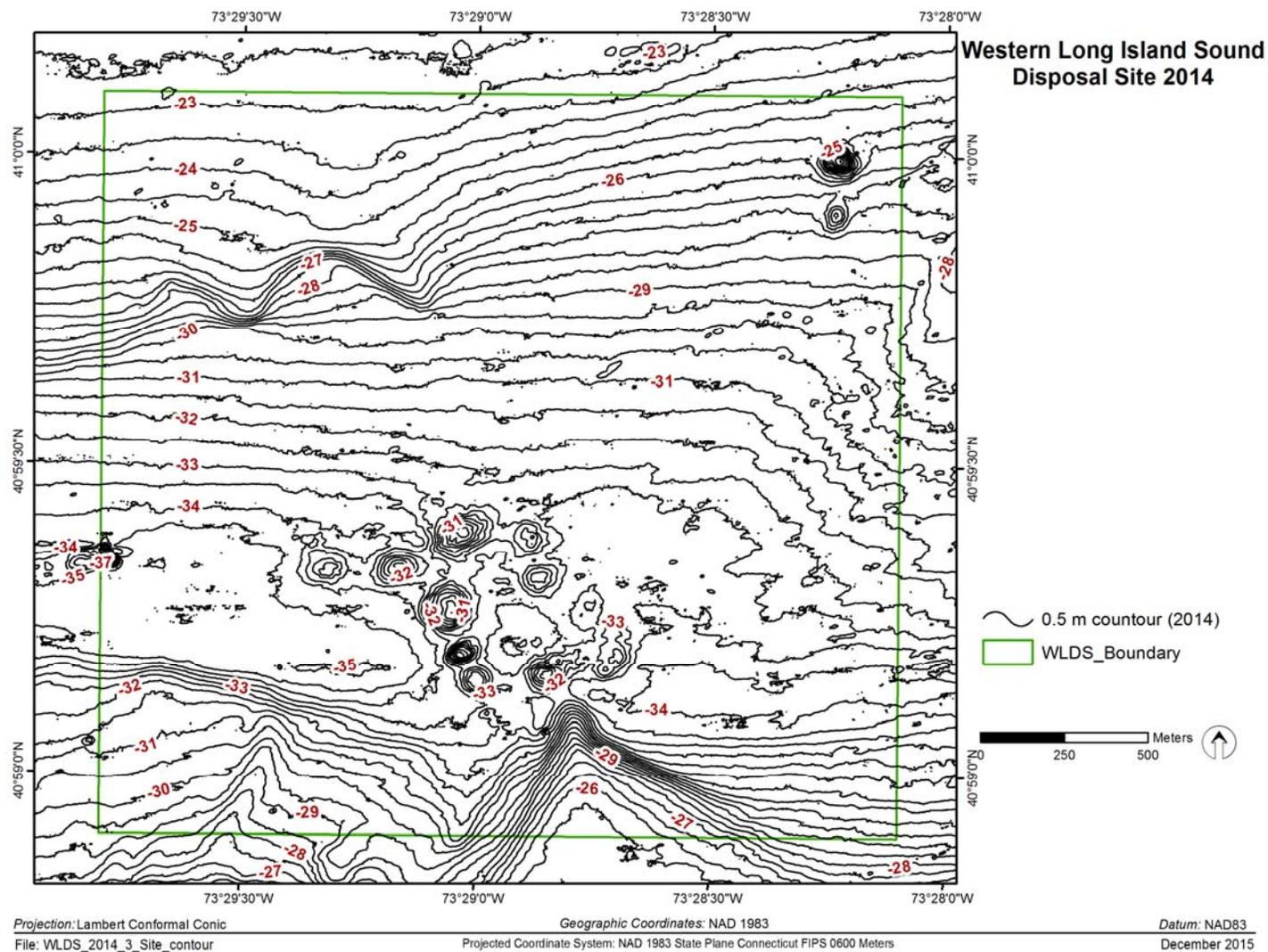
**Figure 3-1.** Bathymetric contour map of WLDS – August 2014
