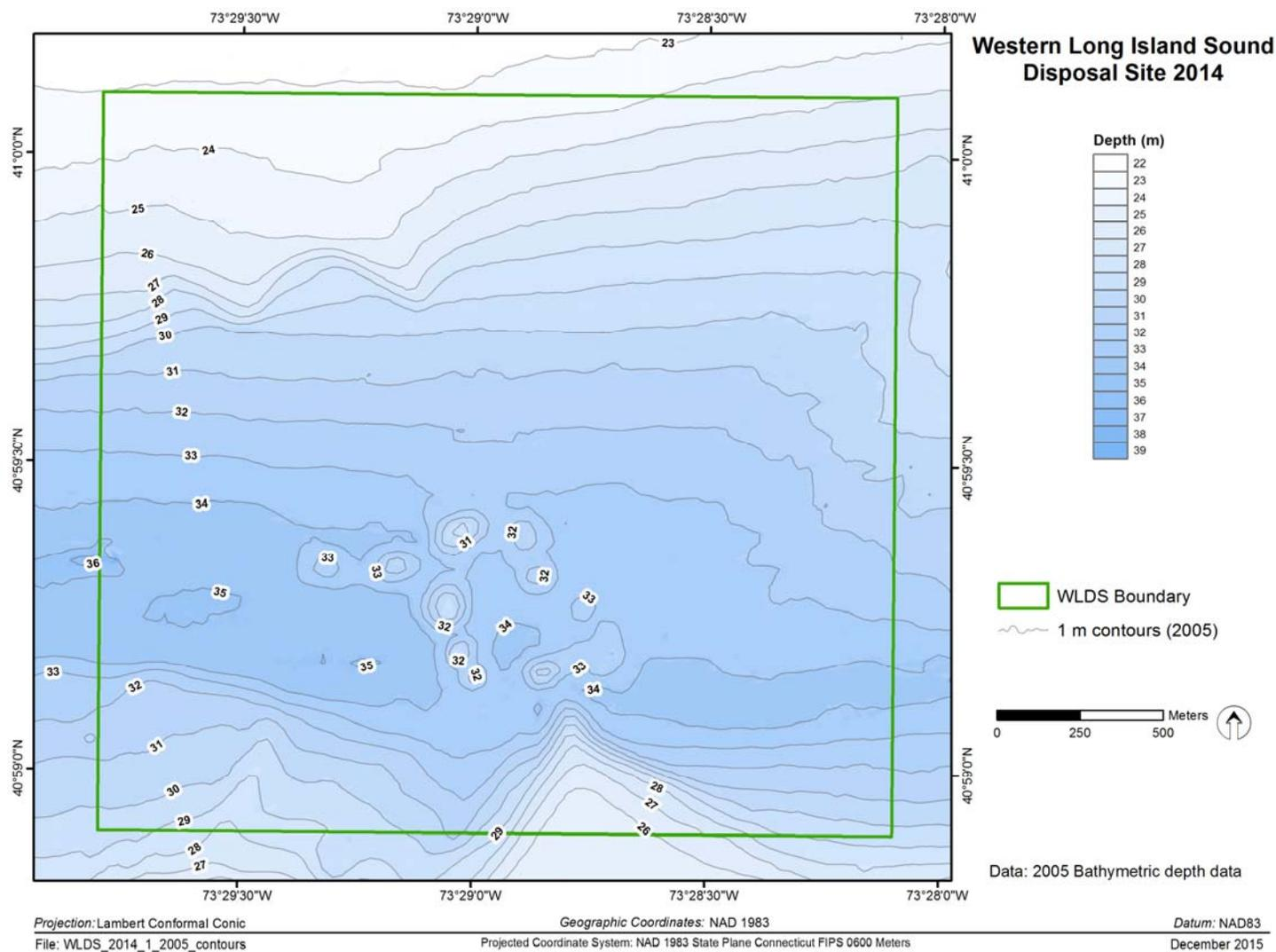
**Figure 1-3.** Bathymetric contour map of WLDS survey area, July 2005 (1-m contour interval)
