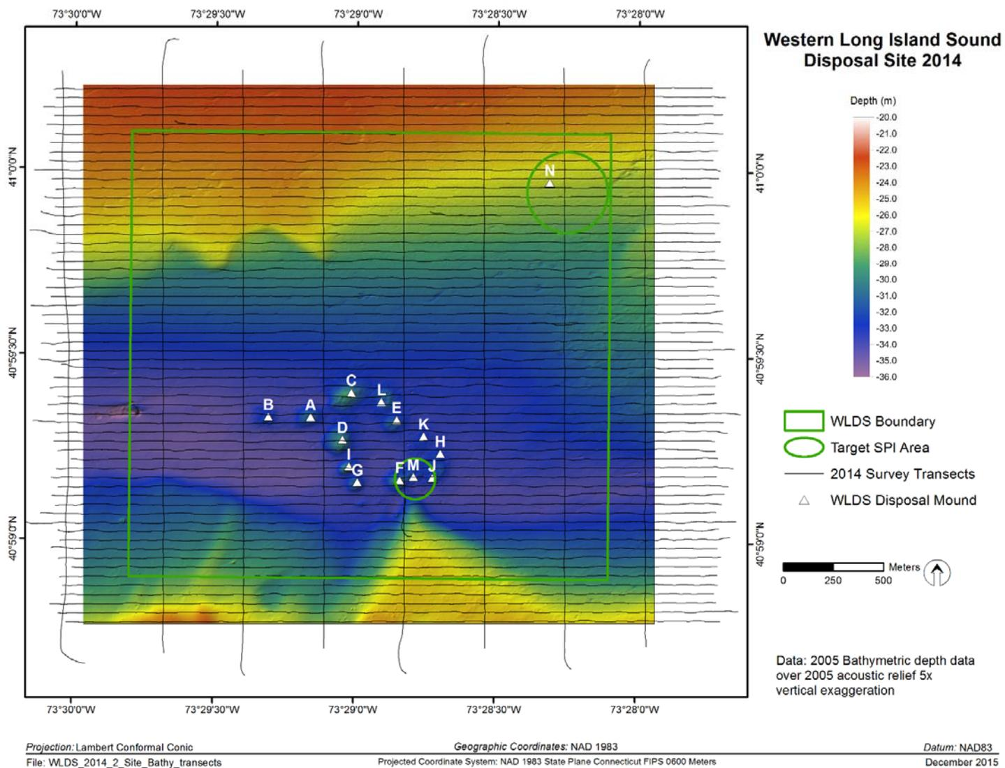
**Figure 2-1.** WLDS bathymetric survey area and tracklines
