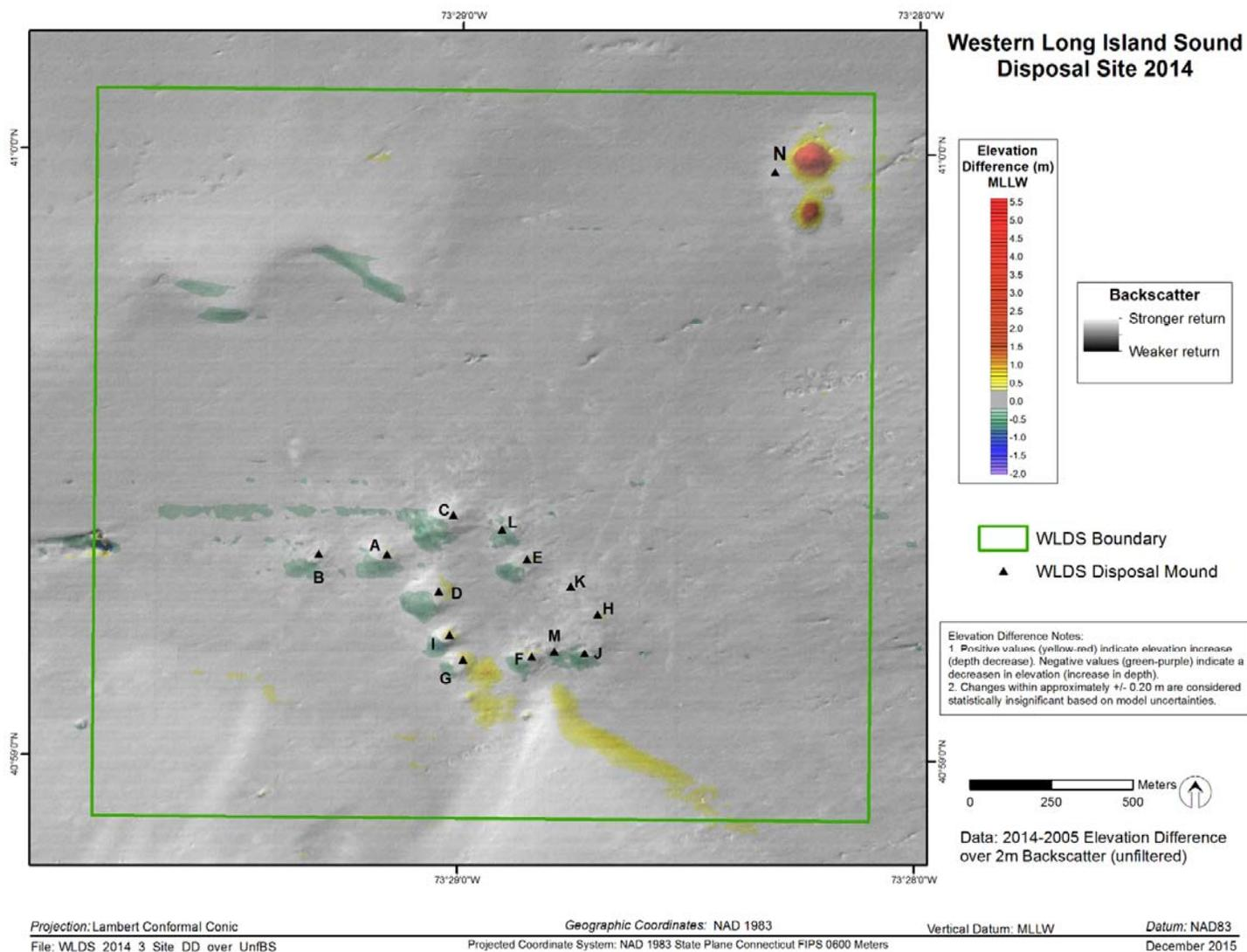
**Figure 4-2.** WLDS elevation difference 2005 vs. 2014 over unfiltered backscatter
