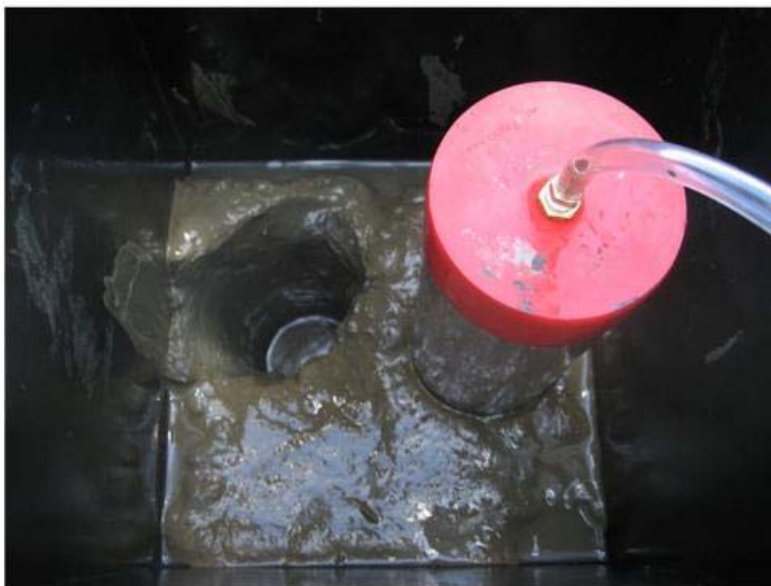
Figure 4-9: Box core with manually collected sub-core to capture minimally disturbed sediment water interface at the ambient stations
