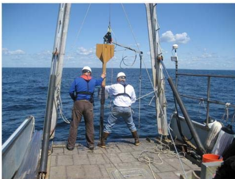
Figure 4-10: Piston core used to penetrate through the placed dredged material into the underlying ambient sediment
