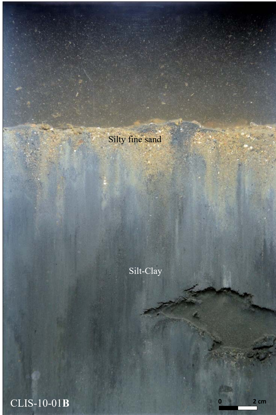
Figure 3-28. Profile image at CLIS-10-01 illustrating a thin surface layer of light brown fine sand followed by gray/black silt-clay
