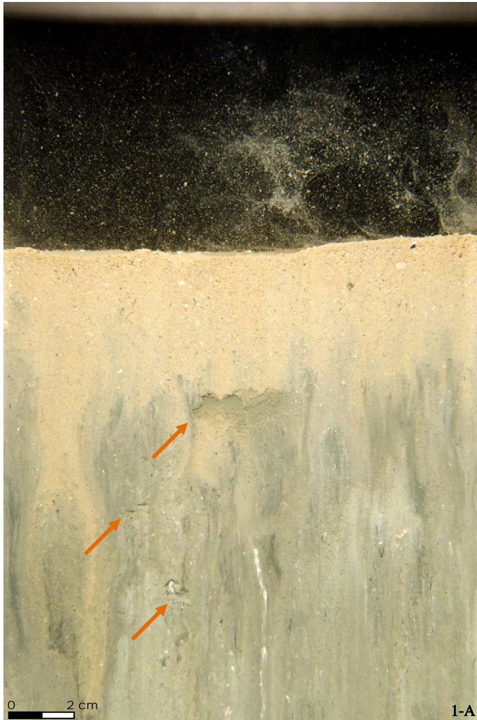
Figure 3-28. Sediment-profile image from Station 1, located in the deeper areas of the disposal site where the majority of the dredged material accumulated, showed active feeding voids (arrows) at depth.
