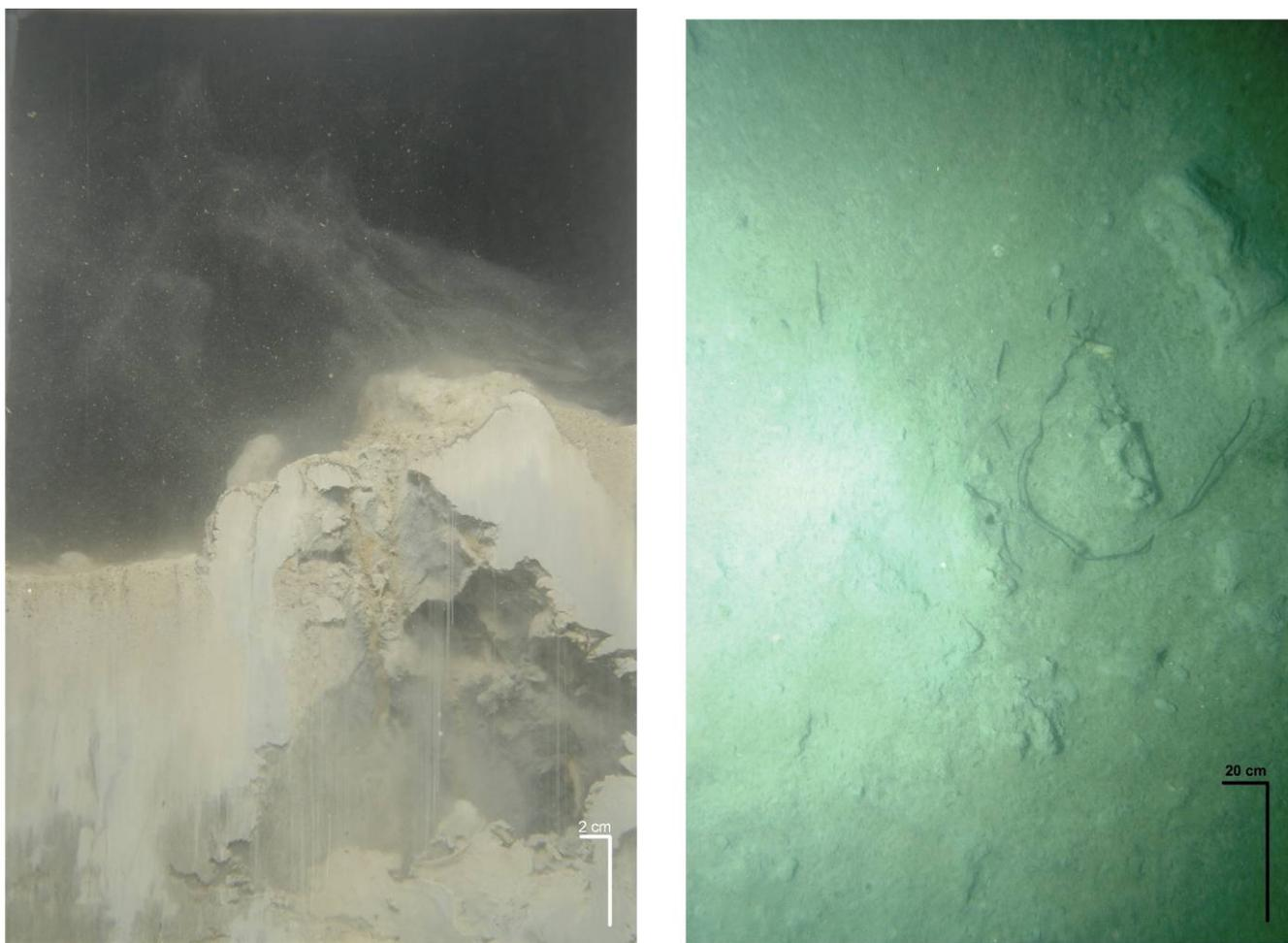
**Figure 3-22.** Evidence of consolidated clay clumps from the clamshell operation can still be seen at the sediment surface at PDA98-07 as shown in the profile (left) and plan view (right) image from this location.
