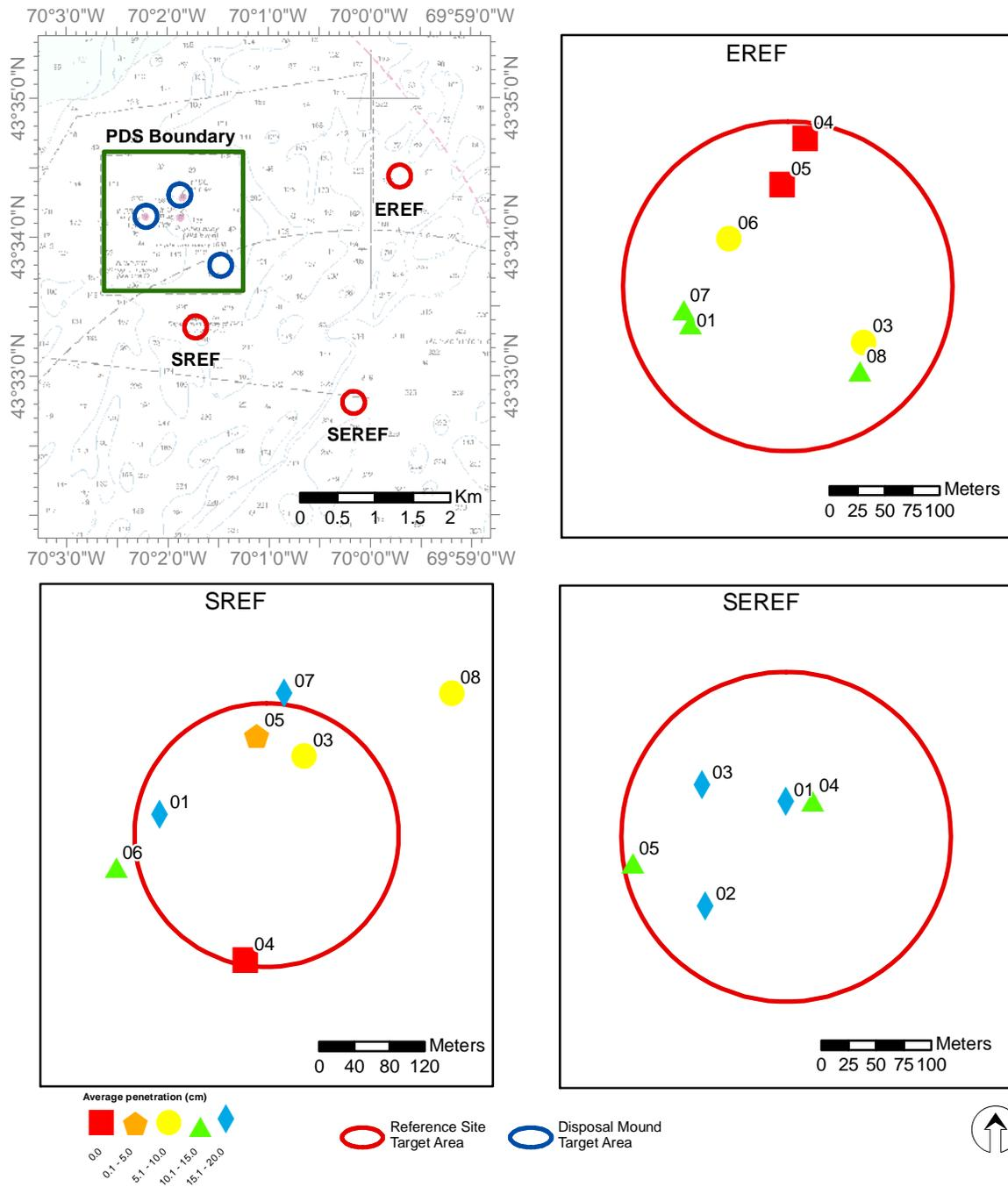
**Figure 3-5.** Spatial distribution of station-averaged camera prism penetration depth (cm) at PDS reference areas
