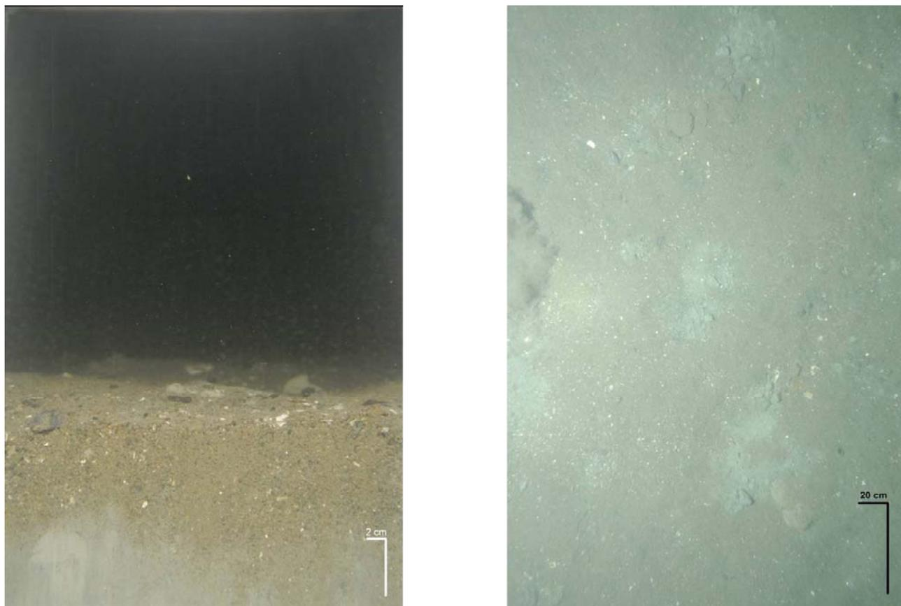
**Figure 3-14.** The surface layer of sand seen in this profile image from Station PDA-A-4 (left) is not continuous, as evidenced by the patches of mud seen on the sediment surface in the larger-scale corresponding plan view image (right).
