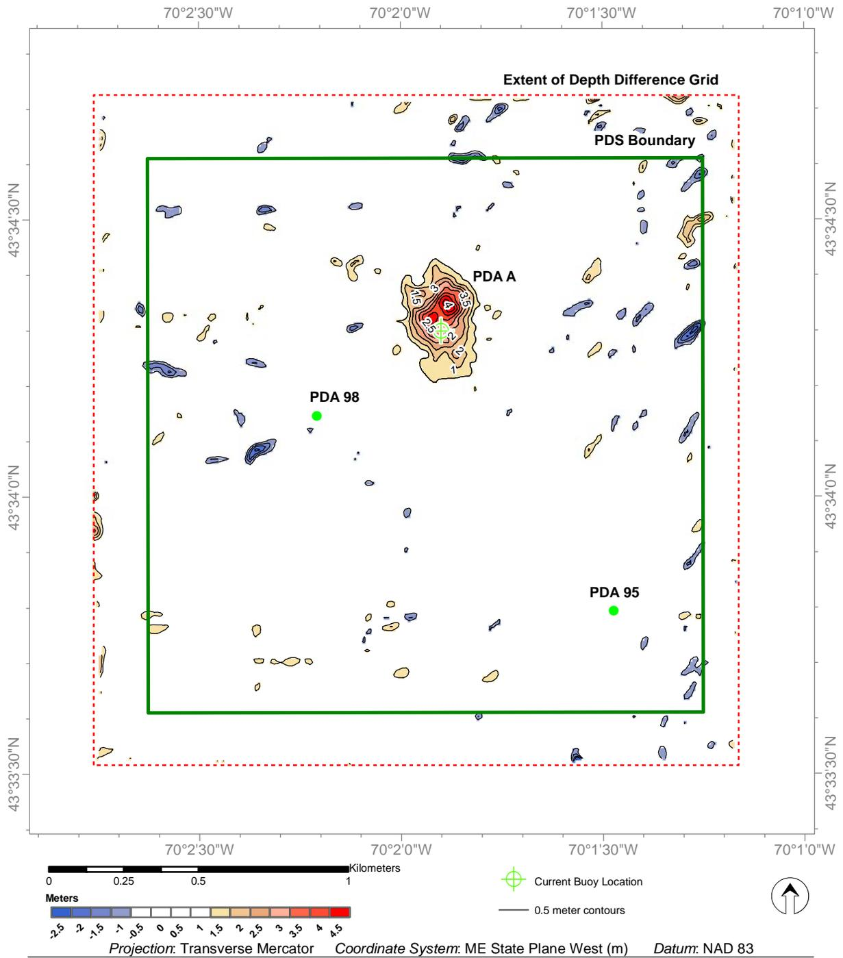
**Figure 3-2.** Depth difference contour map of PDS survey area, July 2000 vs. August 2007 survey results (0.5-m contour interval)
