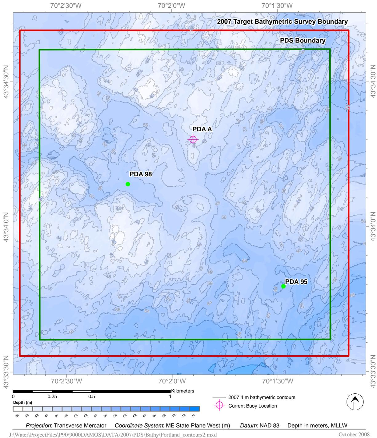
Figure 3-1. Bathymetric contour map of PDS survey area, August 2007 (4-m contour interval)
