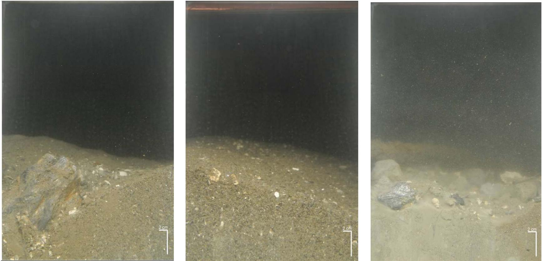
**Figure 3-18.** The small-scale surface boundary roughness elements seen in these example profile images from the PDA A Mound were all of physical origin, caused by the wide range in grain size (cobble or rocks projecting above the surface) or from surface ripples.
