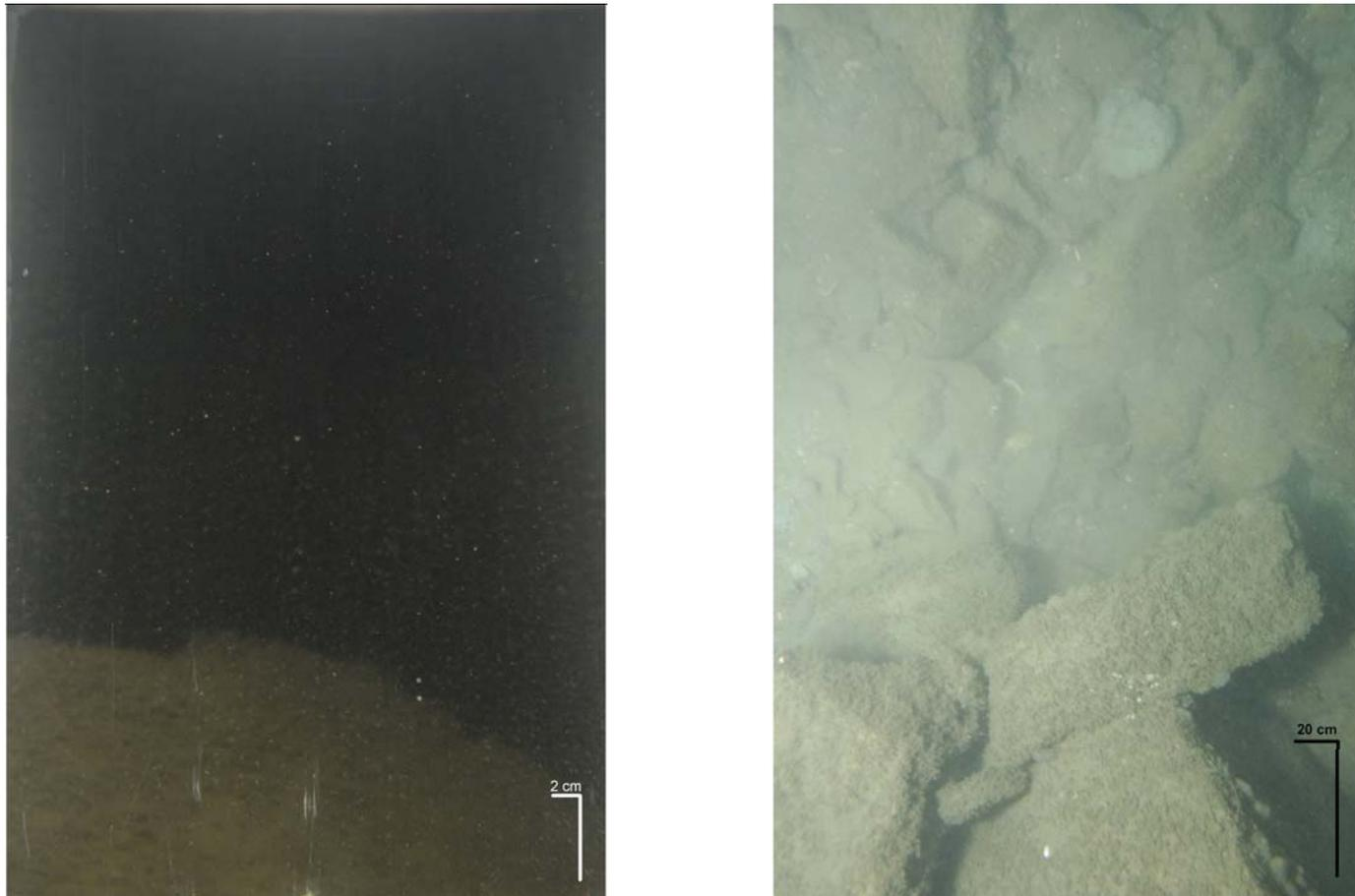
**Figure 3-12.** The sediment-profile image (left) and corresponding plan view image (right) from Station PDA-A-14 show rocks mixed in with the sand and silt deposited at the site; note the rock surfaces have already been colonized by a fouling community.
