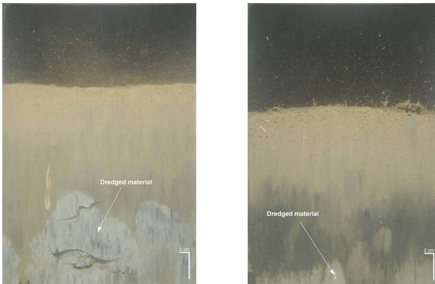
**Figure 3-25.** Evidence of dredged material can still be seen in these profile images from Stations PDA95-08 (left) and PDA95-15 (right) despite the extensive recolonization and subsurface reworking by benthic infauna.
