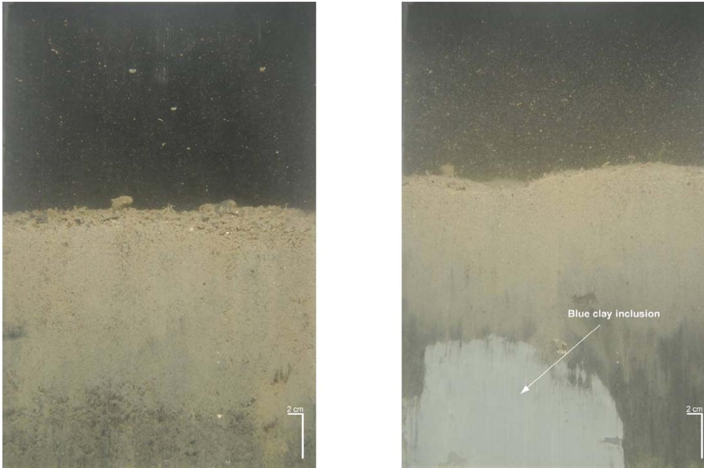
**Figure 3-24.** These representative profile images are the only two locations on the PDA 95 Mound that were not dominated by fine-grained sediments. Station 06 (left) shows poorly-sorted silty fine sand with some larger granules at the sediment surface. Station 14 (right) has a layer of silty very fine sand overlying reduced muddy sediments with a blue clay inclusion.
