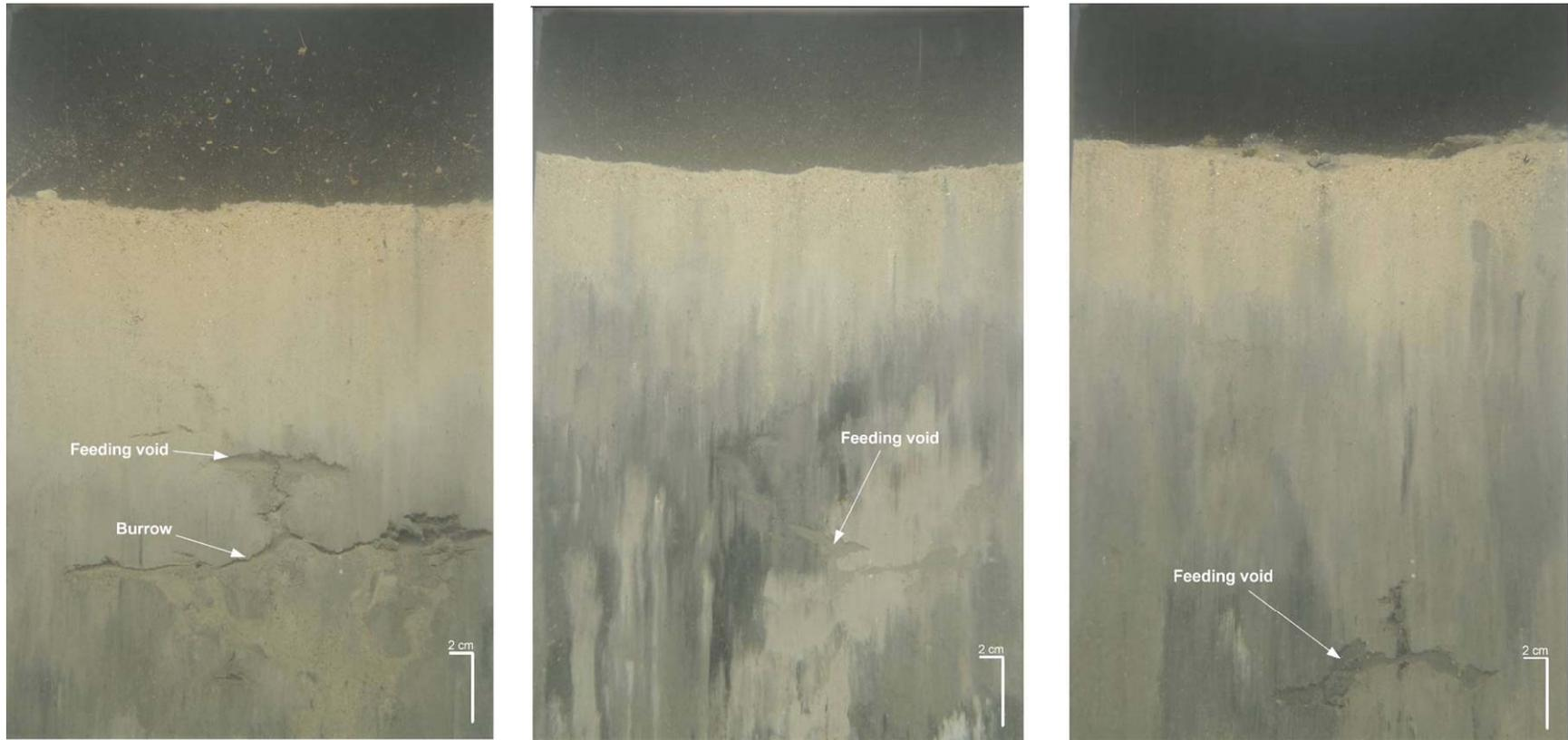
**Figure 3-23.** These representative sediment-profile images from the PDA 98 Mound show the degree to which the subsurface sediments have been reworked by infaunal burrowing and deposit feeding activities (voids and burrows highlighted by arrows on the images) (left, Station 01; center, Station 06; right, Station 11).
