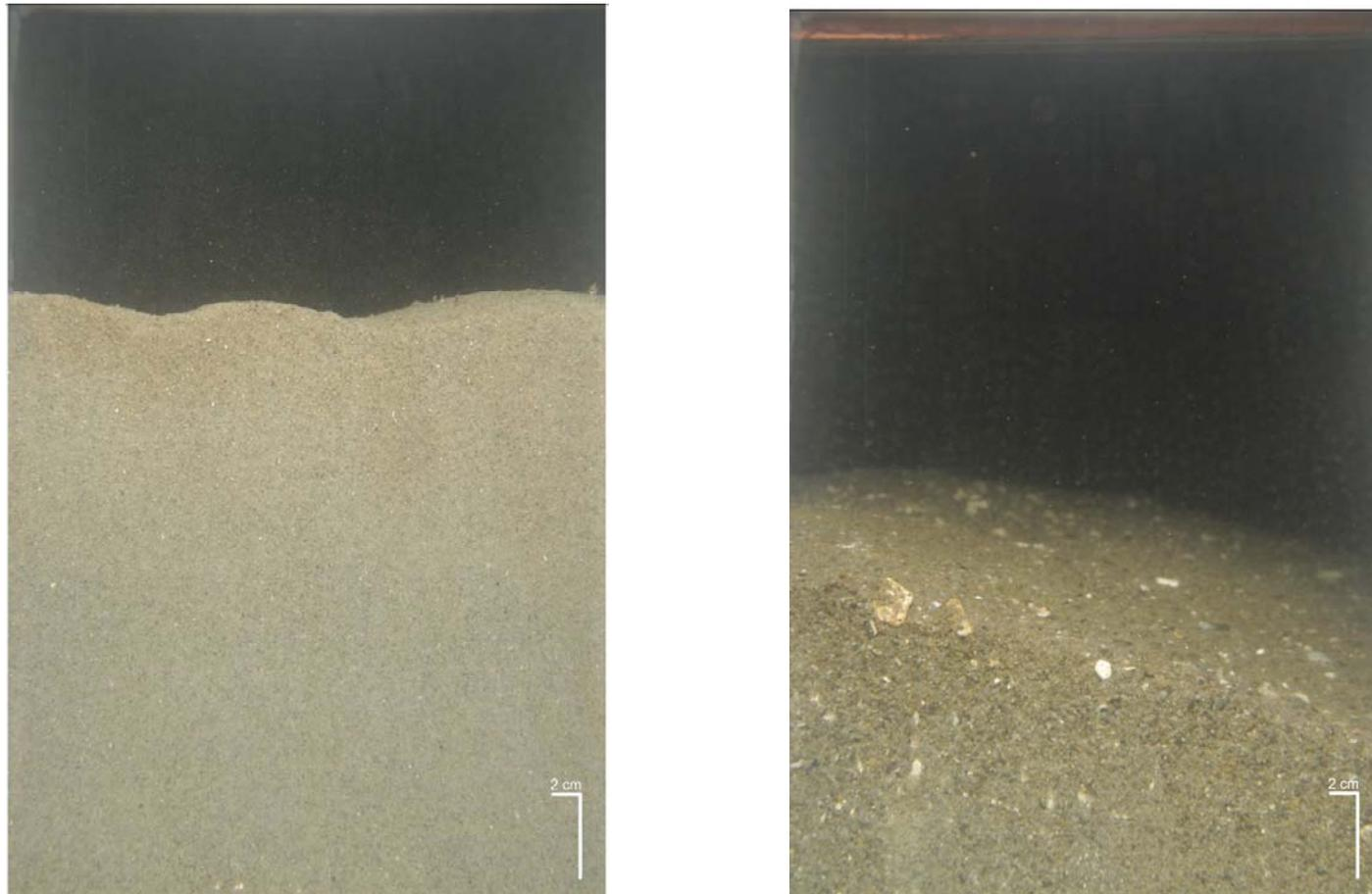
**Figure 3-15.** Profile images from Station PDA-A-10 (left) and PDA-A-13 (right) show homogeneous surface deposits of fine sand (left) and medium sand (right).
