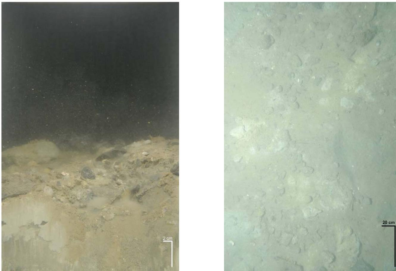
**Figure 3-13.** The consolidated clay clumps seen at the sediment surface in this profile (left) and plan view (right) image from Station PDA-A-01 are characteristic of recently disposed material dredged by a clamshell operation.
