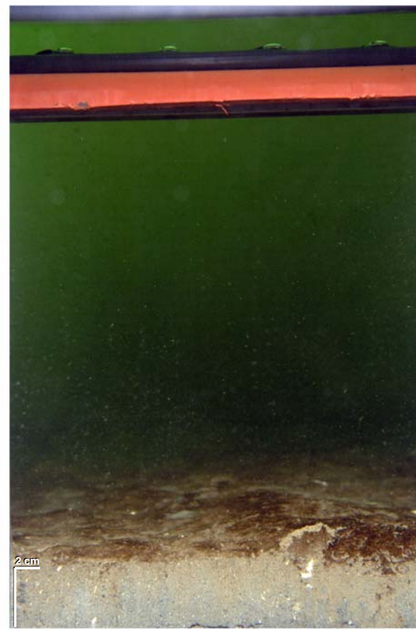
Figure 3-5. While the majority of stations sampled within the Douglas Island disposal site boundary had a sediment grain-size major mode in the silt-clay range as shown in this image from Station 5 (left), a few stations, as shown in this image from Station 6 (right), had a sediment grain-size major mode in the very fine sand range
