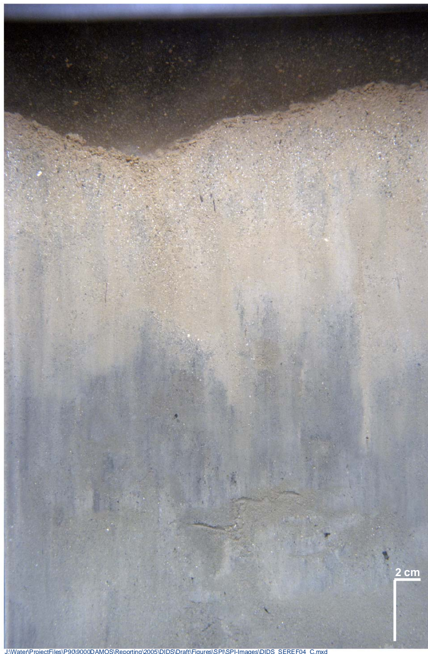
Figure 4-1. A recently-deposited 3 cm-thick layer of muddy very fine sand can be seen on top of the former sediment-water interface in this profile image from Station SEREF 04
