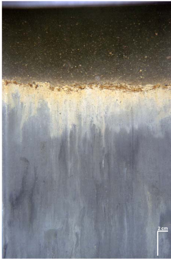
Figure 3-5. While the majority of stations sampled within the Douglas Island disposal site boundary had a sediment grain-size major mode in the silt-clay range as shown in this image from Station 5 (left), a few stations, as shown in this image from Station 6 (right), had a sediment grain-size major mode in the very fine sand range
