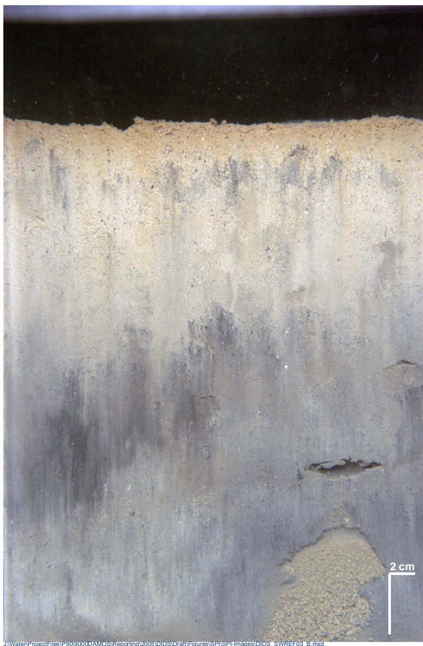
Figure 3-17. This sediment profile image from Station SWREF 03 shows evidence of deep infaunal re-working and bioturbation
