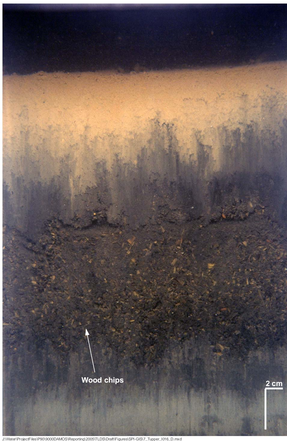
Figure 3-10. One quite common diagnostic feature of disposed sediment at the Tupper Ledge Disposal Site was the presence of wood chips and fibers, as can be seen in this profile image from Station I16
