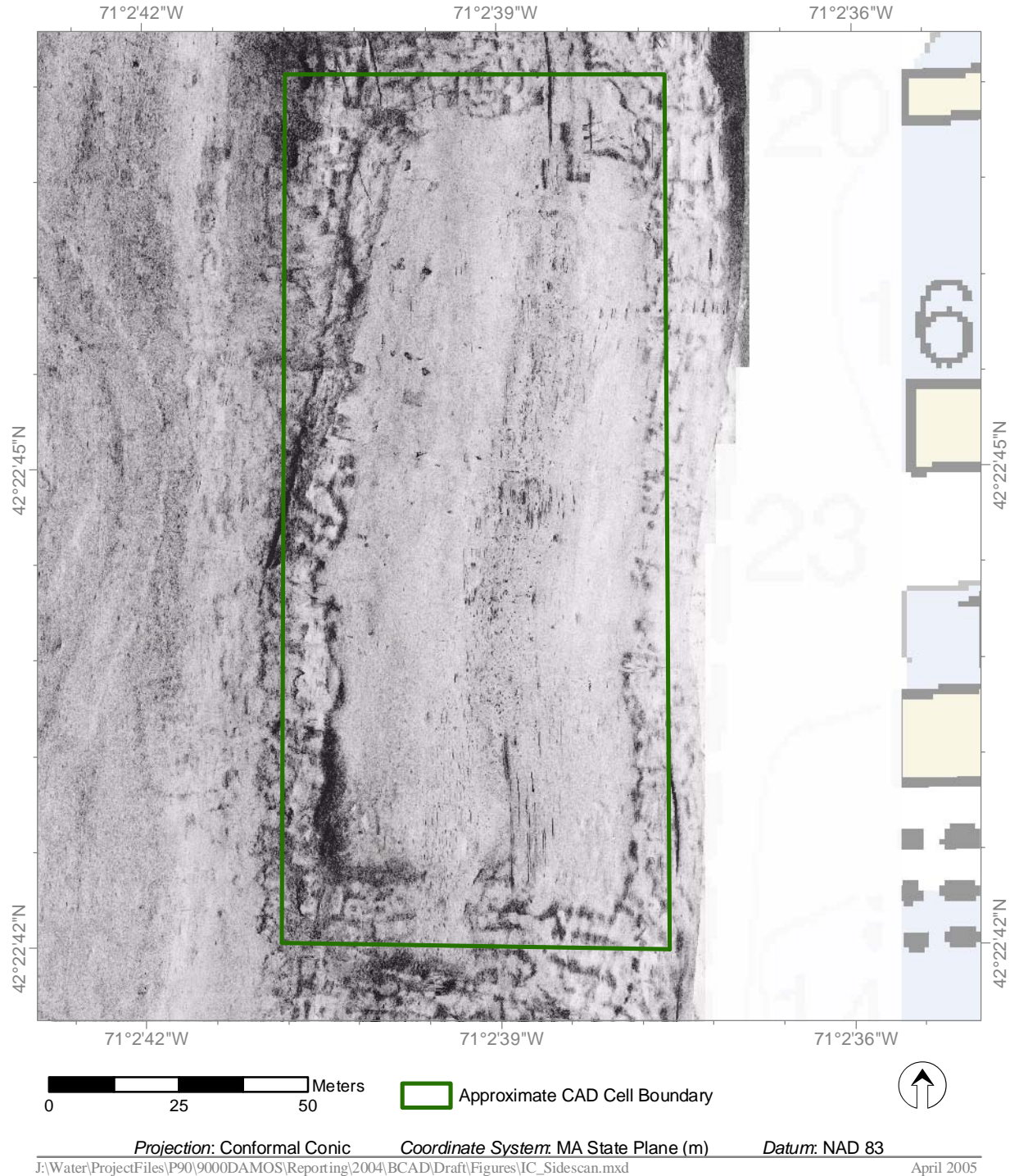
Figure 3-19. Side-scan sonar image of Inner Confluence cell IC2, August 2004
