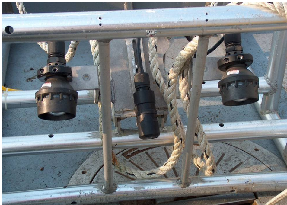
Figure 2-4. Towed video sled and camera setup
