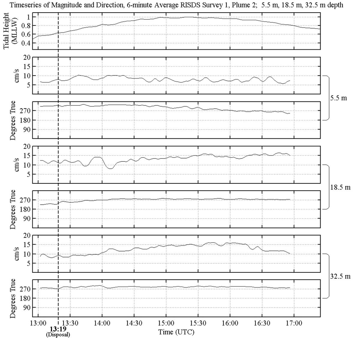
**Figure 3-23.** Time-series (UTC) plot of current magnitude and direction during Plume 2 at the near-surface level ( $\sim 5.5$  m; top two panels) and the two selected drogue depth levels of  $\sim 18$  m (middle two panels) and  $\sim 32$  m depth (bottom two panels). Currents were sampled at 1 minute intervals, and filtered with six minute Low Pass Filter (LPF) to reduce high-frequency noise. Dashed line (13:19) represents barge disposal time.
