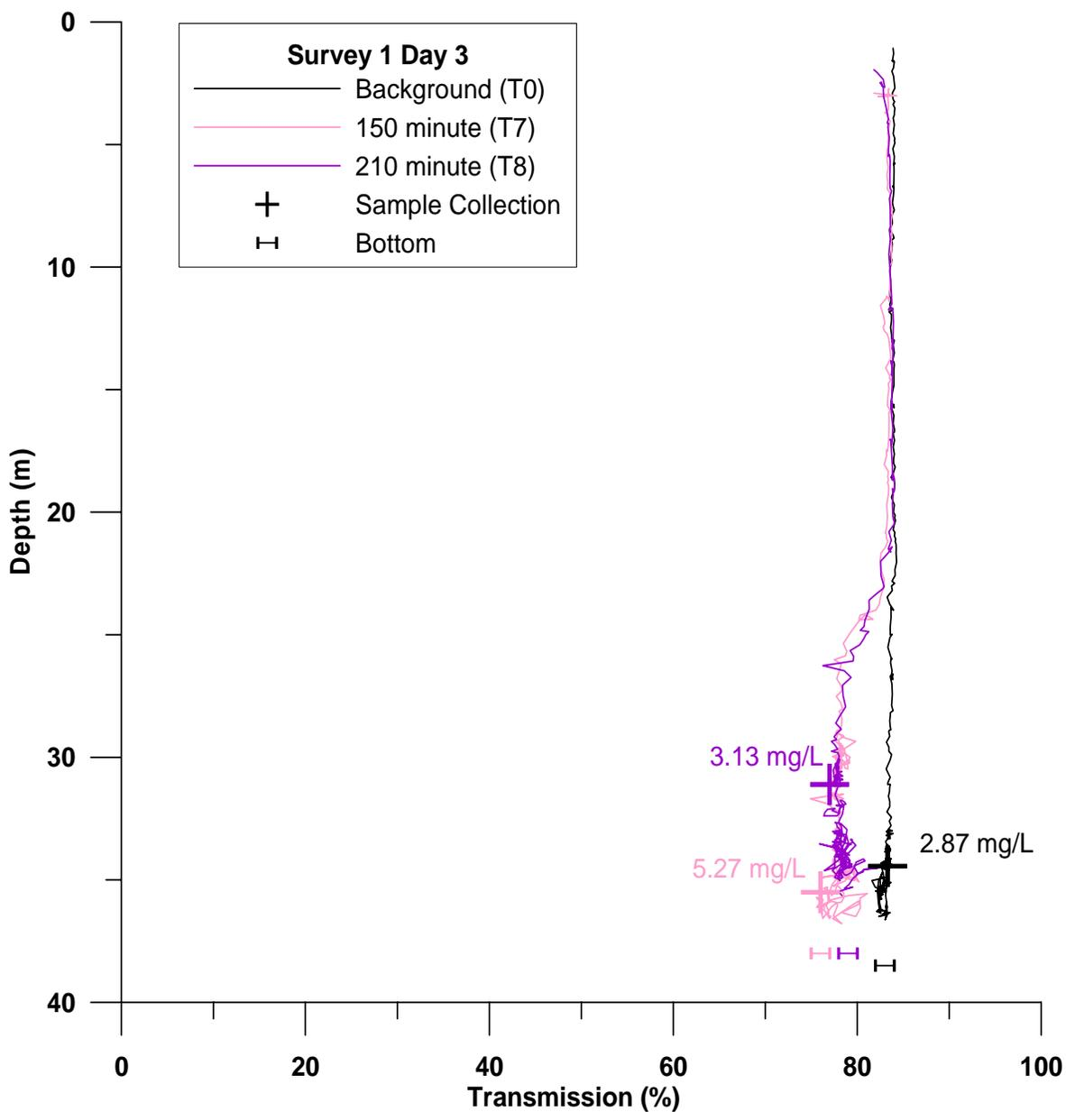
**Figure 3-49.** Profile plot of percent light transmission and sensor depth acquired during CTD sample intervals T7 and T8 for Plume 3. Locations of water sample collections within the plume are also shown.
