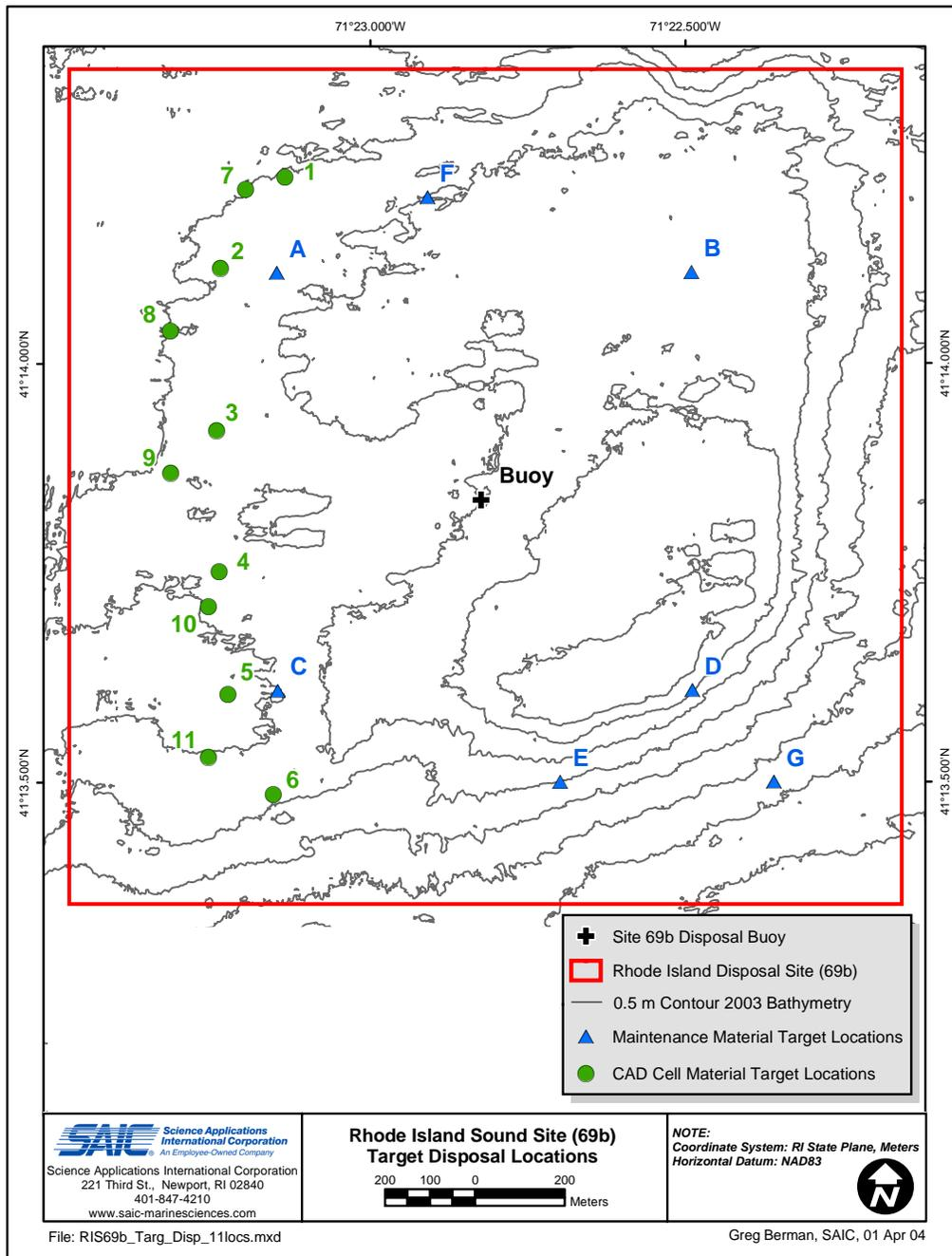
**Figure 1-3.** Location of the target disposal locations for maintenance material (blue) and CAD cell material (green) relative to the boundaries of RISDS.
