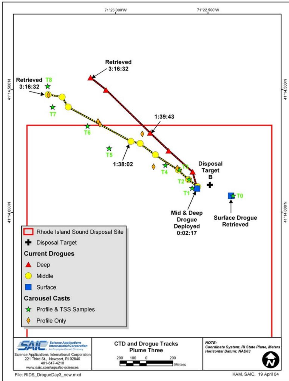
**Figure 3-41.** Map indicating current drogue trajectories and CTD cast locations during the tracking of Plume 3. Locations of water samples are also shown. Times represent elapsed time since disposal operations.
