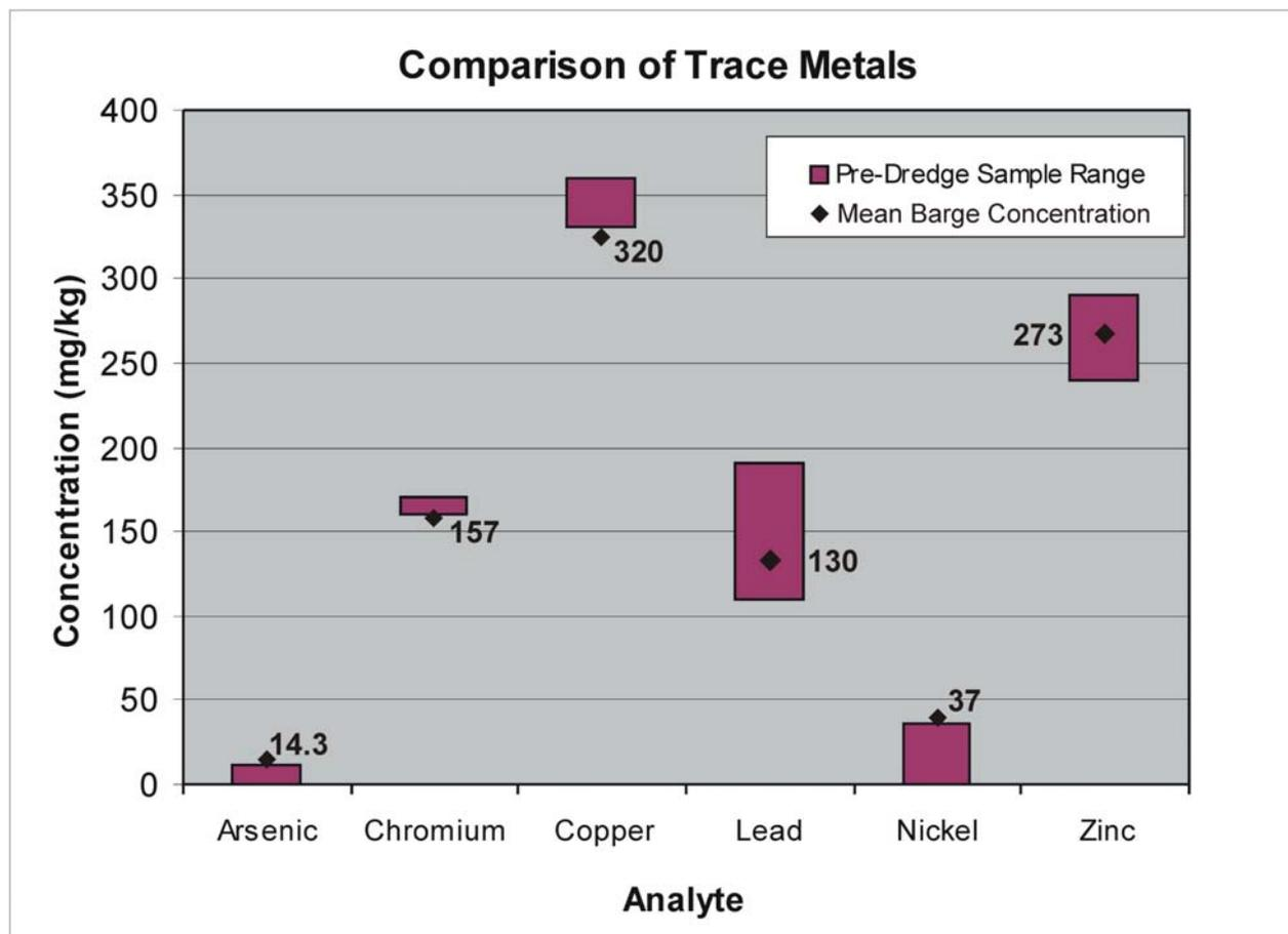
**Figure 5-7.** Chart showing the relationship between the mean concentration of trace metals in the April 2004 disposal barge samples to the range of concentrations detected in the 1992 and 1994 pre-dredge samples of in-place sediments within Sabin Point Reach.
