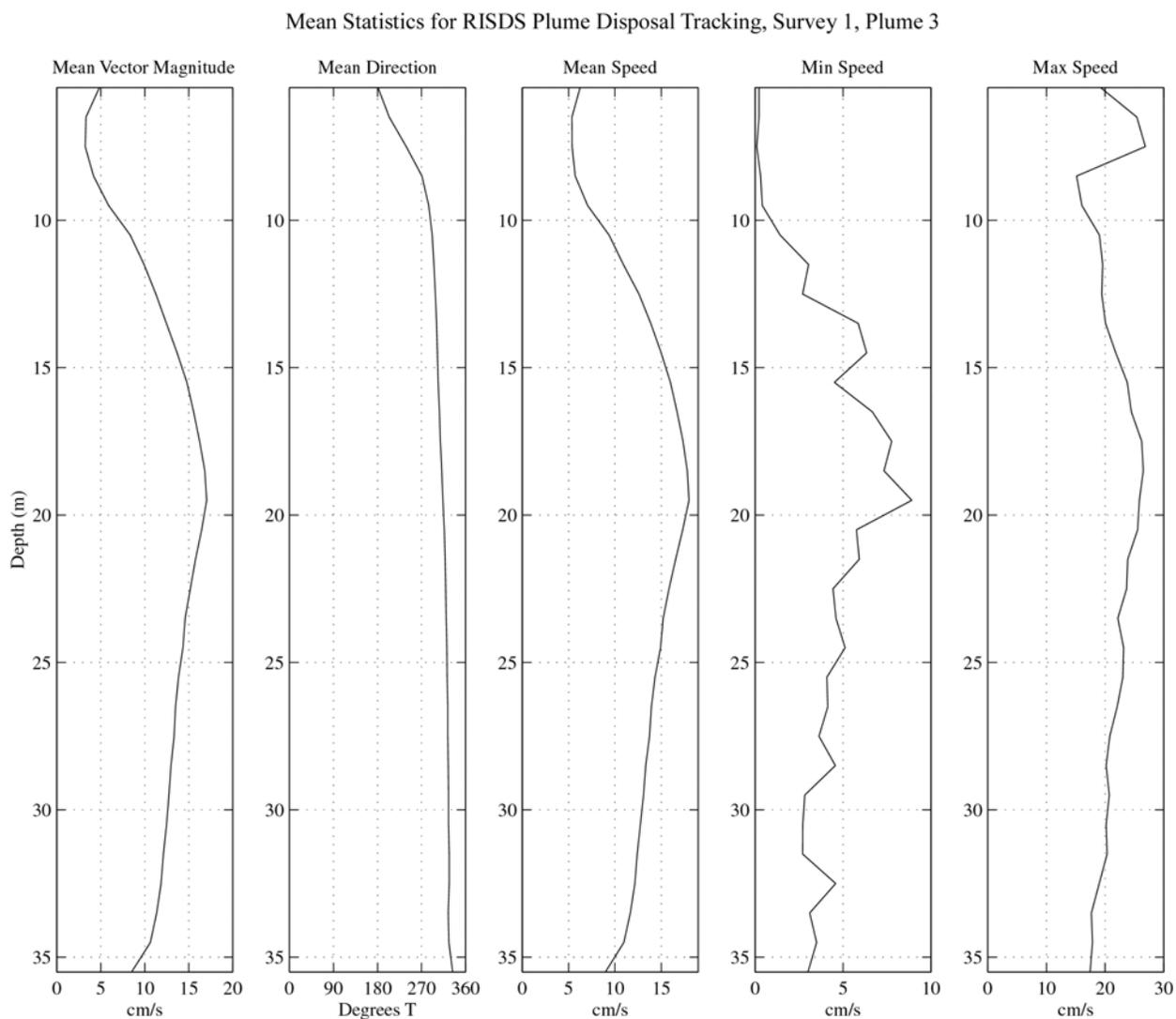
**Figure 3-42.** Statistics of moored current meter data collected on site during Plume 3 disposal monitoring activities. Current meter deployed for extent of the survey period (3.5 hours). Parameters plotted include mean vector magnitude, mean vector direction, mean speed (regardless of direction), minimum speed and maximum speed.
