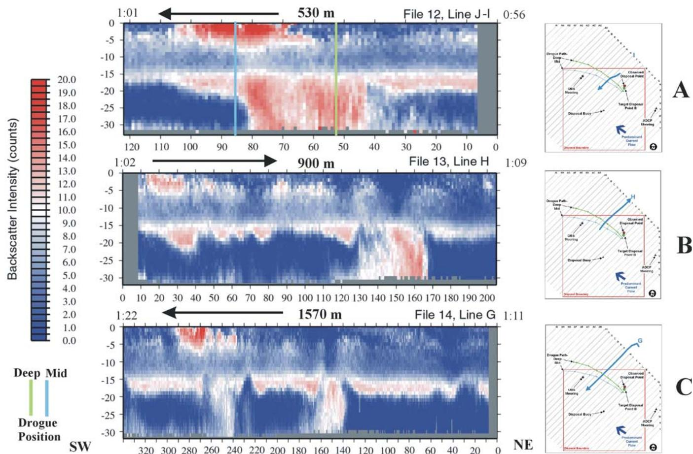
**Figure 3-15.** Profile plots of data collected from ADCP transects J, H, and G on 8 April 2004 (Plume 1) displaying acoustic backscatter intensity within the water column minus the raw backscatter intensity to illustrate plume morphology 56 to 82 minutes after the dredged material disposal event at Point B.
