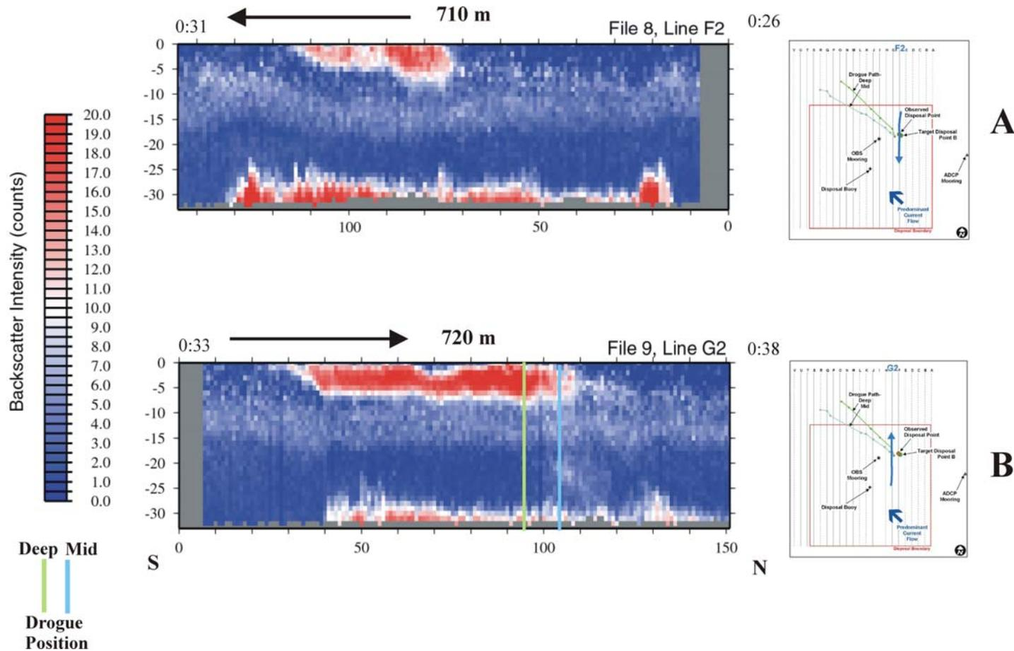
**Figure 3-53.** Profile plots of data collected from ADCP transects F2 and G2 on 10 April 2004 (Plume 3) displaying acoustic backscatter intensity within the water column minus the raw backscatter intensity to illustrate plume morphology 26 to 38 minutes after the dredged material disposal event at Point B.
