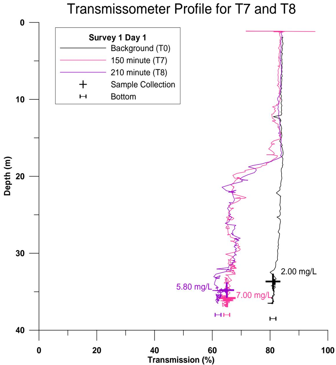
**Figure 3-11.** Profile plot of percent light transmission and sensor depth acquired during CTD sample intervals T7 and T8 for Plume 1. Locations of water sample collections within the plume are also shown.
