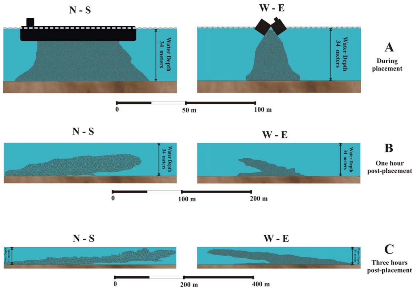
**Figure 5-5.** Schematic representation of the morphology of a typical sediment plume formed over RISDS immediately following disposal (A), one-hour post placement (B) and three-hours post placement (C).
