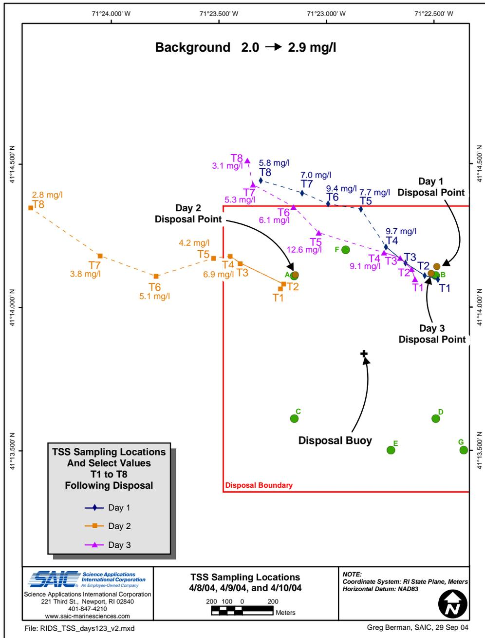
**Figure 5-6.** Graphic representing the various positions of the centroid of the three sediment plumes tracked during the April 2004 plume monitoring survey relative the RISDS boundaries.
