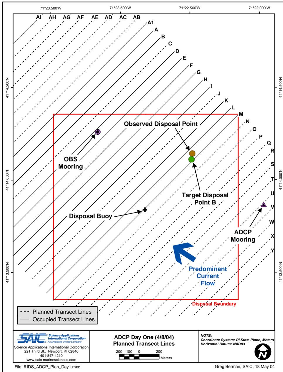
**Figure 2-2.** Survey track lines for acoustic monitoring of suspended sediment occupied as part of the Plume 1 monitoring event during the RISDS plume survey. Solid lines represent survey lines that were occupied during the course of the survey day, while dashed lines represent those that were pre-established but not occupied.
