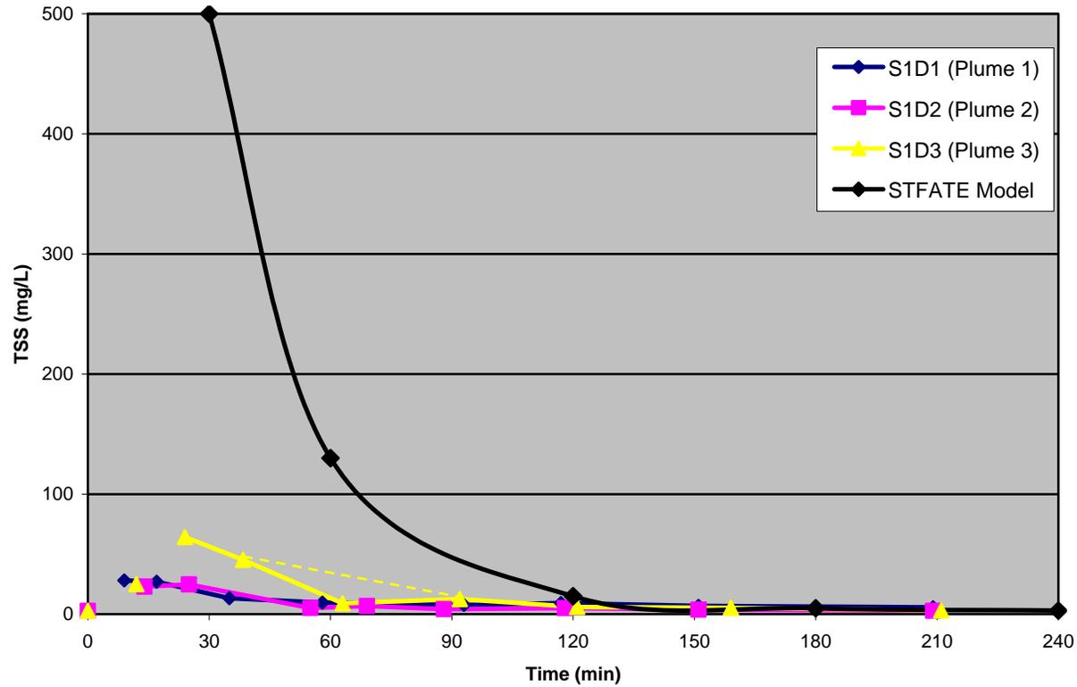
**Figure 5-2.** Plot of total suspended solids (TSS) concentration versus time for discrete water samples collected during CTD profiling operations for RISDS plume monitoring in comparison to TSS concentrations predicted for the disposal of 4,600 m<sup>3</sup> (6,000 yd<sup>3</sup>) of material dredged from Providence River (USACE 2001).
