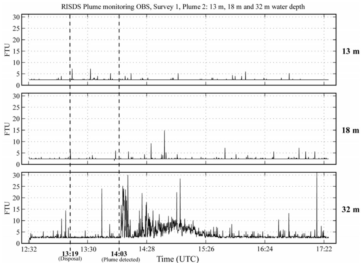
**Figure 3-39.** Time-series (UTC) plot of OBS data collected on 9 April 2004 (Plume 2) from three levels in the water column (13 m, 18 m, and 32 m), displaying changes in turbidity (FTU) over time resulting from sediment plume passage. Dashed lines represent barge disposal time (13:19) and an increase in suspended sediment (14:03), indicating the possible of the leading edge of the plume.
