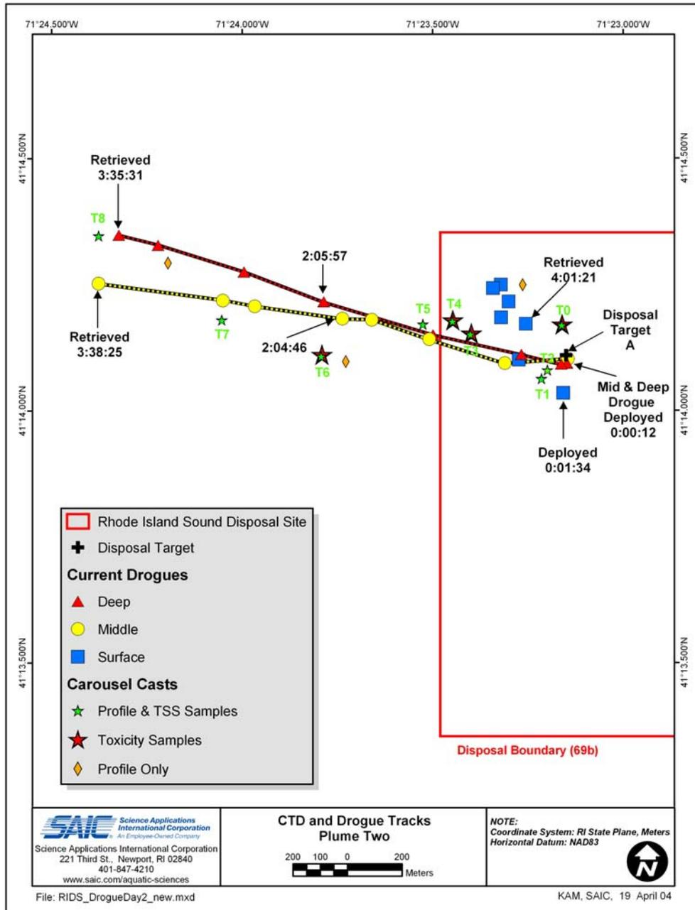
**Figure 3-21.** Map indicating current drogue trajectories and CTD cast locations during the tracking of Plume 2. Locations of water samples are also shown. Times represent elapsed time since disposal operations.
