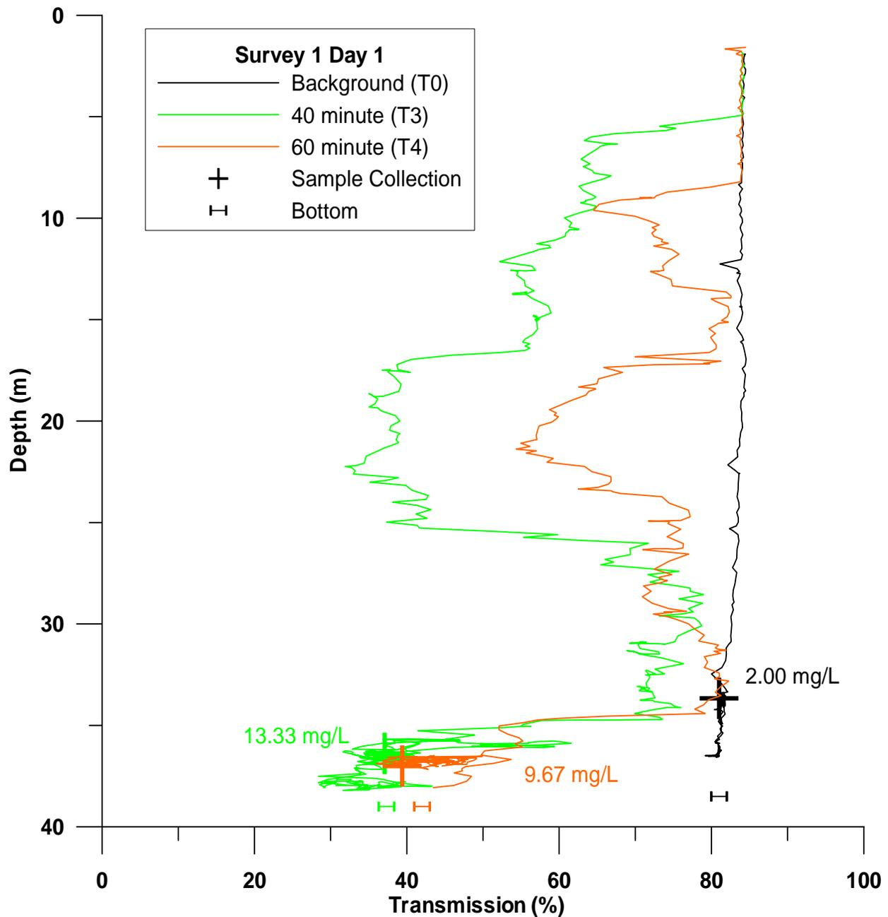
**Figure 3-8.** Profile plot of percent light transmission and sensor depth acquired during CTD sample intervals T3 and T4 for Plume 1. Locations of water sample collections within the plume are also shown.
