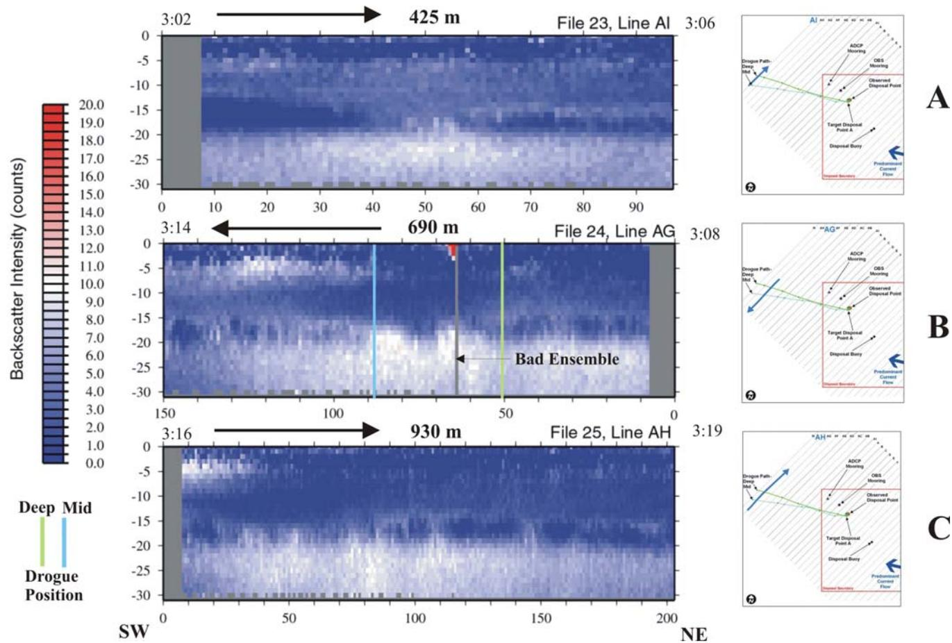
**Figure 3-38.** Profile plots of data collected from ADCP transects AI, AG, and AH on 9 April 2004 (Plume 2) displaying acoustic backscatter intensity within the water column minus the raw backscatter intensity to illustrate plume morphology 182 to 199 minutes after the dredged material disposal event at Point A.
