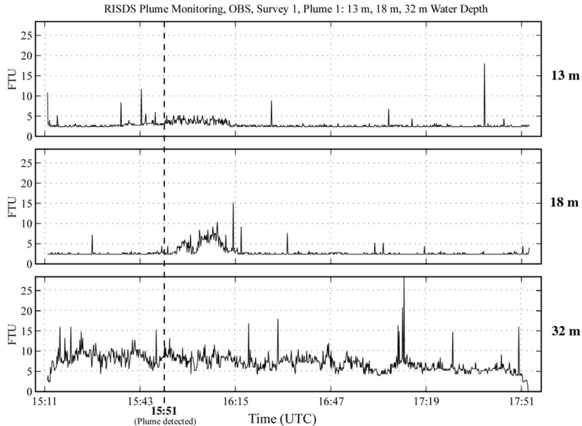
**Figure 3-19.** Time-series (UTC) plot of OBS data collected on 8 April 2004 (Plume 1) from three levels in the water column (13 m, 18 m, and 32 m), displaying changes in turbidity (FTU) over time resulting from sediment plume passage. Dashed line (15:51) represents an increase in suspended sediment, indicating the possible of the leading edge of the plume.
