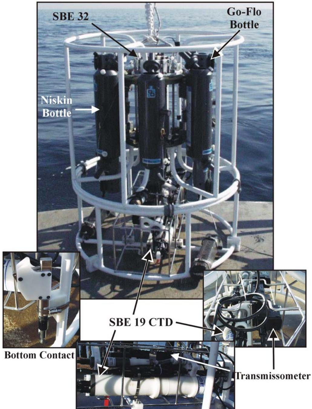
**Figure 2-1.** Photograph of the Seabird (Model SBE-32) Carousel Water Sampler used for plume tracking and water quality monitoring.
