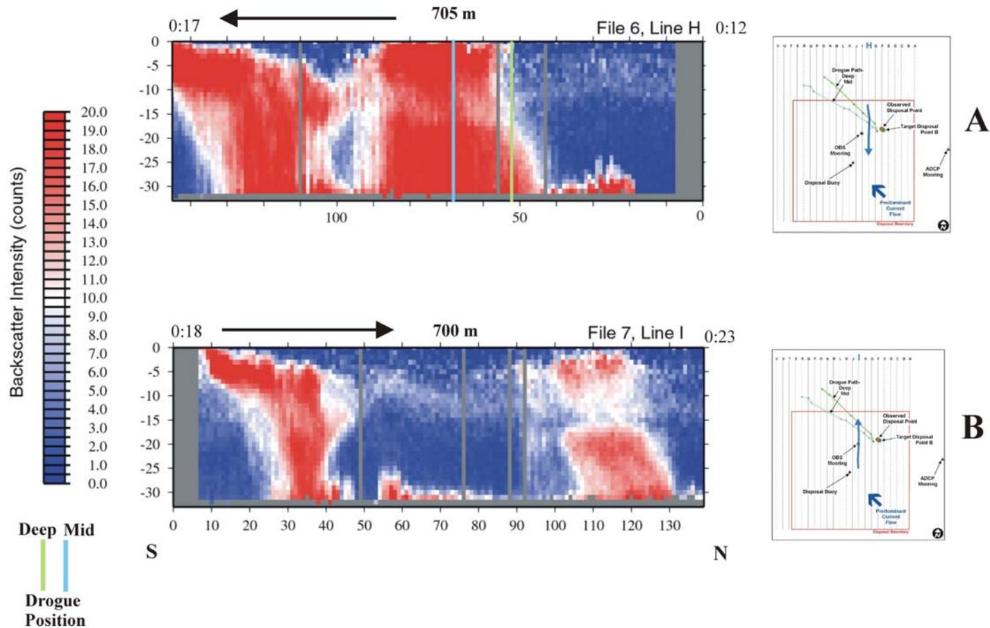
**Figure 3-52.** Profile plots of data collected from ADCP transects H and I on 10 April 2004 (Plume 3) displaying acoustic backscatter intensity within the water column minus the raw backscatter intensity to illustrate plume morphology 12 to 23 minutes after the dredged material disposal event at Point B.
