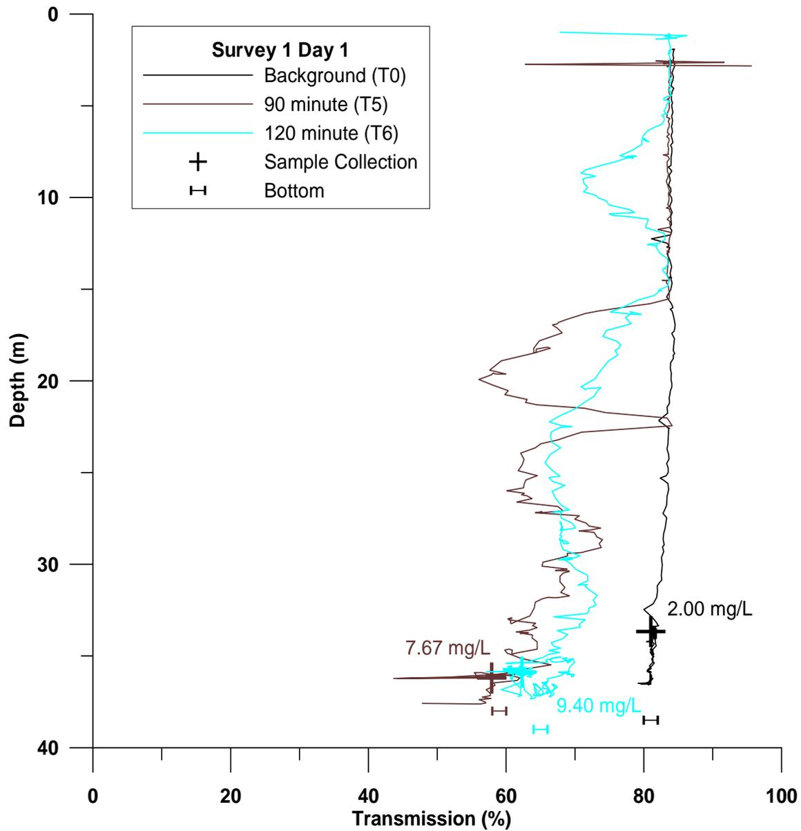
**Figure 3-10.** Profile plot of percent light transmission and sensor depth acquired during CTD sample intervals T5 and T6 for Plume 1. Locations of water sample collections within the plume are also shown.
