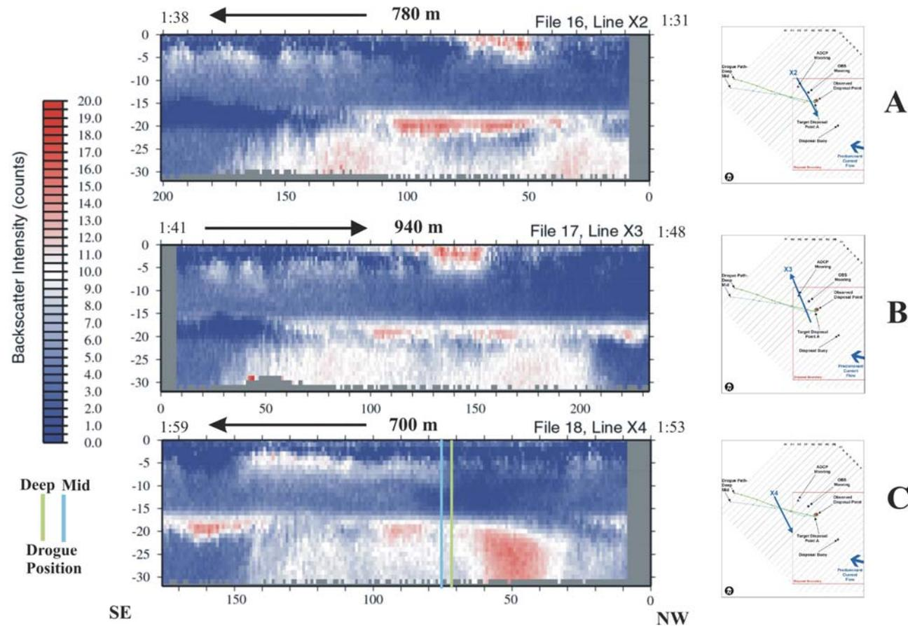
**Figure 3-35.** Profile plots of data collected from ADCP transects X2, X3, and X4 (northwest-southeast orientation) on 9 April 2004 (Plume 2) displaying acoustic backscatter intensity within the water column minus the raw backscatter intensity to illustrate plume morphology 91 to 119 minutes after the dredged material disposal event at Point A.
