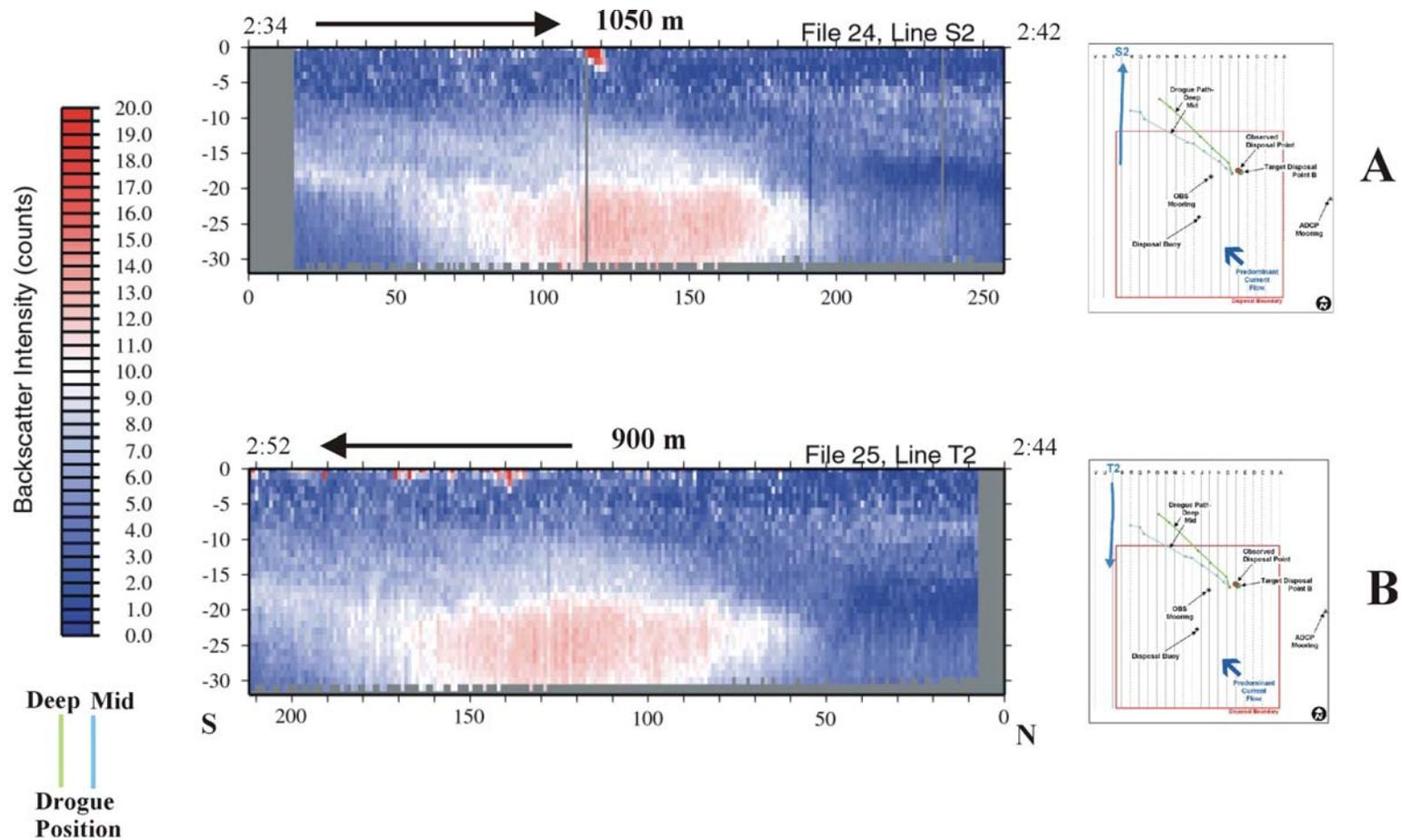
**Figure 3-58.** Profile plots of data collected from ADCP transects S2 and T2 on 10 April 2004 (Plume 3) displaying acoustic backscatter intensity within the water column minus the raw backscatter intensity to illustrate plume morphology 154 to 172 minutes after the dredged material disposal event at Point B.
