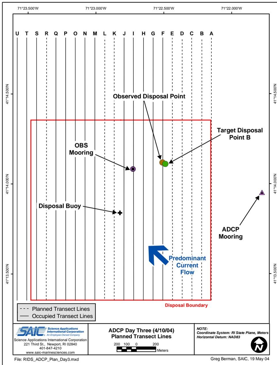
**Figure 2-4.** Survey track lines for acoustic monitoring of suspended sediment occupied as part of the Plume 3 monitoring event during the RISDS plume survey. Solid lines represent survey lines that were occupied during the course of the survey day, while dashed lines represent those that were pre-established but not occupied.
