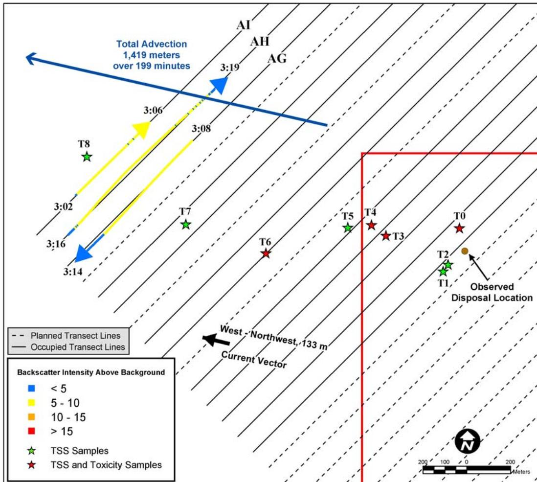
**Figure 4-7.** Residual acoustic backscatter intensity values from the 32 m depth interval representing suspended sediment concentrations along individual survey lines occupied during the Plume 2 monitoring survey, 182 to 199 minutes after the disposal event.
