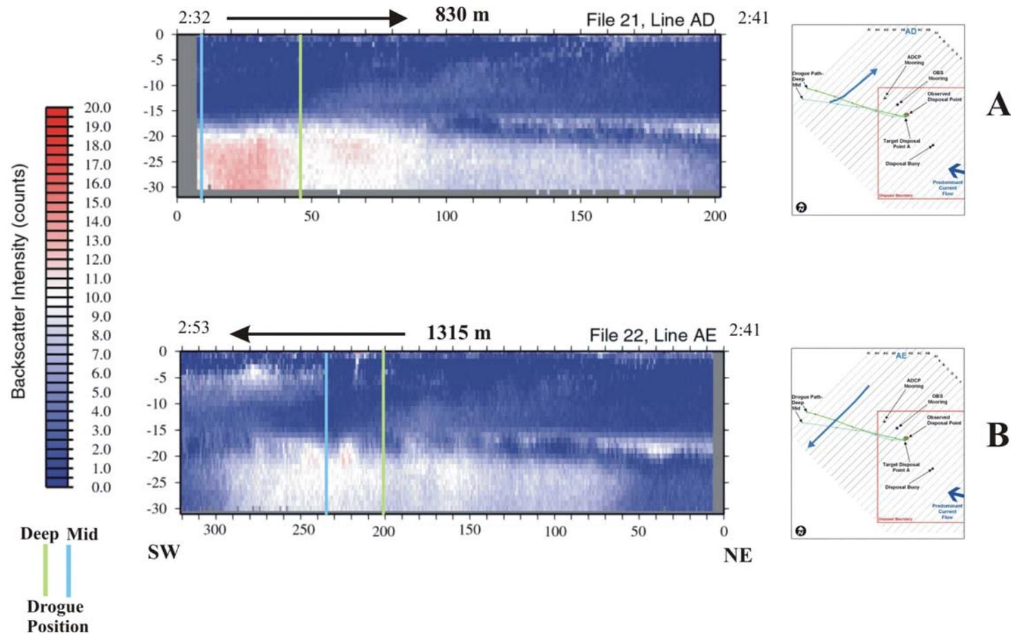
**Figure 3-37.** Profile plots of data collected from ADCP transects AD and AE on 9 April 2004 (Plume 2) displaying acoustic backscatter intensity within the water column minus the raw backscatter intensity to illustrate plume morphology 152 to 173 minutes after the dredged material disposal event at Point A.
