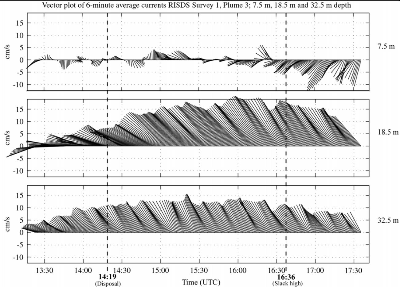
**Figure 3-44.** Time-series (UTC) plot of current vectors (6-min LPF) during Plume 3 at the near-surface level (7.5 m; top panel) and the two selected drogue depth levels of ~18m (middle panel) and ~32m depth (bottom panel). Dashed lines represent the time of barge disposal (14:19) and the slack high tide (16:36).
