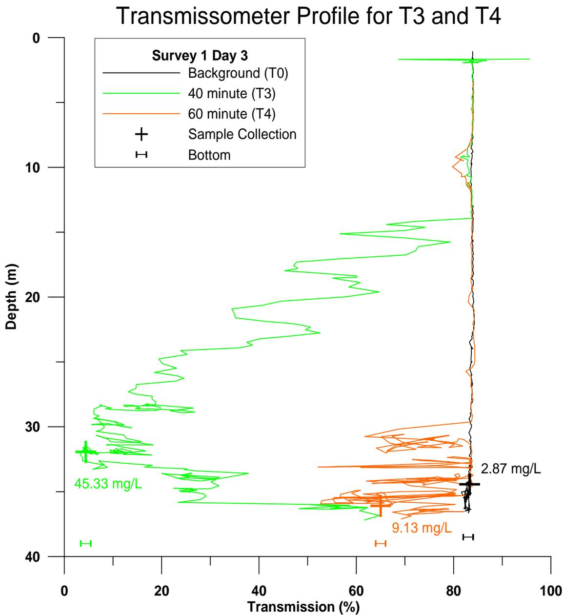
**Figure 3-47.** Profile plot of percent light transmission and sensor depth acquired during CTD sample intervals T3 and T4 for Plume 3. Locations of water sample collections within the plume are also shown.
