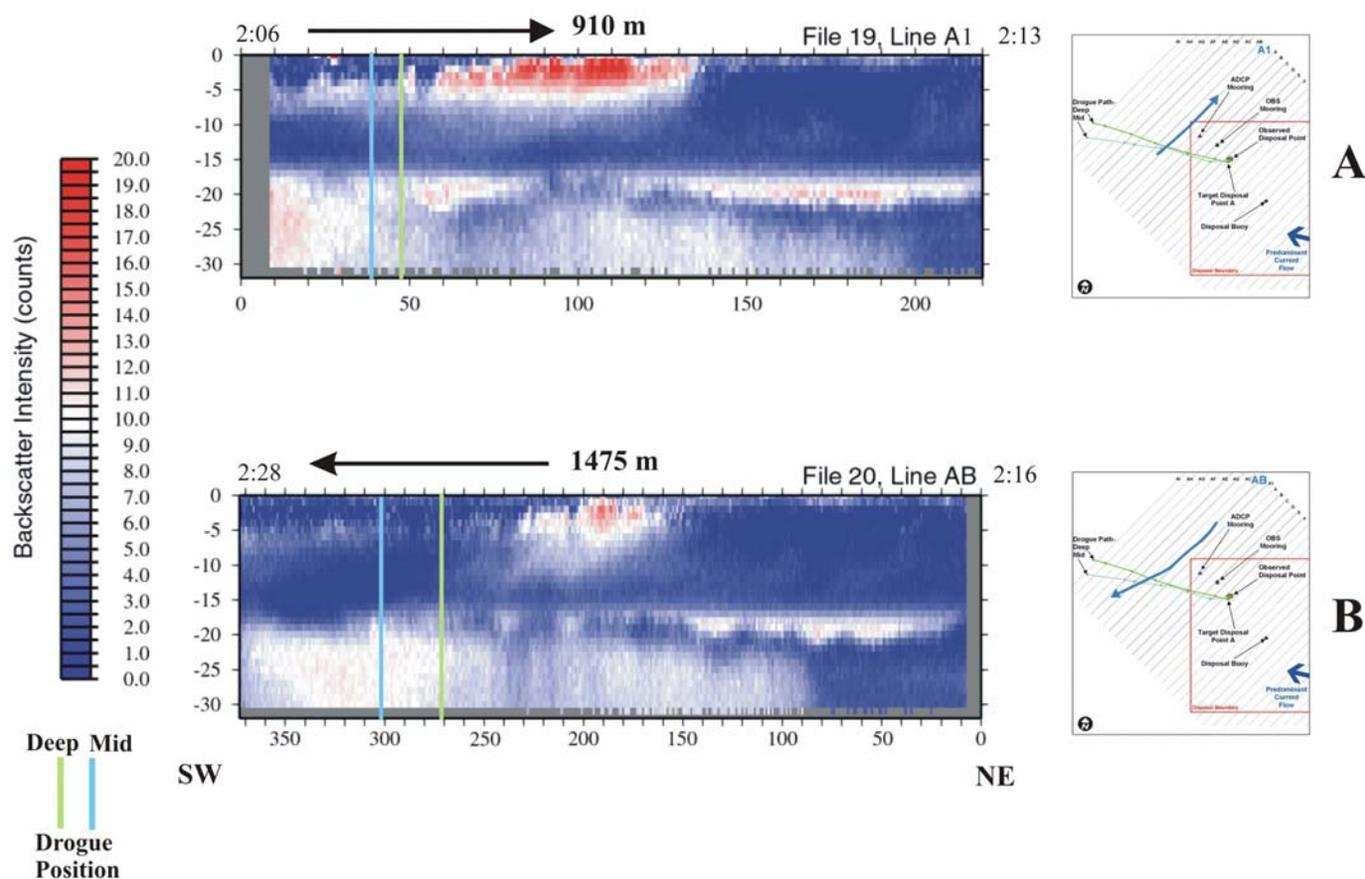
**Figure 3-36.** Profile plots of data collected from ADCP transects A1 and AB (northeast-southwest orientation) on 9 April 2004 (Plume 2) displaying acoustic backscatter intensity within the water column minus the raw backscatter intensity to illustrate plume morphology 126 to 148 minutes after the dredged material disposal event at Point A.
