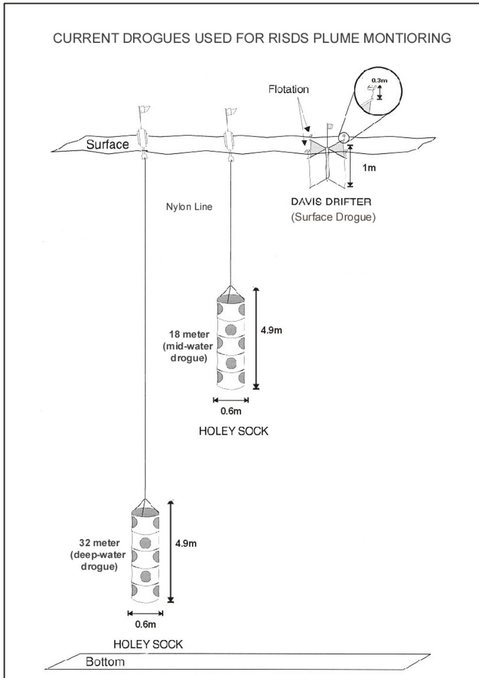
**Figure 2-5.** Drawing of holey sock drogues and Davis drifter used for real-time assistance with tracking plume advection at mid-water, deep-water, and surface levels.
