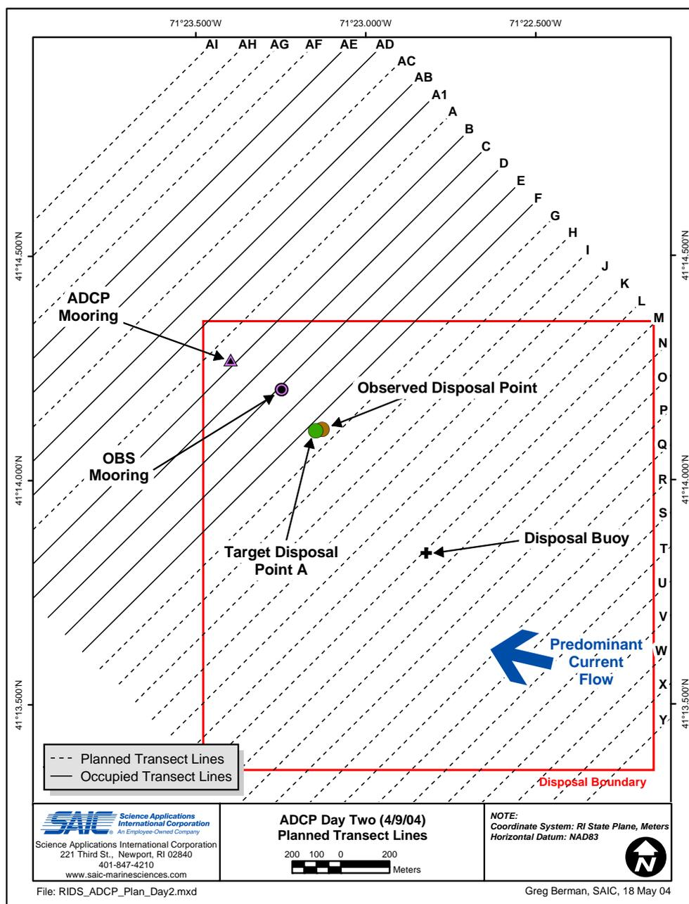
**Figure 2-3.** Survey track lines for acoustic monitoring of suspended sediment occupied as part of the Plume 2 monitoring event during the RISDS plume survey. Solid lines represent survey lines that were occupied during the course of the survey day, while dashed lines represent those that were pre-established but not occupied.
