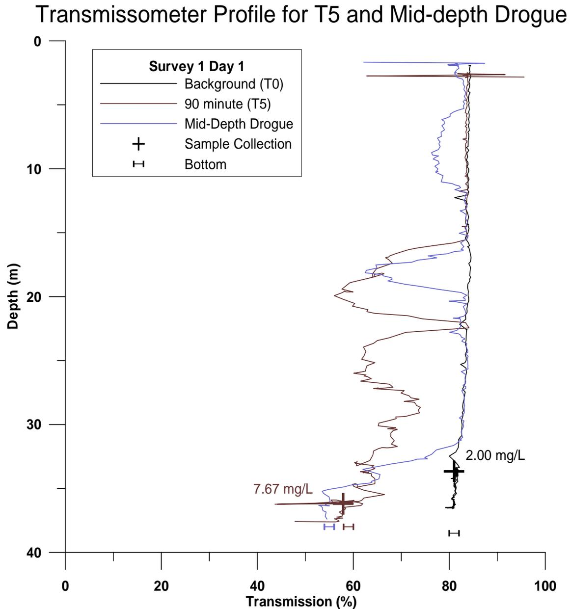
**Figure 3-9.** Profile plot of percent light transmission and sensor depth acquired during CTD sample interval T5 and the mid-depth drogue for Plume 1. Locations of water sample collections within the plume are also shown.
