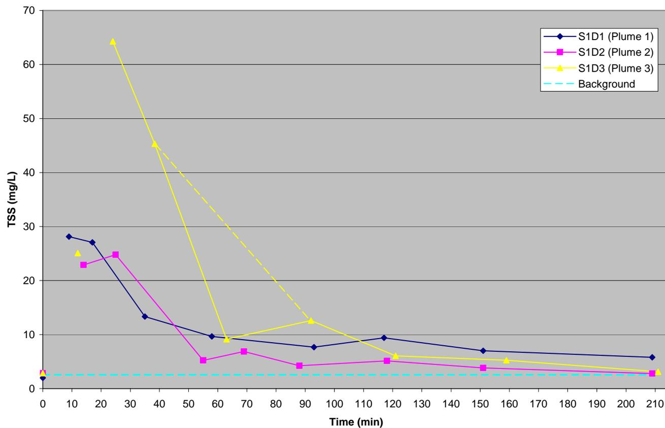
**Figure 5-1.** Plot of total suspended solids (TSS) concentration versus time since plume event for discrete water samples collected during CTD profiling operations for RISDS plume monitoring.
