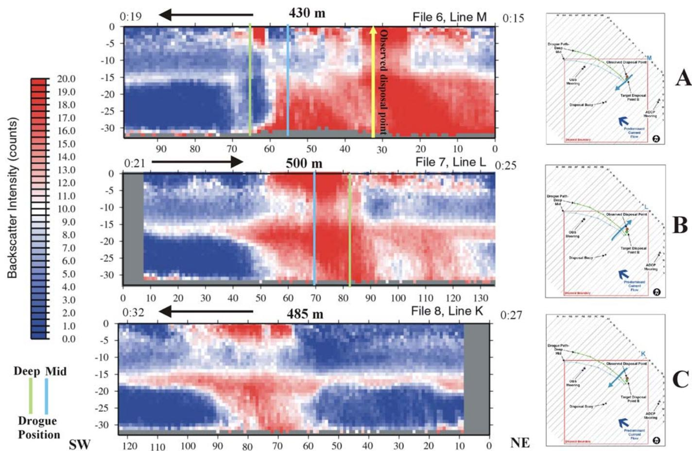
**Figure 3-13.** Profile plots of data collected from ADCP transects M, L, and K on 8 April 2004 (Plume 1) displaying acoustic backscatter intensity within the water column minus the raw backscatter intensity to illustrate plume morphology 15 to 32 minutes after the dredged material disposal event at Point B.
