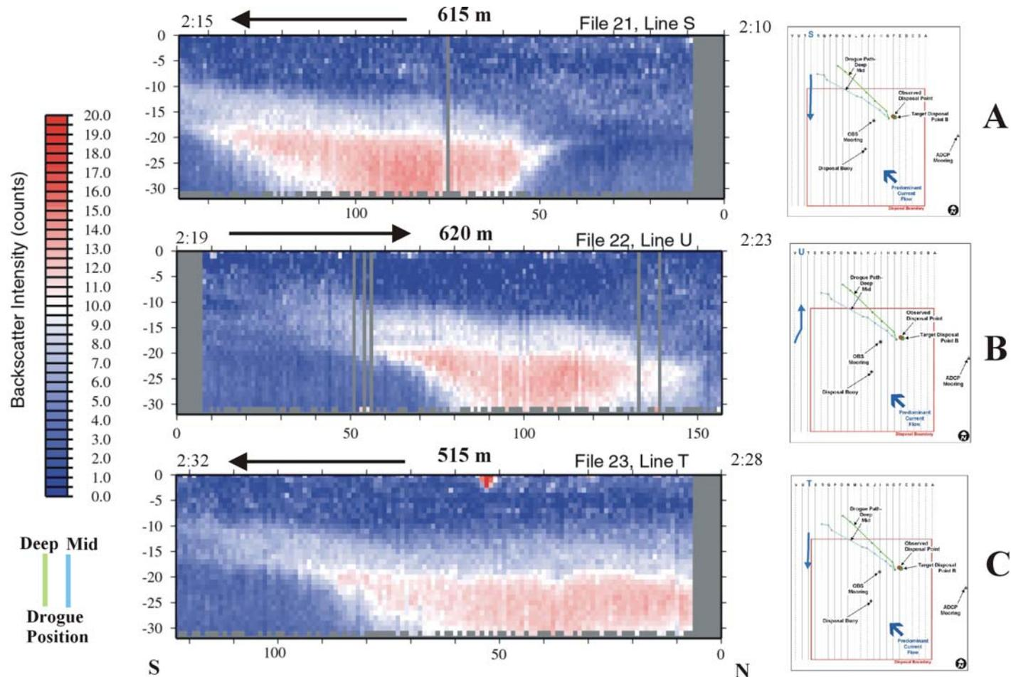
**Figure 3-57.** Profile plots of data collected from ADCP transects S, U, and T on 10 April 2004 (Plume 3) displaying acoustic backscatter intensity within the water column minus the raw backscatter intensity to illustrate plume morphology 130 to 152 minutes after the dredged material disposal event at Point B.
