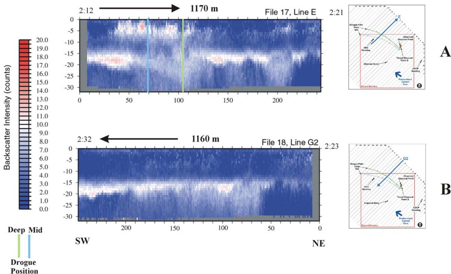
**Figure 3-17.** Profile plots of data collected from ADCP transects E and G2 on 8 April 2004 (Plume 1) displaying acoustic backscatter intensity within the water column minus the raw backscatter intensity to illustrate plume morphology 132 to 152 minutes after the dredged material disposal event at Point B.
