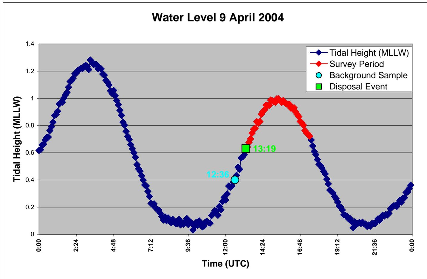
**Figure 3-20.** Water level data from the NOAA tide station in Newport, RI, corrected to the tide zone encompassing RISDS for 9 April 2004. The Background Sample and the Disposal Event are shown in comparison to the tidal stage.
