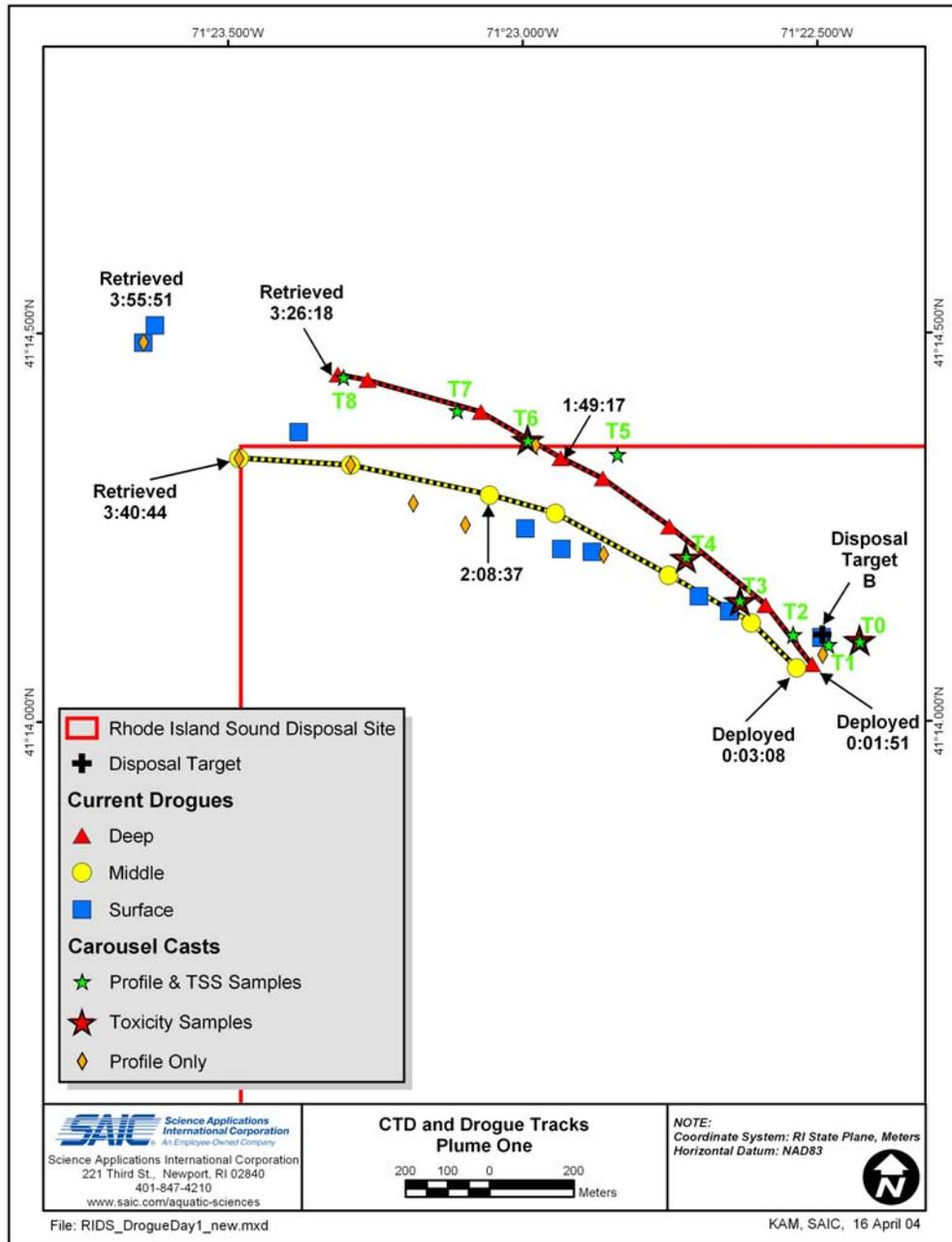
**Figure 3-2.** Map indicating current drogue trajectories and CTD cast locations during the tracking of Plume 1. Locations of water samples are also shown. Times represent elapsed time since disposal operations.
