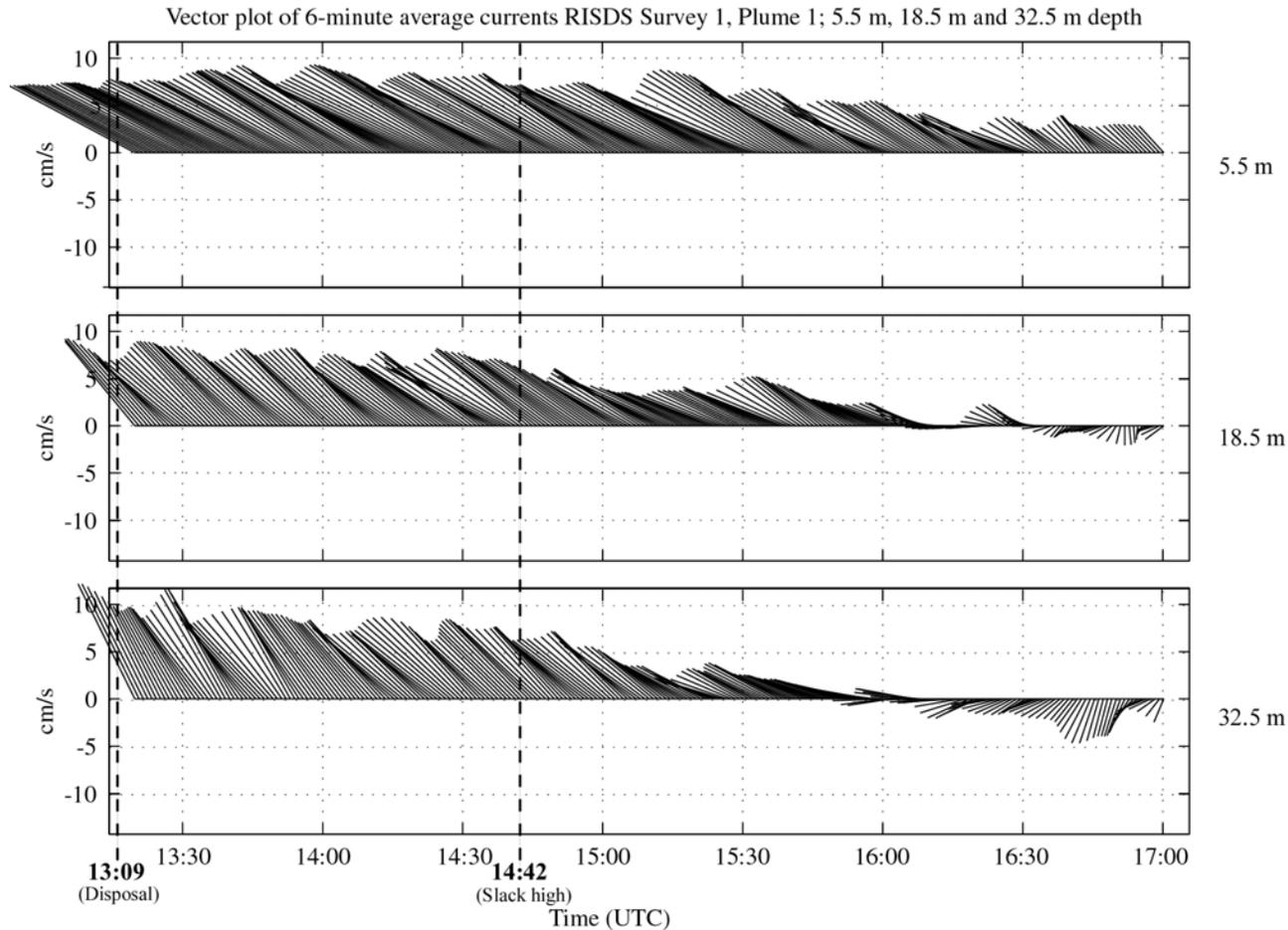
**Figure 3-5.** Time-series (UTC) plot of current vectors (six-minute low pass filtered) during Plume 1 at the near-surface level ( $\sim 5$  m; top panel), as well as the two selected drogue depth levels of  $\sim 18$  m (middle panel) and  $\sim 32$  m (bottom panel). Dashed lines represent time of disposal (13:09) and slack high tide (14:42).
