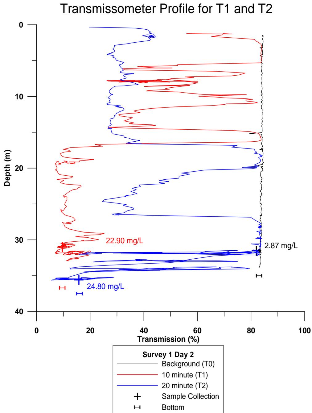
**Figure 3-26.** Profile plot of percent light transmission and sensor depth acquired during CTD sample intervals T1 and T2 during Plume 2. Locations of water sample collections within the plume are also shown.
