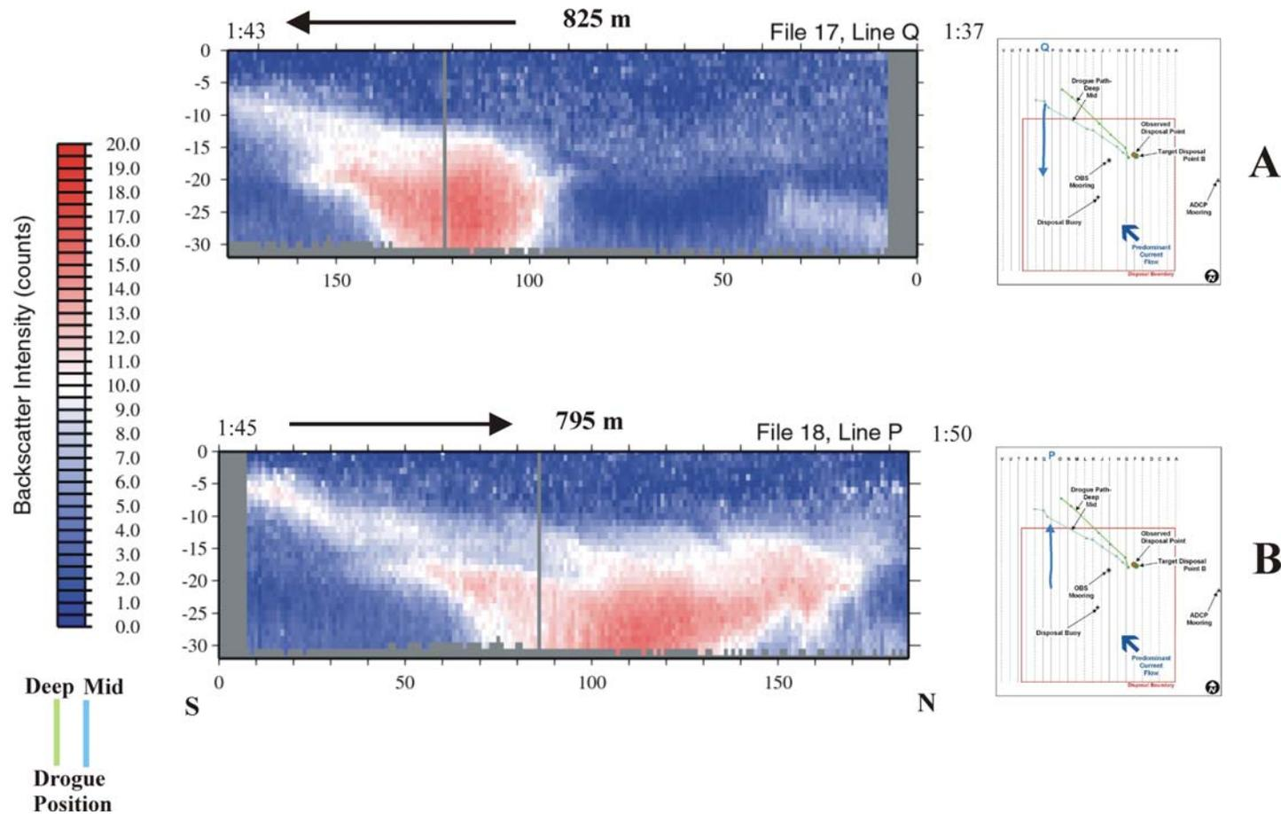
**Figure 3-55.** Profile plots of data collected from ADCP transects Q and P on 10 April 2004 (Plume 3) displaying acoustic backscatter intensity within the water column minus the raw backscatter intensity to illustrate plume morphology 97 to 110 minutes after the dredged material disposal event at Point B.
