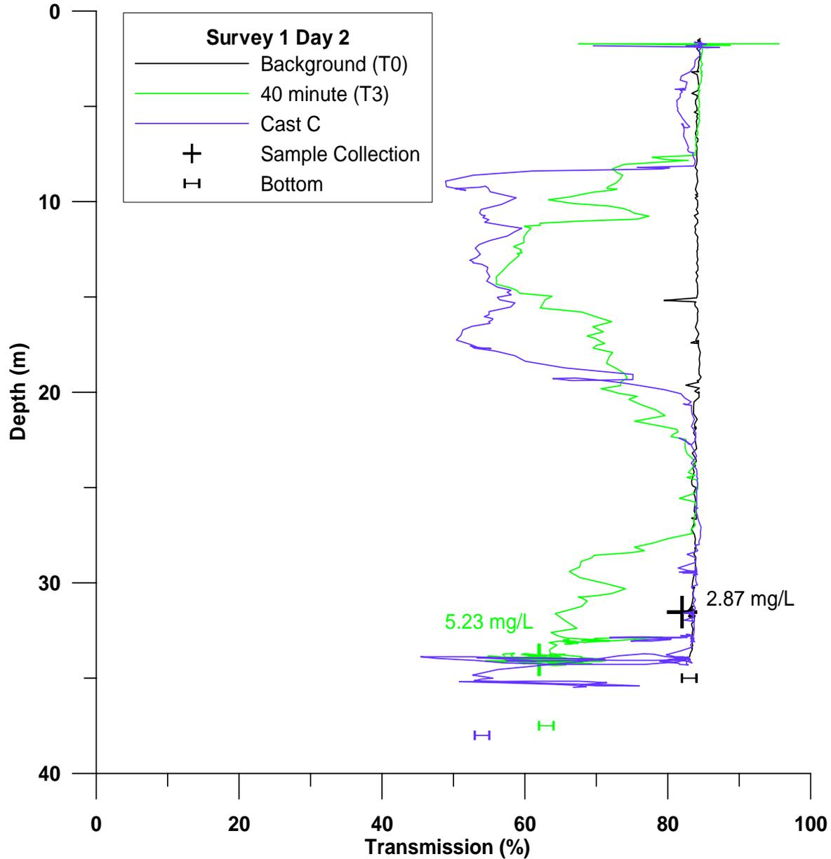
**Figure 3-27.** Profile plot of percent light transmission and sensor depth acquired during CTD sample interval T3 and Cast C for Plume 2. Locations of water sample collections within the plume are also shown.
