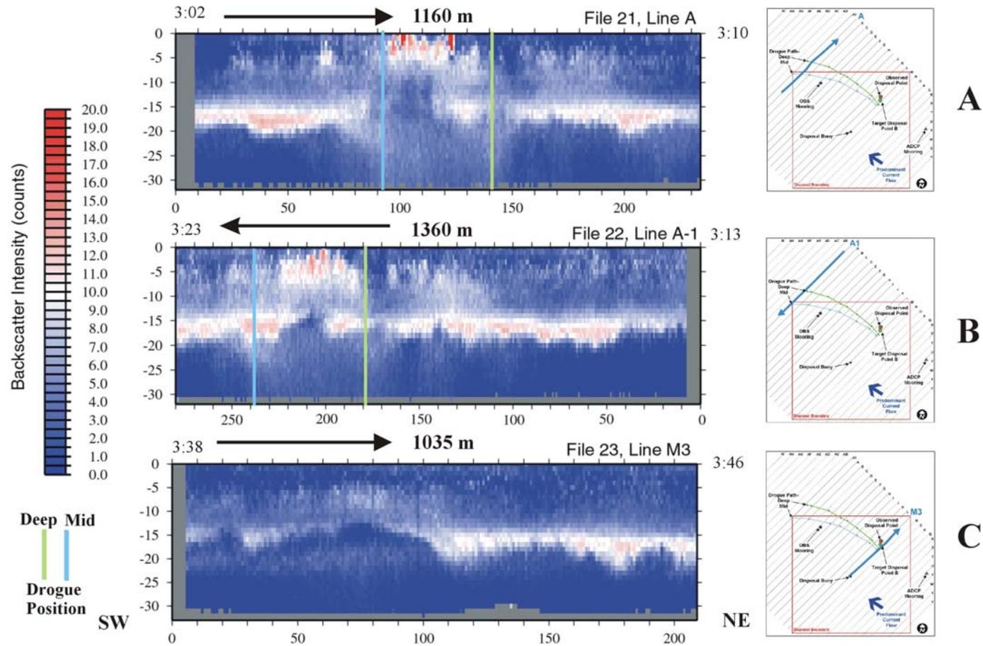
**Figure 3-18.** Profile plots of data collected from ADCP transects A, A-1 and H2 on 8 April 2004 (Plume 1) displaying acoustic backscatter intensity within the water column minus the raw backscatter intensity to illustrate plume morphology 182 to 226 minutes after the dredged material disposal event at Point B.
