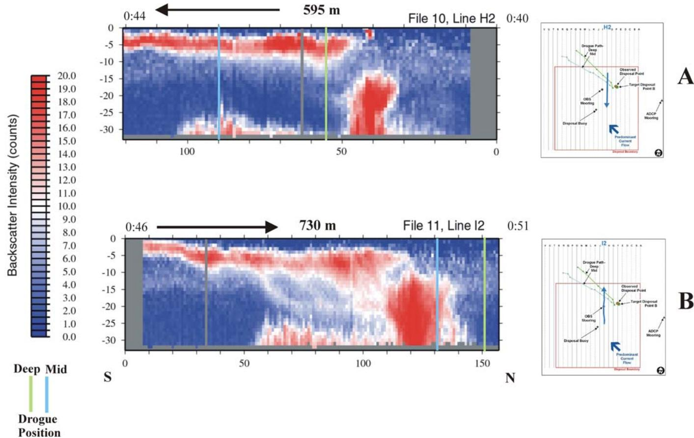
**Figure 3-54.** Profile plots of data collected from ADCP transects H2 and I2 on 10 April 2004 (Plume 3) displaying acoustic backscatter intensity within the water column minus the raw backscatter intensity to illustrate plume morphology 40 to 51 minutes after the dredged material disposal event at Point B.
