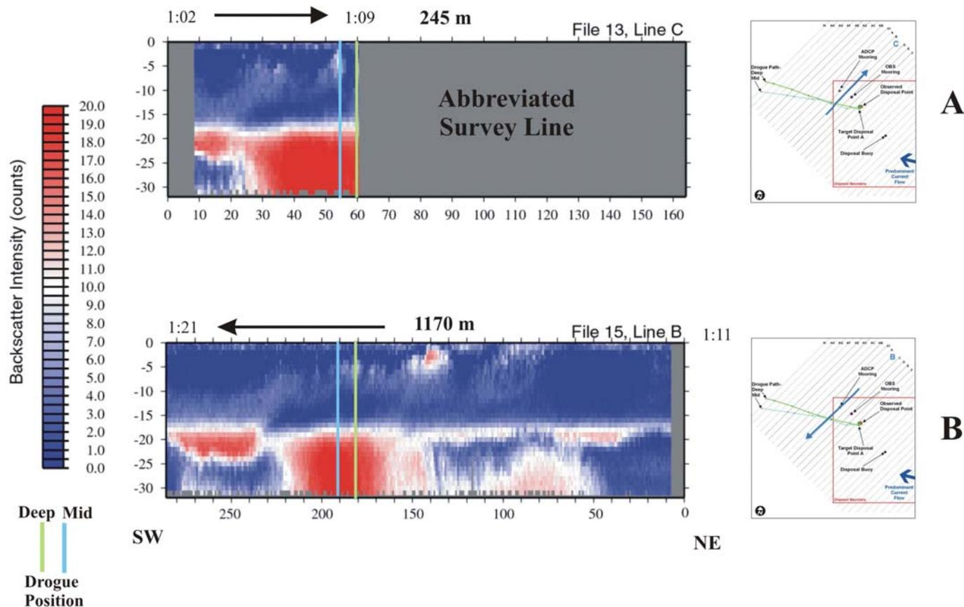
**Figure 3-34.** Profile plots of data collected from ADCP transects C and B on 9 April 2004 (Plume 2) displaying acoustic backscatter intensity within the water column minus the raw backscatter intensity to illustrate plume morphology 62 to 81 minutes after the dredged material disposal event at Point A.
