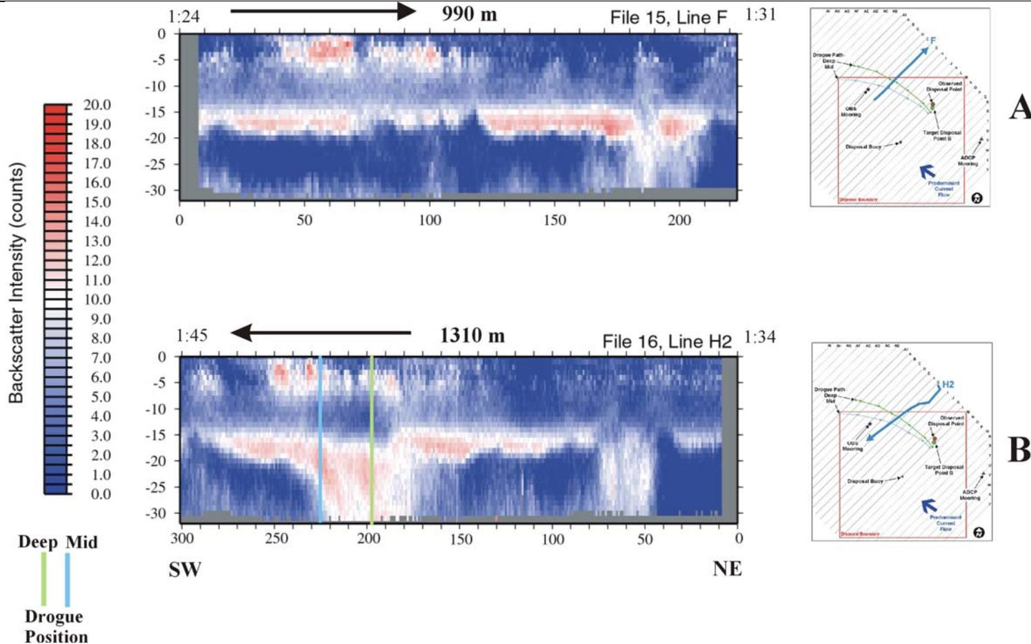
**Figure 3-16.** Profile plots of data collected from ADCP transects F and H2 on 8 April 2004 (Plume 1) displaying acoustic backscatter intensity within the water column minus the raw backscatter intensity to illustrate plume morphology 84 to 105 minutes after the dredged material disposal event at Point B.
