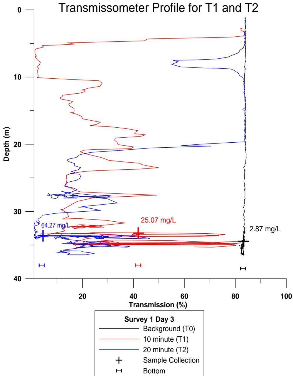
**Figure 3-46.** Profile plot of percent light transmission and sensor depth acquired during CTD sample intervals T1 and T2 during Plume 3. Locations of water sample collections within the plume are also shown.
