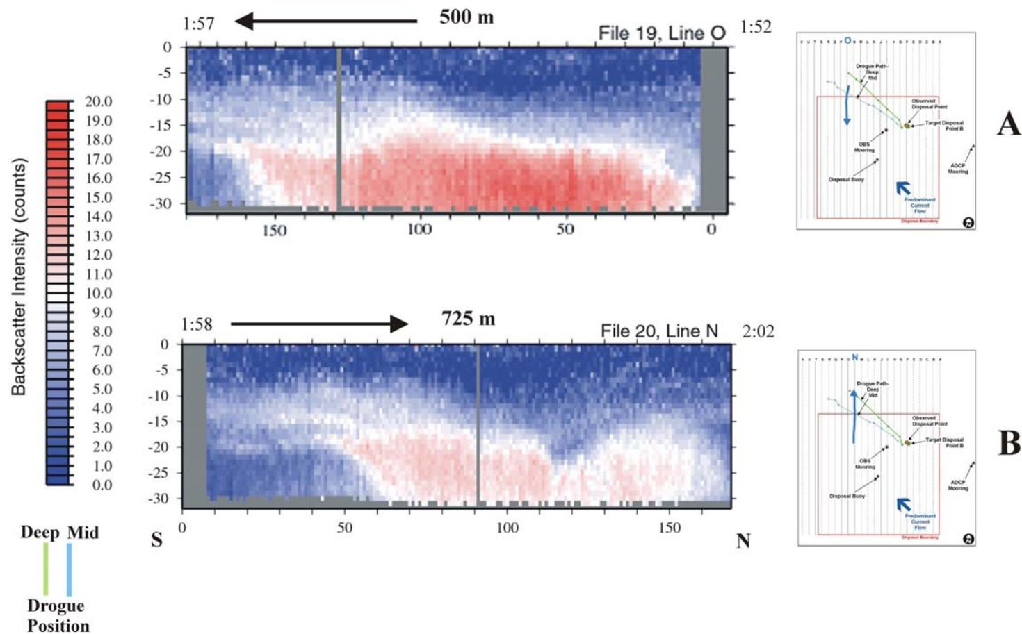
**Figure 3-56.** Profile plots of data collected from ADCP transects O and N on 10 April 2004 (Plume 3) displaying acoustic backscatter intensity within the water column minus the raw backscatter intensity to illustrate plume morphology 112 to 122 minutes after the dredged material disposal event at Point B.
