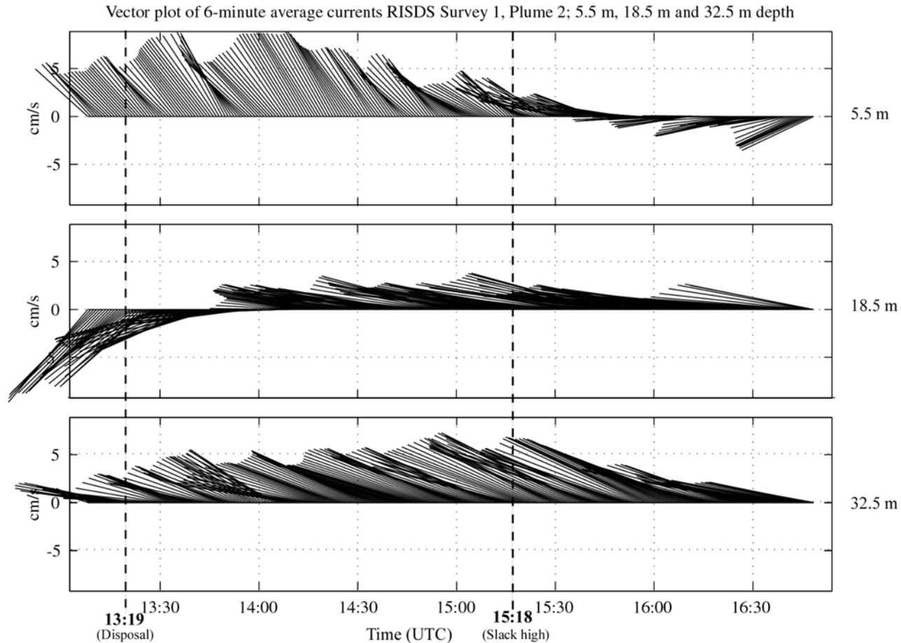
**Figure 3-24.** Time-series (UTC) plot of current vectors (six-minute LPF) during Plume 2 at the near-surface level (5.5 m; top panel) and the two selected drogue depth levels of ~18 m (middle panel) and ~32 m depth (bottom panel). Dashed line (13:09) represents barge disposal time.
