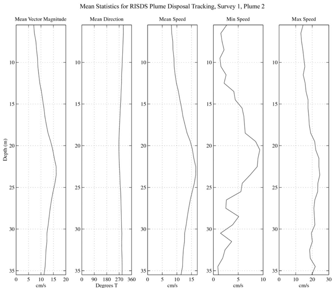
**Figure 3-22.** Statistics of moored current meter data collected on site during Plume 2 disposal monitoring activities. Current meter deployed for extent of survey period (3.5 hours). Parameters plotted include mean vector magnitude, mean vector direction, mean speed (regardless of direction), minimum speed and maximum speed.
