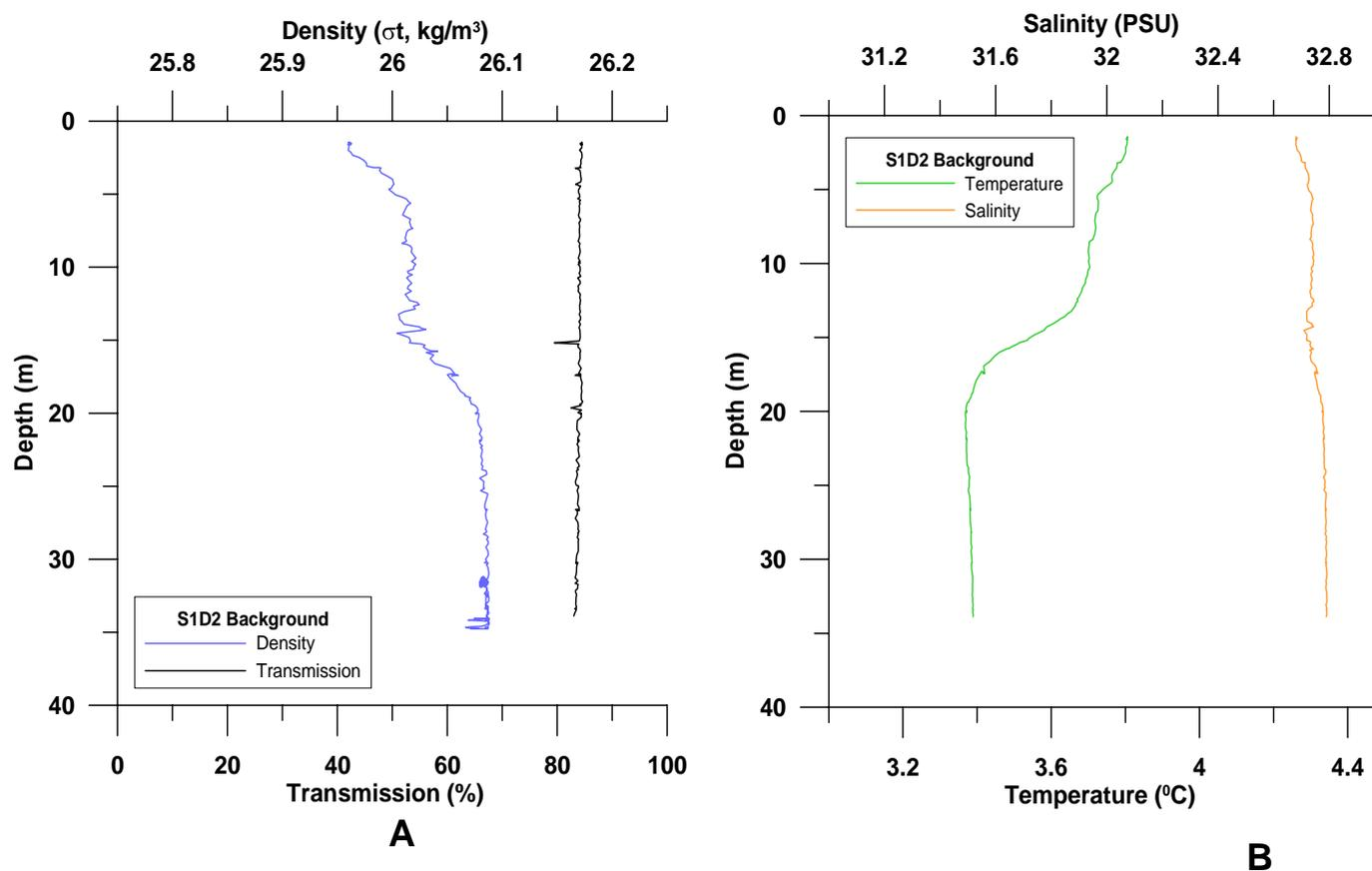
**Figure 3-25.** Profile plots of percent light transmission and seawater density versus depth (A) and temperature and salinity versus depth (B) acquired during the CTD background sample interval for Plume 2. Data are from the downcast profile only.
