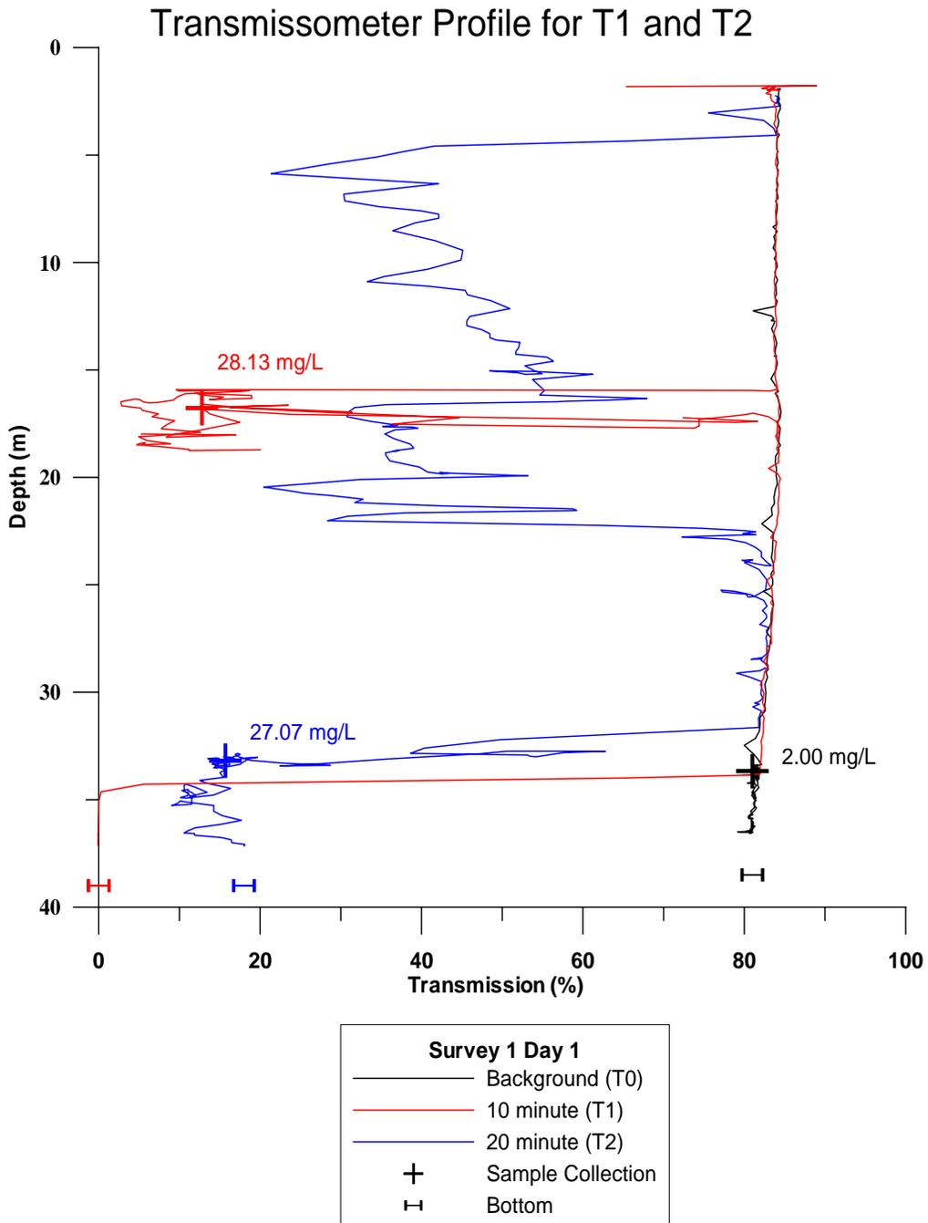
**Figure 3-7.** Profile plot of percent light transmission and sensor depth acquired during CTD sample intervals T1 and T2 for Plume 1. Locations of water sample collections within the plume are also shown.
