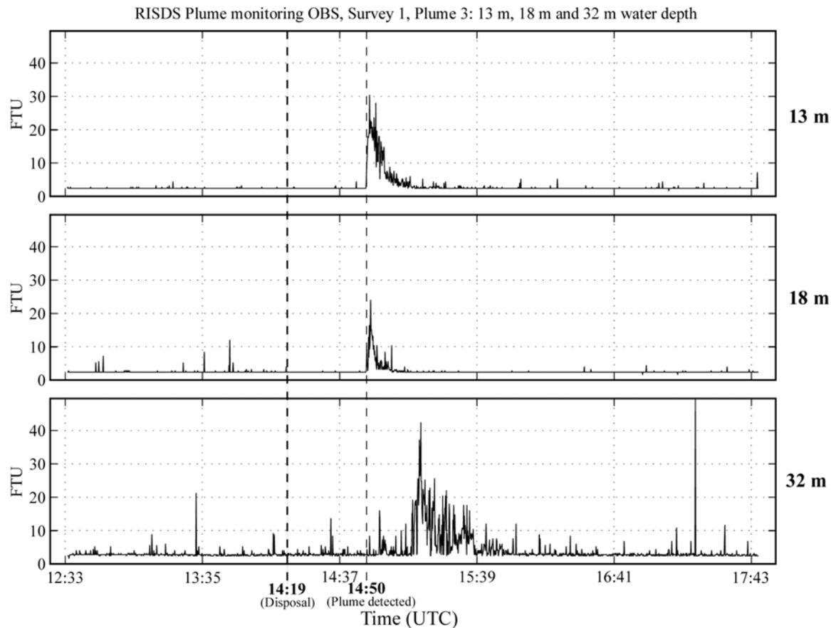
**Figure 3-59.** Time-series (UTC) plot of OBS data collected on 10 April 2004 (Plume 3) from three levels in the water column (13 m, 18 m, and 32 m), displaying changes in turbidity (FTU) over time resulting from sediment plume passage. Dashed lines represent barge disposal time (14:19) and an increase in suspended sediment (14:50), indicating the possible of the leading edge of the plume.
