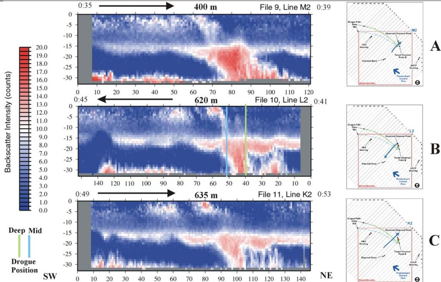
**Figure 3-14.** Profile plots of data collected from ADCP transects M2, L2, and K2 on 8 April 2004 (Plume 1) displaying acoustic backscatter intensity within the water column minus the raw backscatter intensity to illustrate plume morphology 35 to 53 minutes after the dredged material disposal event at Point B.
