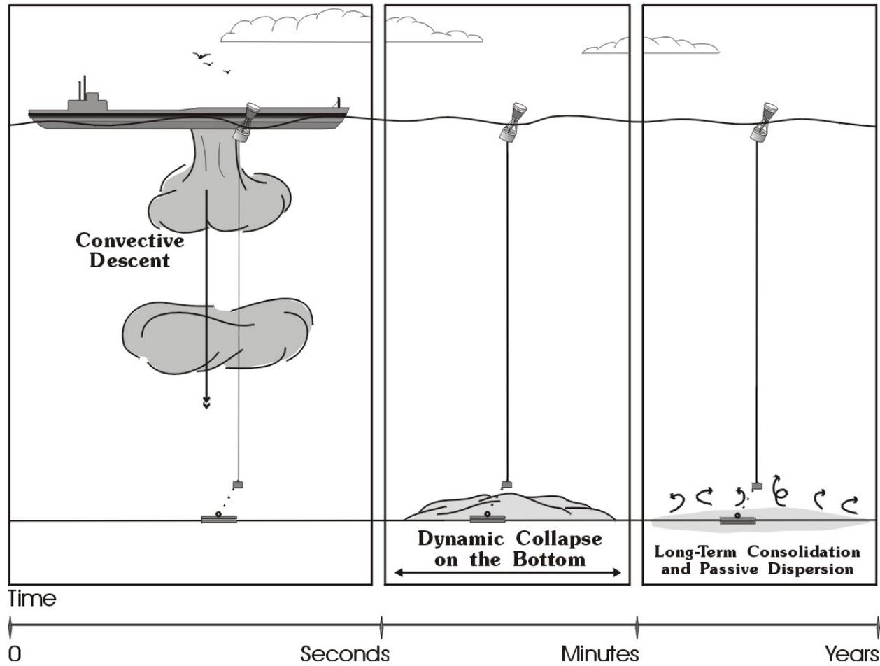
**Figure 1-4.** Schematic diagram of the three phases of descent encountered during a dredged material disposal event.
