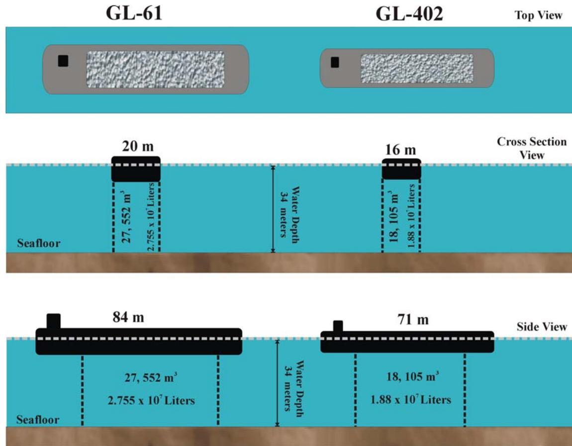
**Figure 5-3.** Scaled drawing depicting the size of the 6,000 yd<sup>3</sup> and 4,000 yd<sup>3</sup> barge relative to the depth of water over RISDS and the volume of water within the barge footprint for the initial mixing of sediments entrained within the water column during a typical disposal event.
