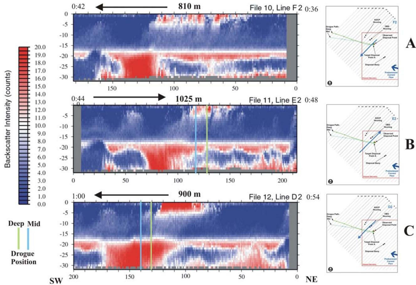
**Figure 3-33.** Profile plots of data collected from ADCP transects F2, E2, and D2 on 9 April 2004 (Plume 2) displaying acoustic backscatter intensity within the water column minus the raw backscatter intensity to illustrate plume morphology 36 to 60 minutes after the dredged material disposal event at Point A.
