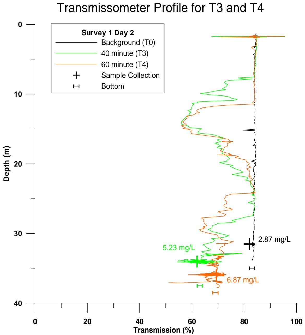
**Figure 3-28.** Profile plot of percent light transmission and sensor depth acquired during CTD sample intervals T3 and T4 for Plume 2. Locations of water sample collections within the plume are also shown.
