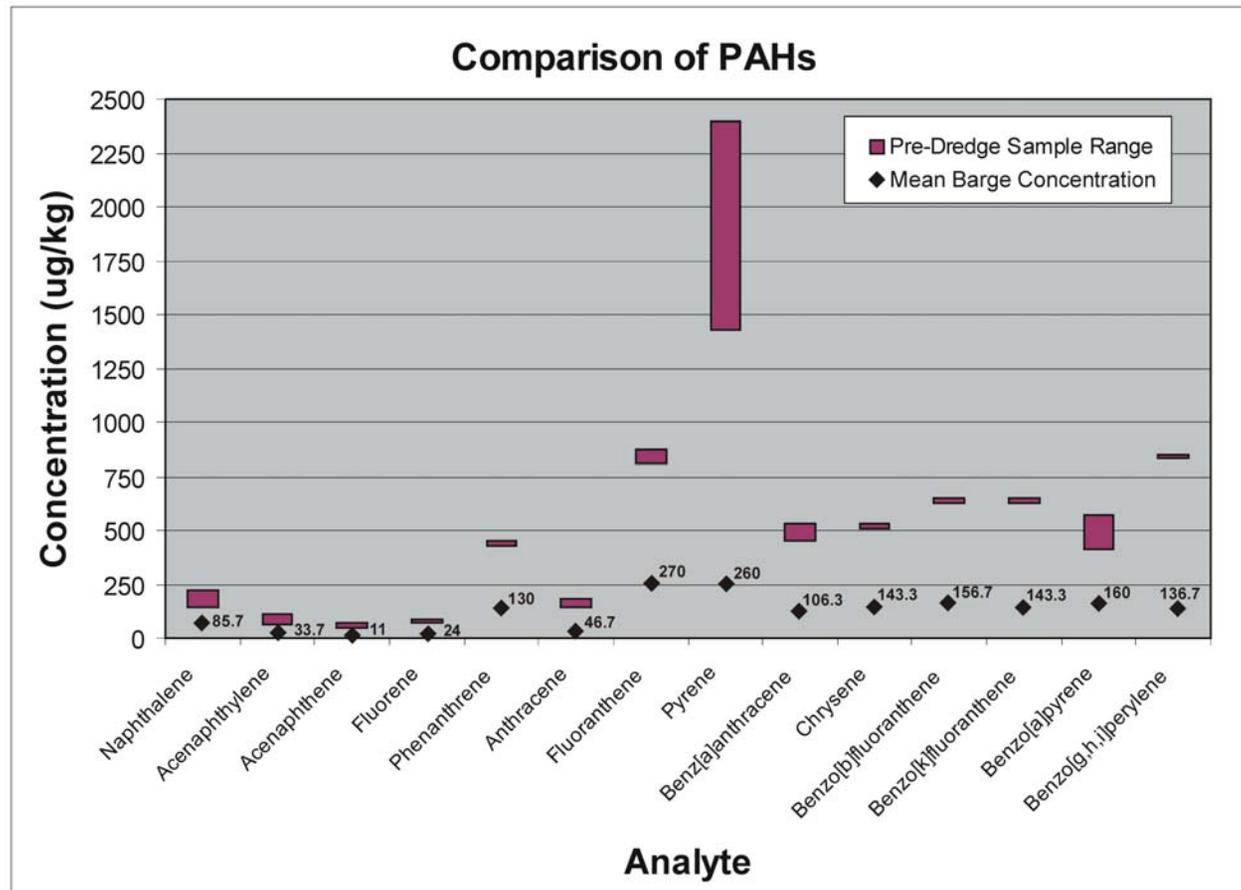
**Figure 5-8.** Chart showing the relationship between the mean concentrations of PAH compounds in the April 2004 disposal barge samples to the range of concentrations detected in the 1992 and 1994 pre-dredge samples of in-place sediments within Sabin Point Reach.
