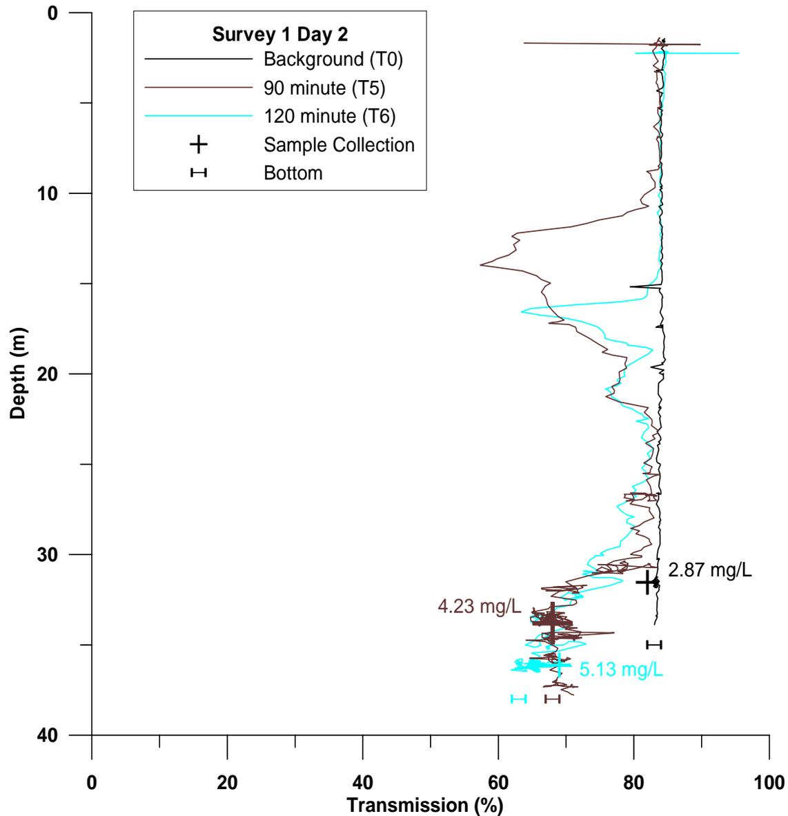
**Figure 3-29.** Profile plot of percent light transmission and sensor depth acquired during CTD sample intervals T5 and T6 for Plume 2. Locations of water sample collections within the plume are also shown.
