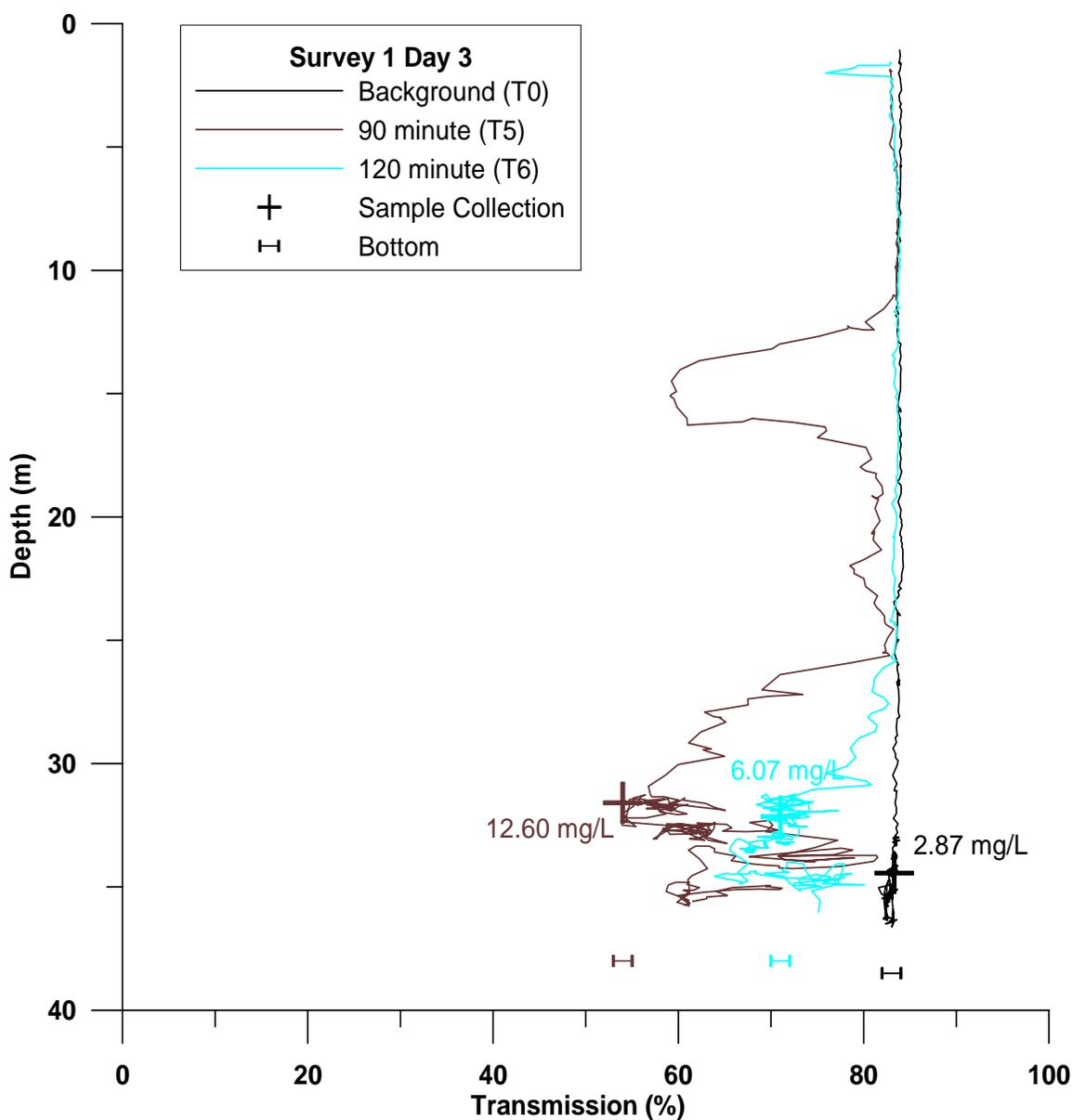
**Figure 3-48.** Profile plot of percent light transmission and sensor depth acquired during CTD sample intervals T5 and T6 for Plume 3. Locations of water sample collections within the plume are also shown.
