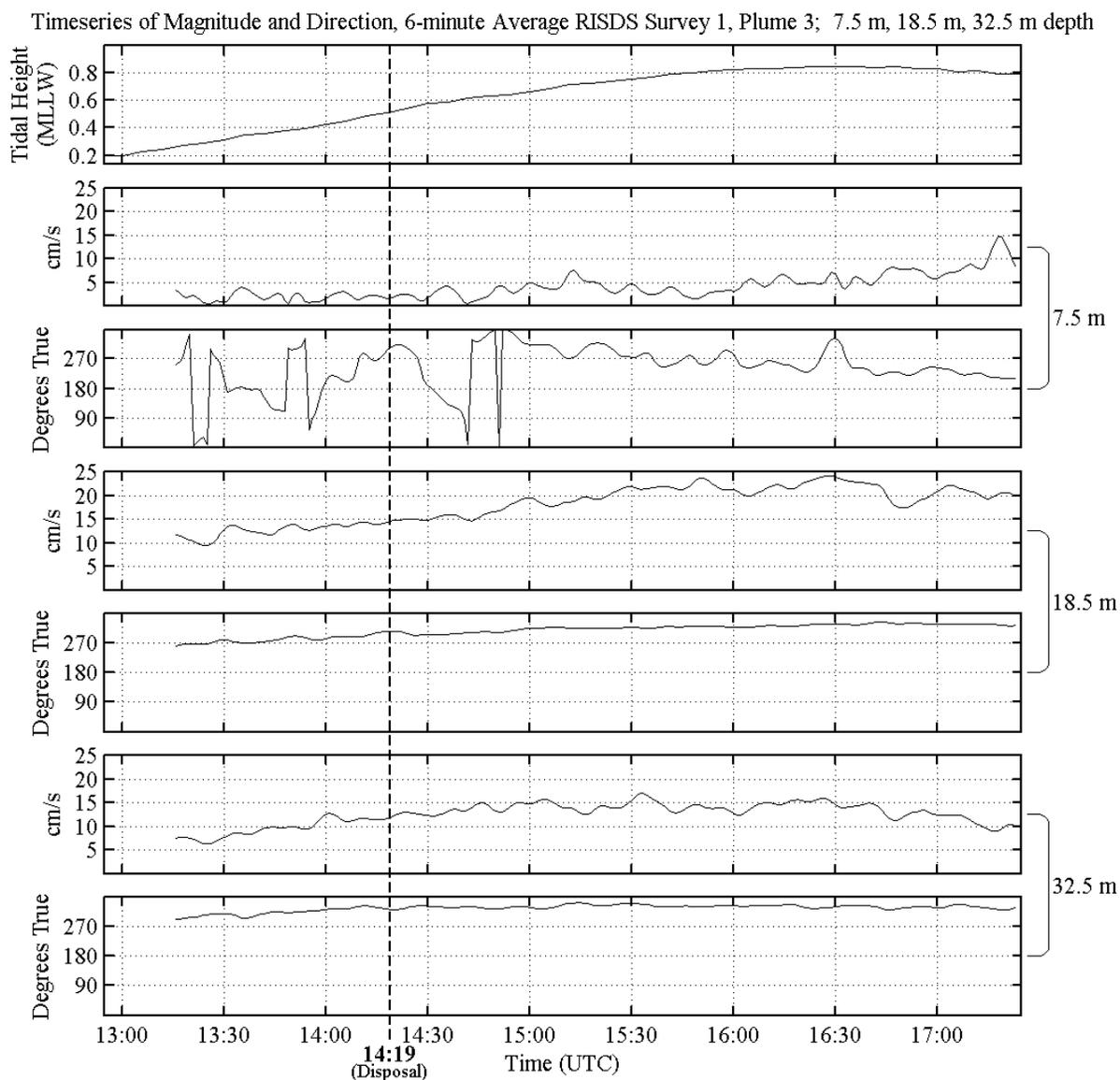
**Figure 3-43.** Time-series (UTC) plot of current magnitude and direction during Plume 3 at the near-surface level (top two panels) and the two selected drogue depth levels of ~18m (middle two panels) and ~32m depth (bottom two panels). Currents were sampled at 1min intervals, and filtered with 6-min Low Pass Filter (LPF) to reduce high-frequency noise. Dashed line (14:19) represents barge disposal time.
