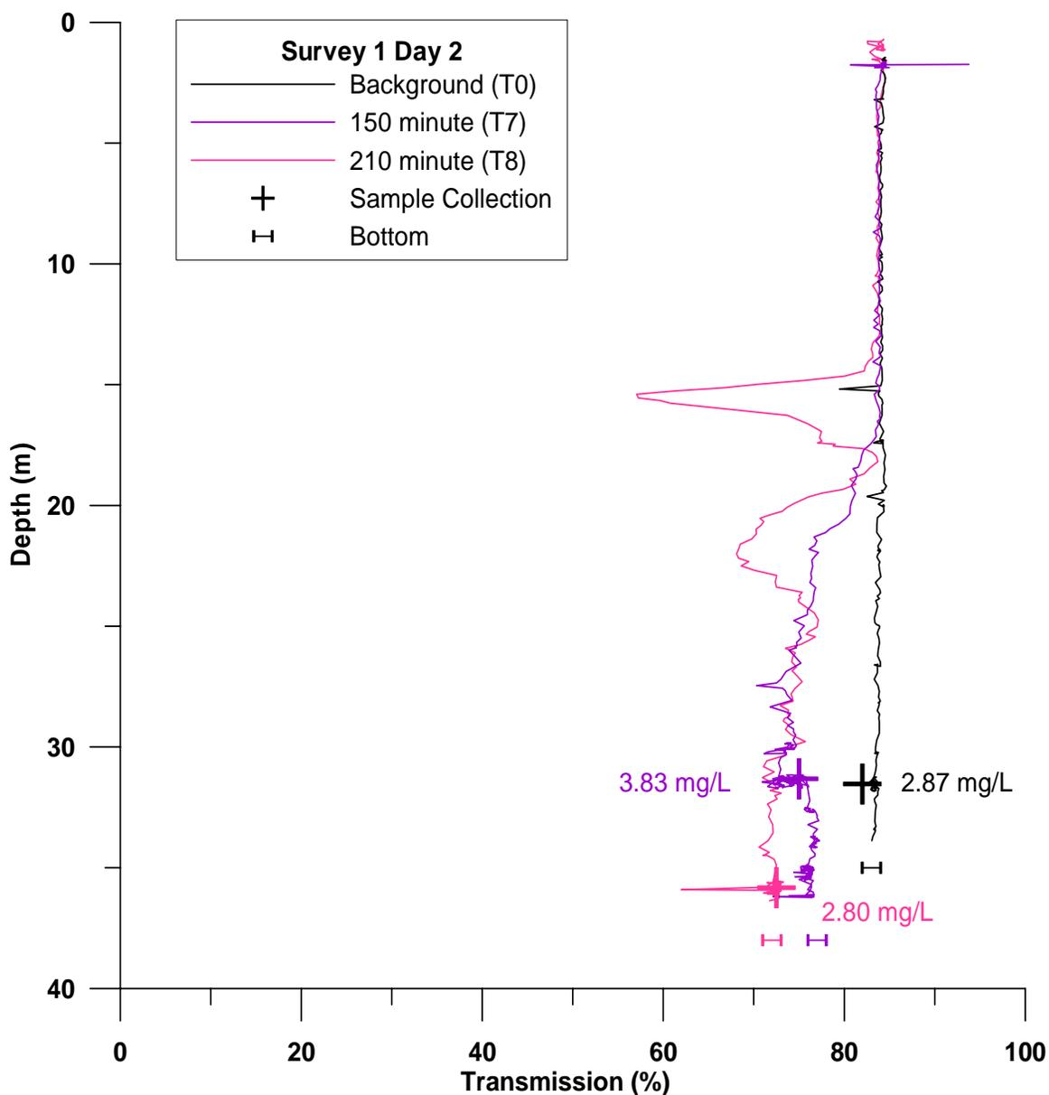
**Figure 3-30.** Profile plot of percent light transmission and sensor depth acquired during CTD sample intervals T7 and T8 for Plume 2. Locations of water sample collections within the plume are also shown.
