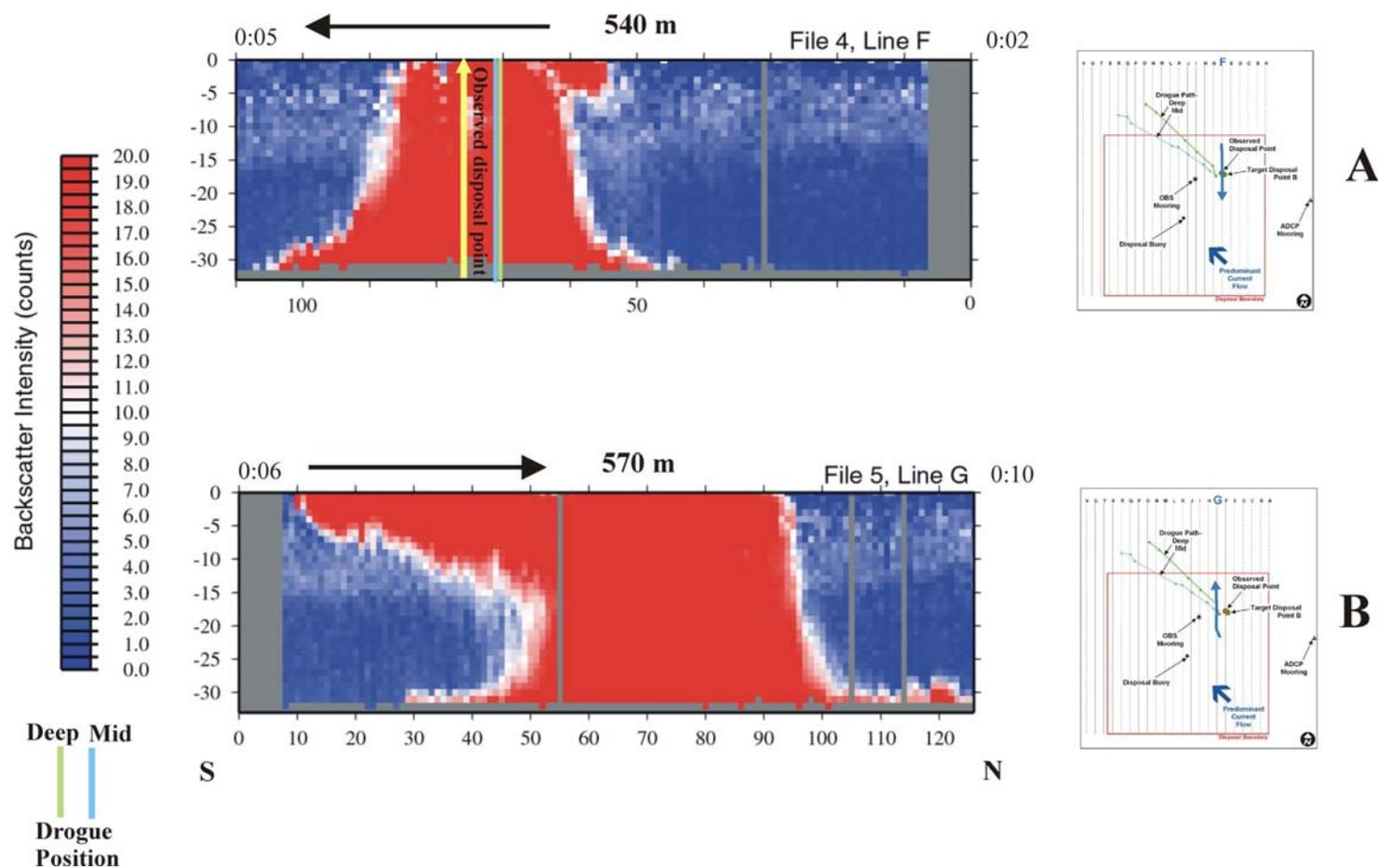
**Figure 3-51.** Profile plots of data collected from ADCP transects F and G on 10 April 2004 (Plume 3) displaying acoustic backscatter intensity within the water column minus the raw backscatter intensity to illustrate plume morphology 2 to 10 minutes after the dredged material disposal event at Point B.
