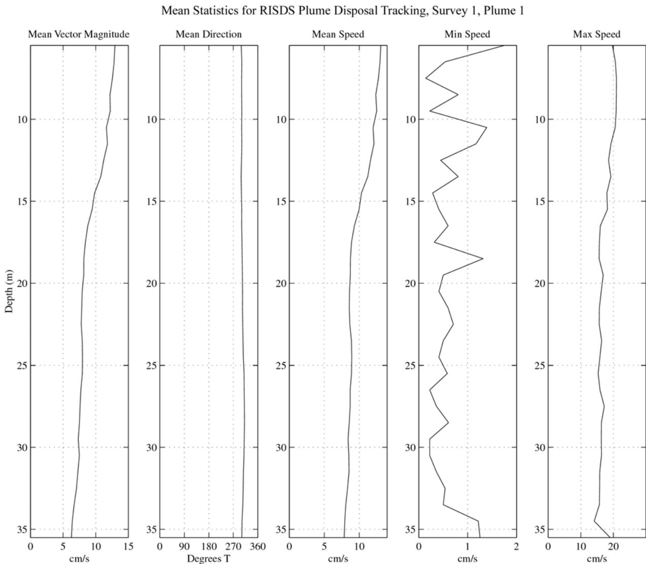
**Figure 3-3.** Statistics of moored current meter data collected on site during Plume 1 disposal monitoring activities. Current meter deployed for extent of survey period (3.5 hours). Parameters plotted include mean vector magnitude, mean vector direction, mean speed (regardless of direction), minimum speed and maximum speed.
