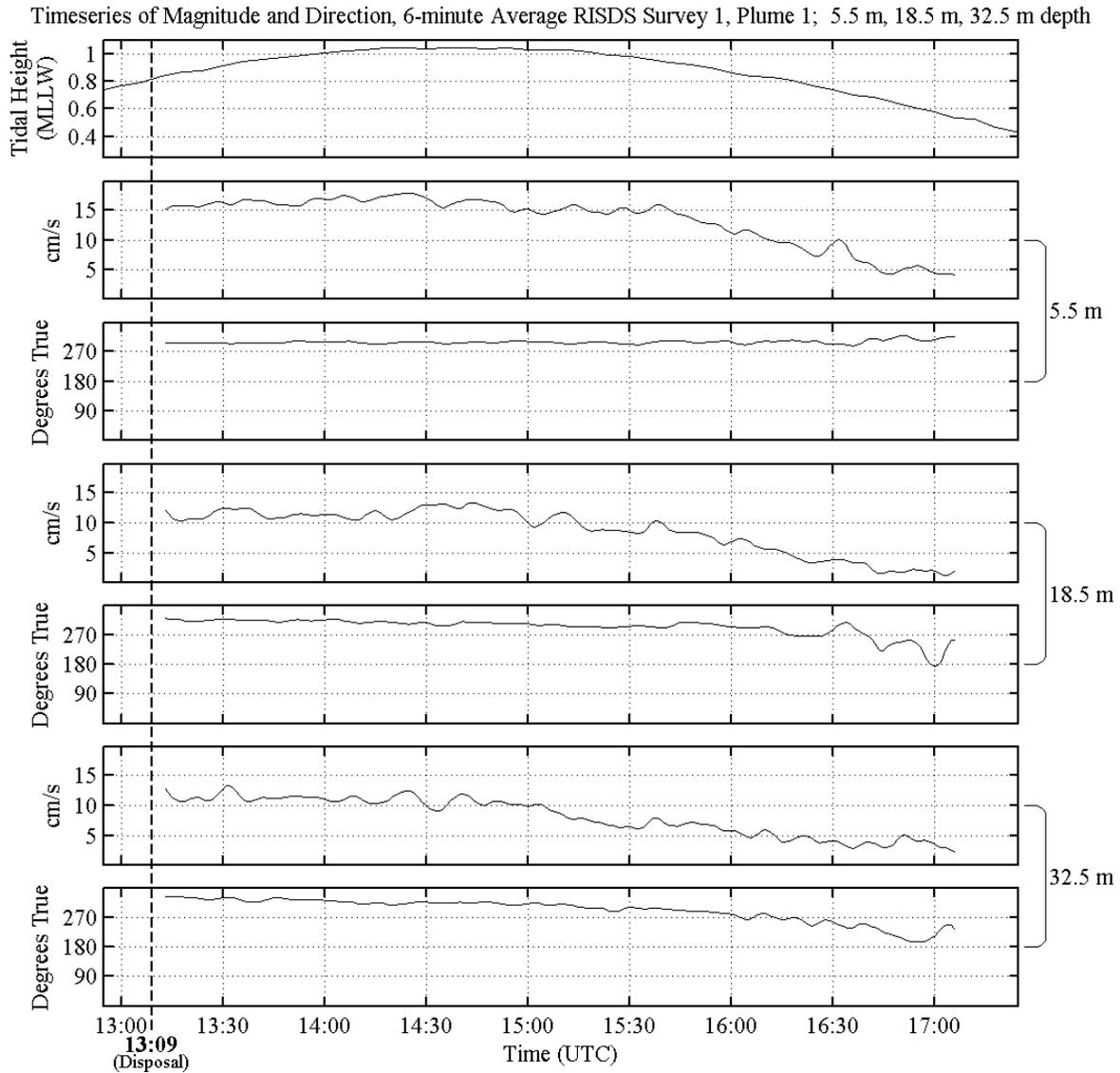
**Figure 3-4.** Time-series (UTC) plot of current magnitude and direction during Plume 1 at the near-surface level ( $\sim 5$  m; top two panels) and the two selected drogue depth levels of  $\sim 18$  m (middle two panels) and  $\sim 32$  m depth (bottom two panels). Currents were sampled at one-minute intervals, and filtered with six-minute Low Pass Filter (LPF) to reduce high-frequency noise. Dashed line (13:09) represents the start of barge disposal.
