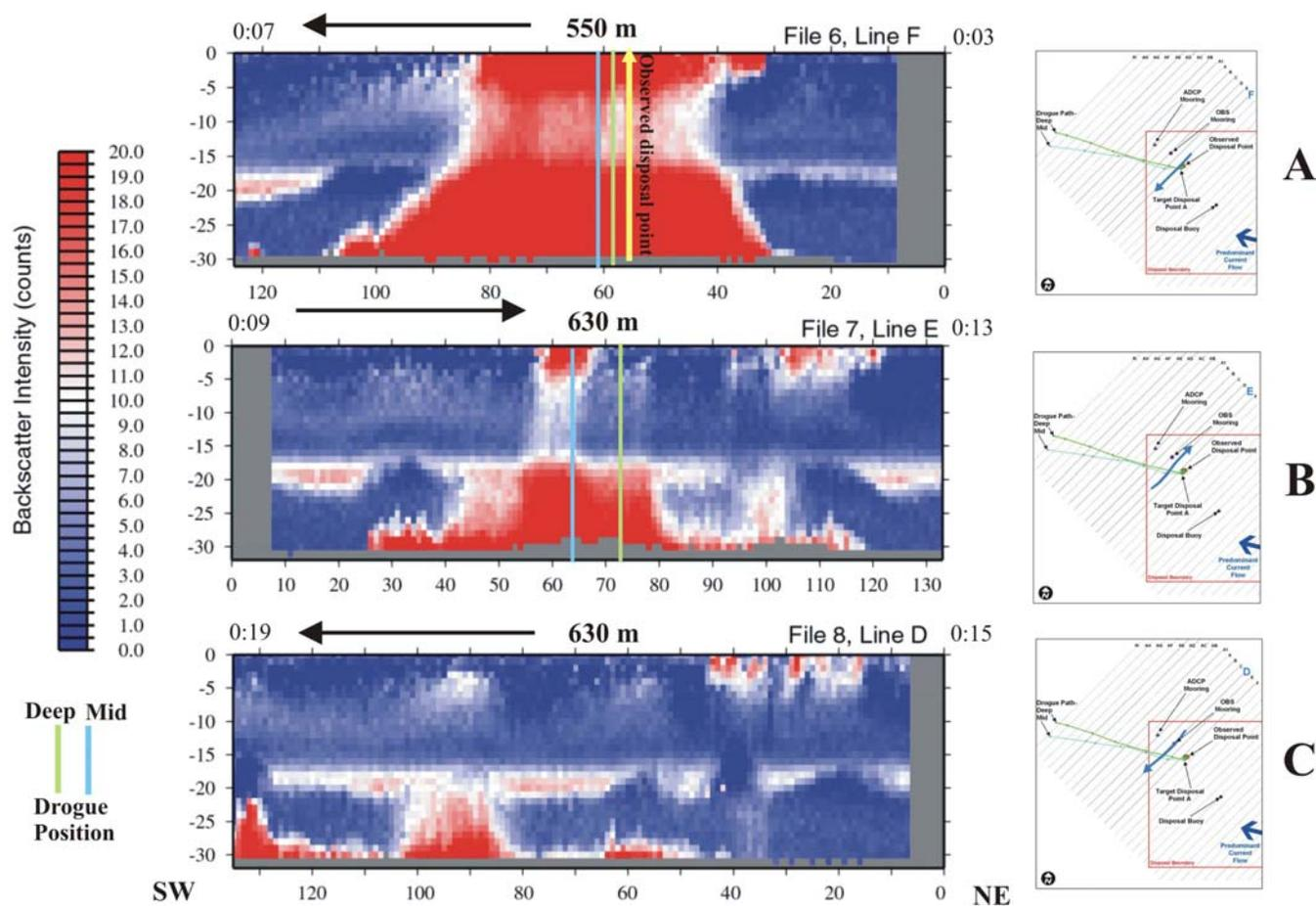
**Figure 3-32.** Profile plots of data collected from ADCP transects F, E, and D on 9 April 2004 (Plume 2) displaying acoustic backscatter intensity within the water column minus the raw backscatter intensity to illustrate plume morphology 3 to 19 minutes after the dredged material disposal event at Point A.
