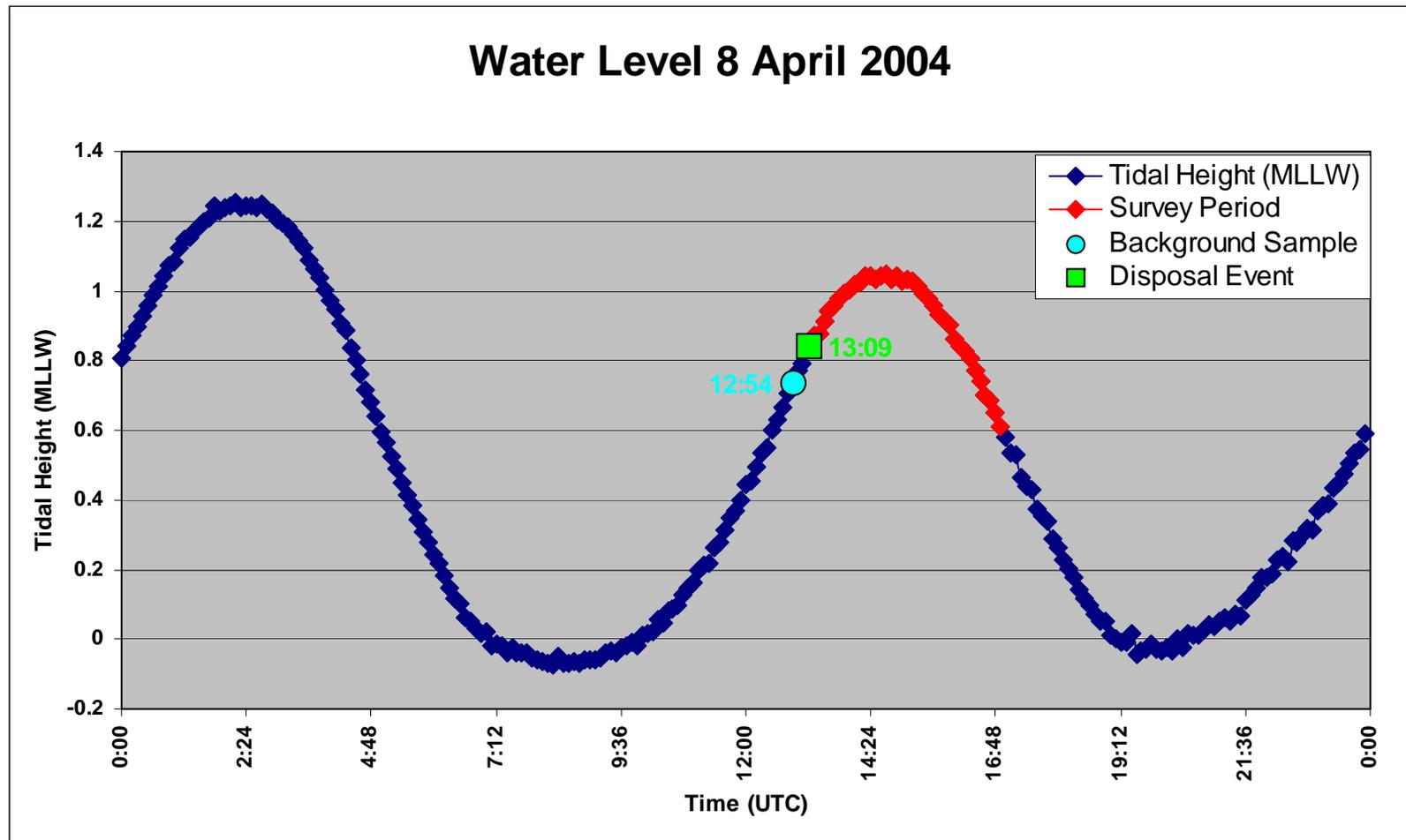
**Figure 3-1.** Water level data from the NOAA tide station in Newport, RI, corrected to the tide zone encompassing RISDS for 8 April 2004. The Background Sample and the Disposal Event are shown in comparison to the tidal stage.
