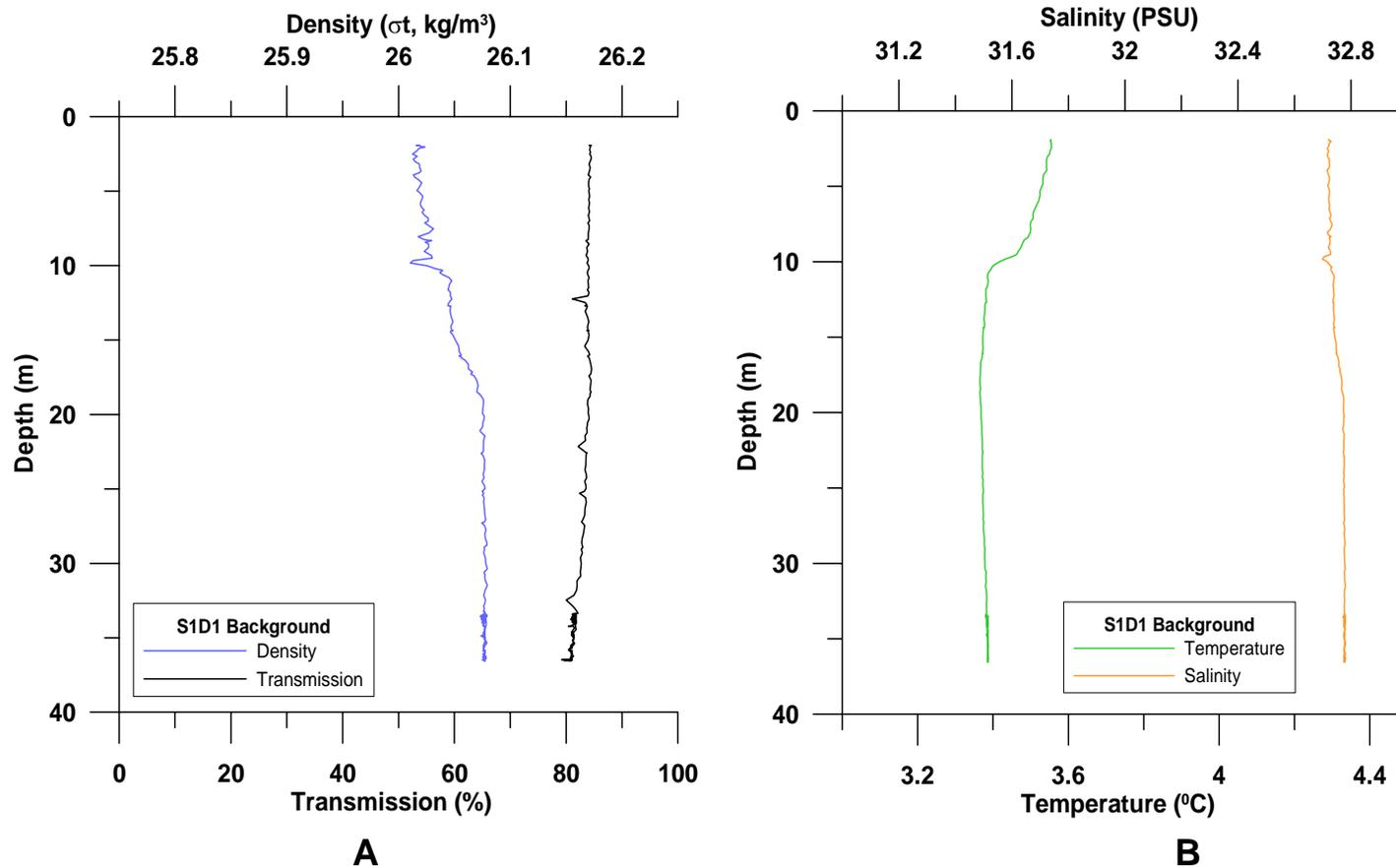
**Figure 3-6.** Profile plots of percent light transmission and seawater density versus depth (A) and temperature and salinity versus depth (B) acquired during the CTD background sample interval for Plume 1. Data are from the downcast profile only.
