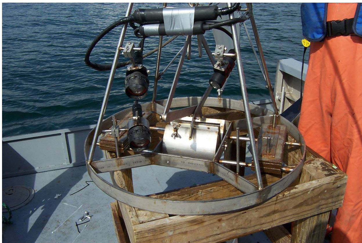
Figure 2-2. Video-assisted sediment grab sampler used at WIHS, 2003
