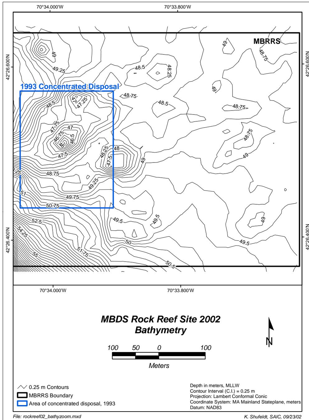
**Figure 3-2.** Bathymetric chart focusing on the center and eastern portions of MBRRS showing bottom features on the Massachusetts Bay seafloor formed by the deposition of rock, 0.25 m contour interval
