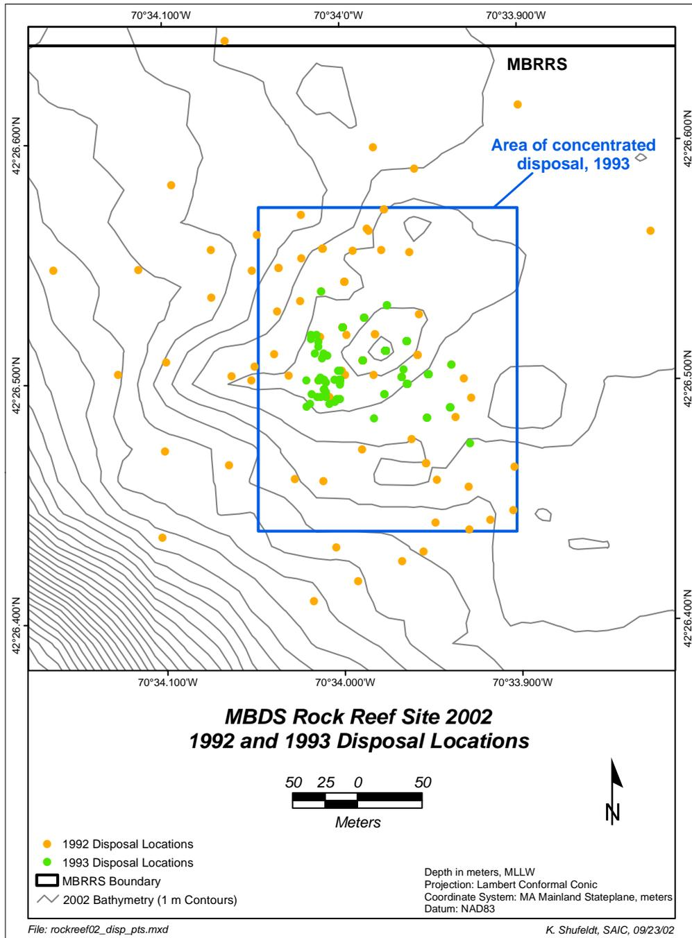
**Figure 1-3.** Reported positions of the rock placement events at MBRRS between June 1992 and October 1993 as recorded in barge disposal logs. The blue box represents the area of concentrated rock disposal for 1993.
