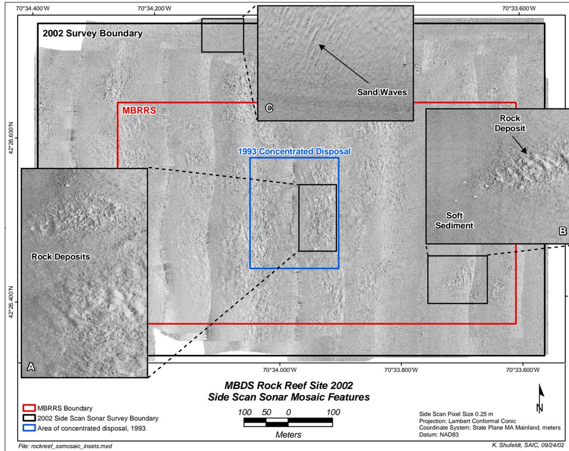
**Figure 3-7.** Results of side-scan sonar imagery collected over MBRRS showing seafloor composition over the area of concentrated disposal (A), contrast in acoustic signature between soft ambient sediments and a single rock deposit (B), and the presence of sand waves along the northern margin of the survey area (C)
