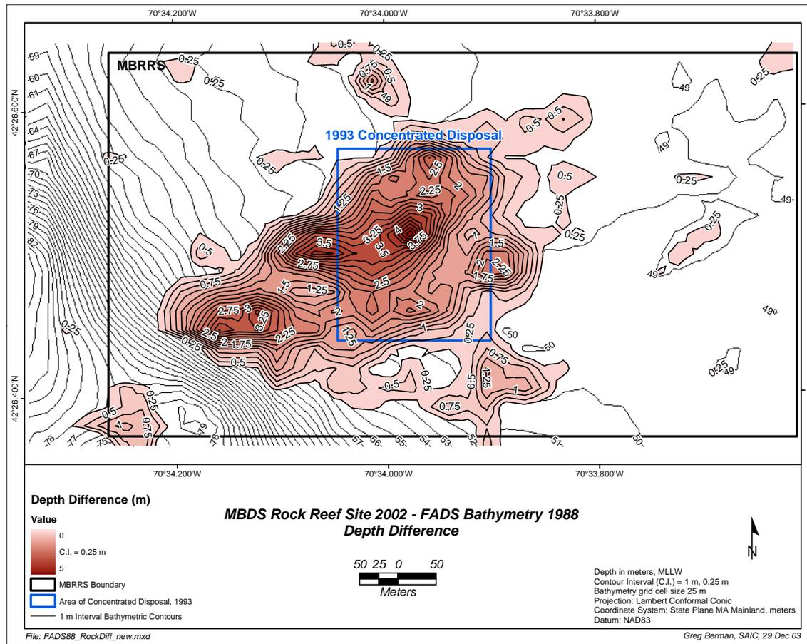
**Figure 3-4.** Depth difference comparison between the June 2002 and November 1998 bathymetric surveys displaying the morphology of the rock reef structure constructed on Stellwagen Bank in 1992 and 1993, 0.25 m contour interval
