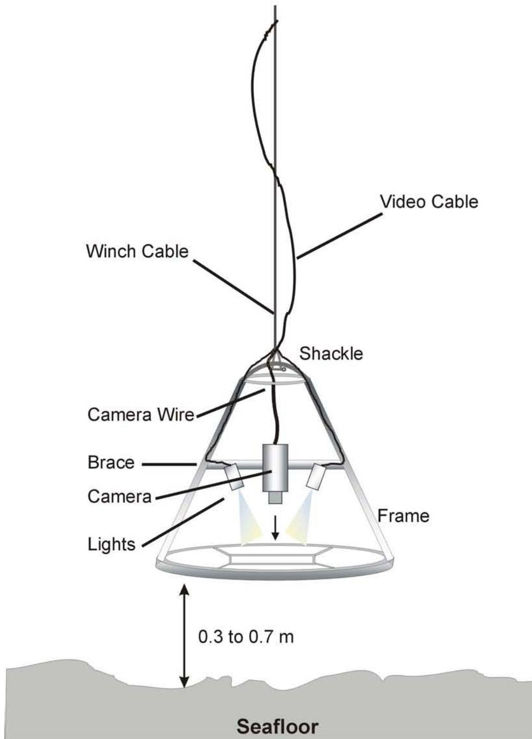
**Figure 2-3.** Schematic diagram of the Outland drop video system used to evaluate benthic conditions over the rock deposits within MBRRS
