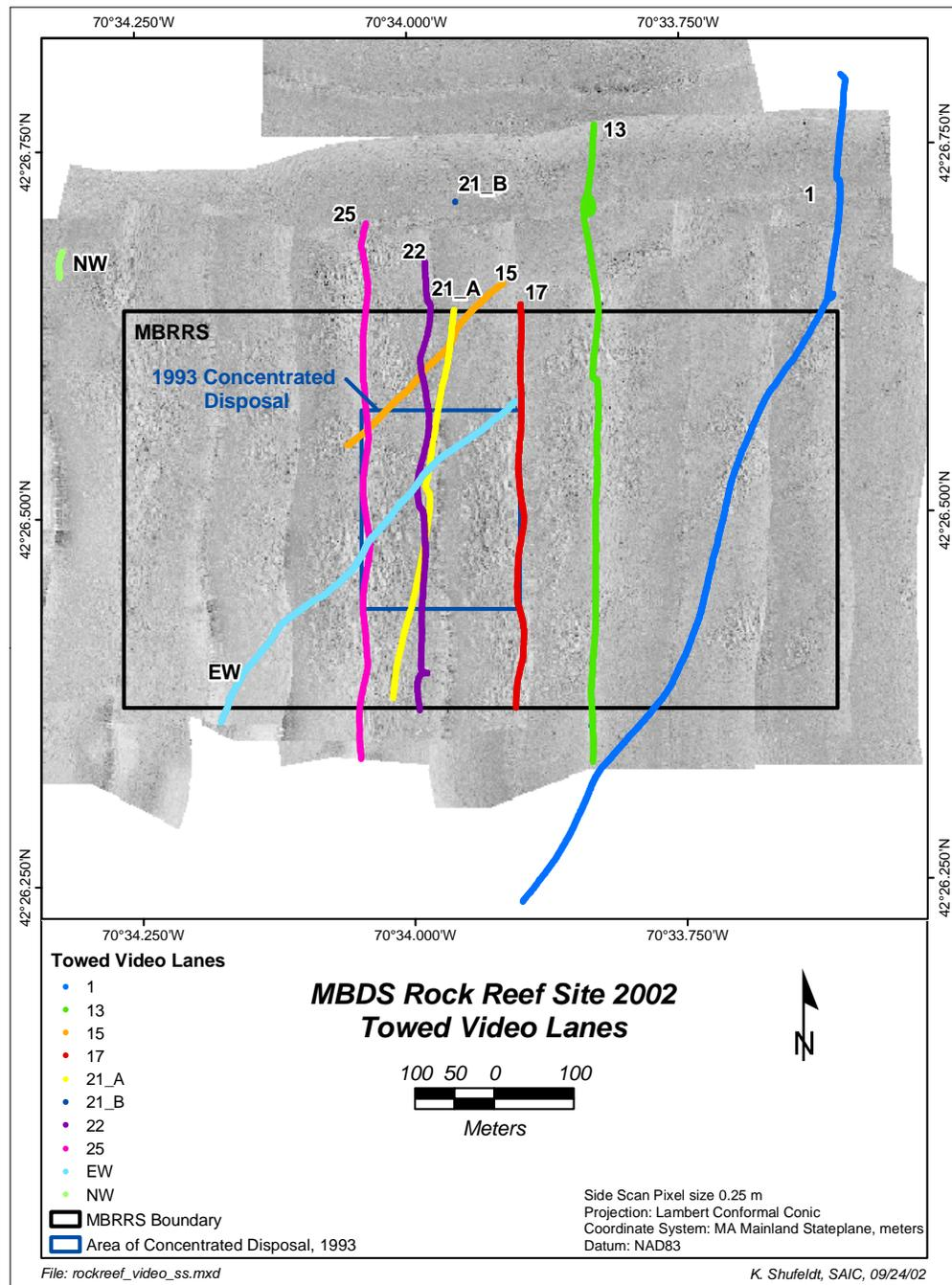
**Figure 2-2.** Color-coded track lines occupied over MBRRS as part of the July 2002 drop video survey. The track lines are overlaid on the side-scan sonar mosaic from Figure 3-5.
