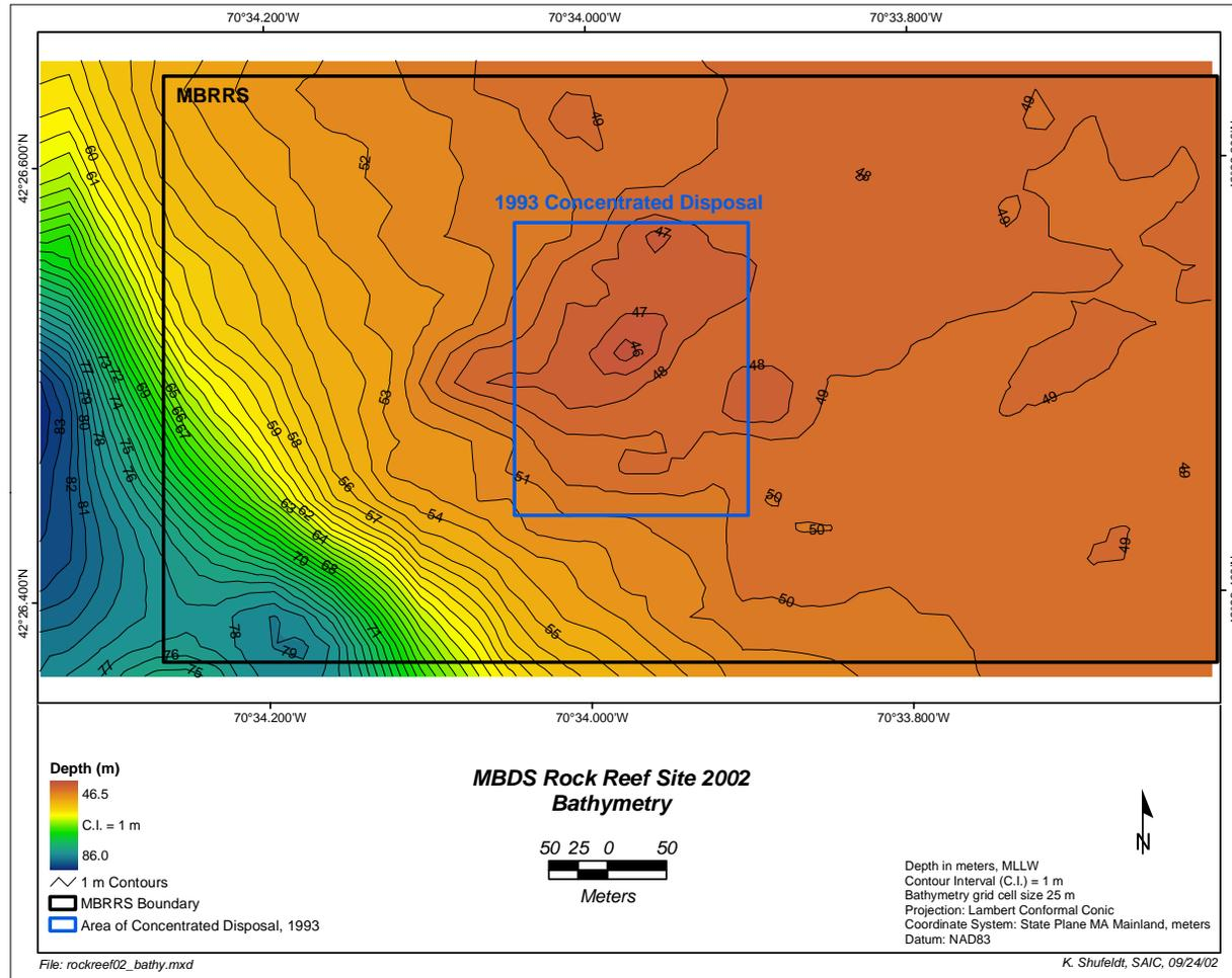
**Figure 3-1.** Bathymetric chart showing the range of water depths detected over MBRRS and the surrounding area during the 2002 monitoring survey, 1.0 m contour interval
