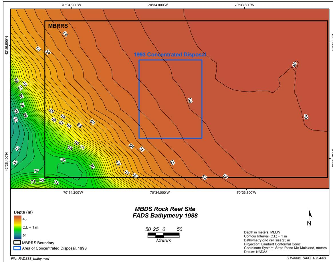
**Figure 3-3.** Bathymetric chart of the area surrounding MBRRS displaying seafloor topography as detected during the November 1988 master bathymetric survey of the Foul Area Disposal Site (FADS) prior to the placement of rock material, 1.0 m contour interval
