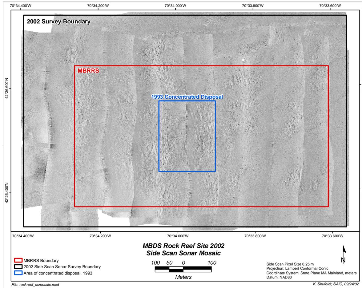
**Figure 3-6.** Side-scan sonar mosaic developed for MBRRS showing differences in surface texture and strength of acoustic return due to the presence of rock deposits on the seafloor
