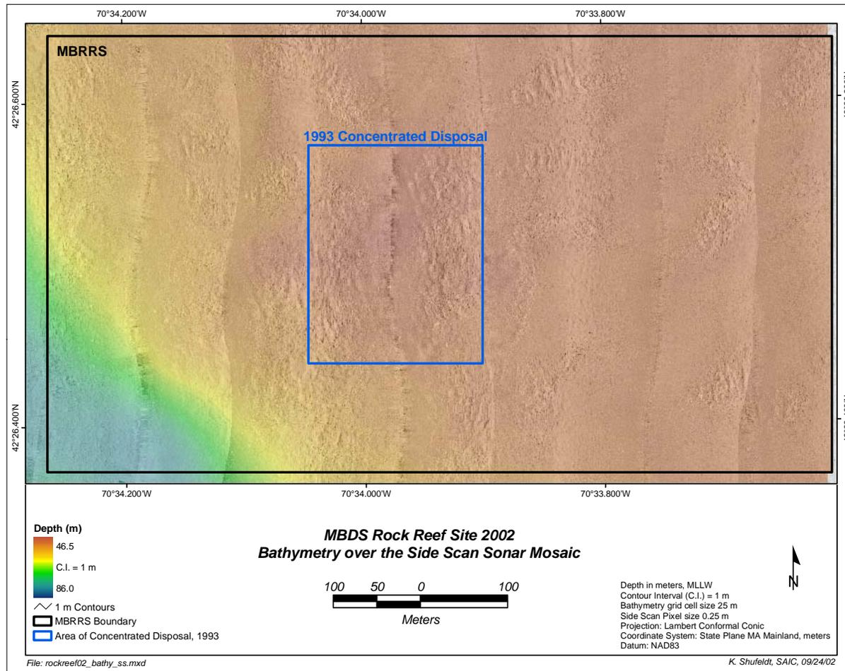
**Figure 3-8.** Composite graphic displaying the side-scan sonar mosaic overlain by bathymetry data to examine the relationship between seafloor topography and seafloor composition, 1 m color gradient
