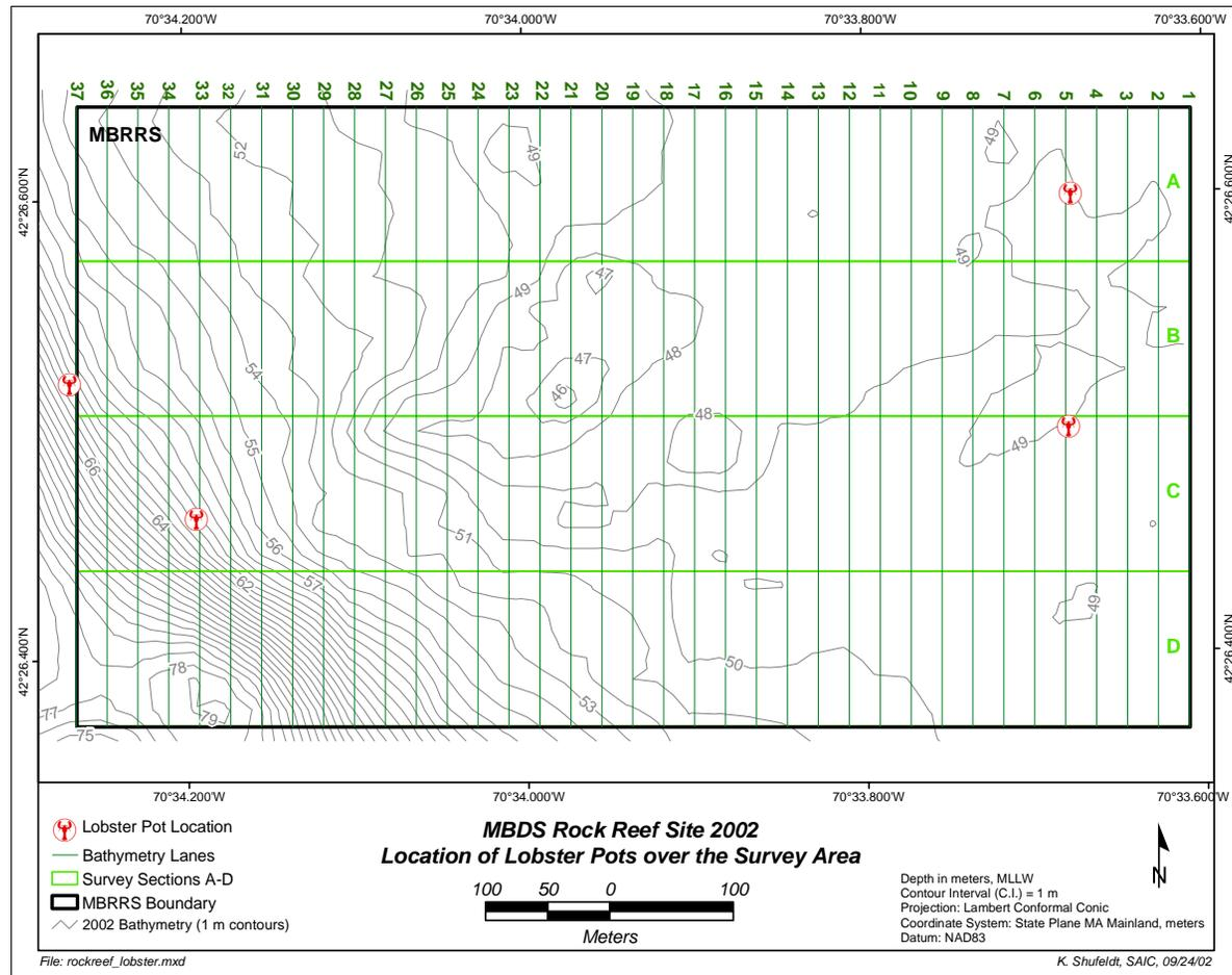
**Figure 3-5.** Plot of surface buoy locations designating lobster trap trawls deployed within the area relative to the bathymetric survey lanes and large-scale bottom features within MBRRS
