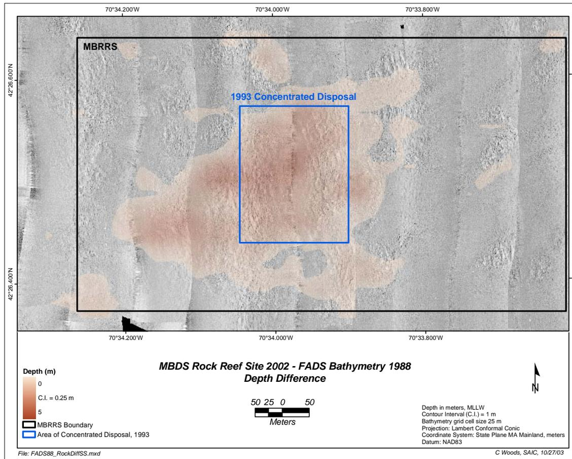
**Figure 3-9.** Composite graphic displaying the side-scan sonar mosaic overlain by bathymetric depth difference results showing the relationship between the morphology of the rock deposits and seafloor composition, 0.25 m color gradient
