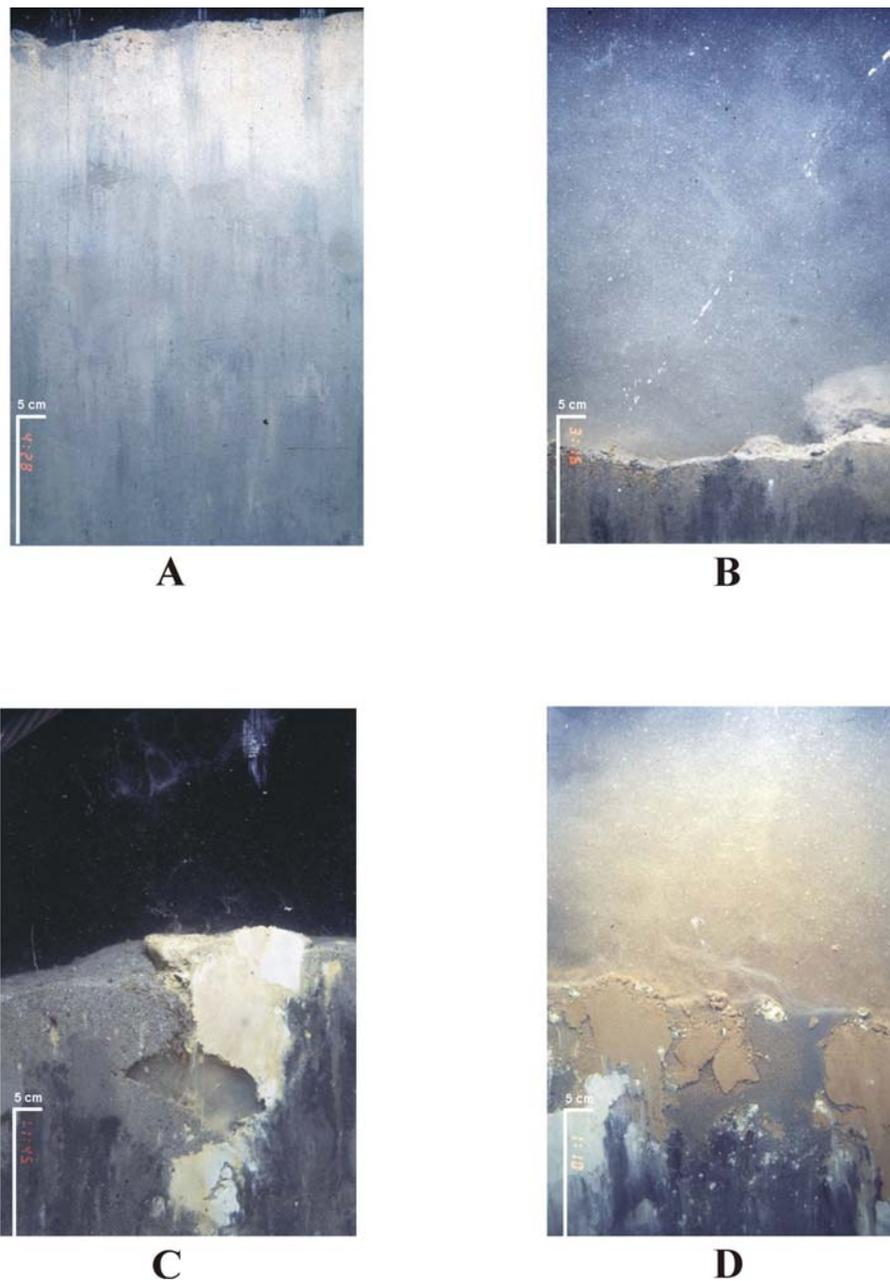
**Figure 4-9.** REMOTS® images collected at Station 100N documenting the development of a capped mound on the seafloor of MBDS. Ambient sediment present during the Baseline survey (A) was covered by UDM in the form of black reduced silt and sand from Cohasset Harbor (B-Single-Barge survey), as well as yellow clay/sand and black silt detected in the Precap Survey (C). A discrete layer of CDM consisting of mottled black and gray clay was visible at this station in the Postcap survey (D)
