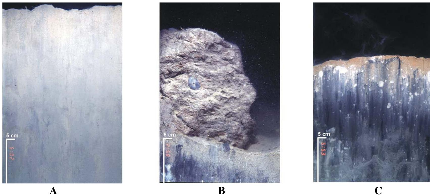
**Figure 4-8.** REMOTS® images illustrating the transition of surface sediment composition at the interior portions of the CHCP Mound (Station 50SW) from ambient fine-grained silt (A-Baseline), to organic UDM with yellow and blue clay influenced by Cohasset Harbor sediment (B-Precap), to CDM consisting of mottled black silt and white clay originating from Chelsea River (C-Postcap)
