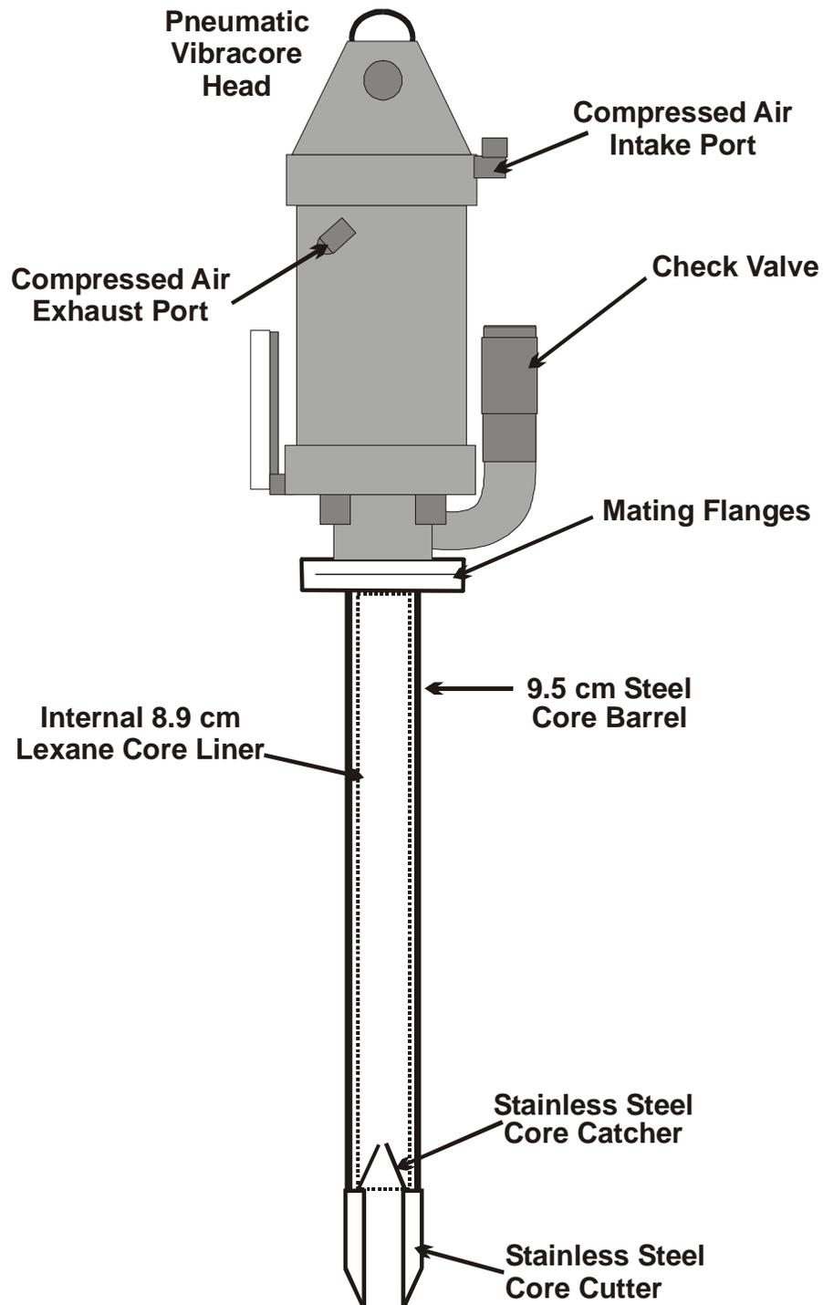
**Figure 2-3.** Diagram of the pneumatic vibracore device utilized as part of the Cohasset Harbor sediment characterization effort
