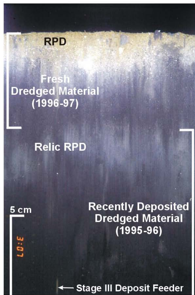
Figure 3-6. REMOTS® images collected from Stations 35 (A) and 6 (B) displaying layers of fresh dredged material over recent (1995-96) dredged material and fresh dredged material over historic dredged material, respectively
