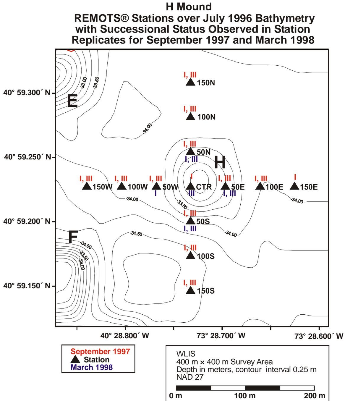
**Figure 3-6.** Distribution of successional stage assemblages over the H mound overlaid on July 1996 bathymetry
