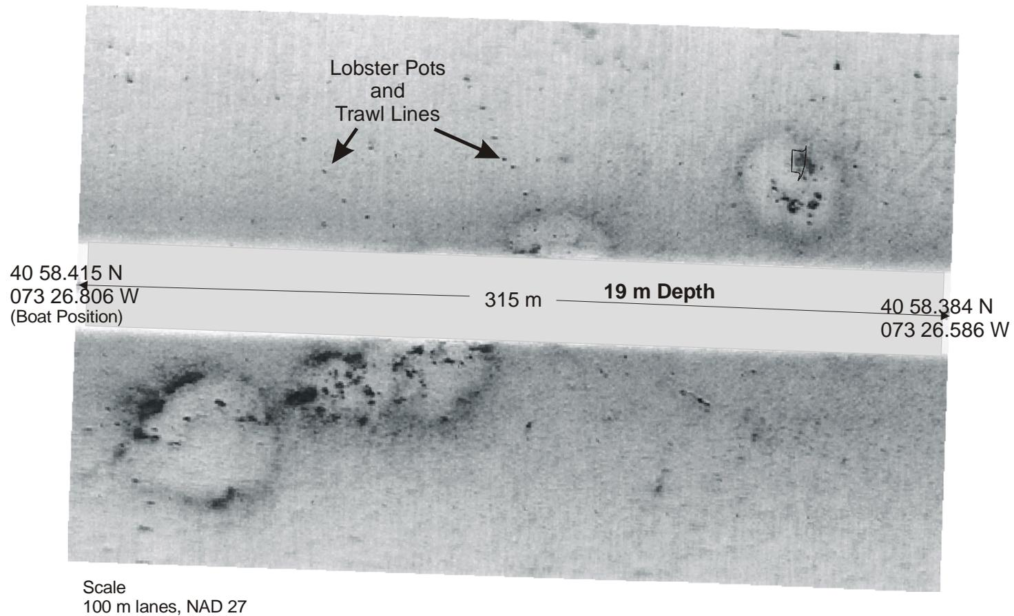
**Figure 3-10.** Detection of historic dredged material deposits in side-scan lane 13, east of SE-REF in side-scan sonar range
