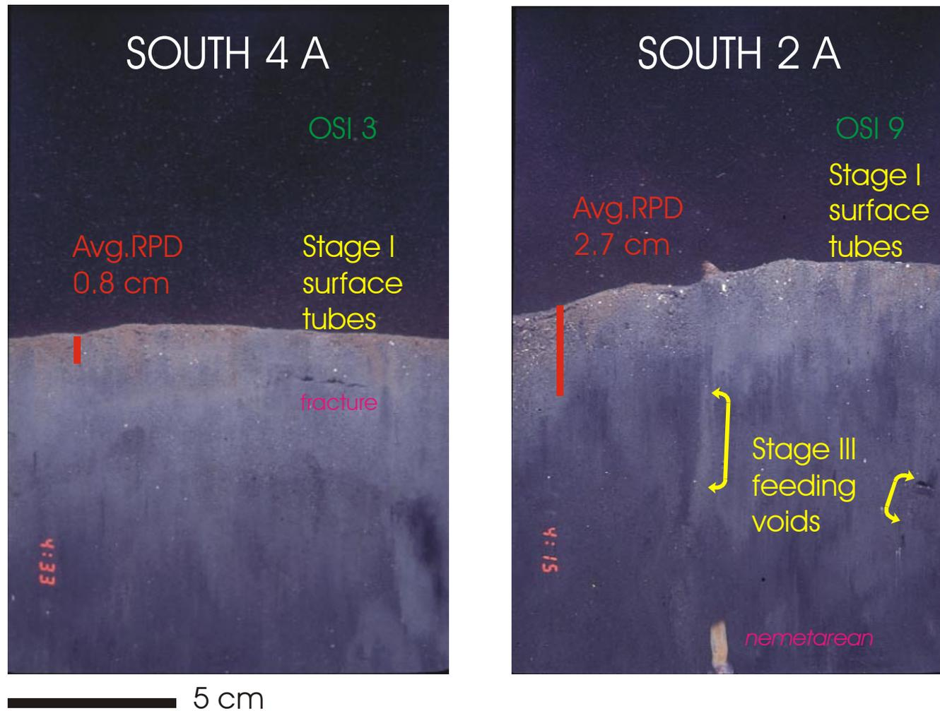
**Figure 4-3.** REMOTS® replicates from the September 1997 survey at SOUTH showing variability in benthic conditions in the reference area
