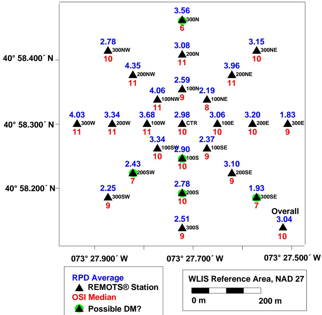
**Figure 3-13.** Distribution of RPD depths and OSI values for March 1998 REMOTS® stations at SE-REF. Stations that have one or more replicates that may indicate dredged material are circled in green.
