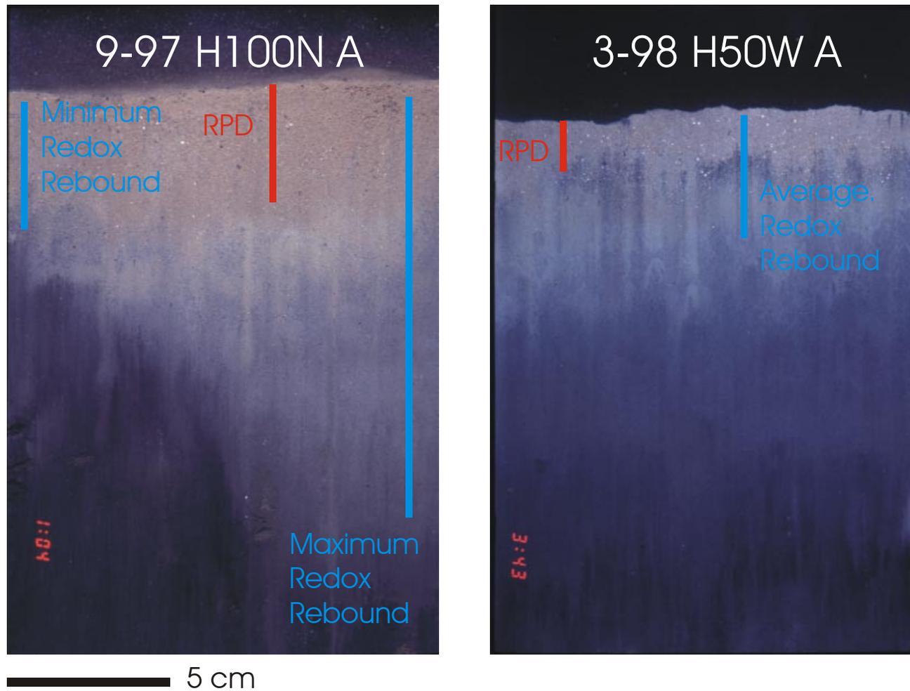
**Figure 4-5.** REMOTS® replicates over the H mound with redox rebounds. H100NA from September shows a highly variable redox rebound and deep RPD. H50WA shows a shallower RPD and more consistent redox rebound.
