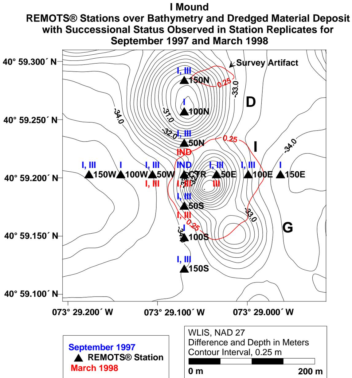
**Figure 3-3.** Distribution of successional stage assemblages over the I mound, overlaid on September 1997 bathymetry and detectable mound margin
