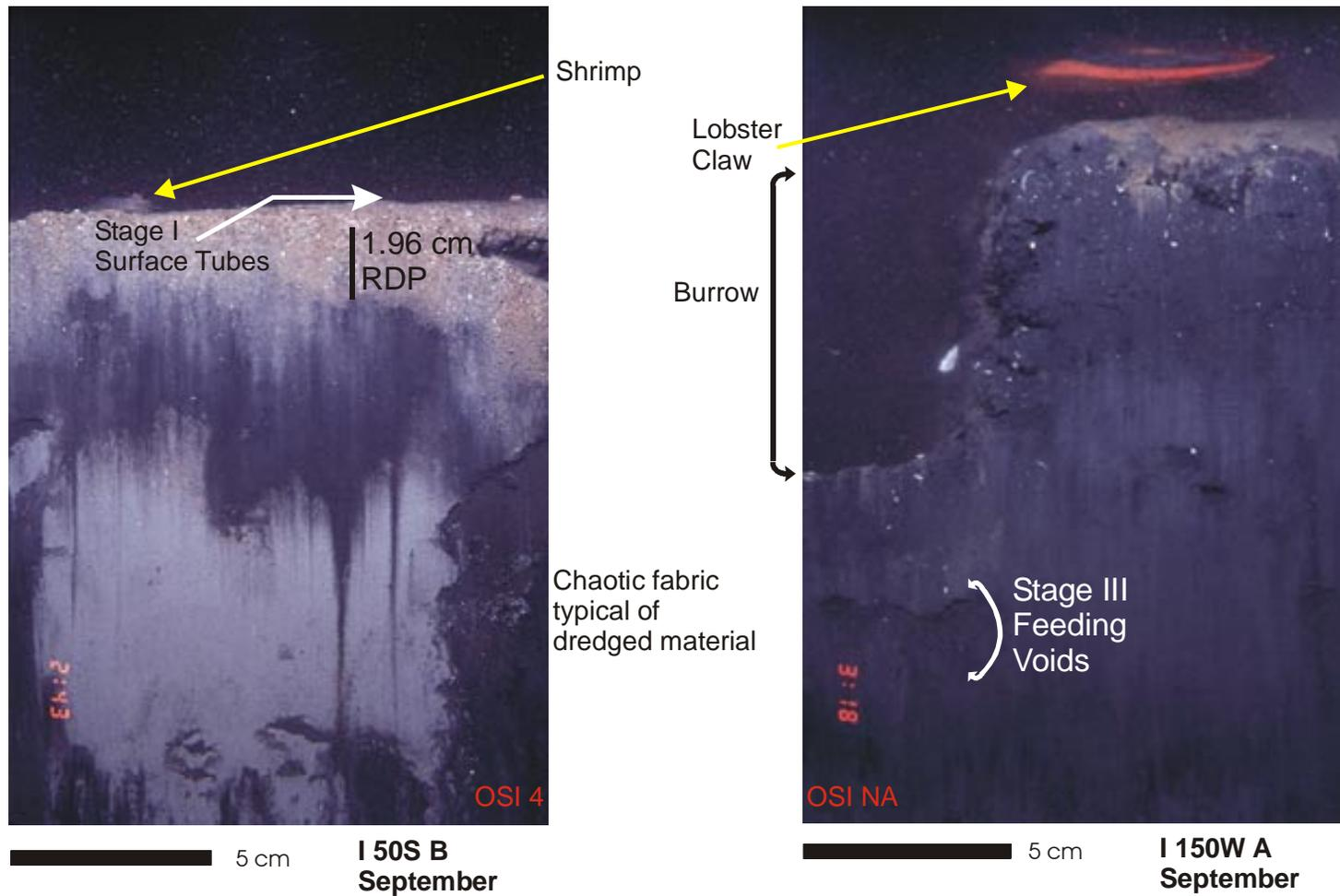
**Figure 4-7.** September 1997 REMOTS® photographs at the I mound showing healthy benthic conditions for a recently disposed dredged material mound with a shrimp and lobster living on the bottom sediments
