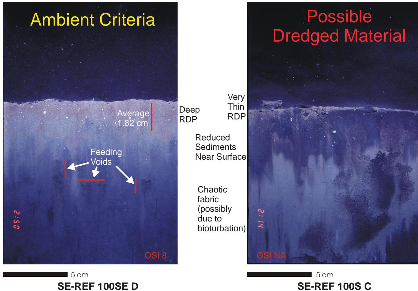
**Figure 4-8.** REMOTS® replicates from the March 1998 survey showing the criteria for ambient sediments and the detection of possible historic dredged material
