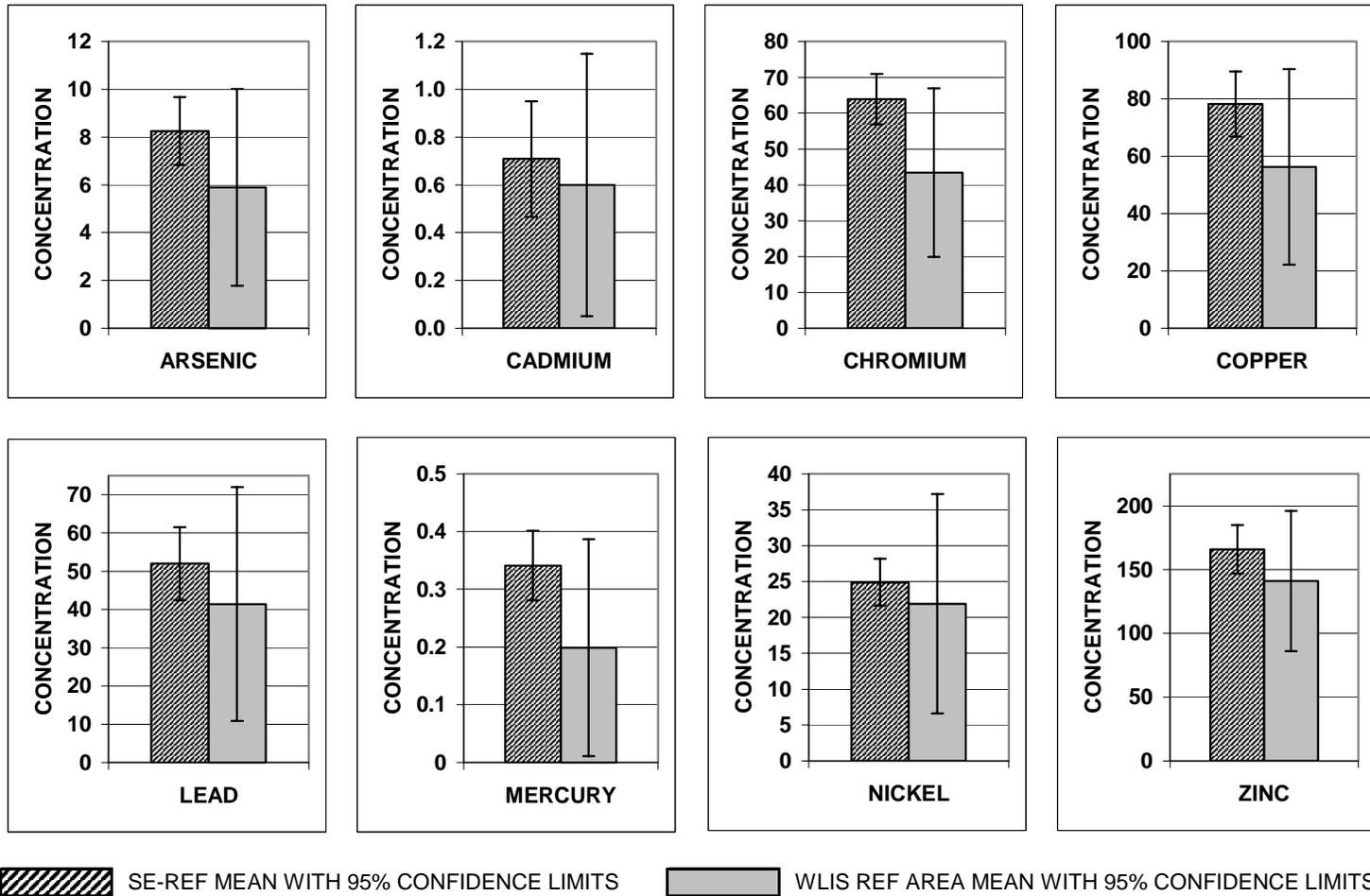
**Figure 3-15.** SE-REF and WLIS Reference Area (Murray 1995) mean metal concentrations (ppm). Comparison of the 95% confidence levels indicates no significant statistical difference between SE-REF and the WLIS reference area dataset.
