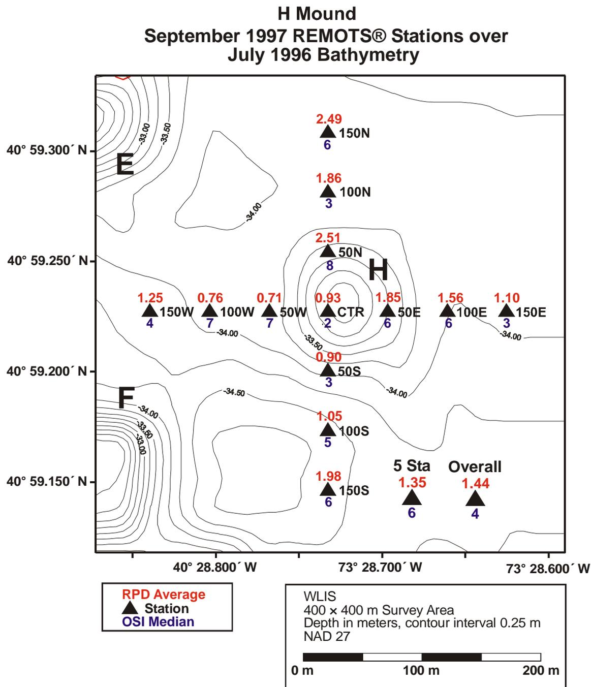
**Figure 3-7.** Distribution of Redox Potential Discontinuity (RPD) depths and Organism-Sediment Index (OSI) values for September 1997 REMOTS® stations overlaid on July 1996 bathymetry of the H mound
