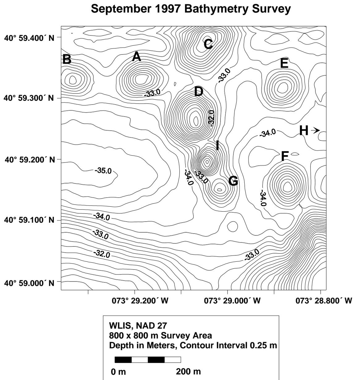
**Figure 3-1.** Bathymetric chart of the September 1997 800 x 800 m survey area
