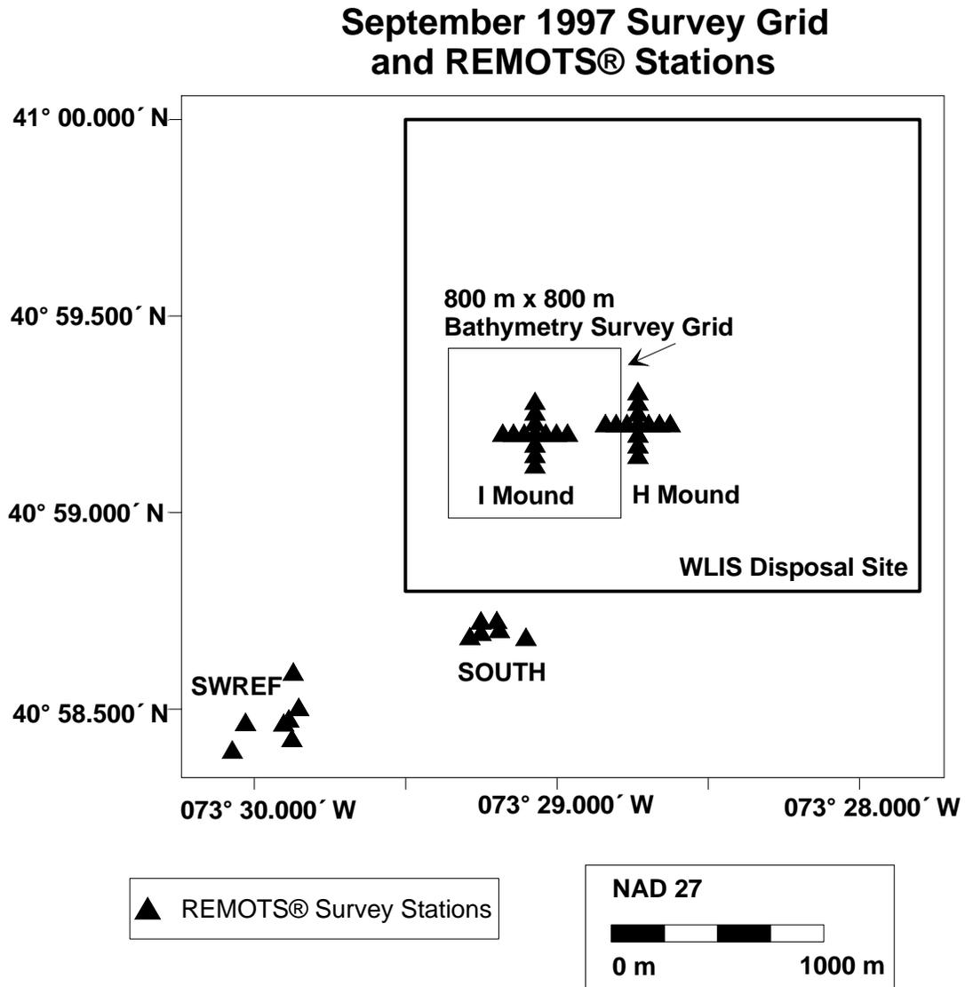
**Figure 2-4.** Chart of the September 1997 bathymetric survey area and REMOTS® stations relative to the WLIS boundaries
