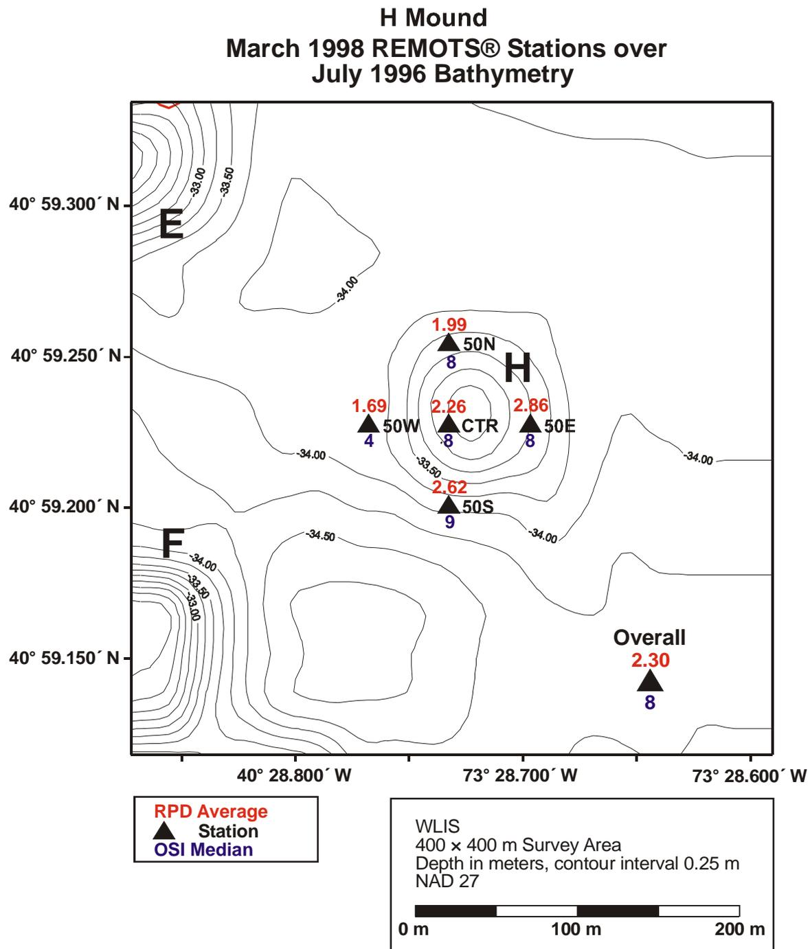
**Figure 3-8.** Average Redox Potential Discontinuity (RPD) depth (cm) and median OSI values for March 1998 REMOTS® stations overlaid on July 1996 bathymetry
