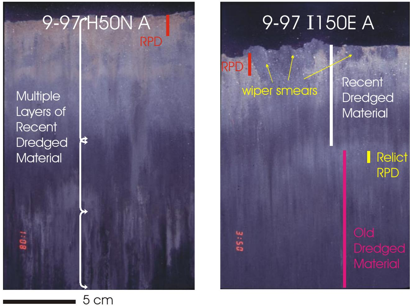
**Figure 4-6.** REMOTS® replicates H50NA showing multiple layers of recently disposed dredged material in contrast to I150EA showing recently disposed dredged material over old dredged material
