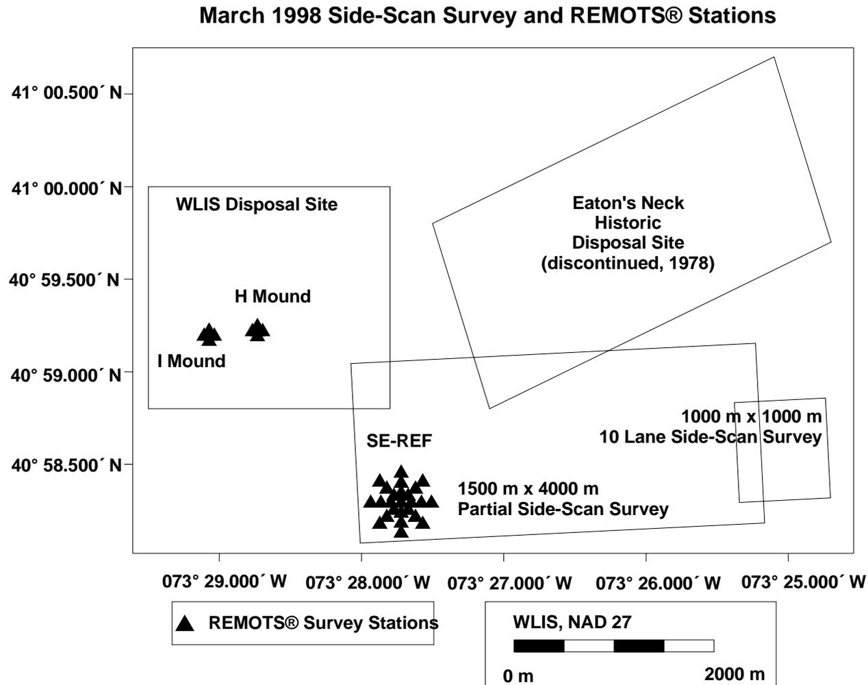
**Figure 2-5.** Chart of the March 1998 side-scan sonar survey area and REMOTS® stations relative to the WLIS boundaries
