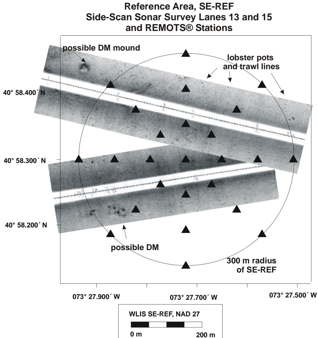
**Figure 3-9.** Side-scan sonar surveys images and REMOTS® stations for the SE-REF reference area investigation. Side-scan images were not mapped according to exact geodetic positions and have been placed as accurately as possible for representation purposes only
