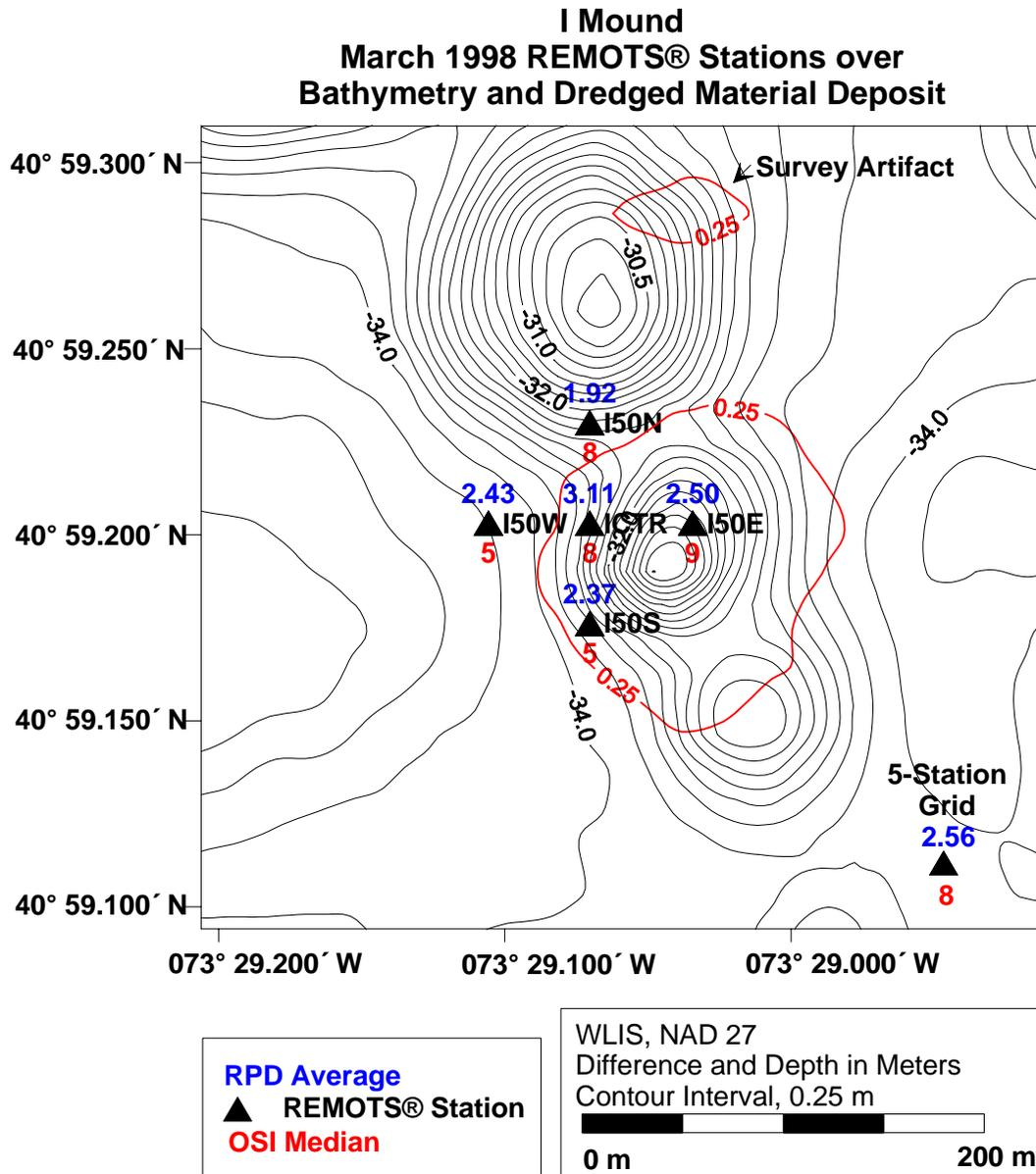
**Figure 3-5.** Distribution of RPD depths and OSI values for March 1998 REMOTS® stations overlaid on bathymetry and detectable mound margin
