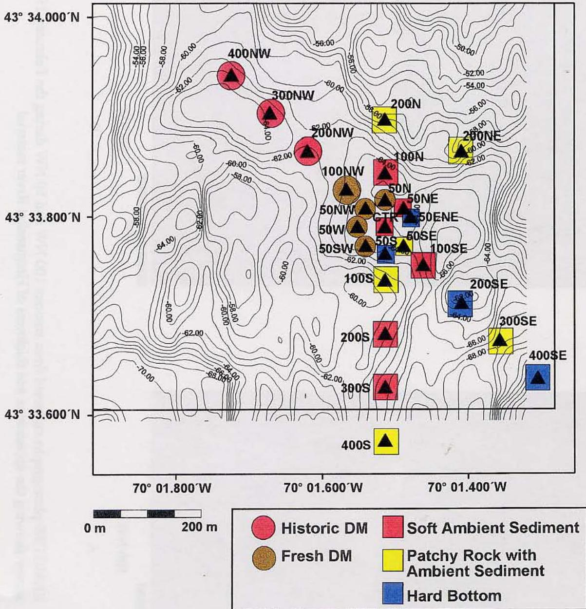
**Figure 4-7.** Characterization of ambient sediments and dredged material within the Royal River Project Area, as detected by the February 1996 REMOTS® camera survey
