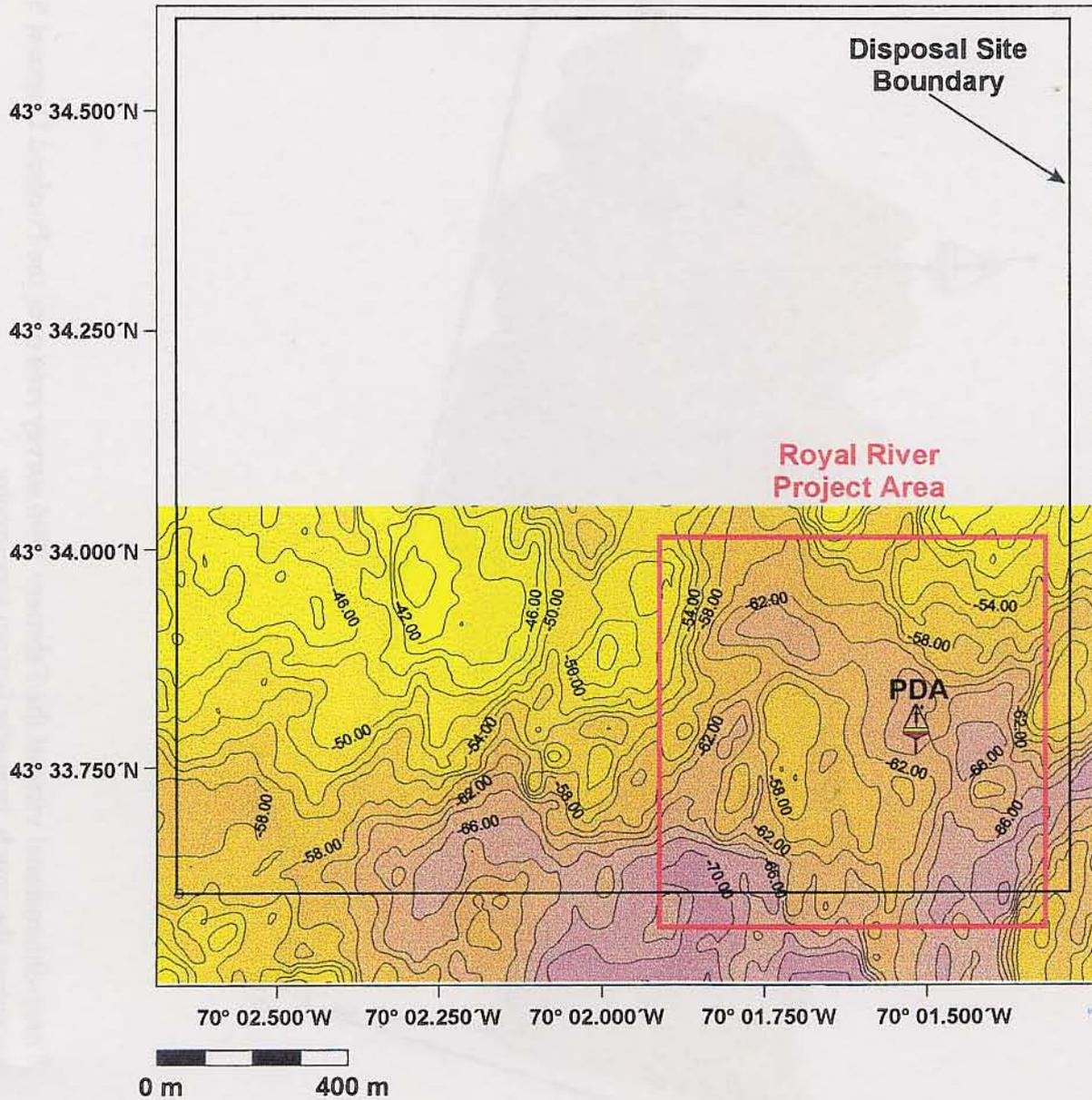
**Figure 4-5.** Bathymetric chart of the February 1996 1950 m × 1000 m survey area (NAD 27) over the southern region of Portland Disposal Site relative to the project area and disposal area boundary, 2.0 m contour interval (MLLW)
