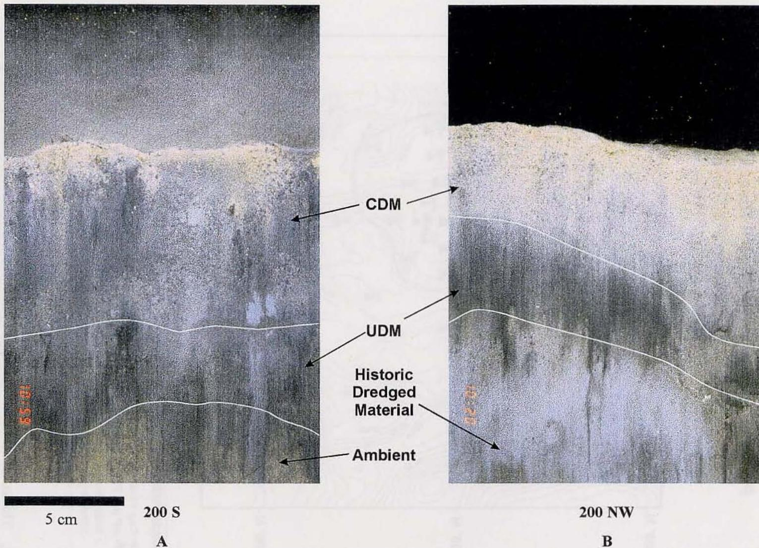
**Figure 4-23.** REMOTS® photographs collected at Stations 200 S and 200 NW as part of the January 1997 CDM survey showing multiple sediment strata within the top 20 cm
