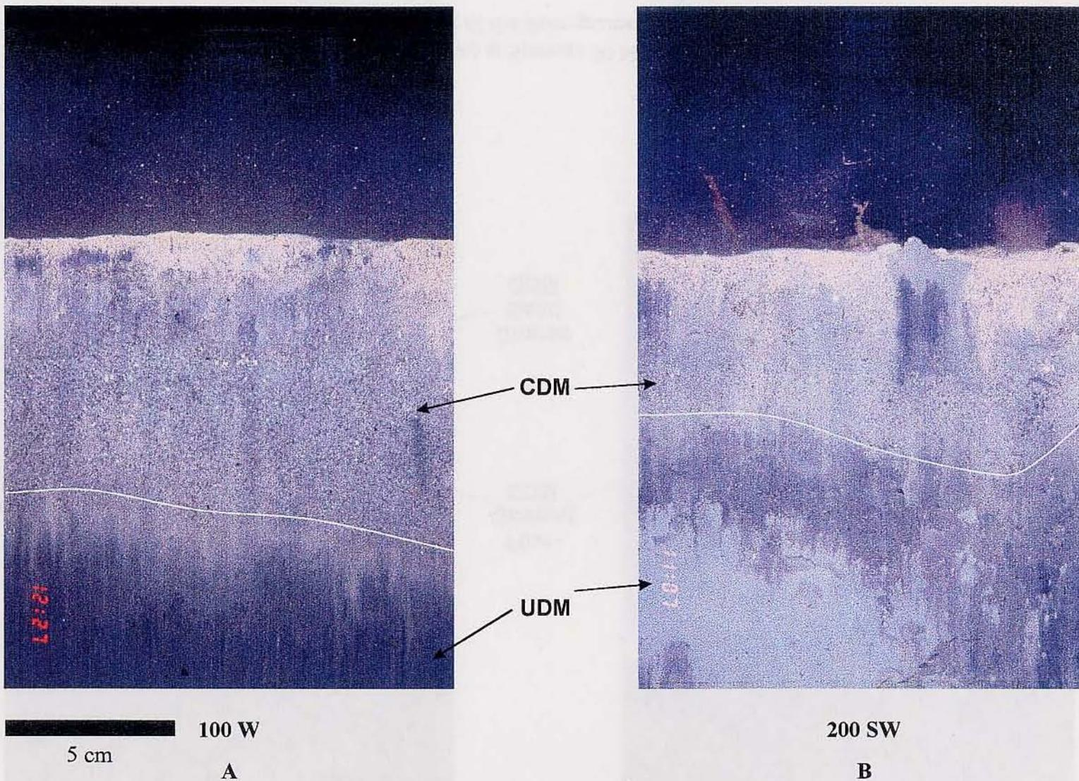
**Figure 4-24.** REMOTS® photographs collected at Stations 100 W and 200 SW as part of the January 1997 CDM survey showing the distinct coarse-grained sand over pseudo-UDM
