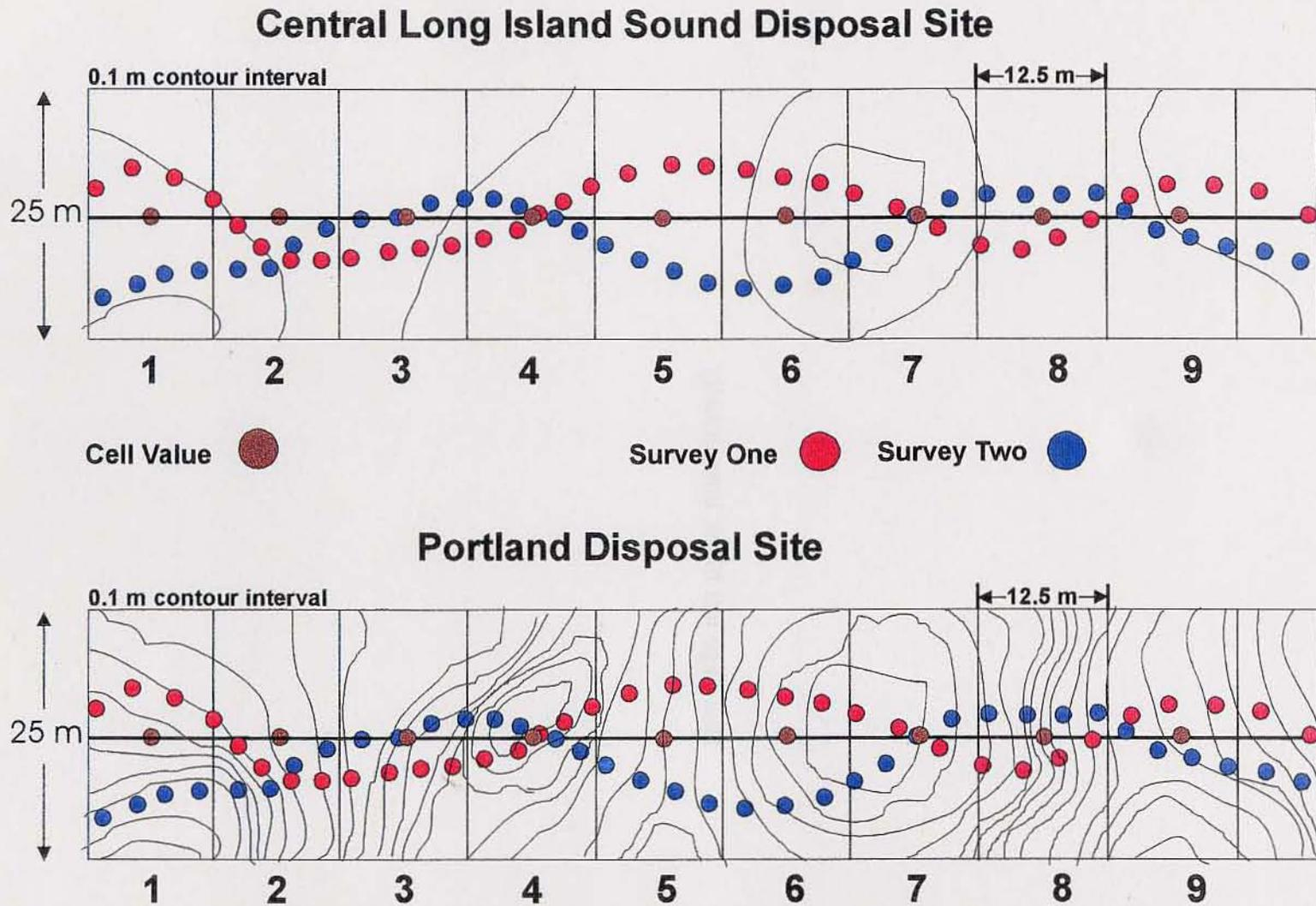
**Figure 2-10.** Comparison of a typical survey lane over the Central Long Island Sound Disposal Site versus the Portland Disposal Site and how gridding and differences in survey vessel track tend to affect the bathymetric data collection
