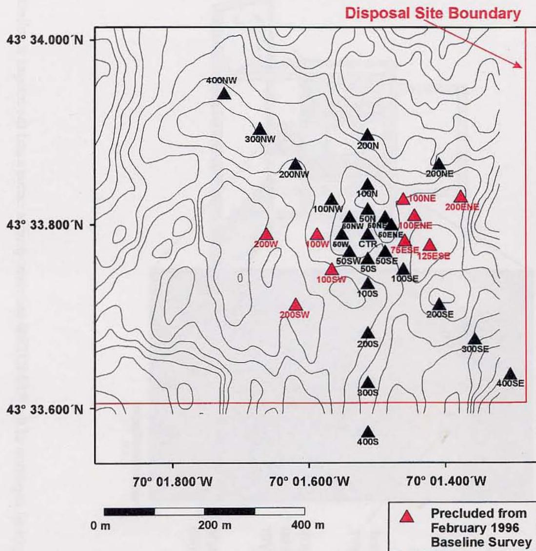
**Figure 3-4.** Bathymetric chart of the Royal River Project Area (NAD 27) showing REMOTS® sediment-profile station locations relative to the disposal site boundary
