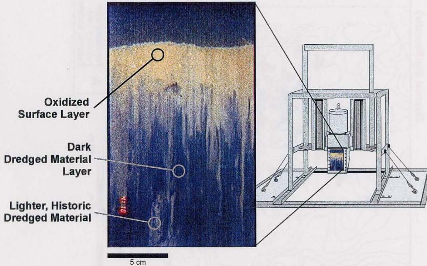
**Figure 3-3.** Graphical depiction of the REMOTS® sediment-profile camera and the images it collects
