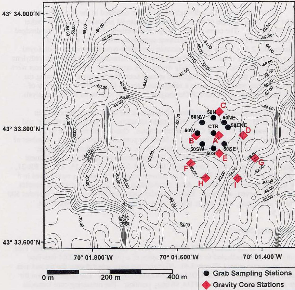
**Figure 3-6.** Bathymetric chart of the Royal River Project Area (NAD 27) showing locations of grab sampling and gravity core stations
