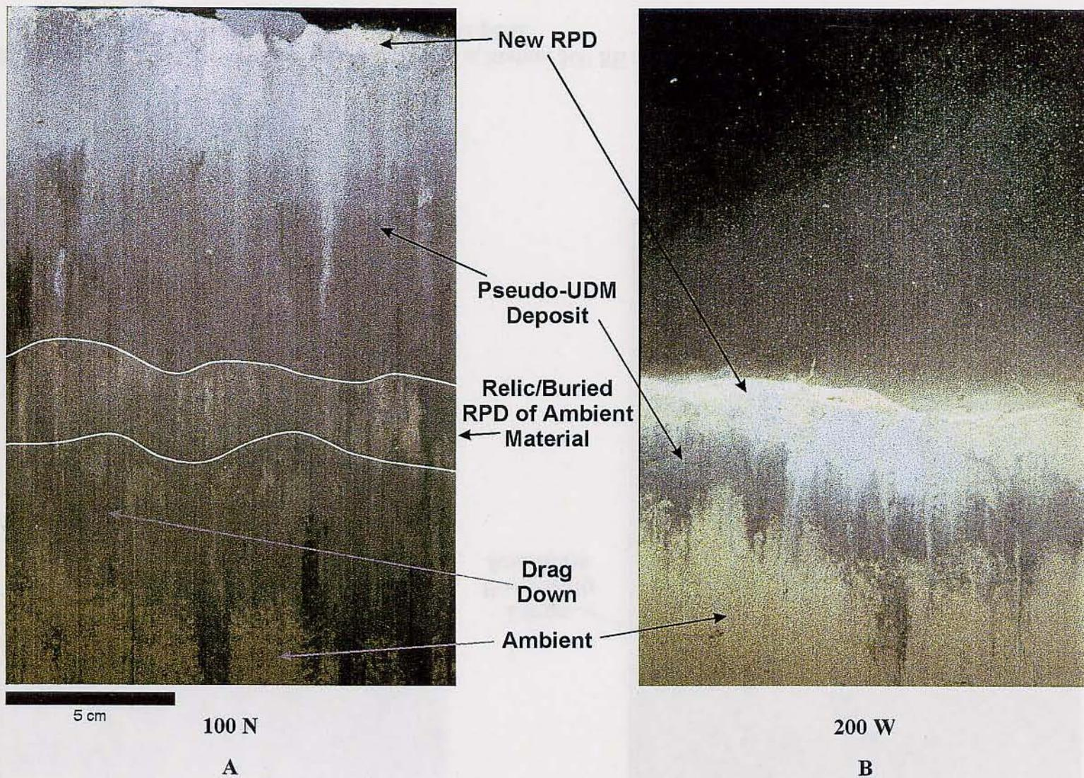
**Figure 4-16.** REMOTS® photographs collected at Stations 100 N and 200 W showing multiple sediment strata visible in the top 20 cm
