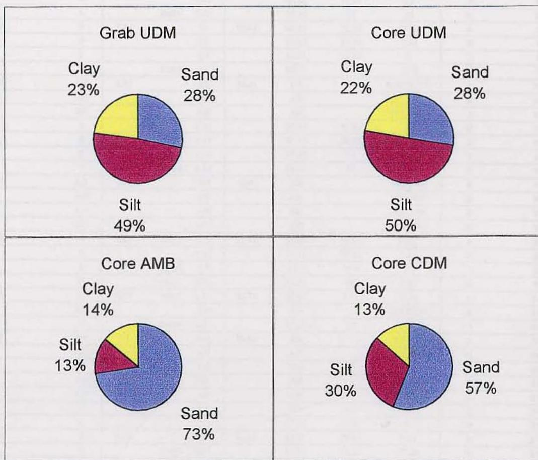
**Figure 4-18.** Mean grain size analysis results for precap (pseudo-UDM) grab samples and postcap (CDM) core samples. Core layers determined by visual observations and microfossil content
