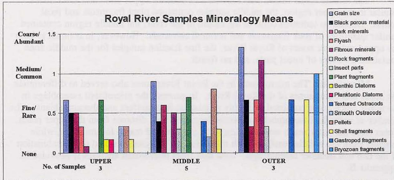
**Figure 4-1.** Histogram comparing mean abundance (rare, common, abundant) and particle size (fine, medium, coarse) for the mineralogical components utilized as sediment tracers from the Royal River cores
