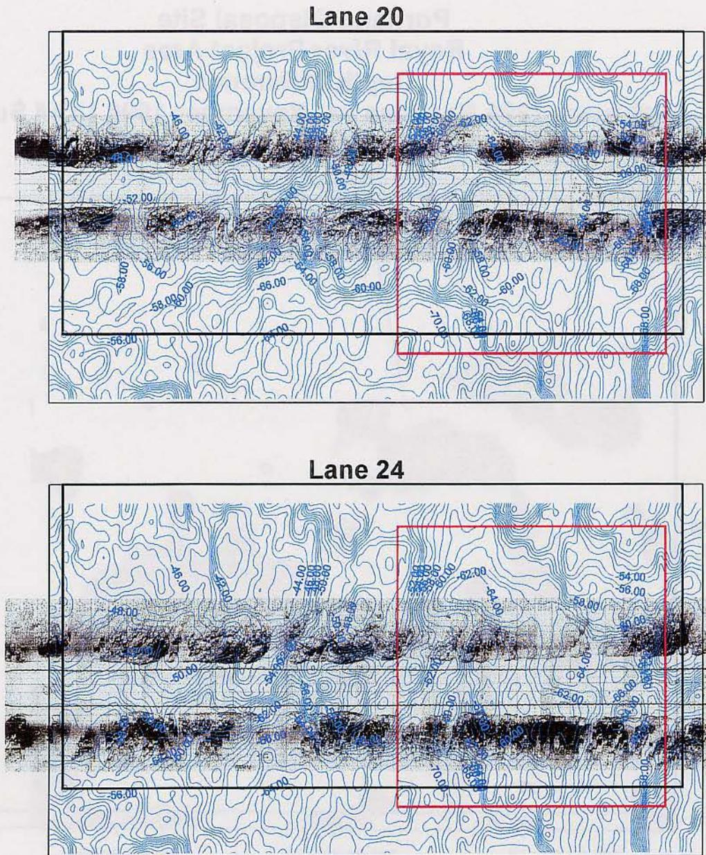
**Figure 4-11.** Side-scan sonar data from February 1996 survey lanes 20 and 24 overlaid with bathymetry showing rapid changes in depth due to bedrock outcrops
