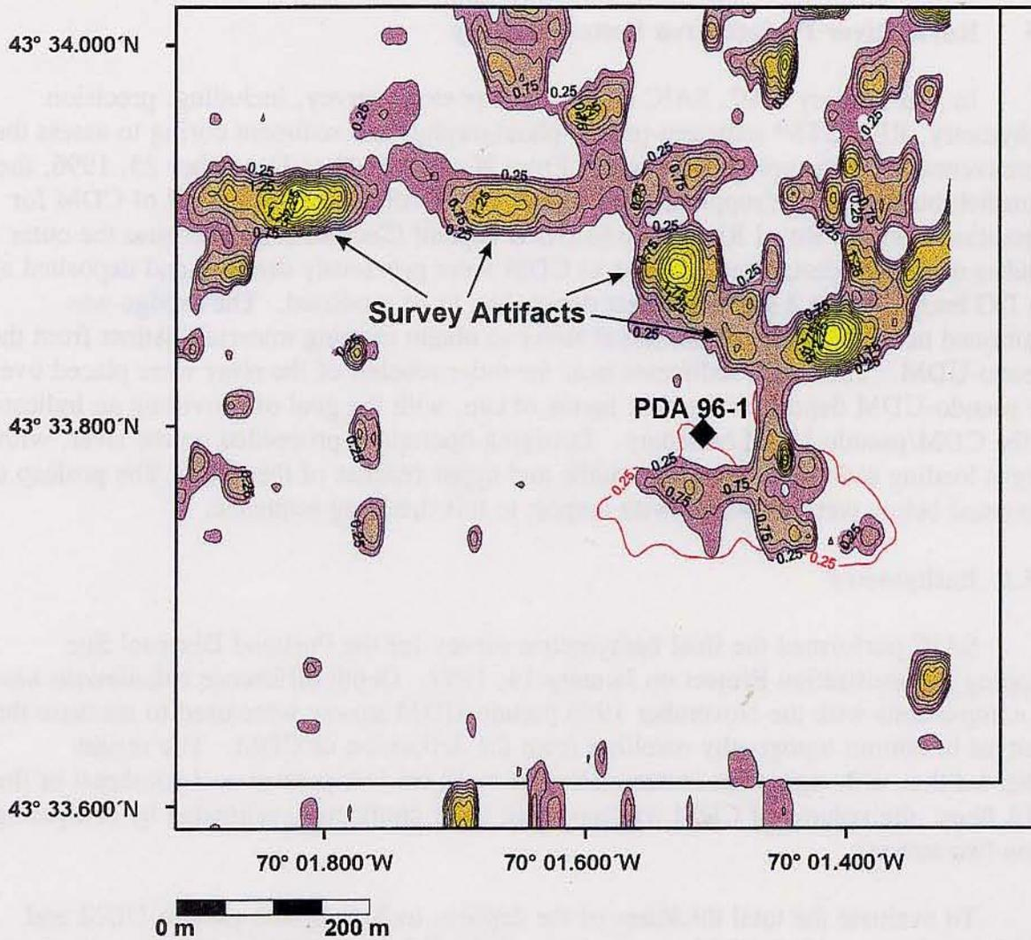
**Figure 4-21.** Depth difference comparison of the January 1997 CDM survey versus the February 1996 baseline survey relative to the pseudo-UDM footprint (red)
