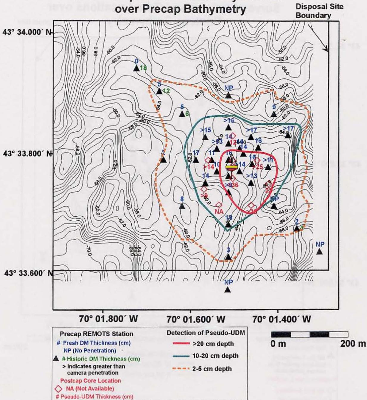
**Figure 5-1.** Thickness of pseudo-UDM measured by REMOTS® and core data overlaid on a postcap bathymetric chart (NAD 27), 1.0 m contour interval (MLLW)
