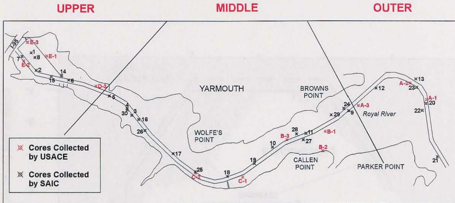
**Figure 2-4.** Royal River, ME showing navigation channel and anchorage areas dredged for the Capping Demonstration Study. A-E core series were collected by the USACE; cores 1-30 were collected as part of the pre-dredging sediment characterization study performed by SAIC.
