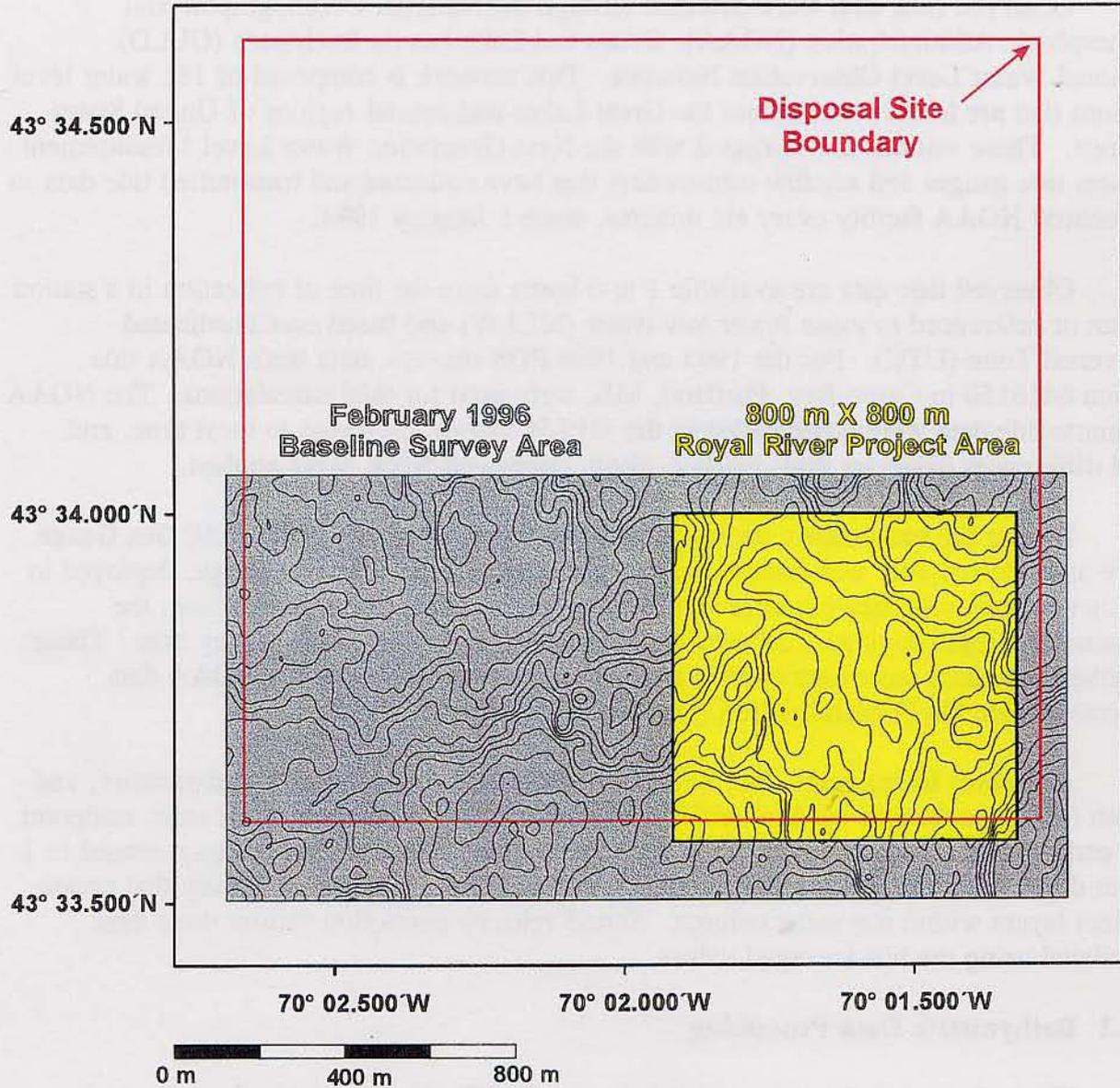
**Figure 3-1.** Base map showing the 1950 m × 1000 m bathymetric survey area during the February 1996 baseline survey (NAD 27) in relation to the Royal River Project Area (yellow) at PDS, 2.0 m contour interval (MLLW)
