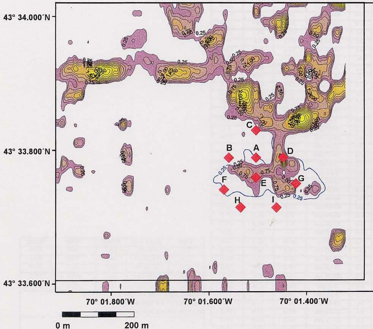
**Figure 4-27.** Depth difference plot showing detectable capped mound deposit (NAD 27) complete with gravity coring station locations
