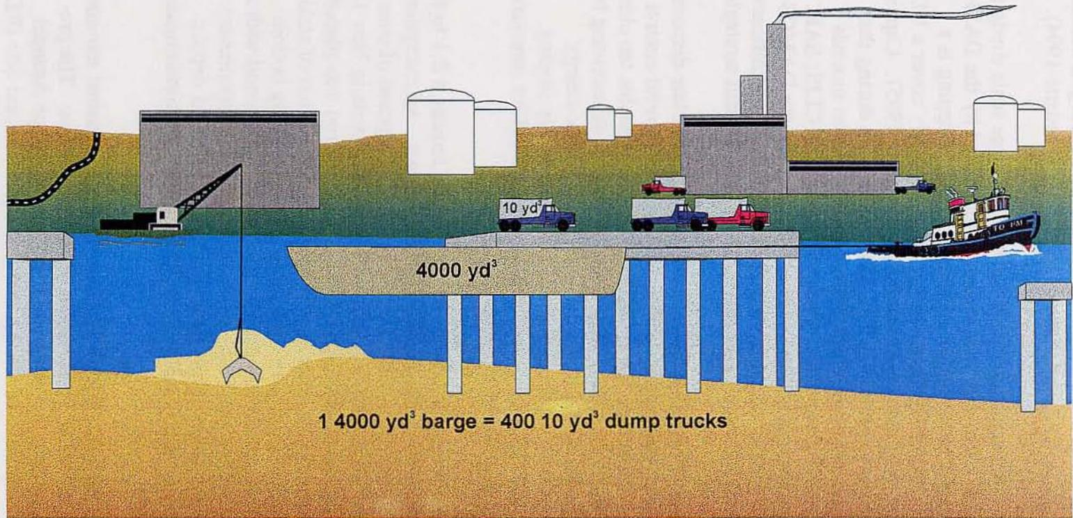
Figure 1-1. Graphical representation of maintenance dredging operations within an industrialized harbor in New England
