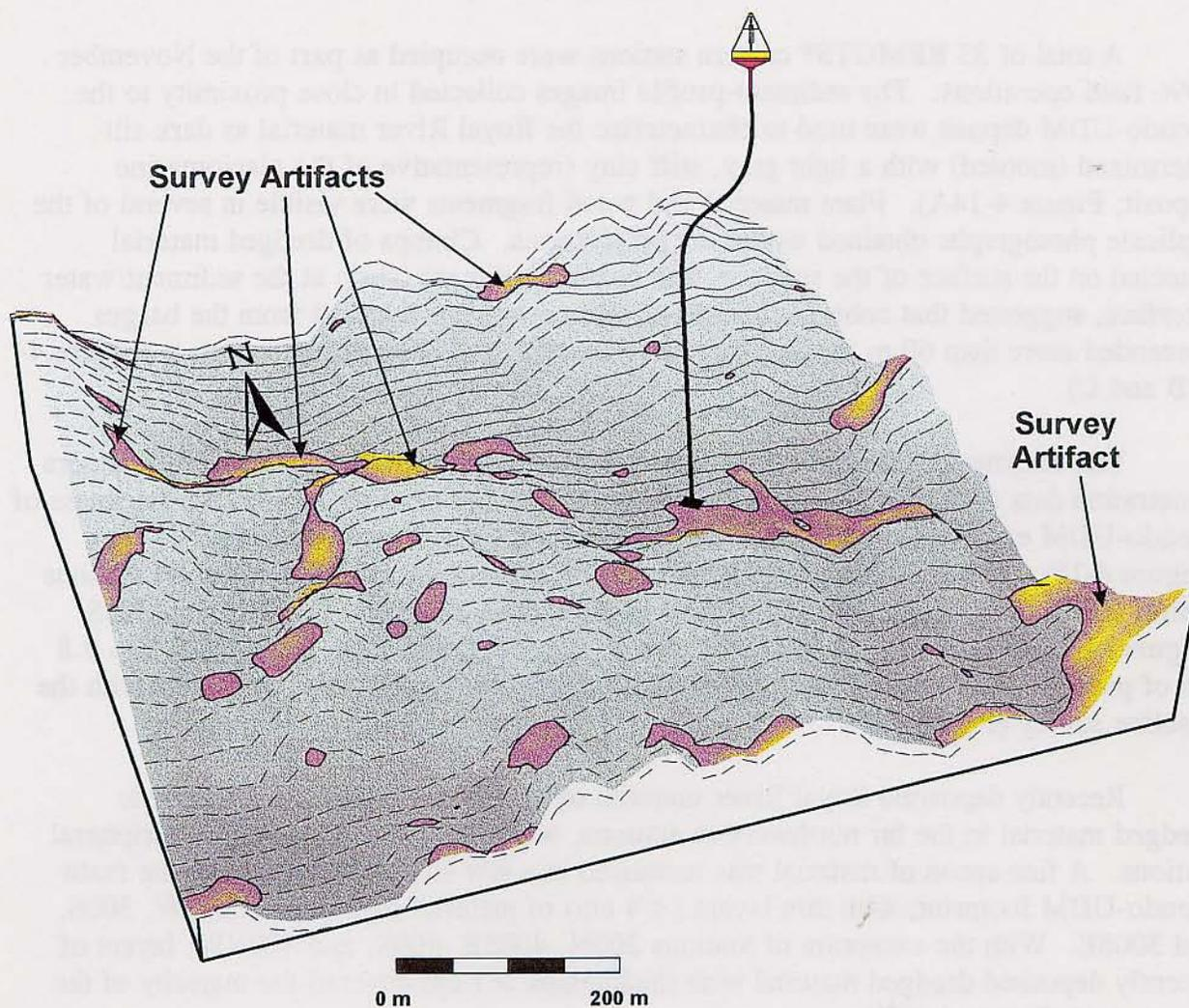
**Figure 4-13.** Three-dimensional view of the 800 m × 800 m survey area over Portland Disposal Site, showing patterns of accumulation and survey artifacts with respect to bathymetric features
