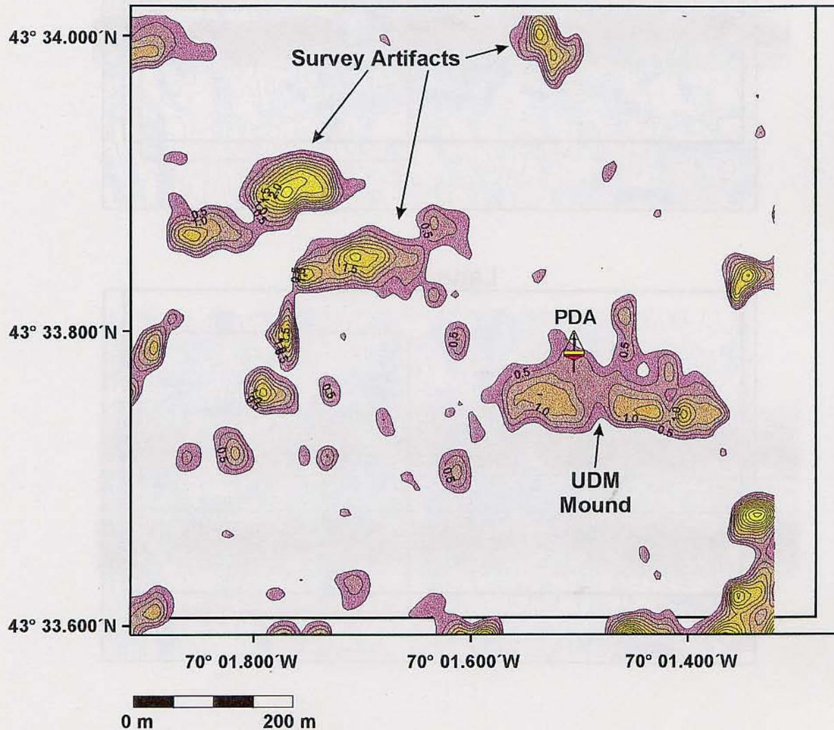
**Figure 4-12.** Depth difference plot of the November 1996 UDM survey versus the February 1996 baseline survey (NAD 27) showing apparent accumulation of pseudo-UDM in close proximity to the PDA buoy, 0.25 m contour interval
