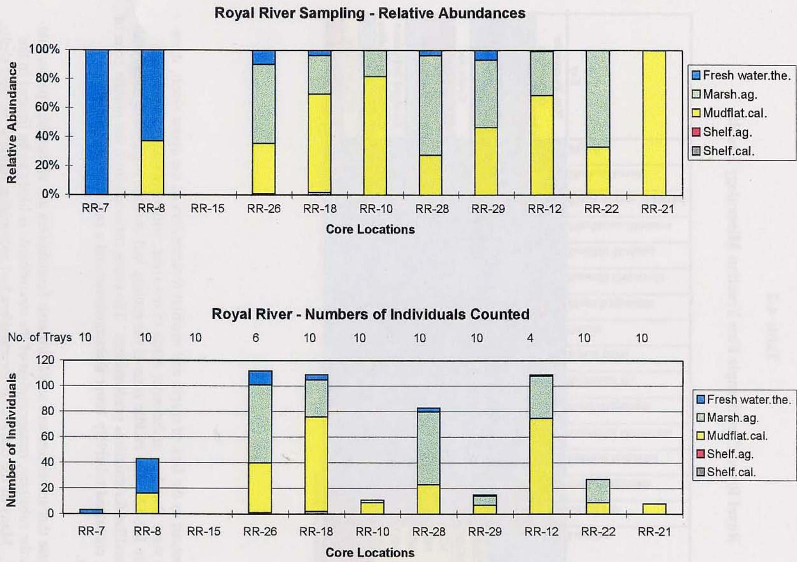
**Figure 4-2.** Histograms comparing relative abundance and density of microfossils used as sediment tracer elements from the Royal River survey
