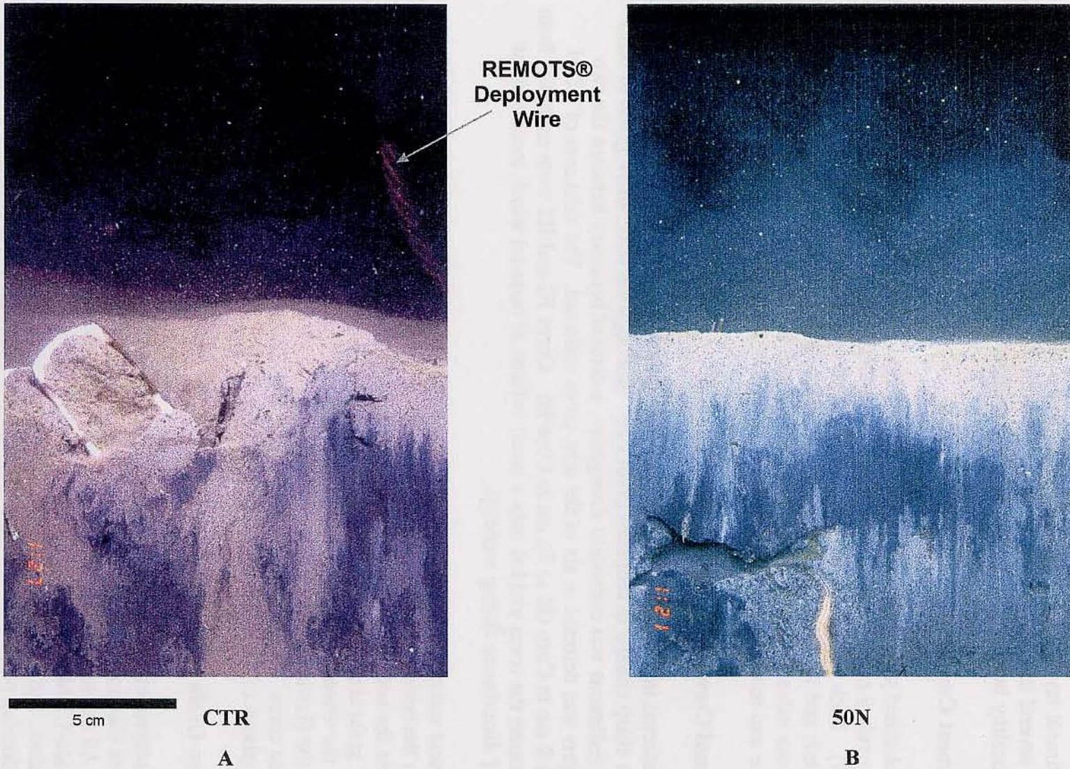
**Figure 4-26.** REMOTS® photographs collected at Stations CTR and 50 N as part of the January 1997 CDM survey showing evidence of the estuarine origin and biologic activity in the dredged material
