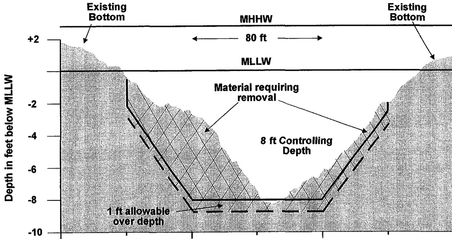
Figure 2-5. Example of a channel cross-section used to graphically display the riverbed and estimate volumes of material to be removed from the channel
