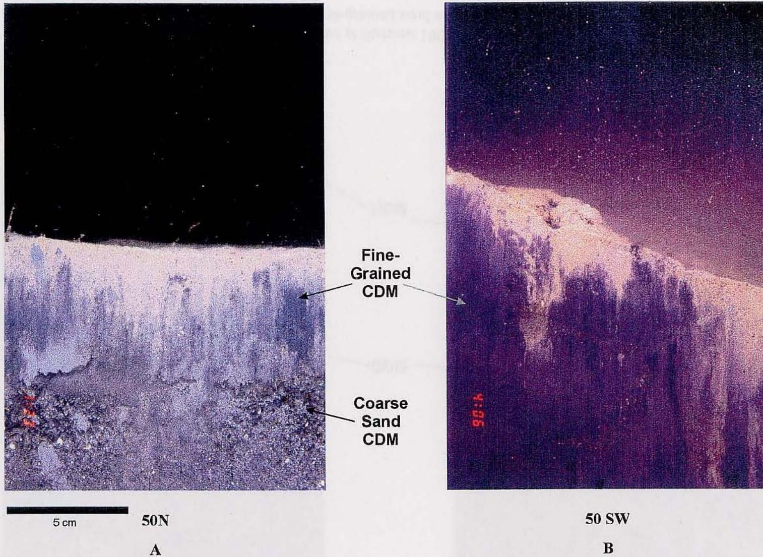
**Figure 4-25.** REMOTS® photographs collected at Stations 50 N and 50 SW as part of the January 1997 CDM survey showing the composition of the finer-grained CDM detected at several stations
