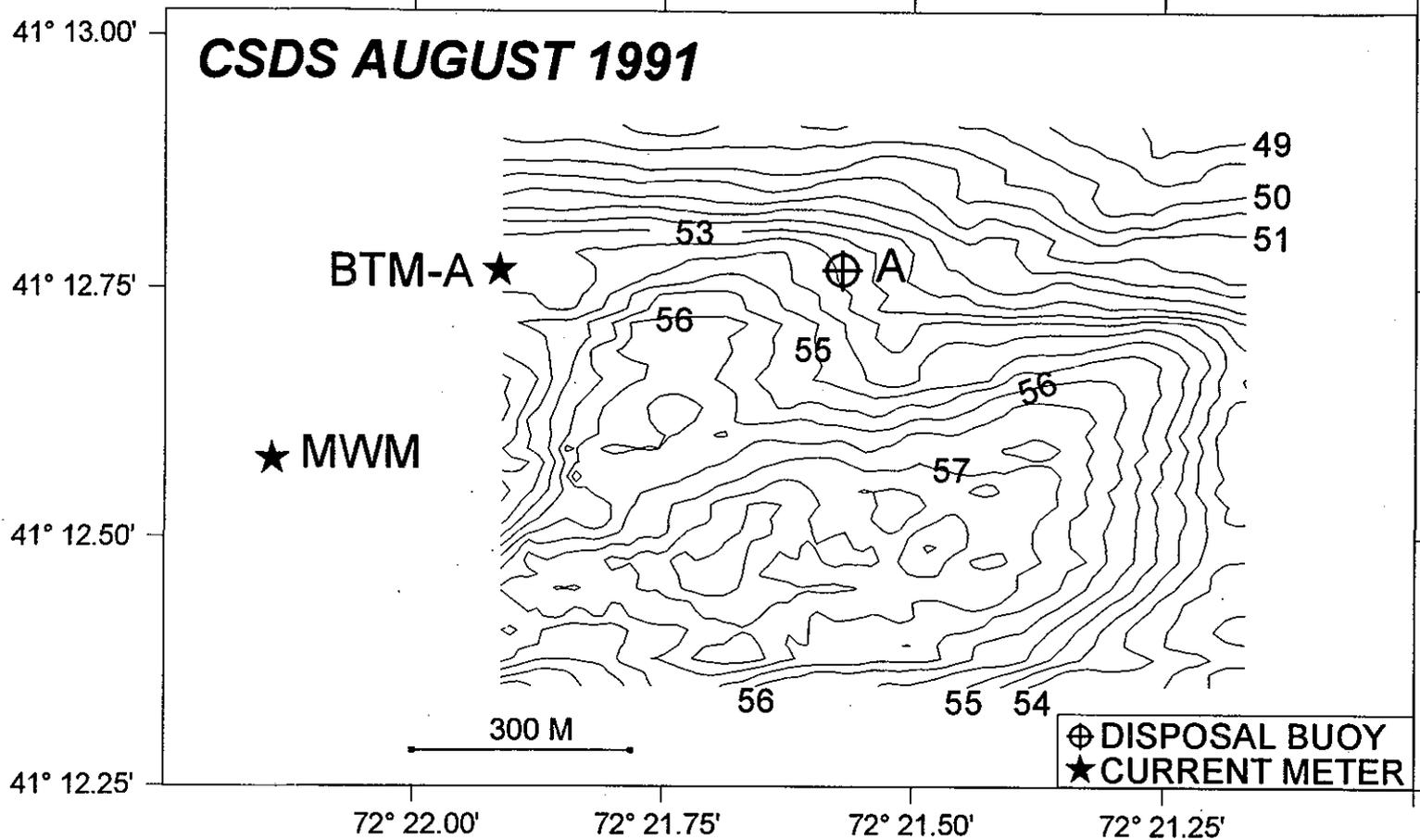
Figure 3-1. Predisposal bathymetric contour plot at CSDS, August 8, 1991 (depth in meters)
