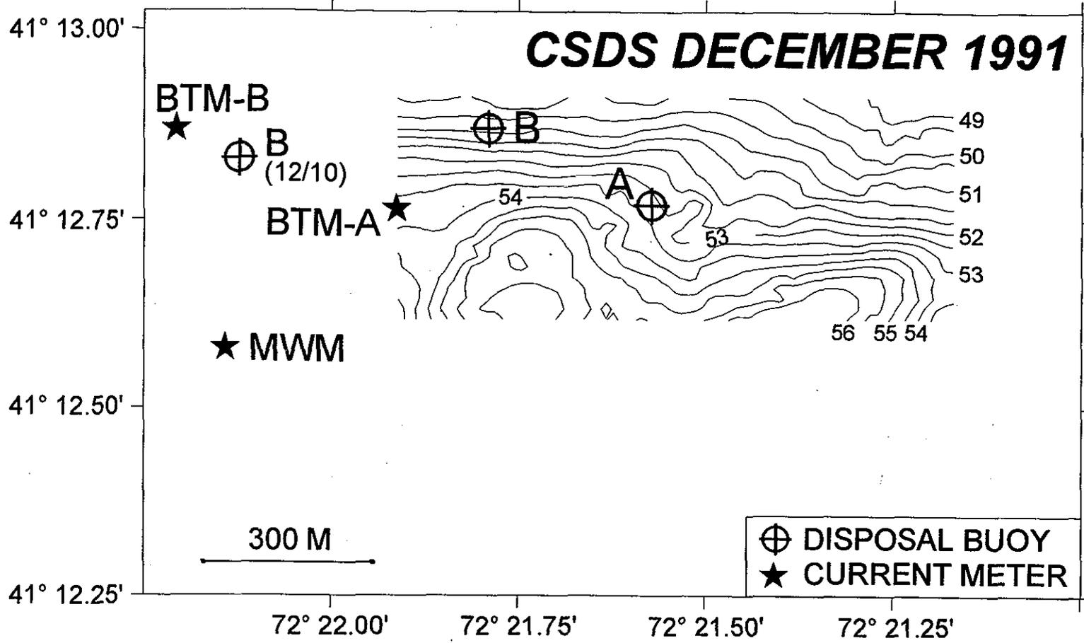
Figure 3-5. Bathymetric contour plot at CSDS during dredging and disposal of North Cove sediment, December 10, 1991 (depth in meters)
