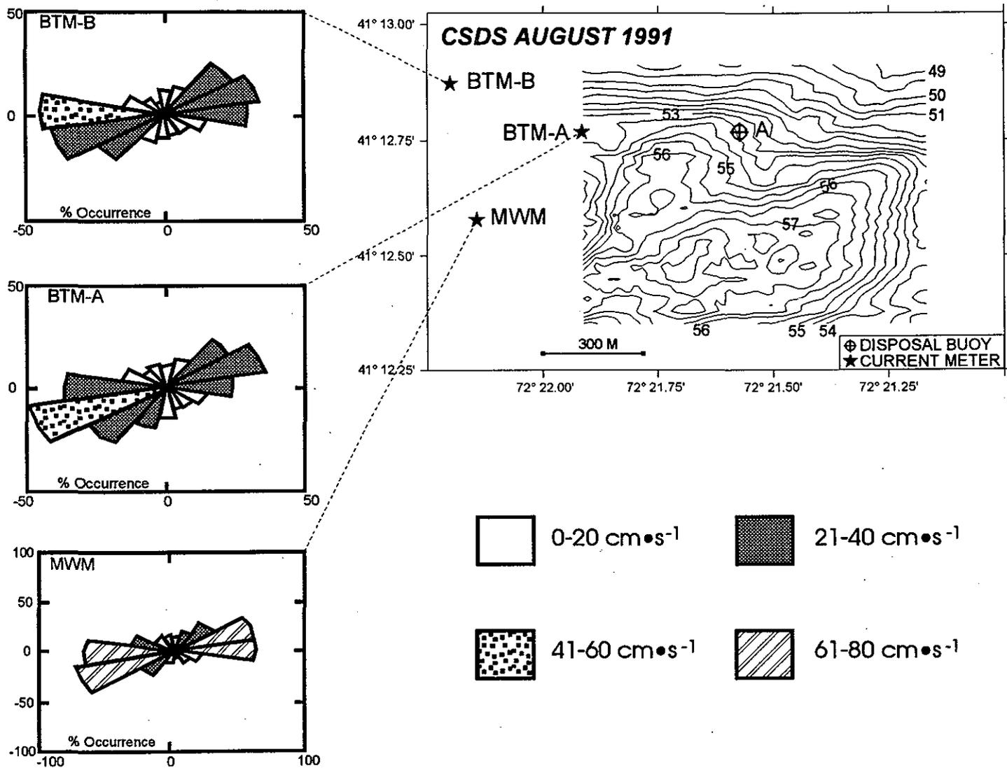
**Figure 3-10.** Current meter data with mooring locations for bottom mooring A (BTM-A), bottom mooring B (BTM-B), and the mid-water mooring (MWM)
