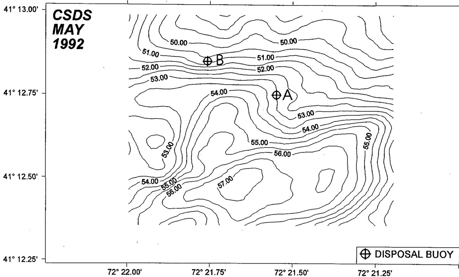
Figure 3-7. Bathymetric contour plot at CSDS after completion of North Cove dredging/disposal, May 12, 1992 (depth in meters)
