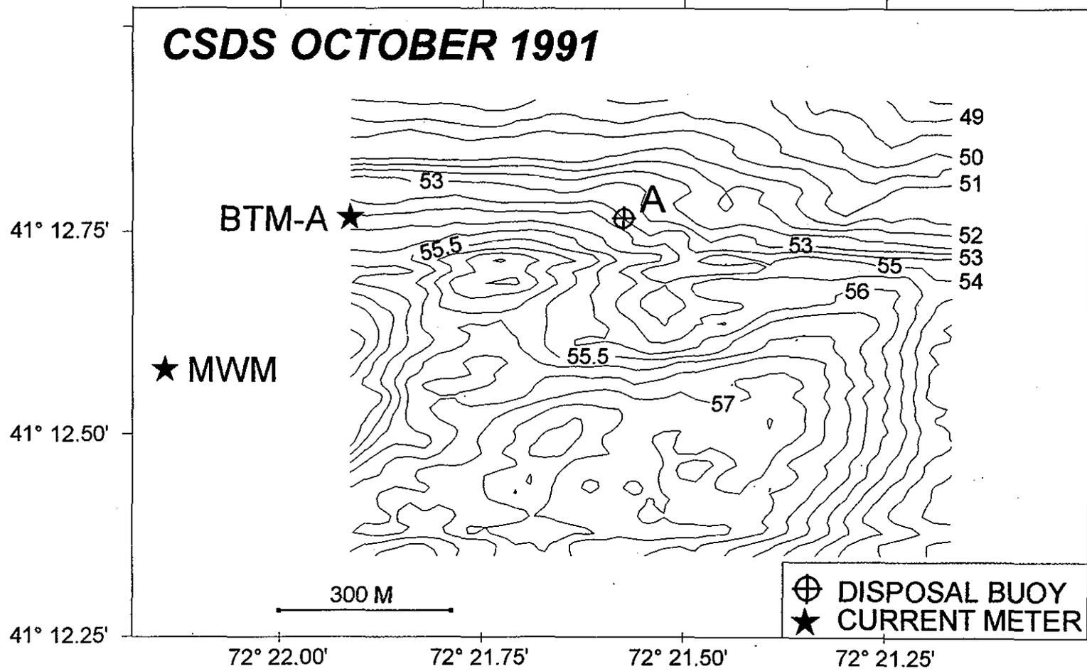
Figure 3-2. Bathymetric contour plot at CSDS after completion of Connecticut River dredging and disposal, October 18 and 19, 1991 (depth in meters)
