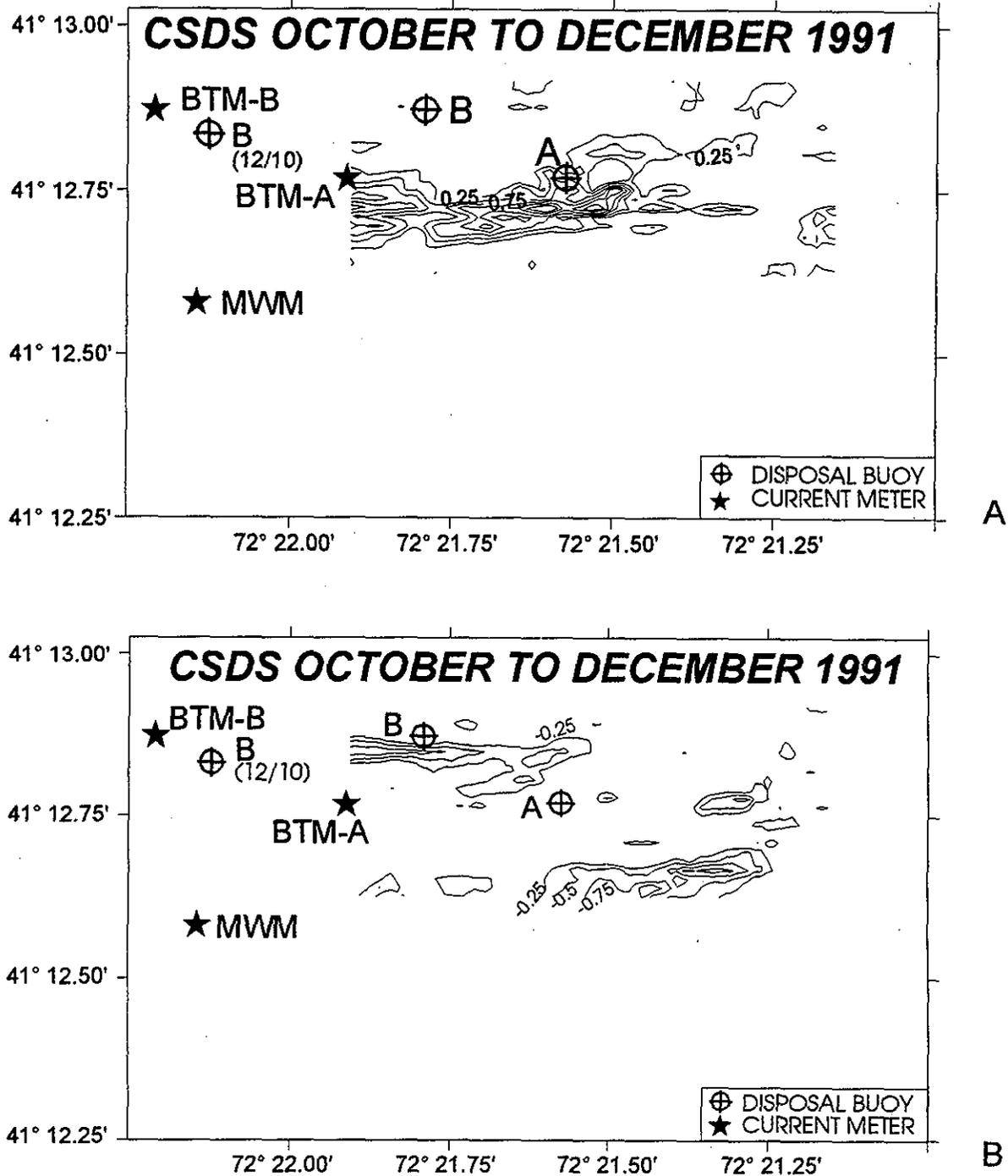
**Figure 3-6.** Accumulation (A) and erosion (B) at CSDS, October 18 and 19, 1991 to December 10, 1991 (depth in meters)
