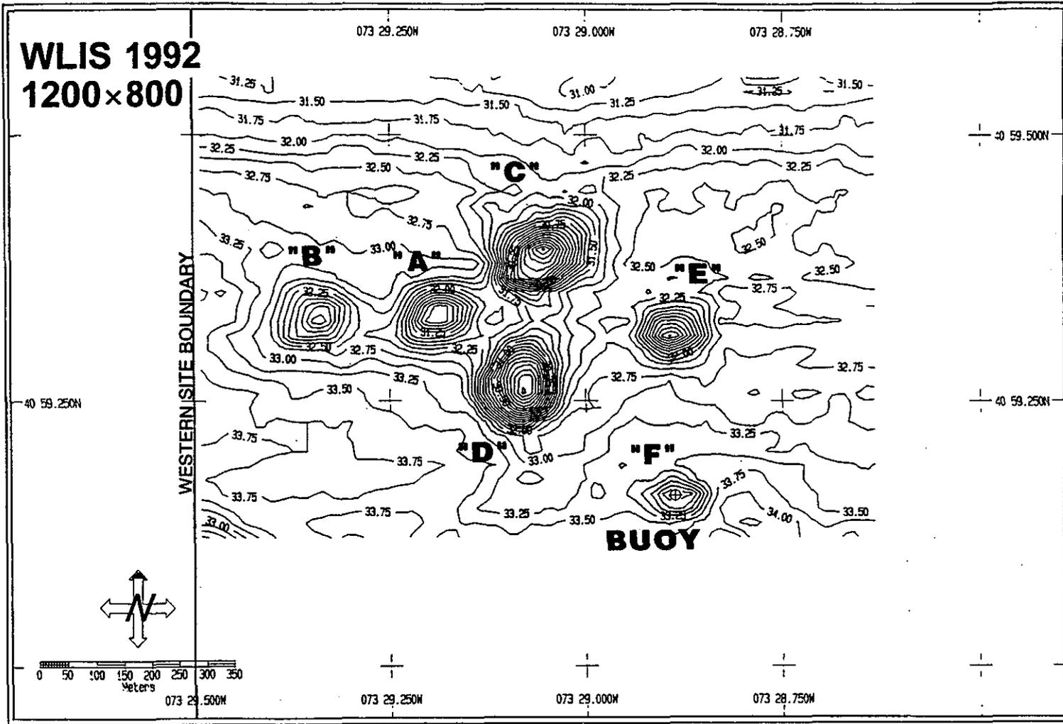
Figure 3-5. Bathymetric contour plot from the 1992 WLIS survey (corrected to prior survey, 1200 × 800 m survey area)
