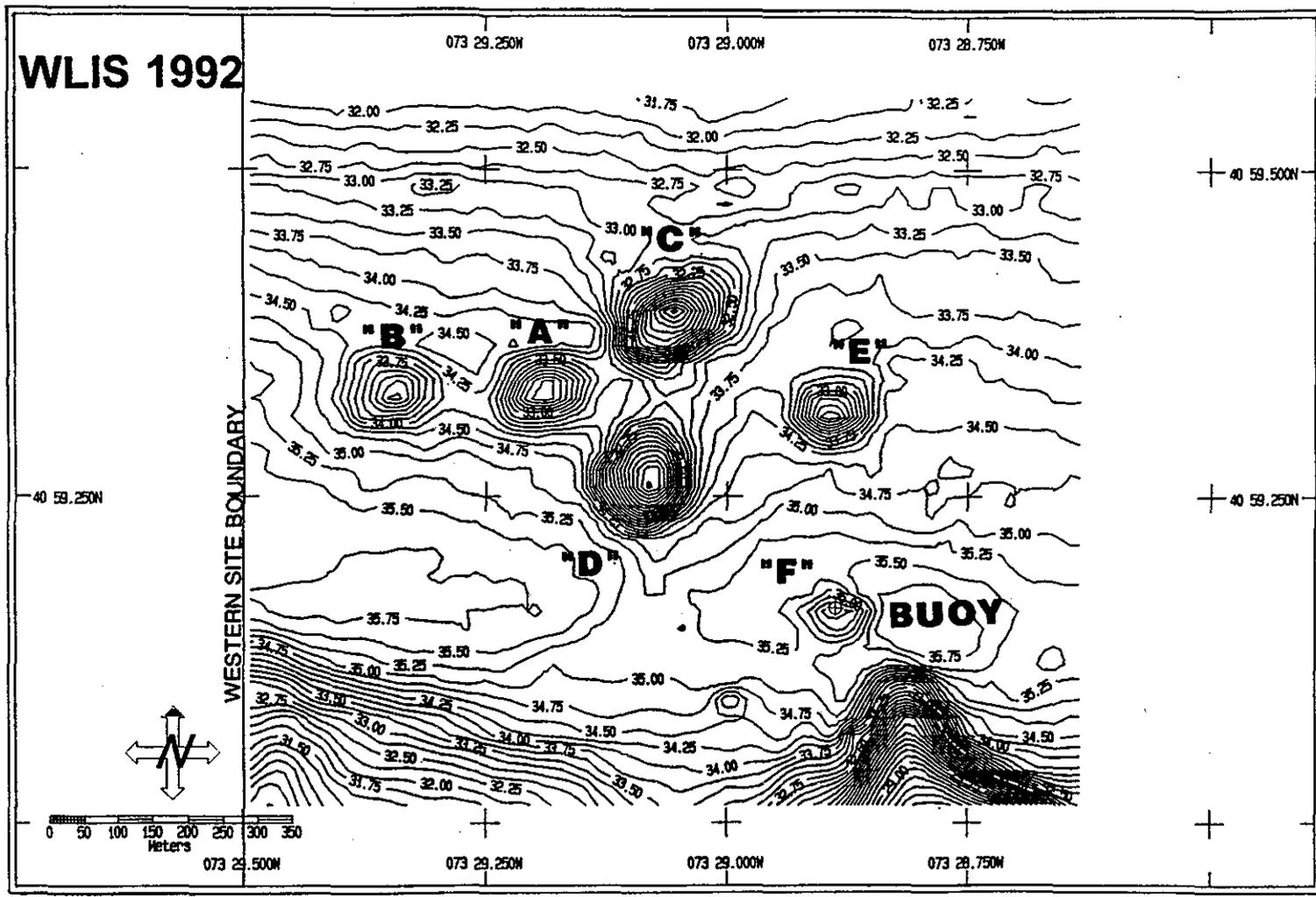
Figure 3-4. Bathymetric contour plot from the 1992 WLIS survey (not corrected to prior survey)
