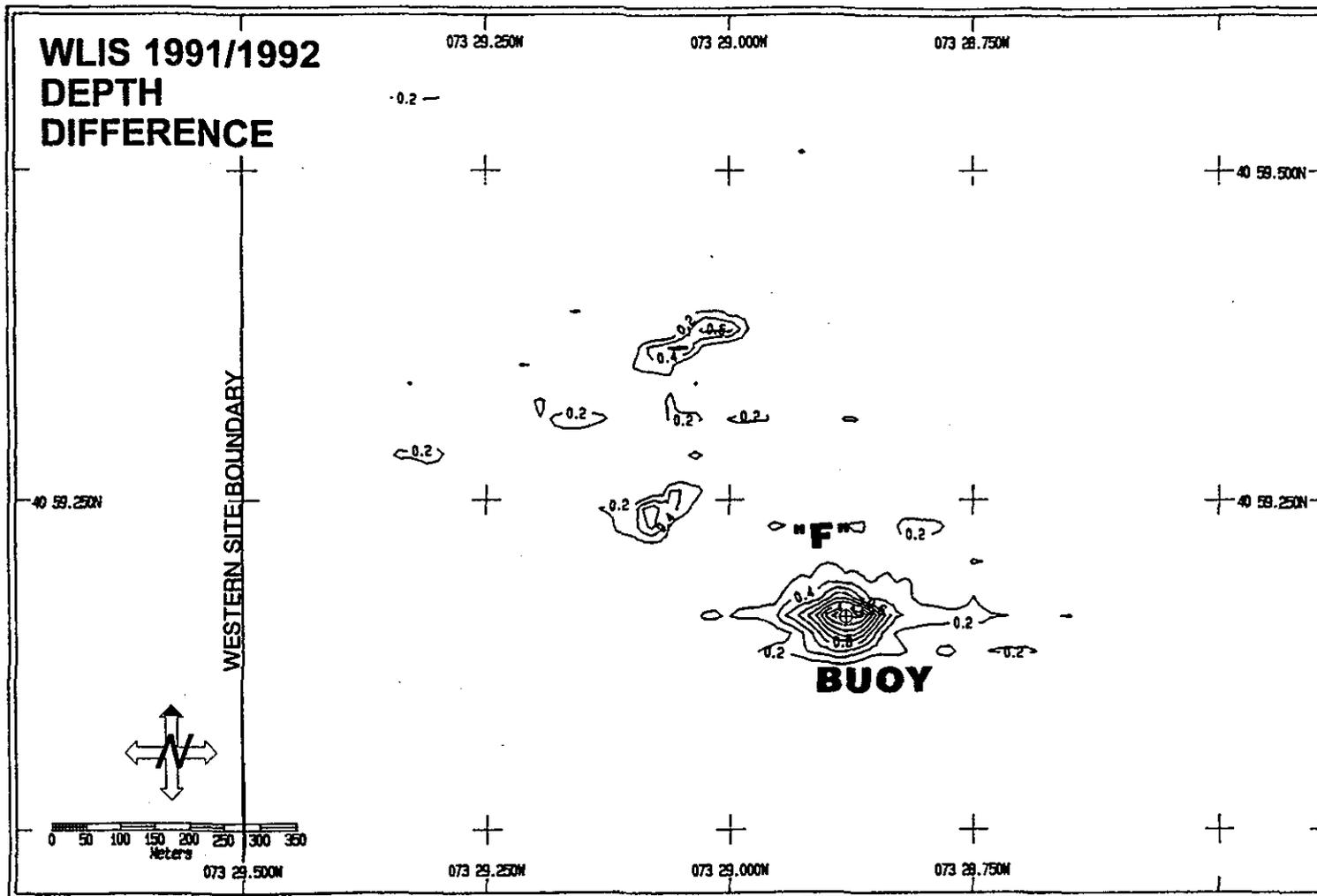
Figure 3-6. Depth difference plot for 1992 and 1991 surveys
