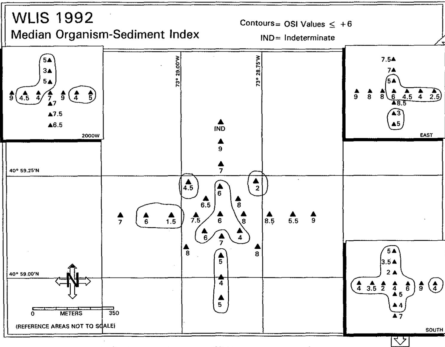
Figure 3-22. Mapped distribution of OSI values at WLIS and reference stations
