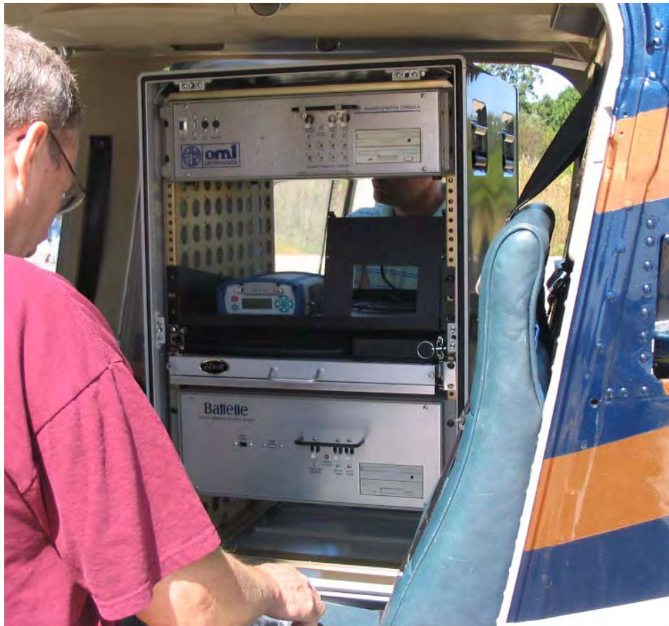
Figure 1-3: Rack-mount components inside the helicopter for the VG-22 system. These include the recording console, an extendable flat screen monitor, extendable keyboard and mouse shelf for navigation system, and the navigation system with CRT display and the GPS positioning console.
