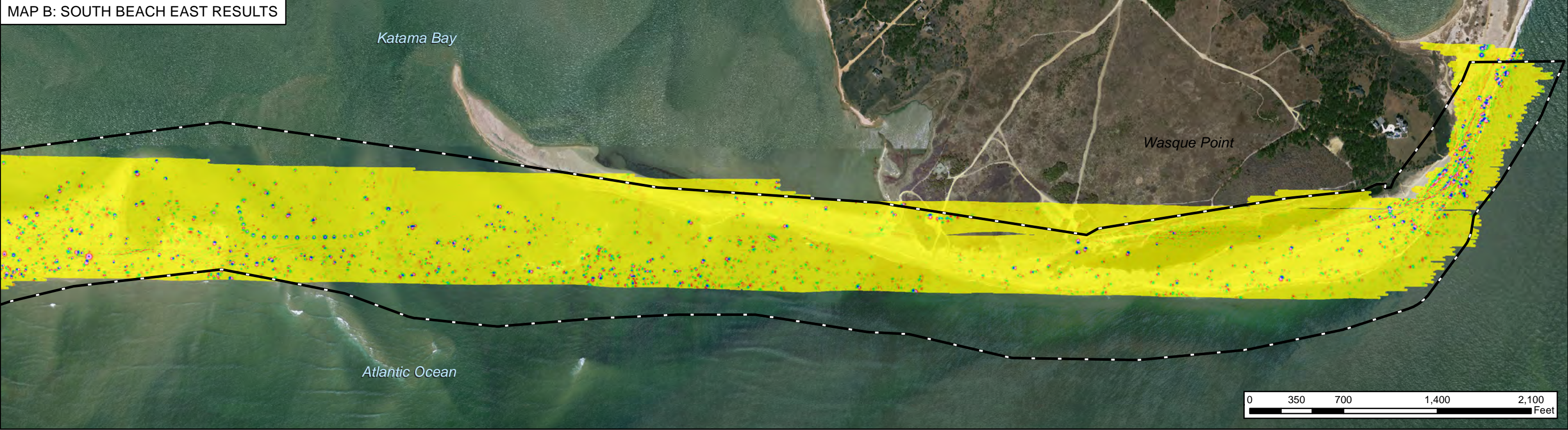
FIGURE 5-1 Air Magnetometer Results - Former Moving Target Machine Gun Range at South Beach Investigation Area, Martha's Vineyard, MA
