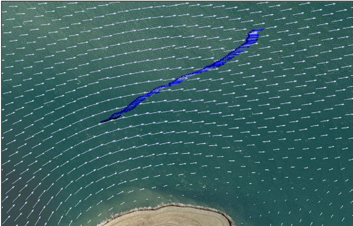
Figure 30. Boat ADCP data Transect 3 02/08/05 20:12 compared to model data at 20:00
