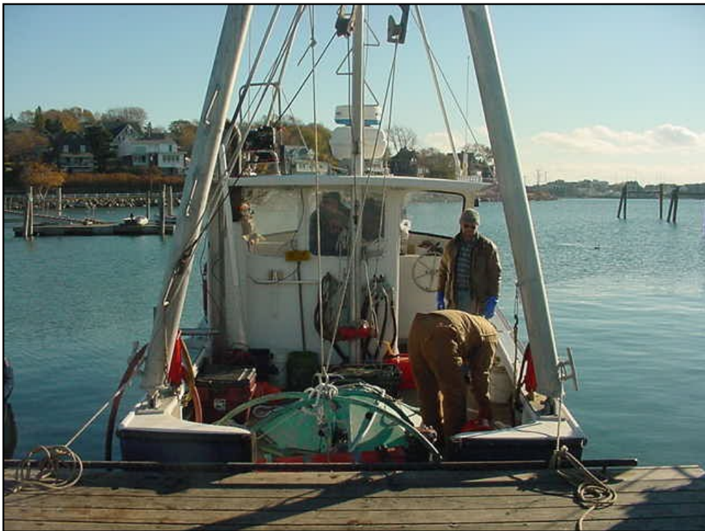
Figure 11. A-frame on Sakonnet used to deploy current-meter moorings.
