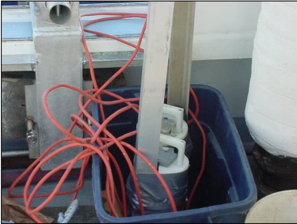
Figure 7. Water-level gage mounted on angle iron.
