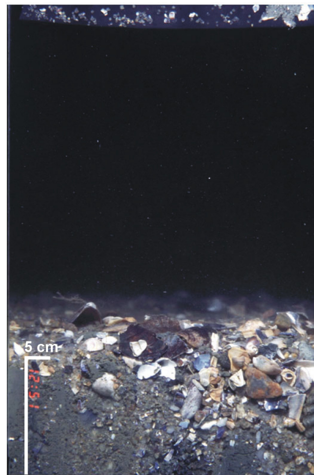
Figure 3-25. Two REMOTS ® images collected from Station M19-5 illustrating a grain size major mode of 2 to 1 phi sand, mixed with larger (1 phi) sand and shell. The relatively shallow penetration of the REMOTS ® camera prism suggests that the sand is relatively compact
