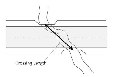
For calculating openness length is measured as a straight line connecting the channel midpoint where it enters a structure and where it exits the structure.
