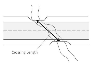
For calculating openness length is measured as a straight line connecting the channel midpoint where it enters a structure and where it exits the structure.
