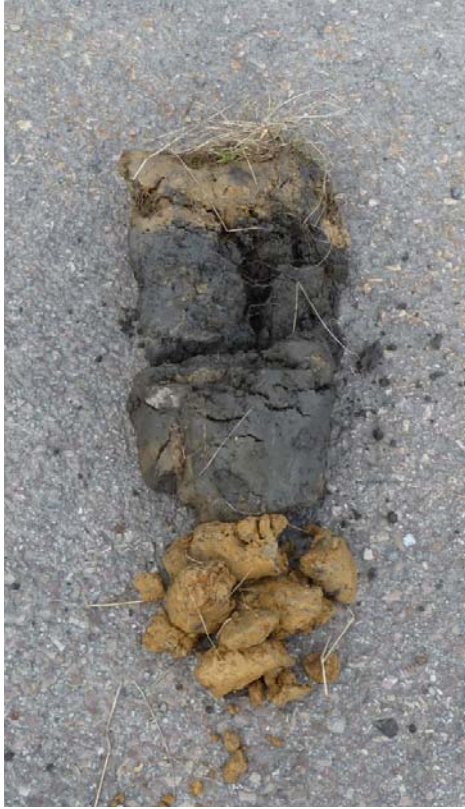
Photo 33. GT1. Soil from restored R.O.W. Topsoil was clearly buried.
