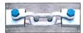
TYPICAL FLOATING BARRIER CONNECTION DETAIL SCALE: N.T.S.
