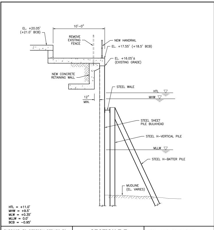
PURPOSE: TO PERFORM REPAIRS TO SHORELINE STRUCTURES INCLUDING BULKHEAD AND RIP RAP
