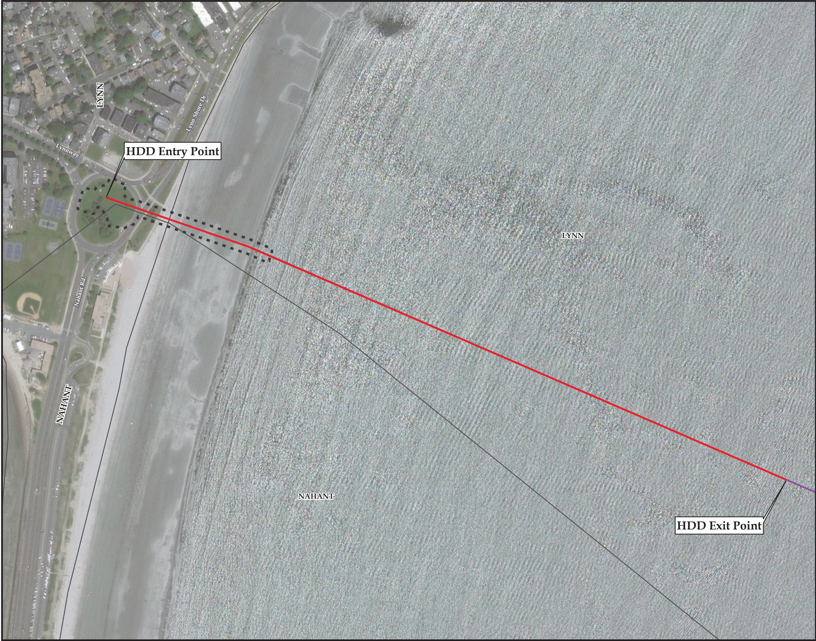
Figure 1: Horizontal Directional Drill Path and Temporary Workspace Amitié Submarine Cable System Lynn, MA September 2020
