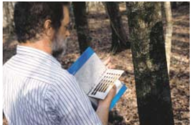
Wetland Delineator uses soil color chart to make a wetland determination
