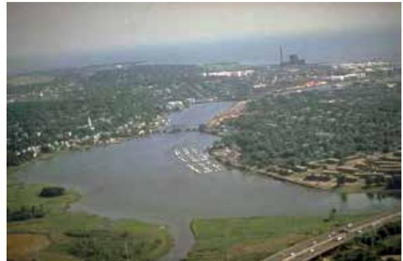
The proposed project consists of deepening the main ship channel, maneuvering area, and turning basin to - 40 feet mean lower low water (MLLW) and widening the main channel and turning basin to allow larger vessels to efficiently access the port of New Haven's terminals.
