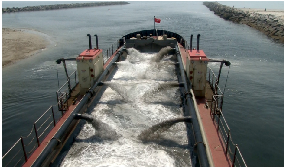
The Currituck pumps dredged material into its hull.
