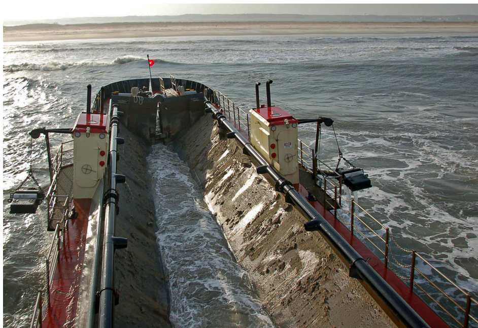
The hull of the Currituck splits and releases dredged material at a designated disposal site.
