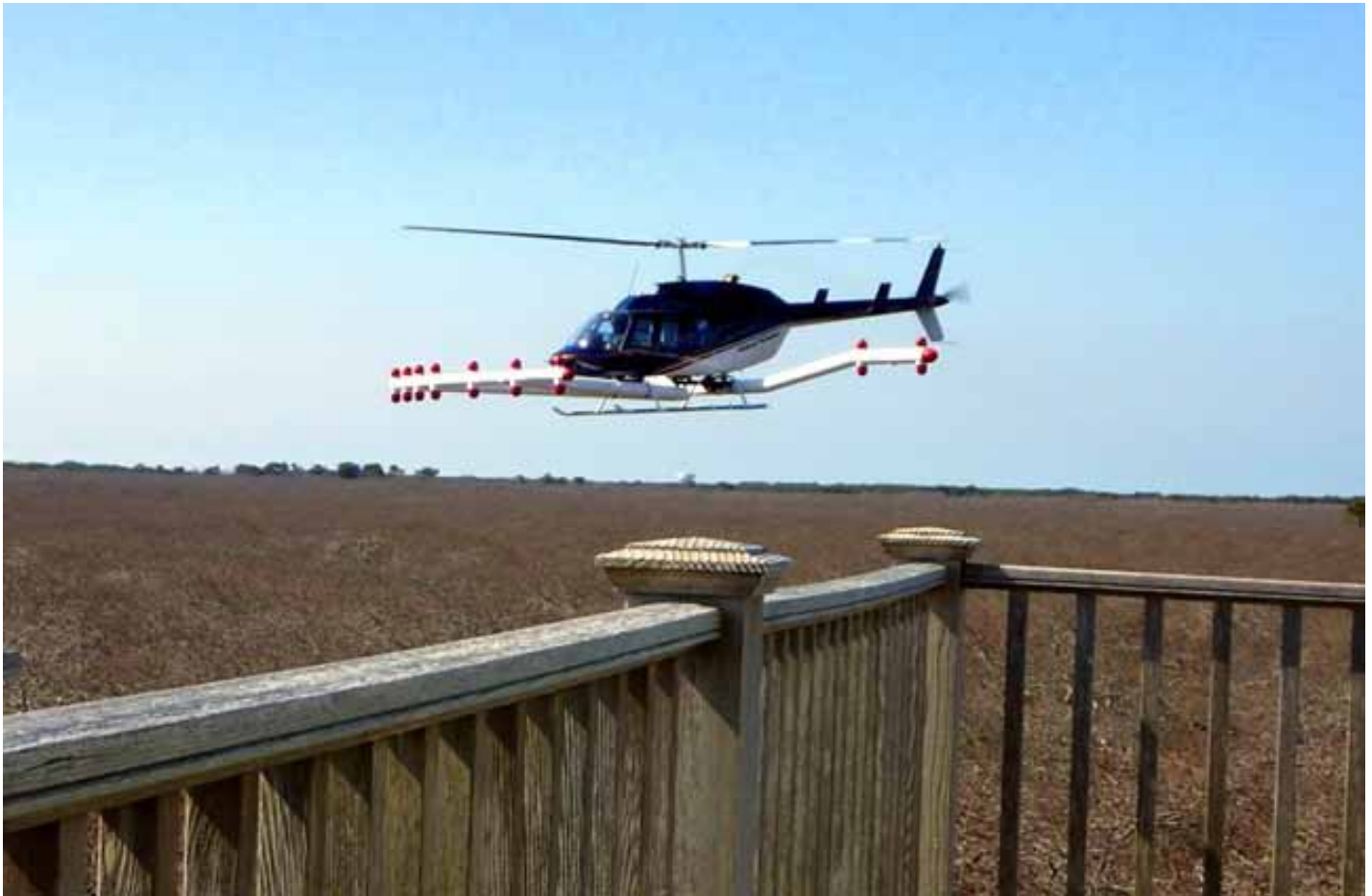
A helicopter flies over Nantucket, Mass., to conduct an aerial geophysical survey.
