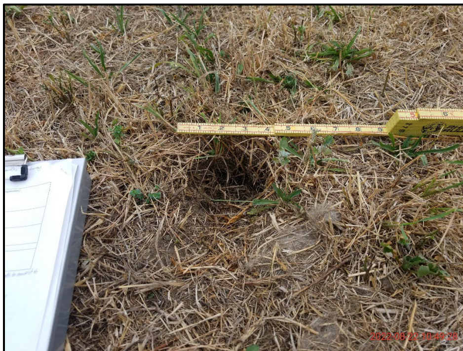
Photograph 9. One of two small relic burrows identified on the soil cap. (22 August 2022).
