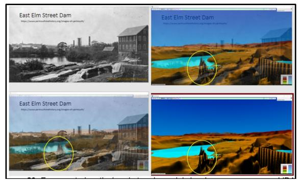
Figure 37: Exaggerated vertical scale terrain model showing some erroneous LiDAR points near Gooch Island (yellow circle)
