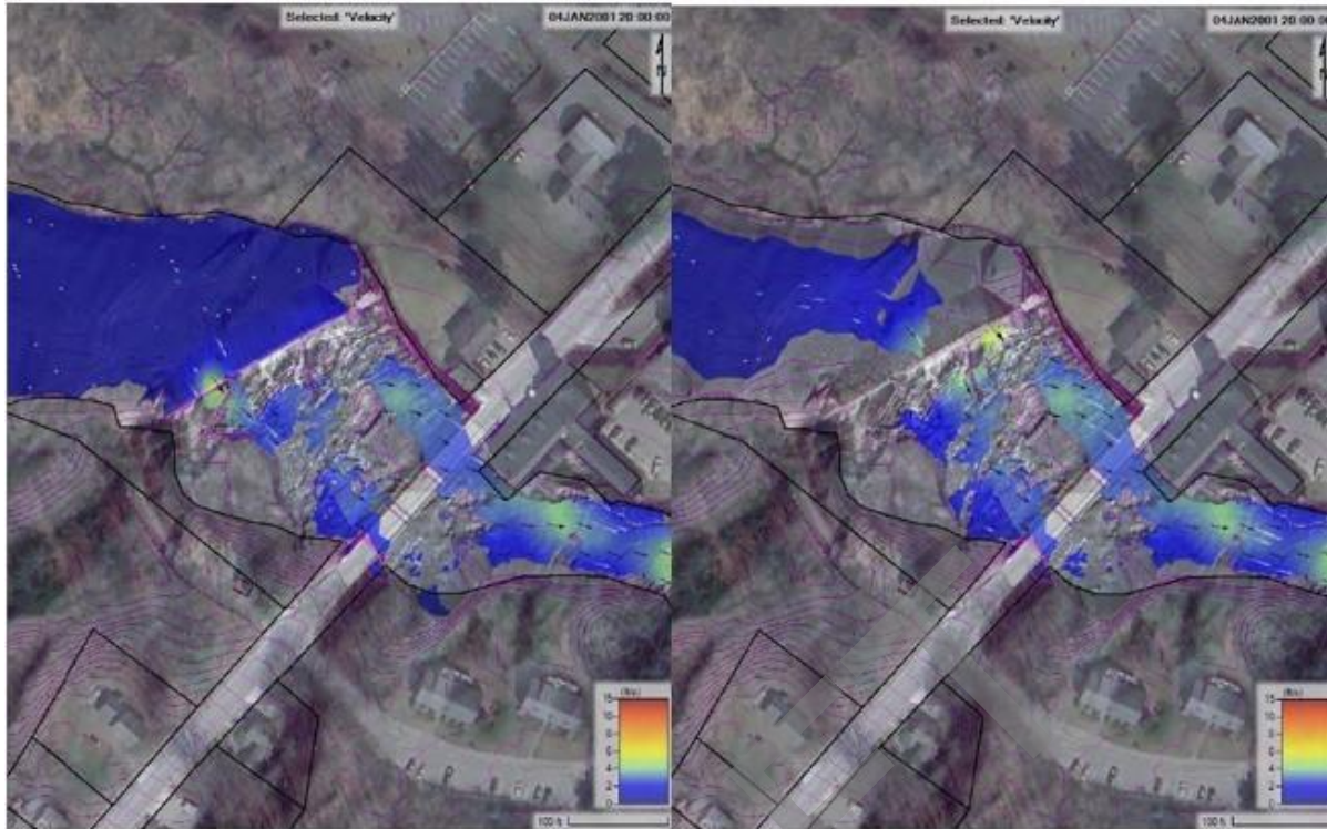
Figure 3. Side-by-side comparison of velocity and inundation before and after dam removal at Bridge Street dam.
