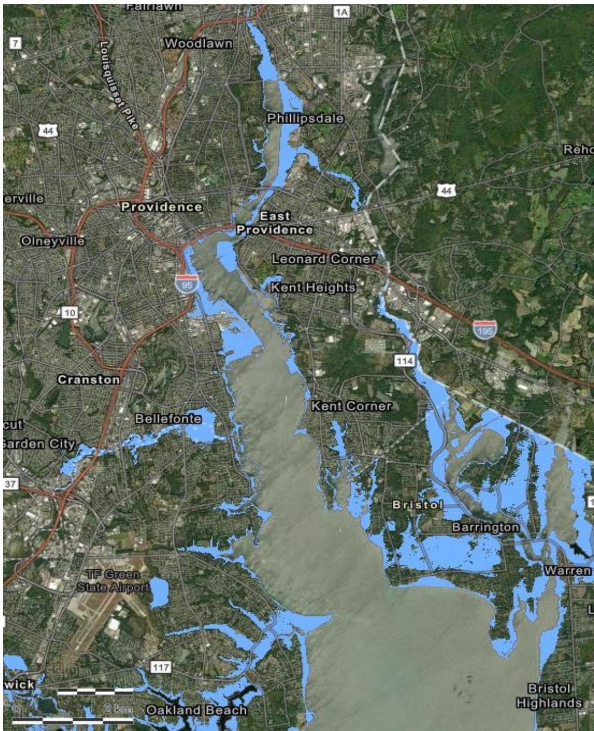
**Figure B 8-3:** 2080 1-percent AEP inundation under intermediate SLC—Warwick, Cranston, Providence, Pawtucket, East Providence, Barrington, Warren
