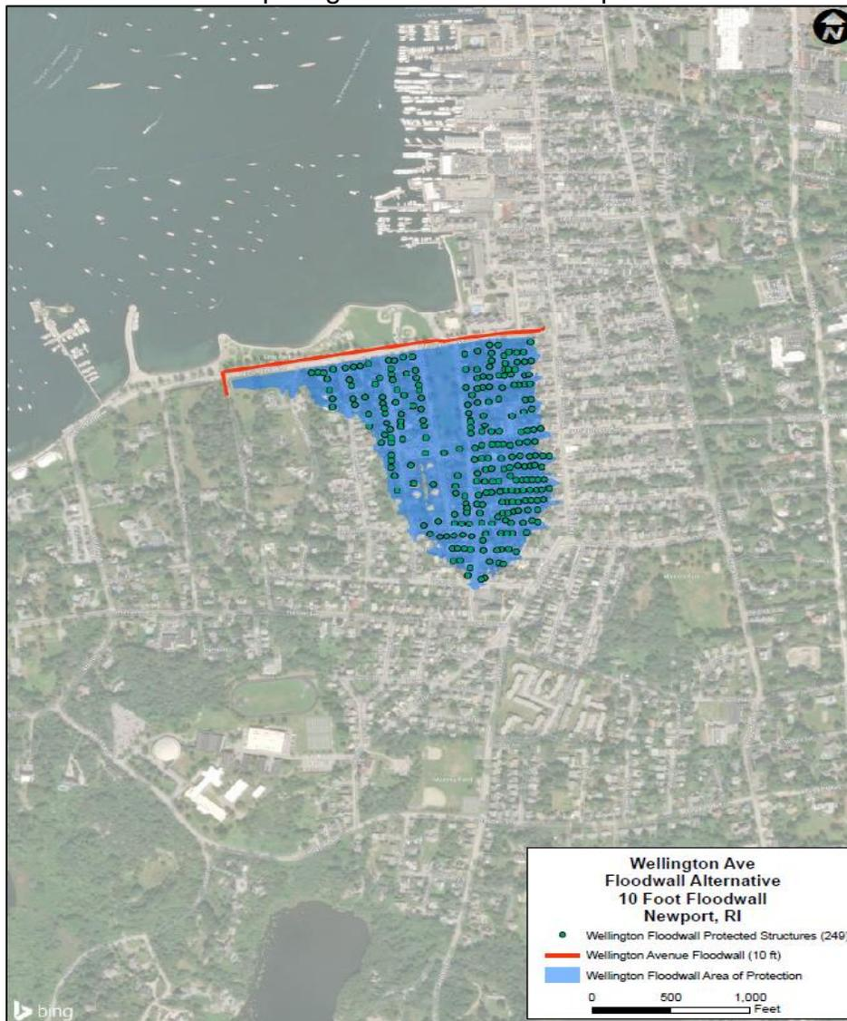
**Figure B 8-10:** Wellington floodwall and levee alignment with area of risk reduction
