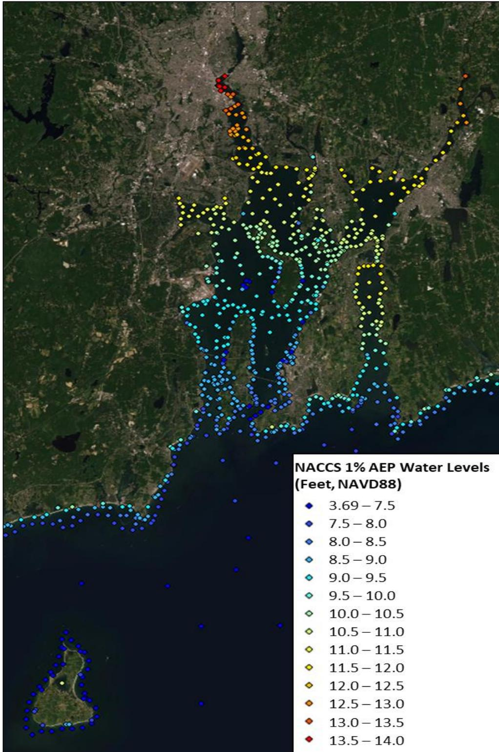
**Figure B 5-3:** NACCS 1-percent AEP water levels in feet, NAVD88
