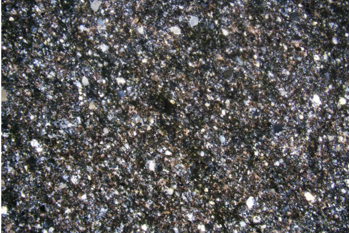
FD16-07, Phyllite 9OW_002.jpg/PPL/FOV = 4.00 x 5.83 mm ALTERED CHLORITE-KFELDSPAR-QUARTZ SCHIST showing typical appearance (same view as (9OW_001.jpg).
