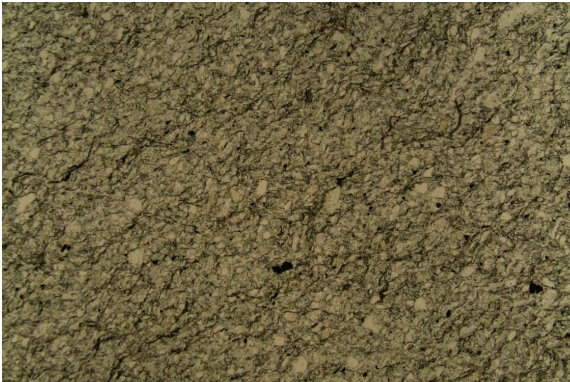
FD16-09,C-1,136.2-140.2 ft 9OW_010.jpg/PPL/FOV = 4.00 x 5.83 mm ALTERED CARBONATE-SERICITE-QUARTZ SCHIST showing typical appearance (same view as 9OW_009.jpg).
