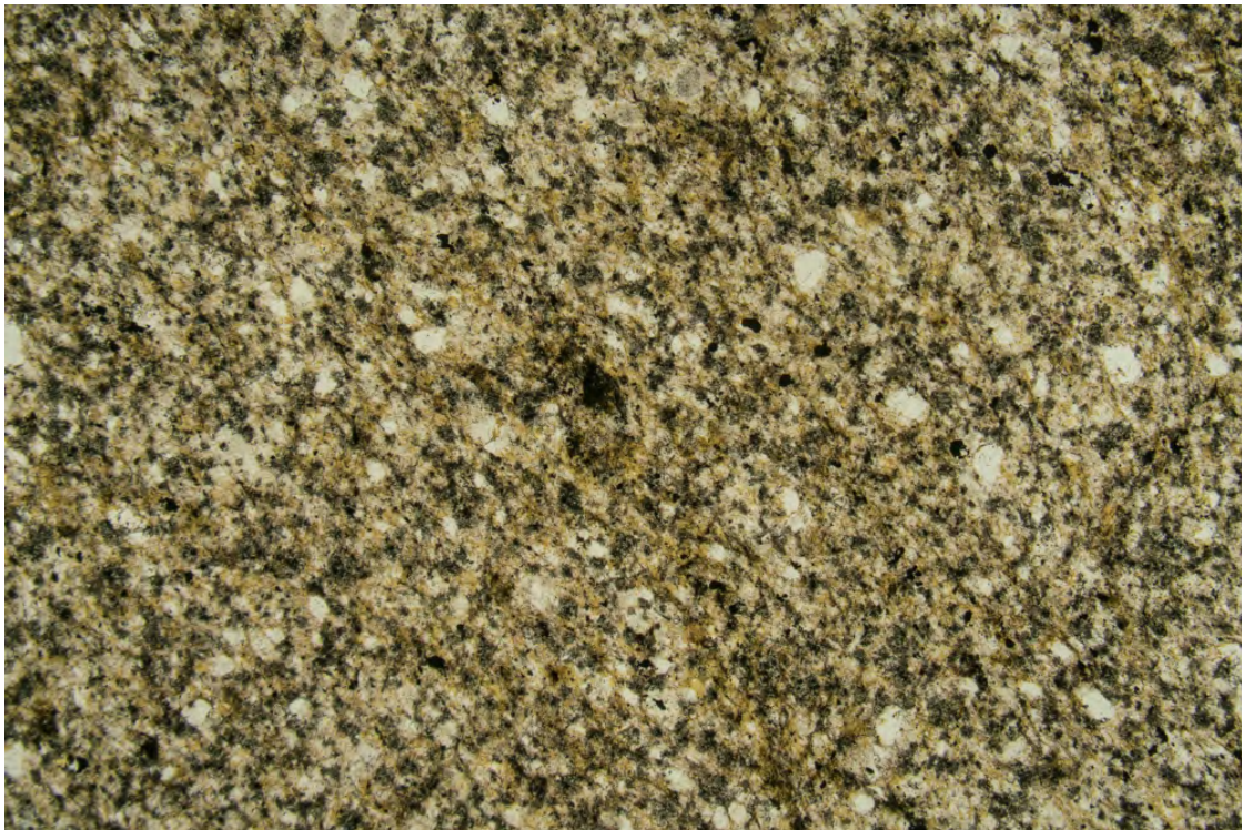
FD16-07, Phyllite 9OW_002.jpg/PPL/FOV = 4.00 x 5.83 mm ALTERED CHLORITE-KFELDSPAR-QUARTZ SCHIST showing typical appearance (same view as (9OW_001.jpg).
