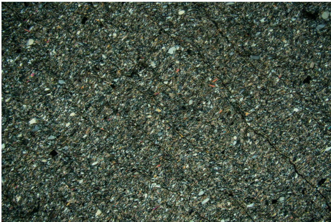
FD16-01, C-1 9OW_006.jpg/PPL/FOV = 4.00 x 5.83 mm ALTERED CARBONATE-SERICITE-QUARTZ SCHIST showing typical appearance (same view as 9OW_005.jpg).
