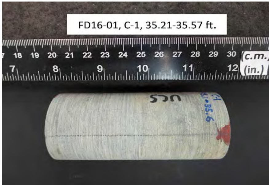
After cutting and grinding
