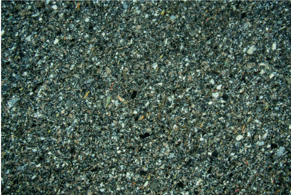
FD16-09,C-1,136.2-140.2 ft 9OW_010.jpg/PPL/FOV = 4.00 x 5.83 mm ALTERED CARBONATE-SERICITE-QUARTZ SCHIST showing typical appearance (same view as 9OW_009.jpg).
