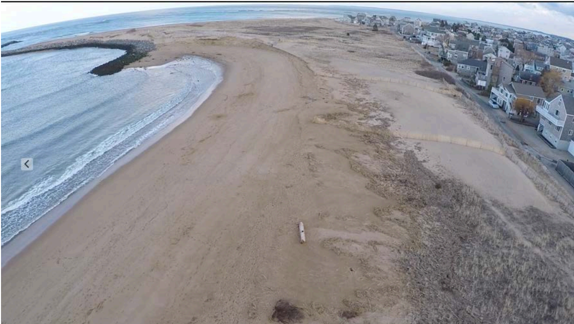
Figure 2. Overview photo showing loss of dune, fence, and the importance of DCR's sand additions that formed a protective barrier stopping tidal surge from the late January storm. Note the extent of wrack deep into the dune system, stopping at the foot of the dune nourishment. (Photo date: January 27, 2017.)
