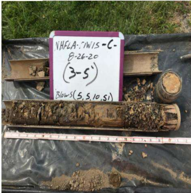
Split-spoon sample collected from MW15
