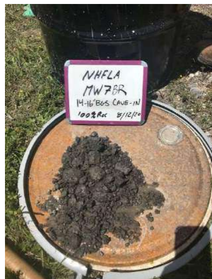
MW7BR 14-16' bgs cave in. Top of competent rock is heavily fractured.
