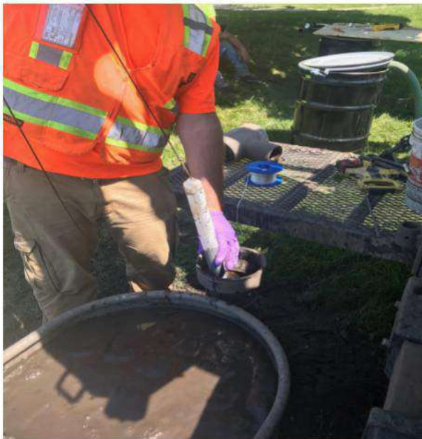
Bailing water out of borehole to confirm recharging capabilities of competent bedrock at MW5BR.
