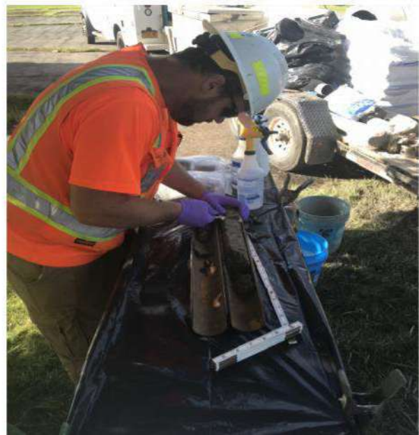
Soil characterization of split-spoon sample at MW5OB
