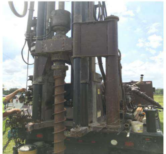
Auguring to below ground surface at MW10
