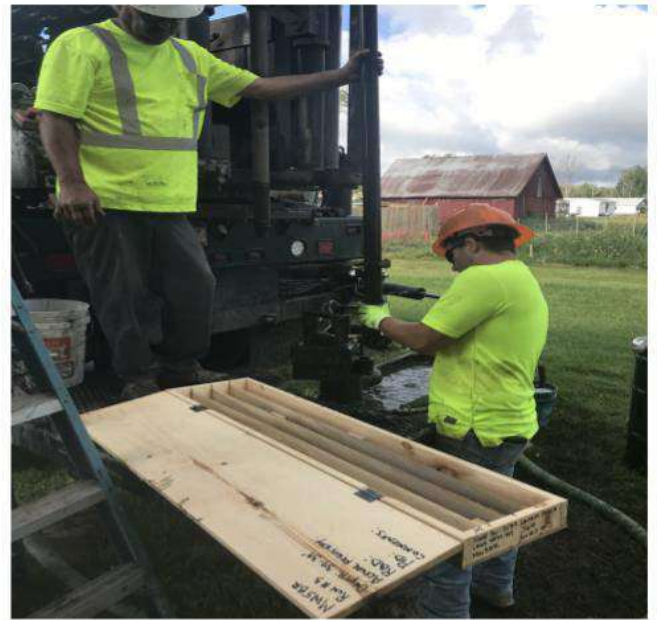
Bedrock core extraction at MW5BR
