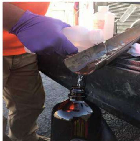
Equipment blank collection from split-spoon (Vehicle was not running)
