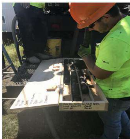
Rock core retrieval (Run#1) at MW1BR
