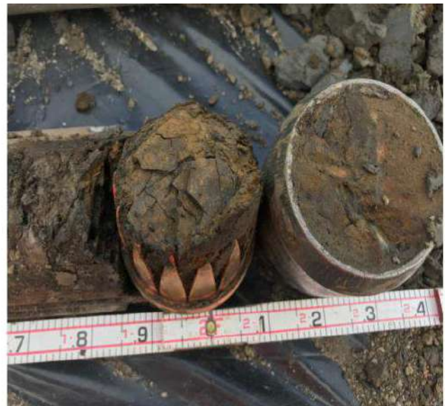
Fractured bedrock in split-spoon sample
