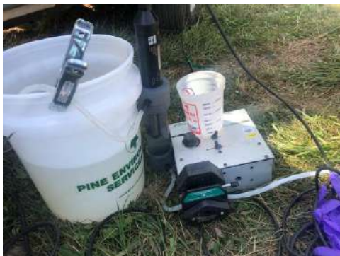
Example sampling set-up with peristaltic pump and YSI
