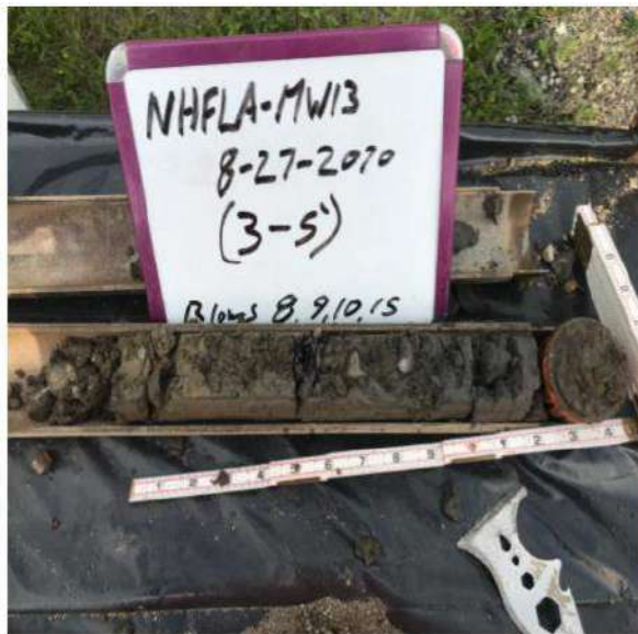
Split-spoon sample retrieval at MW13
