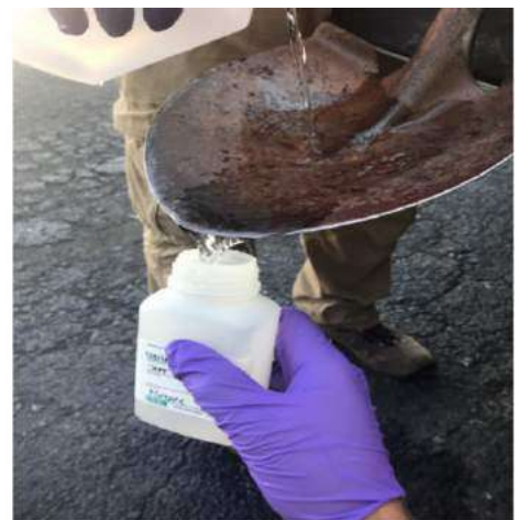
Equipment blank sample collection from shovel used to collect surface sample at MW16.
