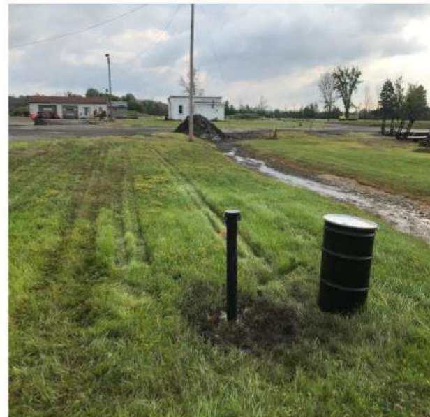
Well completion at MW13 with protective stick-up casing. Includes labeled non-hazardous investigation derived waste drum for soil cuttings.
