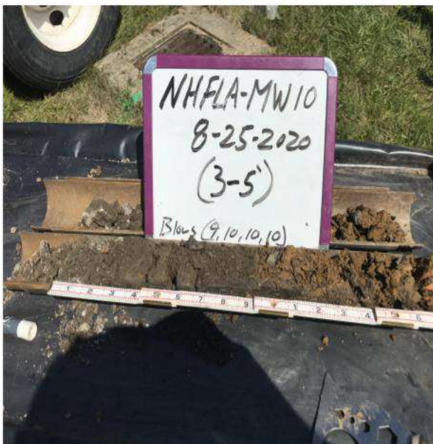
Split-spoon sample collected from MW10
