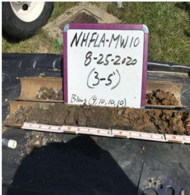
Split-spoon sample collected from MW10
