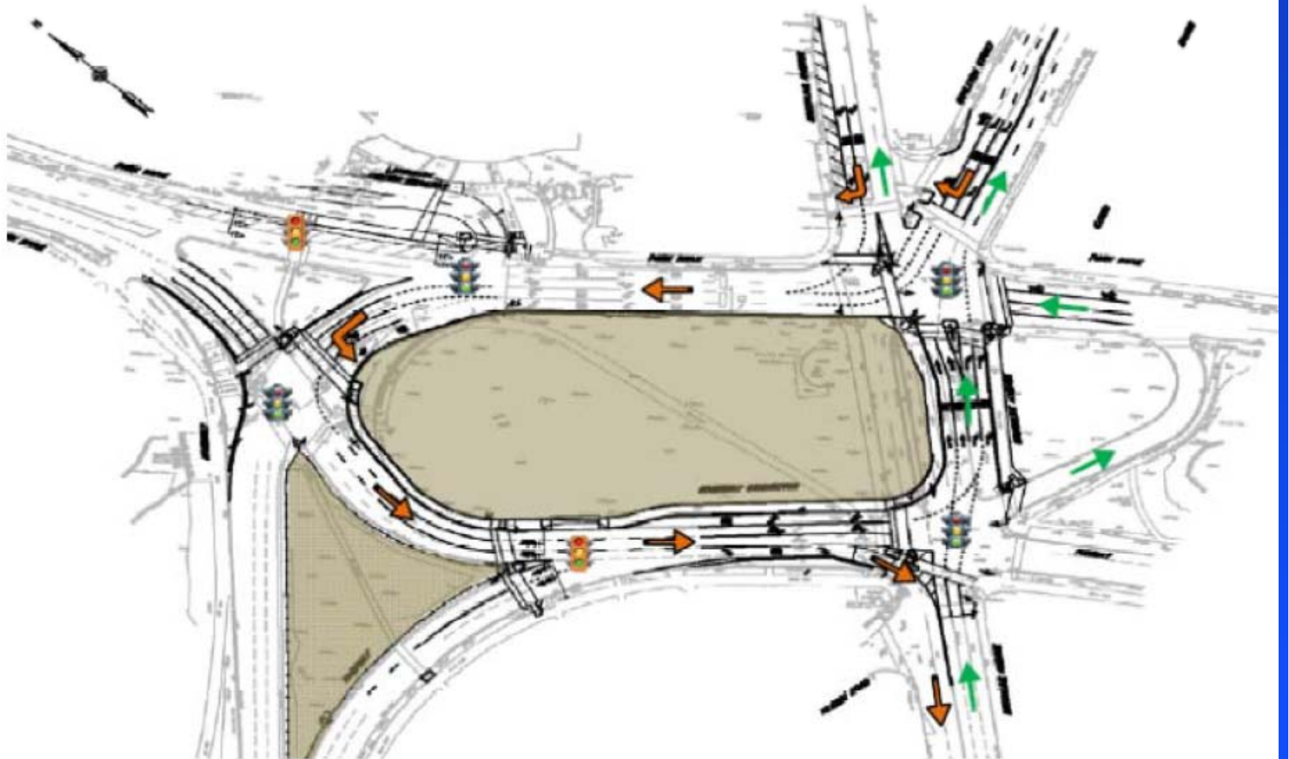
TRAFFIC MANAGEMENT DURING INITIAL BROOKLINE AVENUE CULVERT INSTALLATION
