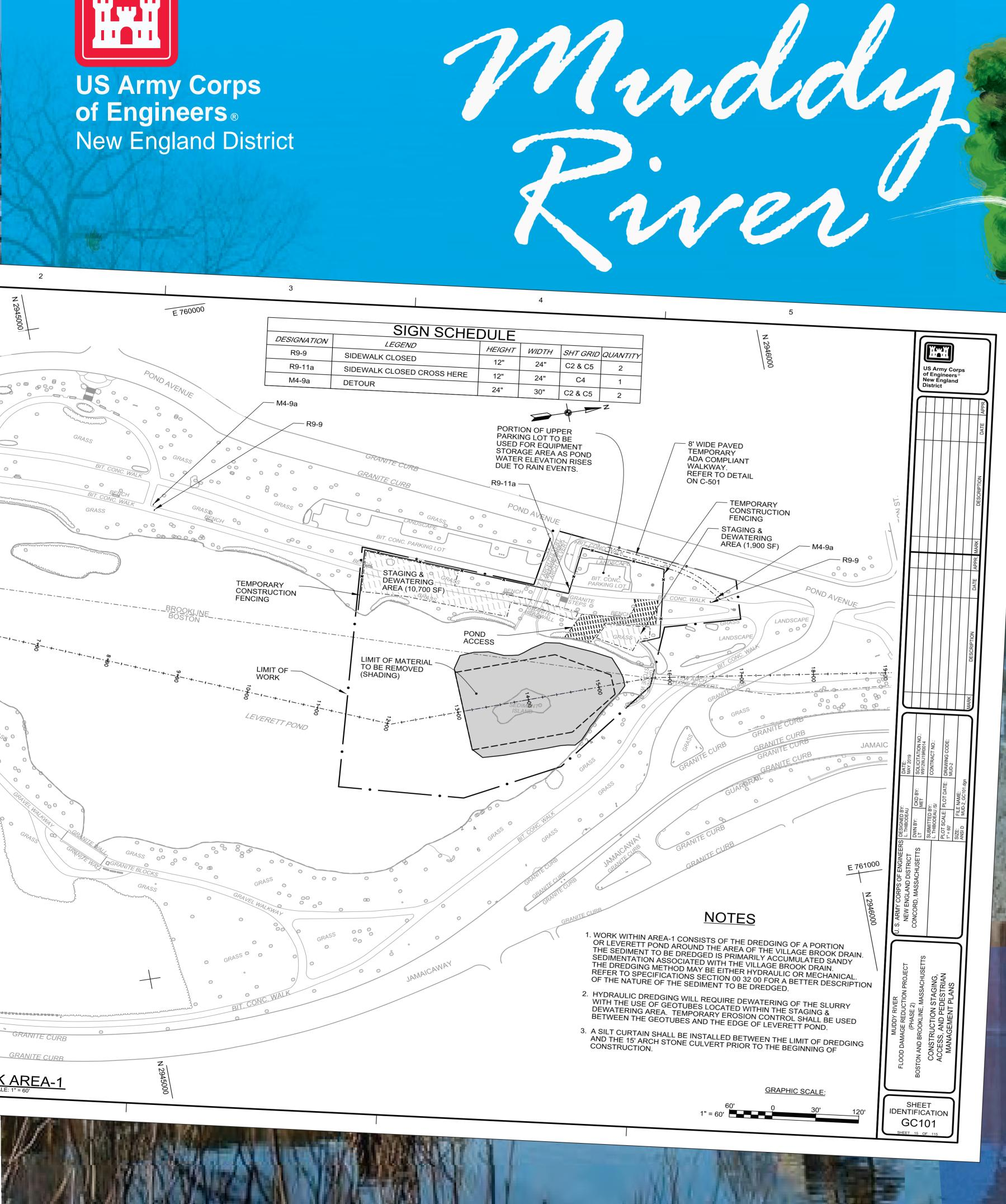
Leverett Pond – work consists of excavating the sandbar and island at Leverett Pond and dredging this area to Elevation -5'. The flood risk management channel varies from 120' to 30' at the outlet.
