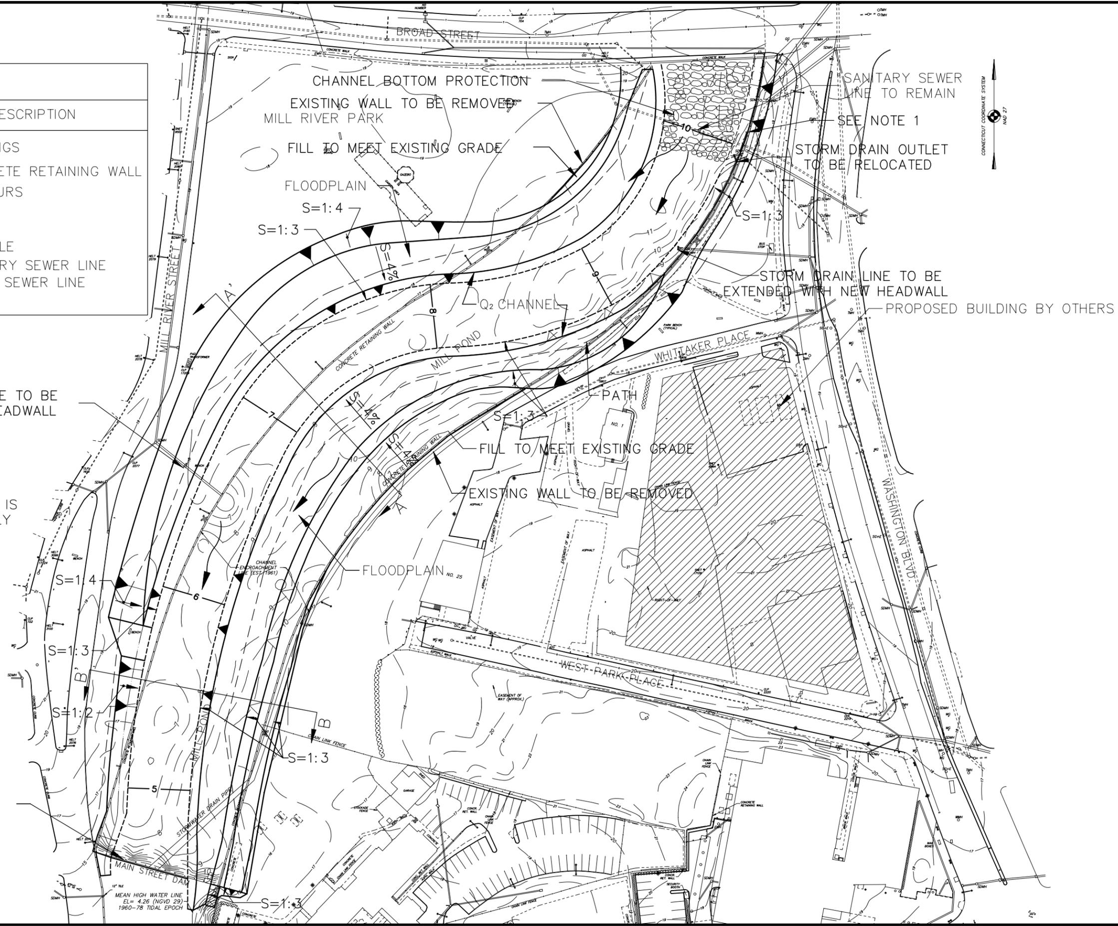
STORM DRAIN LINE TO BE MODIFIED WITH NEW HEADWALL
