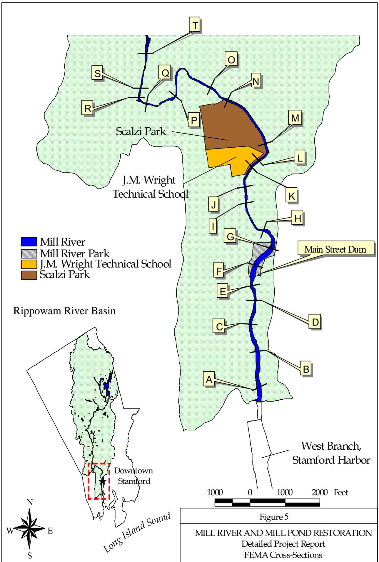
FIGURE 5: FEMA Cross-Section locations within the Project Area.
