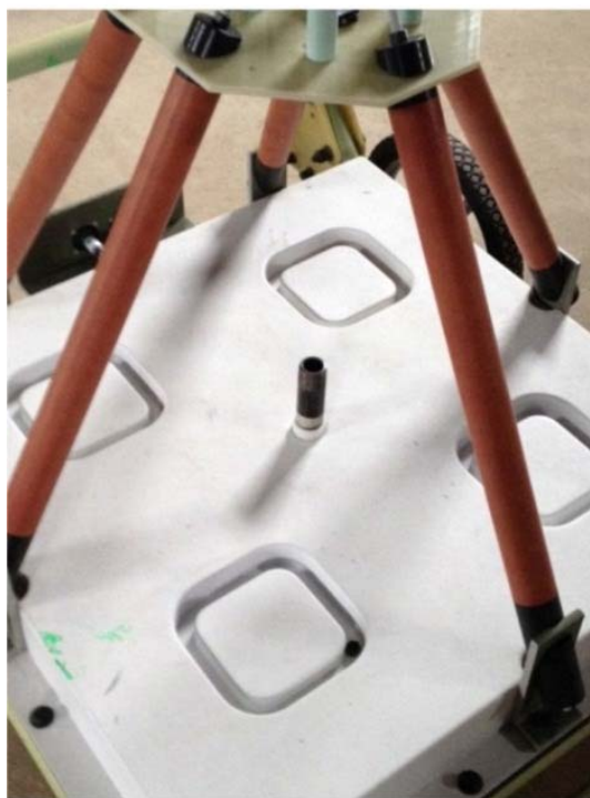
Figure 6 , left panel – photograph of the standardized test object on the TEMTADS sensor. Right panel – screen snapshots of the data logger
