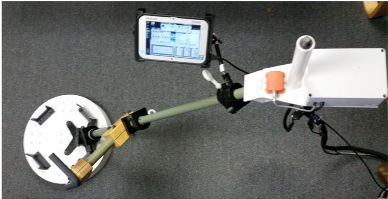
Figure 1. Photo of MPV sensor with attached boom for dynamic data collection.
