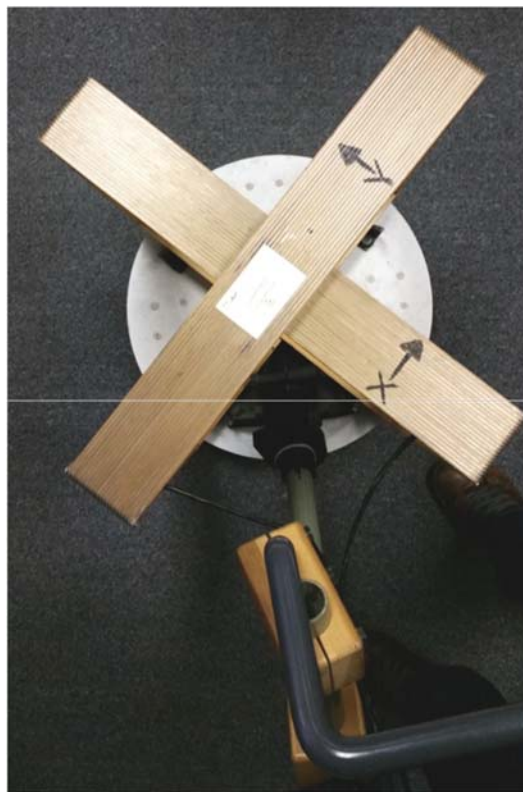
Figure 2. Top view of the MPV sensor with pair of orthogonal horizontal axis transmitter coils for cued data collection.
