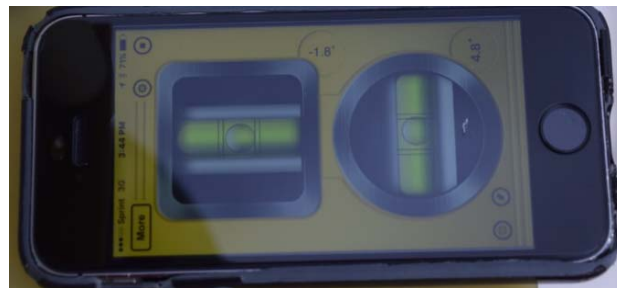
Figure 4. Cell phone running SPIRIT Level, an independent measurement of sensor roll and pitch, to guard against materially significant bias in the IMU sensor.
