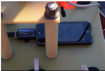
Figure 4. Cell phone running SPIRIT Level, an independent measurement of sensor roll and pitch, to guard against materially significant bias in the IMU sensor.
