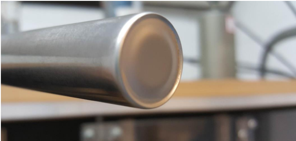
Condition: poor; heavy pitting, replace horn.
